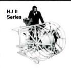
Motorized Take-Up and Pay-Out machinery for reeling and coiling operations with models with reel capacities from 20" to 96", weight capacities from 2,000 lbs. to 10,000 lbs. 12 drive options, hydraulic jack to life reel – standard.
