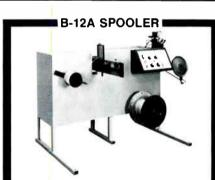
HIGH SPEED SMALL MATERIAL SPOOLERS Level wind – up to 3/8" material; 1 HP variable speed motor; control panel; predetermined stop-to-length counter; run and stop tension controls.
