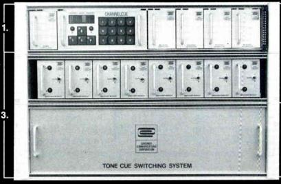
2. Expanded Basic unit provides time switching for up to eight channels with 2,552 switch functions.
