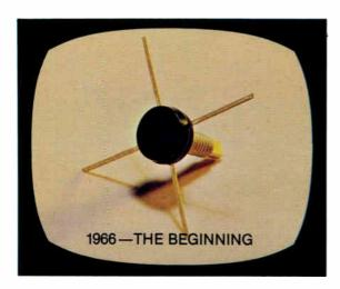
First transistors made and characterized especially for CATV amplifiers.
