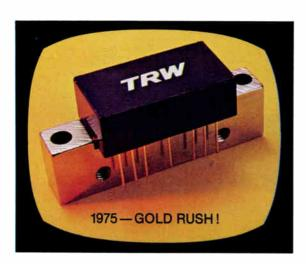
First hybrids with all gold systems, the optimum for ruggedness and reliability. Gold die with ballasting resistors and fine geometry has dramatically improved the performance.
