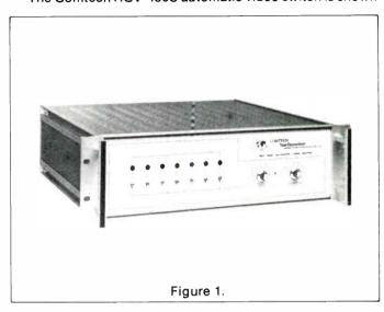
in figure 1. It provides automatic substitution of our RCV-450A receiver for one of up to six on-line receivers on either polarization, should they fail. If our RCV-450F (fixed tuned), or RCV-450A receivers are used as the on-line units they include fault detection of (a) out-of-range power supply voltage, (b) video signal presence, and (c) audio signal presence. These three functions are combined into a
