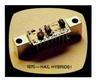
First hybrids for CATV. Elimination of interconnects provides inherent increase in reliability, ease of field repairs. Improved performance over discrete amplifiers.
