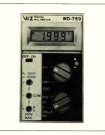
The units also provide for measurement of either high or low power ohms in all ranges—switch selectable. This assures accurate readings when making measurements either in or out of circuits.
