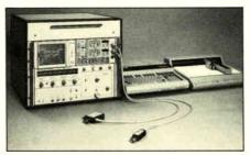
The 5610 makes measurements without interruption. Because the sweeper, SWR Autotester, Detector and programming all cover the 10 MHz to 18 GHz range, it is unnecessary to halt tests to change plug-ins or measurement components. The operator's role is limited to selecting the test parameters, connecting the test device, initiating the test sequence.
