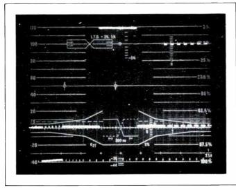
Figure 1. Output of a demodulator with a zero chop pulse generated during the vertical interval.
