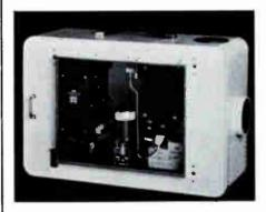
One of the company's newest products was the 60594 earth station video receive equipment—a compact, solid state weather protected downconverter. This downconverter is designed for direct mounting on earth station antenna to convert incoming satellite signals in the 11.7 — 12.2 GHz range to a 70 MHz IF output. The 70 MHz output connects to the optional baseband treatment equipment with up to 500 feet of low cost coaxial cable, without
