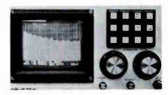
night. In addition to reliable performance, the system offers the following standard features: minimum frontpanel controls, digital storage and refreshed display, alphanumeric readout and a battery-saver. The Wavetek processed system also incorporates a sweep transmitter and a sweep analyzer.
