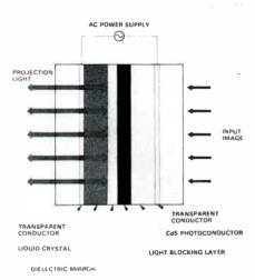
Pictured above is a diagram of the hybrid field effect on the liquid crystal light valve.
