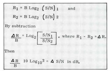
is the relation between excess channel capacity expressed as bit rate and available noise margin expressed as S/N in dB.
