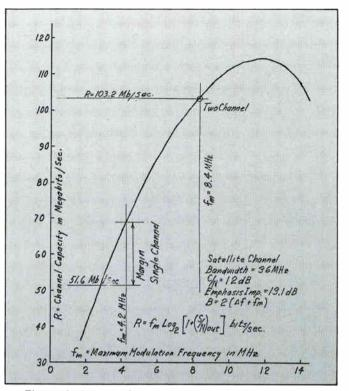
Figure 3. Information rate vs. modulation frequency
