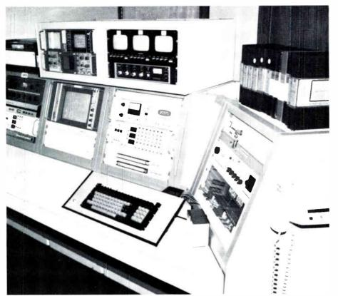
This three-channel airing facility console incorporates a color monitor. vectorscope. wave form monitor and time base correctors.
