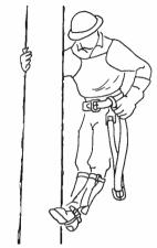
Figure 9: Releasing the safety strap
