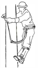
Figure 10: Passing the safety strap to the right hand
