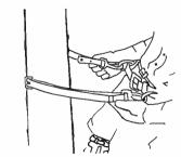
Figure 3: Position of the safety strap when in use
