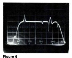
Vertical—10 dB/cm Horizontal—1 MHz/cm RCA CTM—10 modulator, bandpass filter and AML. Video carrier at the 90 MHz line. Tuning marker at the 190 MHz line. Sound trap at the 200 MHz line.
