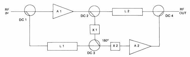
Figure 2 Typical Signal Level Distribution in Feed-Forward Amplifier
