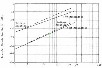
It can be seen that, if the amplifier non-linear distortion is insignificant, the length of an AGC/ASC amplifier cascade may be limited by the amount of transfer modulation that can be tolerated. The use of video carriers as the reference signals aggravates this problem, unless steps are taken, because of the presence of 60 Hz pulses in the video signal.
