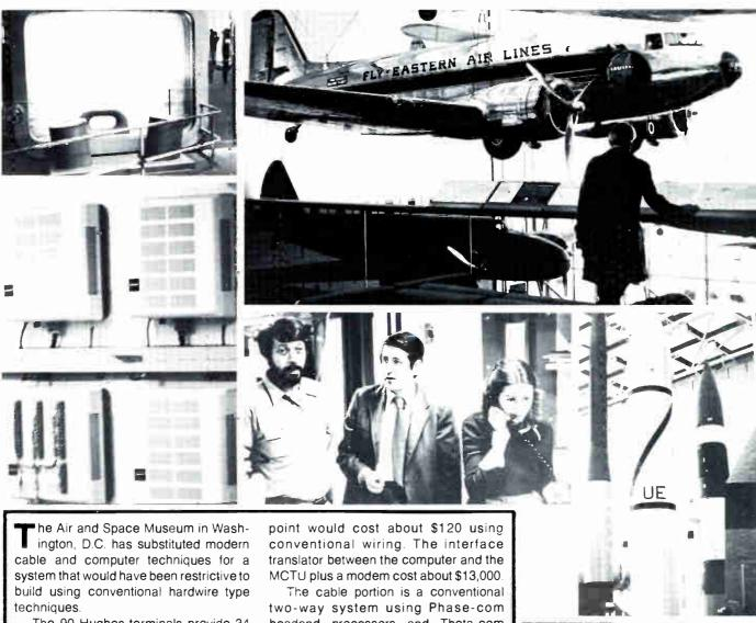
The 90 Hughes terminals provide 34 data points per terminal with 1000 terminal capability per 4 MHz bandwidth on the cable. This means that 34,000 data points could be provided by the present system.
