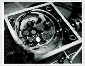
Inside the Bell Northern receiver, the PTN, diode can be seen connected to the end of the optical fiber with the video amplifier included in the same housing.
