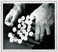
The six strand optical fiber cable can replace up to 20 conventional coax cables.
