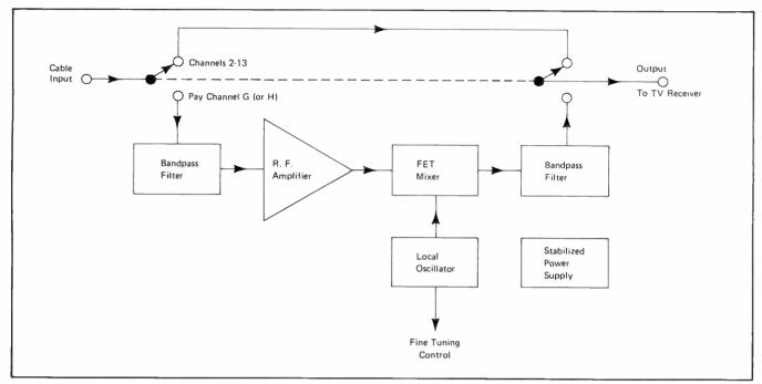
Figure 1. Oak Single Channel Converter Functional Block Diagram
