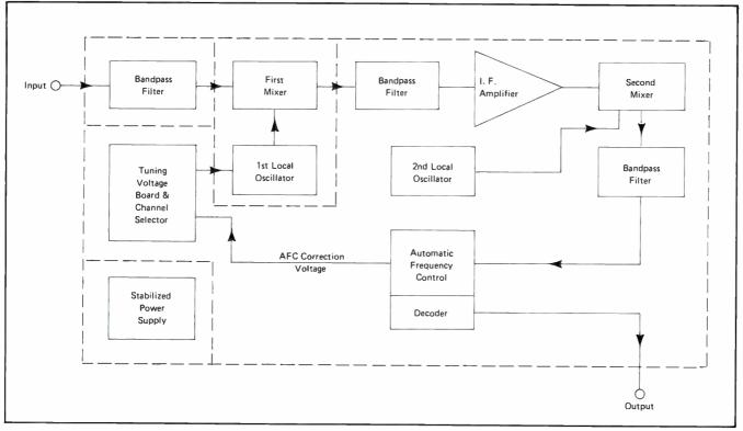
Figure 7. Oak Multi-Code Converter/Decoder Functional Block Diagram
