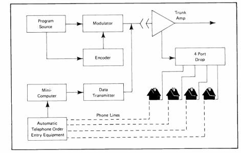
Figure 8. Oak Addresso-Code System Block Diagram
