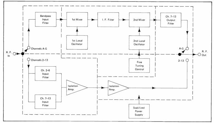
Figure 2. Oak Econobloc Converter Functional Block Diagram
