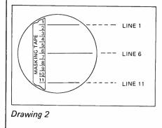
When properly set up, the trace will be on the bottom line (line 11) with no signal and on the top line (line 1) with the signal on. What you are doing here is just voltage measurement. We are taking a 1 volt signal and dividing it into 10 one centimeter segments. Each segment (cm) will now equal 10% of the visual signal level. Leave the signal on.
