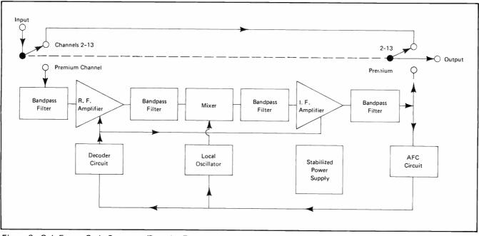
Figure 6. Oak Econo-Code Converter/Decoder Functional Block Diagram
