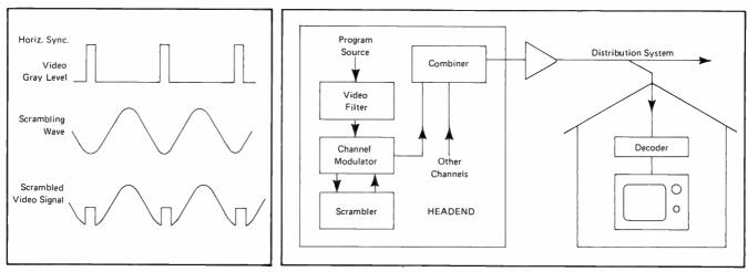
Figure 3. Scrambling Waveforms
