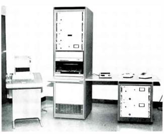
Figure 10. Oak Addresso-Code System Headend Equipment Setup
