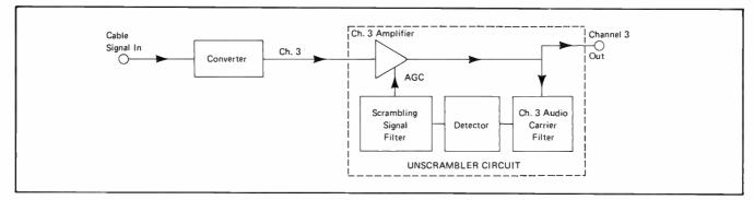
Figure 5. Oak Decoder Block Diagram
