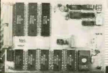
6800 MPU, serial I/O, parallel I/O, RAM, EPROM, 44-pin 4.5" x 6.5" PCB
