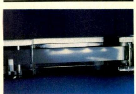
High speed tape without the "edge pressure reduction guide" seldom enters tape guides parallel to the top and bottom. The edge pressure which results creates "scalloping" or "coining" on the tape. The effect is data loss due to head-to-tape separation, flaking media that smears across the head, and "redeposit nodules" that create hard errors.
