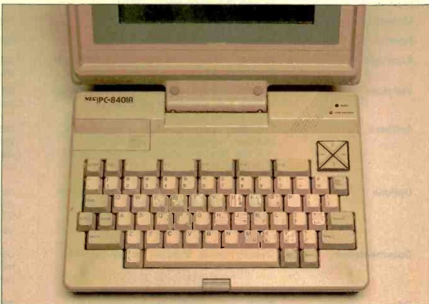
Photo 6: The NEC PC-8401A 68-key keyboard.
