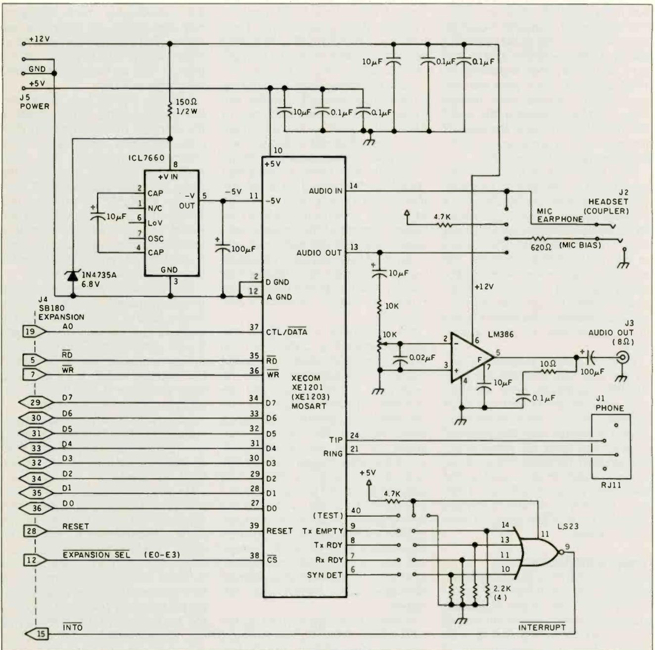
Figure 1: The schematic diagram of the Circuit Cellar COMMI80 modem expansion board.
