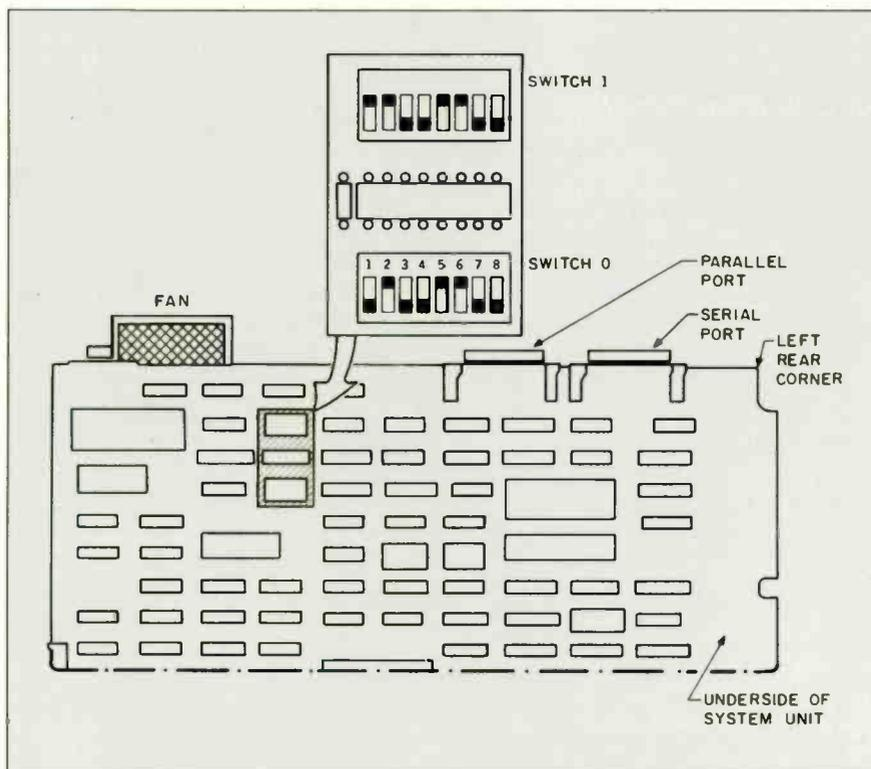
Figure 1: The bottom right corner of the AT&T PC 6300's motherboard, showing the location of DIP switches and switch settings for 640K bytes of RAM.
