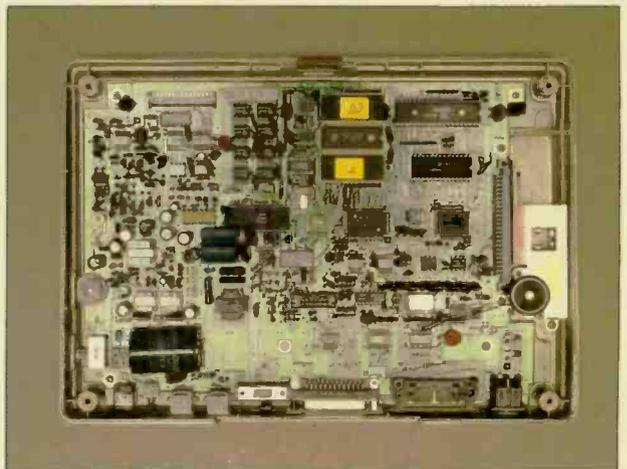
The NEC PC-8401A's internal circuitry.
