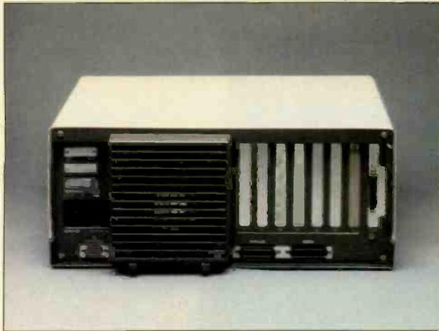
Rear view of the AT&T PC 6300 showing connectors for the serial port, parallel port, keyboard, and monitor. Note the oversize cooling fan, protective shroud, and connector access slots for the seven expansion boards.
