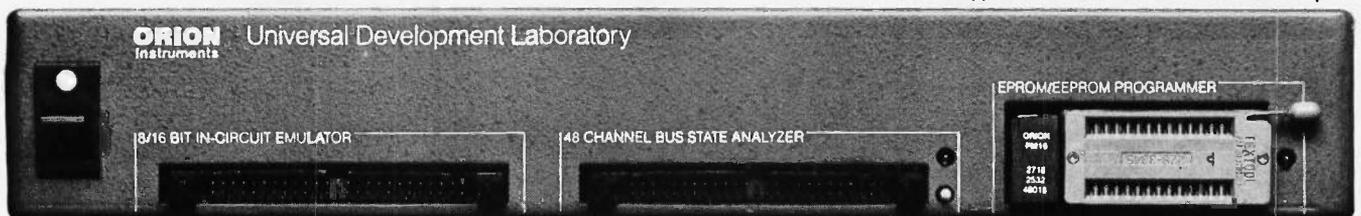
**32K bytes** of EMULATION ROM (128K max) allows you to make program patches instantly. Since the target ROM socket connects data and address lines to both the analyzer and the emulator, no expensive adaptors or personality modules are needed.
