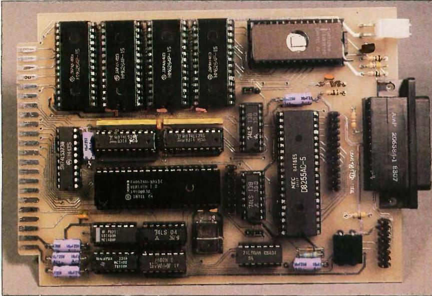
Photo 1: The Circuit Cellar BASIC-52 computer/controller prototype.
