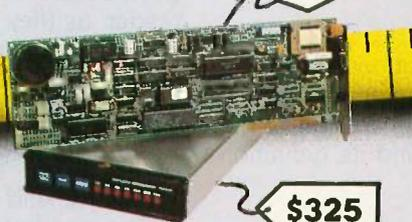
Our modems are fully Hayes compatible with features such as low heat dissipation, low power consumption, software volume control for the speaker, and large-scale-integration "Modem on a chip" for high reliability. It also comes with communications software which lets you emulate VT100 or IBM 3101. External \$325, Internal \$275
