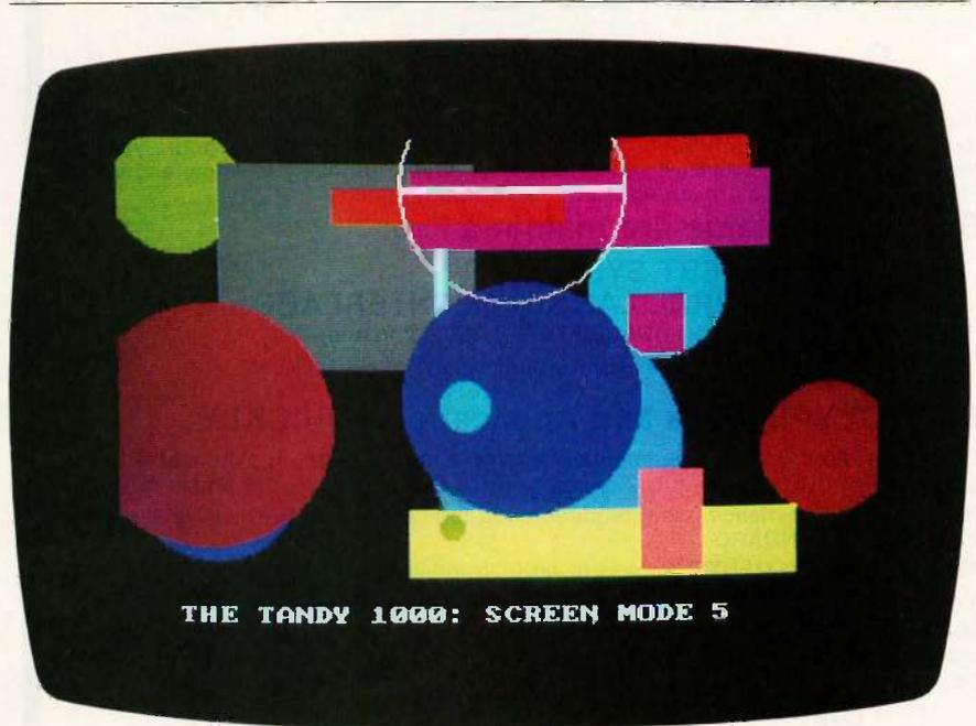
Photo 4: An example of color graphics on the Tandy 1000's RGB display. Note that in medium-resolution mode (320 by 200 pixels) the monitor can display a total of 16 colors, four times the number available on the IBM PC.
