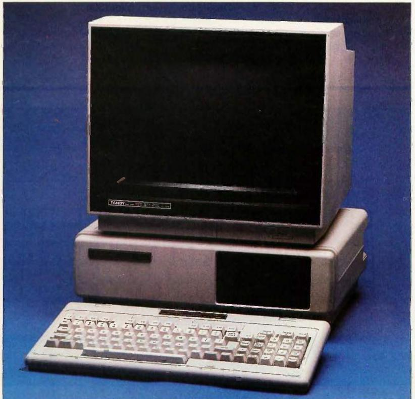
Photo 1: The Tandy 1000 with RGB display and two floppy-disk drives.
