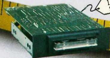
20 MB cassette and 60 MB cartridge back-up systems come with controller, cables and drive. Back-up 20 MB in 6 minutes. You can even do fast Image back-up and then file-by-file retrieval. Works on IBM PC, XT or AT. Internal 10 MB \$499, 20 MB \$699, 60 MB \$899. External 10 MB \$675, 20 MB \$875, 60 MB \$995.
