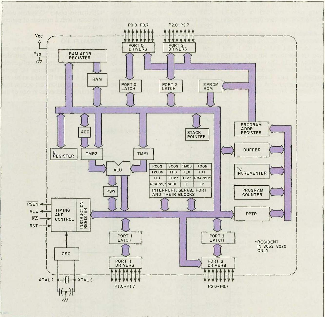
Figure 4: Block diagram of the Intel 8052AH-BASIC chip.
