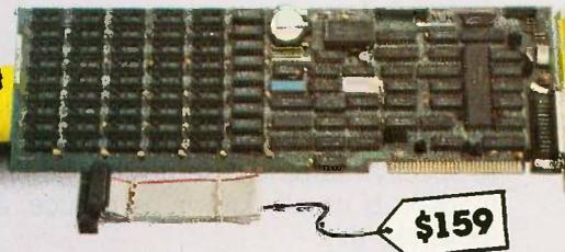
It gives you more than just added memory. It gives you reliable memory expansion (up to 384K), a serial port, a parallel port, a game port, and a battery back-up clock calendar. Includes RAM disk, print spooler, and clock utilities. (The 64K RAM set is only \$15.) With 2 serial ports \$175.
