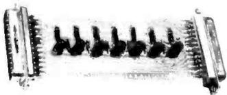
LET THE RS-232 TESTER HELP YOU SOLVE YOUR COMPUTER INTERFACE PROBLEMS. DESIGNED TO CONNECT IN SERIES WITH ANY RS-232 INTERFACE, IT DISPLAYS THE STATUS OF SEVEN OF THE MOST IMPORTANT LINES: TRANSMIT DATA, RECEIVE DATA, REQUEST TO SEND, CLEAR TO SEND, DATA SET READY, CARRIER DETECT, AND DATA TERMINAL READY. THE RS-232 TESTER REQUIRES NO POWER AND MAY BE LEFT IN THE LINE PERMANENTLY.
