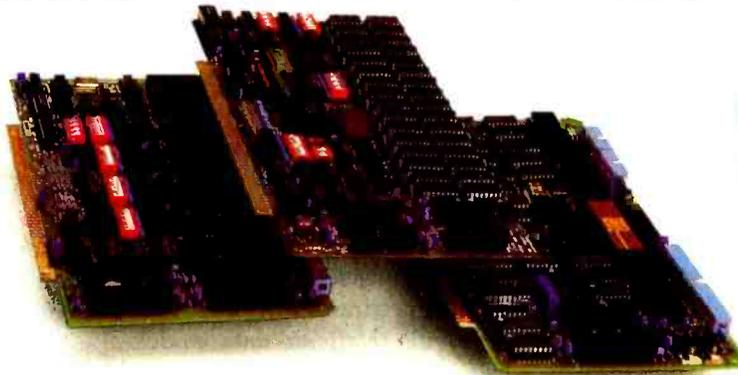
**DOUBLE DENSITY FLOPPY DISK CONTROLLER BOARD** — controls up to four 5¼-inch or 8-inch disk drives using IBM soft sectored formats. It features 1K of on-board buffering, DMA controlled data transfers and the performance characteristics of the superior NEC 765 chip.
