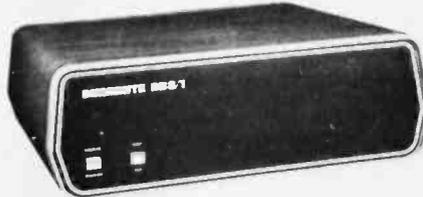
DB 8/1 64 — 64K RAM SYSTEM WITH Z80 CPU and 2 serial and 1 parallel I/O. List \$3395.
