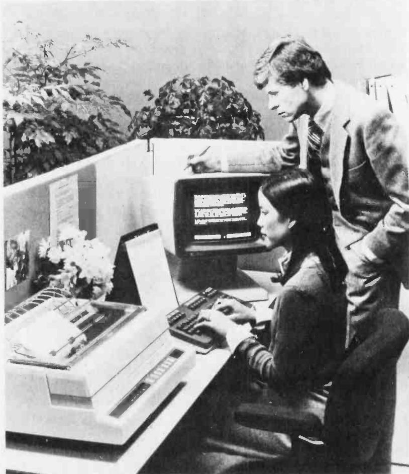
There are two HP 125 modules from which to choose: the Model 10 and the Model 20. The Model 10 uses dual 5-inch floppy-disk drives with 500 K bytes of storage. The Model 20 offers 2.4 megabytes of memory on 8-inch disks. Both models can be expanded with additional drives.
