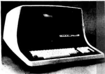
64K Double or Quad Density units available. Uses two Z-80 CPU's. Commercial-type terminal with 12" monitor. Dual double density minifloppies. Over 350 kilobytes of storage (twice that with quad density drives). Two serial RS232 ports, I/O ports standard.
