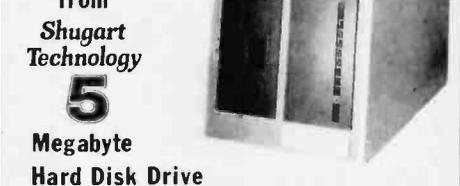
Packaged in the same physical size as the industry standard 5 1/4" minifloppy disk drive. The micro-Winchester stores thirty times as much data (6.38 megabytes unformatted), accesses data twice as fast (170 milliseconds) and transfers data twenty times faster (5.0 megabits per second.)
