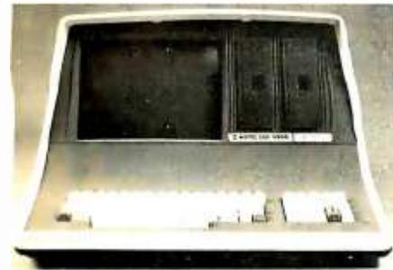
Self-contained computer with dual disks and two RS232C ports. Complete with CP/M™ 2.2 and BASIC.
