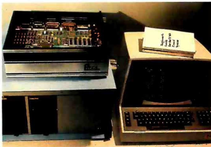
Figure 1: The Pascal Microengine is shown here in a system which includes two Shugart 8-inch disk drives in an Integrand cabinet and a Xerox IQ120 terminal. The computer uses a 16-bit processor chip and it executes p-code directly through the use of three integrated circuits on which the processor microinstructions are stored. The Microengine also includes 64 K bytes of memory, a 24-bit parallel port, and two RS-232C serial interfaces. The software provided is the UCSD extended Pascal system.
