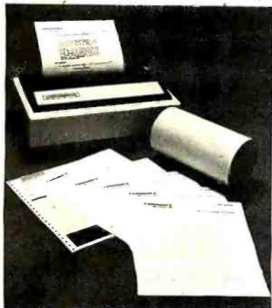
The model 737 dot-matrix printer features right-margin justification, proportional spacing, forward and reverse paper motion, and three-way paper handling. It prints 7-by-8 dot-matrix characters at 10 and 16.5 characters per inch for standard data processing tasks, and generates n-by-9 dot-matrix characters in the proportional character spacing used for data and text processing. The printer incorporates an adjustable nine-wire, free-flight printhead. Under manual or software control, the
