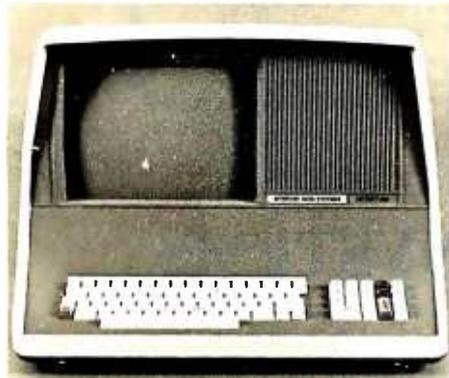
12" Display; 24 x 80 format; 18-key numeric keypad; 128 upper/lower case ASCII characters; Reverse video, blinking; Complete cursor addressing and control; Special user-defined control function keys; Protected and unprotected fields; Line insert/delete and character insert/delete editing; Eleven special line drawing symbols.
