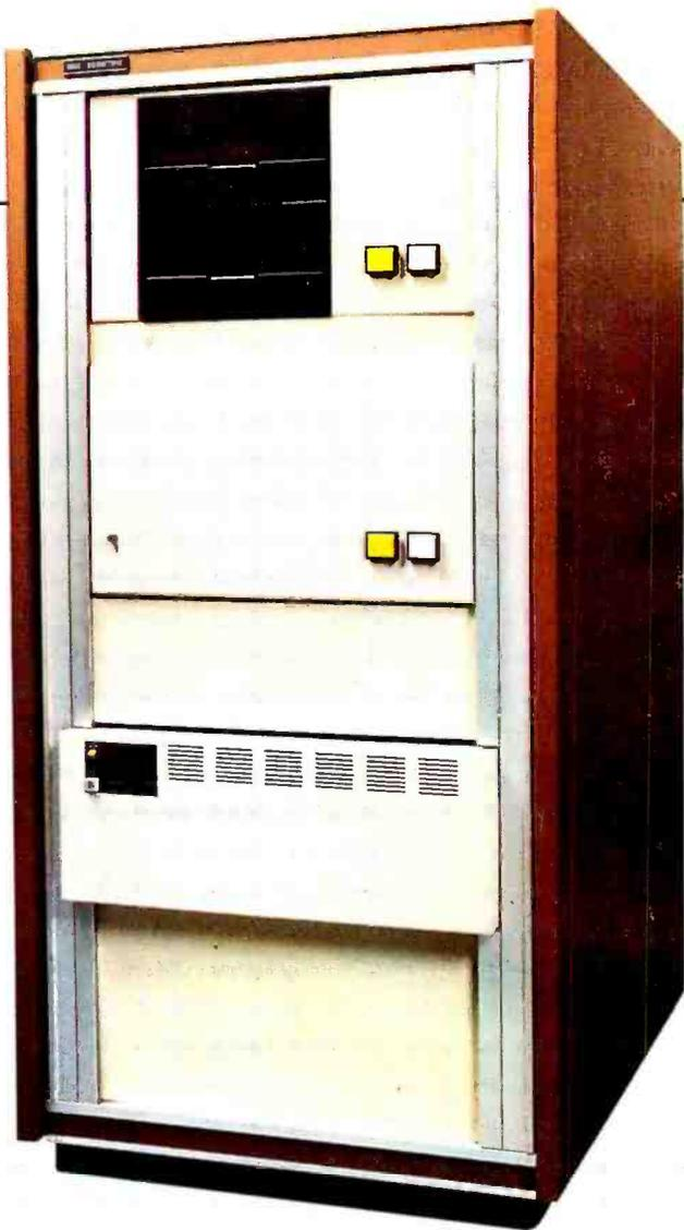
Series, the C3-B. Its specifications are the same as those of the C3-C. However, the C3-B offers a 74 Megabyte Winchester drive.
