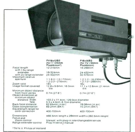
The new Canon 18x series for major broadcast cameras. With the best relative aperture, superior wide angle and shorter M.O.D. Choice of manual or servo focus and zoom. Built-in servo/manual operated 1.5x and 2x extenders. And interchangeable, plug-in servo modules, for easier service. All at a competitive price.
