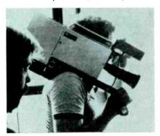
compensator, 3 Plumbicon® (Satican®) tubes and I and Q encoder, pre-heat circuit—low power consumption of approximately 30 watts AC. Easily adapts to battery. Optional adaptor for use with 12V car or truck batteries. No wonder top TV news crews use.
