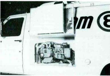
Onan generator provides auxiliary power for van's equipment. External AC power is used when available.
