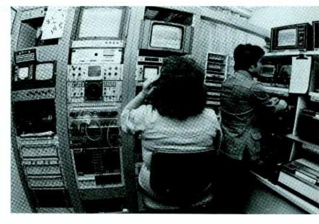
Eye Control: the heart of the ENG newsroom. Microwave controls are on left, patching and test gear in center rack. Two Microtime 2020s, one with Image Plus, are in righthand rack.
