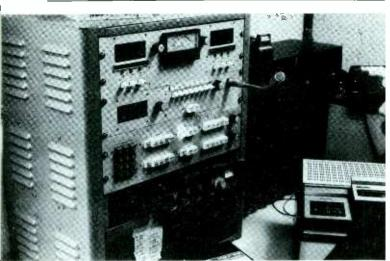
Console in ENG decision room allows communications with all areas of WFAA operation through intercom system. Any in-house source can be routed to station's editors.
