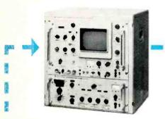
SWOF VIDEOSKOP A video sweep generator tracking selective (3 kHz) receiver, and display unit. Range: Frequency, 20 kHz to 20 MHz, (1 GHz with sideband adapter); Sweep Width: 1 to 16 MHz, continuously variable; sweep duration 50 ms to 5.5 s.
