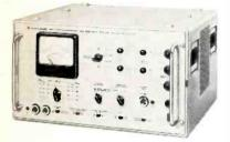
Designed for noise voltage measurements on TV cameras, film scanners, video tape recorders, radio links, coaxial lines, TV transmitters, receivers and transposer, with synch. Signals.
