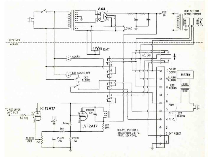
Fig. 9. Alarm circuit using twin triode derives its power from the companion receiver; failsafe feature is included.
