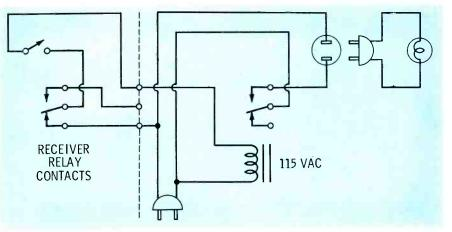
Fig. 12. Arrangement for use with alarm having external-indicator contacts.
