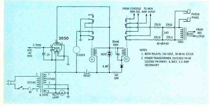
Fig. 7. Schematic diagram of the thyratron EBS alarm unit. No DC power supply is required for this alarm circuit.
