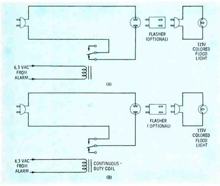
Fig. 11. Floodlight, with flasher if desired, serves as inaudible indicator.
