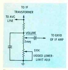
Fig. 3. Variable resistor is added to control to insure volume is audible.
