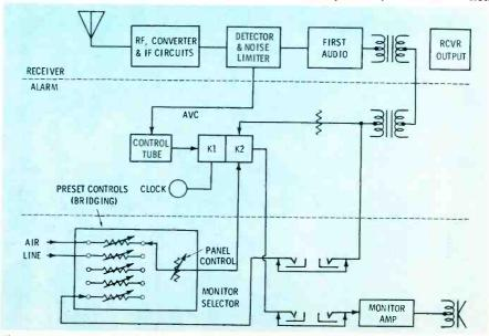
Fig. 5. Diagram shows use of alarm receiver with monitor system in station.
