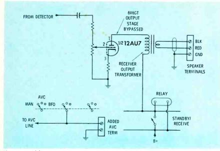
Fig. 6. Modifications to communications receiver used with system of Fig. 5.
