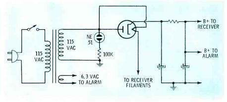
Fig 13. Power-supply modification for safe use of AC-DC radio with alarm.
