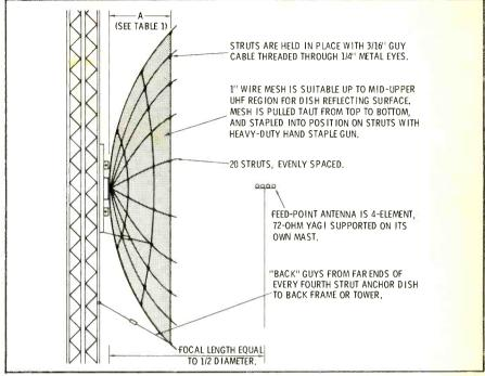
2. Physical construction of the experimental limited-aperture parabolic. Fig.
