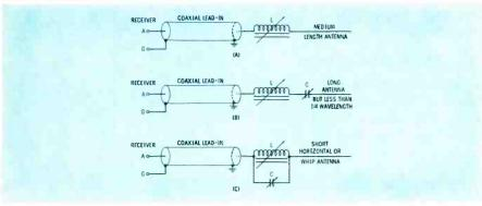
Fig. 10. Methods of connecting antennas through a coaxial transmission line.
