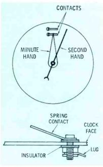
Two insulated contacts are mounted on the clock face and wired in series so that the minute hand and second hand must close the circuits simultaneously. We used a DC relay and supply with a large capacitor across the relay to prevent skipping or intermittent tone operation. A little adjustment of the contacts and hands was required, but once the system was set up, it worked fine.
