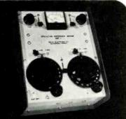
Delta Model OIB-1 Operating Impedance Bridge measures "in circuit" impedance of networks, transmission lines and antennas while operating at full or reduced power. Accuracy:  $\pm 5\% \pm 1$  Ohm. Power Rating: 5kw with VSWR of 3:1.
