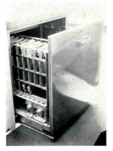
Fig. 2. Pull-out chassis at desk ends contain the solid-state circuit modules.
