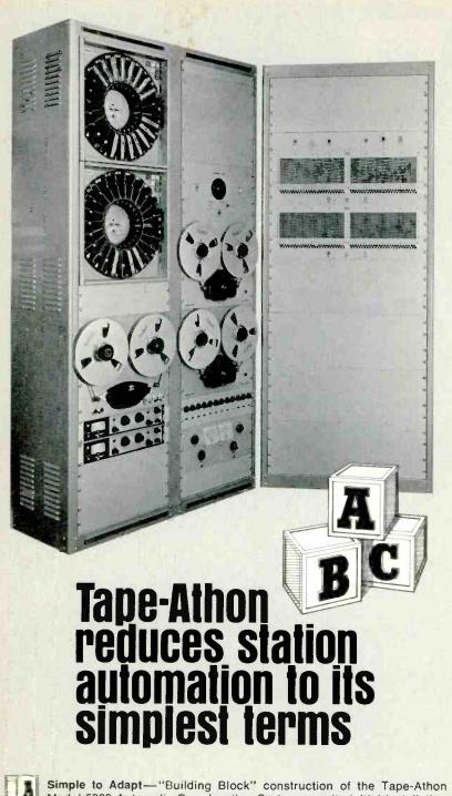
Simple to Adapt—"Building Block" construction of the Tape-Athon Model 5000 Automatic Broadcasting System permits initial installation of basic system to fit budget and/or station requirements. Then, system may be easily expanded to increase capacity as needs arise.
