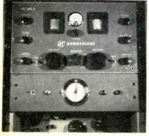
Fig. 4. Alarm uses thyratron, clock.
