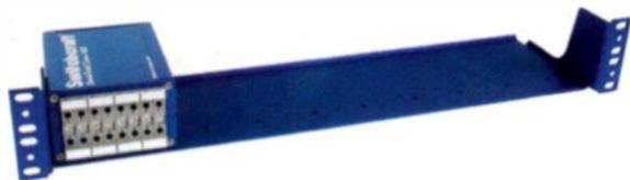
Modular design provides audio engineers with a premium-quality TT patch bay that can be used as an individual eight-channel patch module or mounted up to five across into a 1.5RU rack tray; EZ Norm technology enables signal flow to be changed from the front of each channel using a standard screwdriver, and programmable ground lift switches are easily accessed by removing the rear panel; each module connects using two DB25 connectors wired to the TASCAM DTRS.
