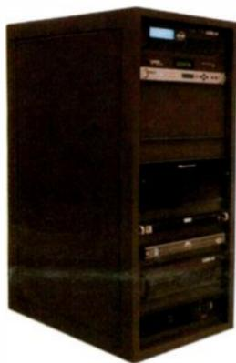
A fully integrated multichannel digital LPTV transmission system integrates the new OCTANE encoder/multiplexer; features multiple baseband inputs, up to four multiplexed SD channels and an integrated dynamic PSIP; is ATSC closed-captioning compliant; a Pathwaves digital microwave STL system is optional.
