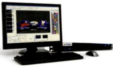
Offers both HD-SDI and SD-SDI functionality, as well as the specs and feature set of a full-size system in a rugged 1RU chassis; ideal for channel-branding applications, with software options including NewsScroll with RSS, which provides the power of multiple crawls, logos, a real-time clock, live weather updates, ratings, and live RSS feeds.
