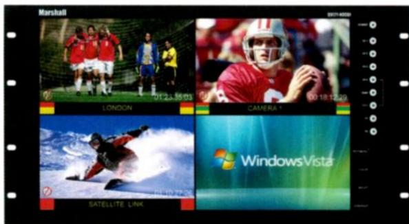
Full-resolution monitors with IMD; available in different sizes; allows viewing of four different inputs at once with three different layouts to choose from; does not require external under monitor display; supports the following protocols: Image Video, NVISION, TSL and MEI; offers a full-resolution 1920 x 1200 display; new unique RotoMenu feature enables fast, direct and easy menu navigation.
