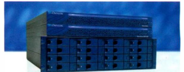
Central server component of an Omneon Spectrum media server; integrates file system, system management, communication and all connectivity, including Fibre Channel, MediaPorts and Ethernet; Fibre Channel interface provides four data paths between the MediaDirector and the MediaStores, supports 4Gb/s SFP transceivers (plug-in modules) with LC optical fiber interfaces.
