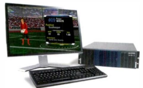
Available as single- or dual-channel; new hardware platform supports SD and HD processing, video capture, 3D animation and dedicated processing for each output channel.
