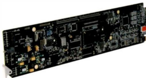
Offers both 5.1-channel and stereo loudness processors using inputs from any source received by the card, or any mixing setting produced by the card; AEROMAX algorithms use a multiband approach to loudness processing and can apply multifaceted loudness correction specifically targeted to various frequency ranges and other characteristics within the program material.
