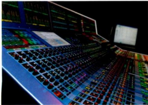
Relies on Bluefin2 for processing; at 48kHz, Bluefin2 gives Apollo up to 1020 channel processing paths, 128 program busses, 96 IFB/track outputs and 48 auxiliaries; at 96kHz, Apollo affords 510 channel processing paths, 64 program busses, 48 IFB/track outputs and 24 auxiliaries; features a second dynamics section in each channel, more than 70 minutes of assignable delay and three independent APFL systems for multiple operator use.
