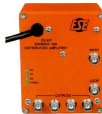
A 1 x 4 3G/HD/SD-SDI distribution amplifier; provides cable equalization, reclocking and distribution; features high performance and low cost; can distribute 3Gb/s, 1.5Gb/s and 270Mb/s data rates; can equalize 400m at 270Gb/s, 200m at 1.5Gb/s and 140m at 3Gb/s of 1694A coax cable; non-SMPTE data rates may be distributed by using the internal reclock enable switch; can pass data rates from 143Mb/s to 2.97Gb/s while in bypass mode; ASI-compliant at 270Mb/s; a separate loop output is also provided.
