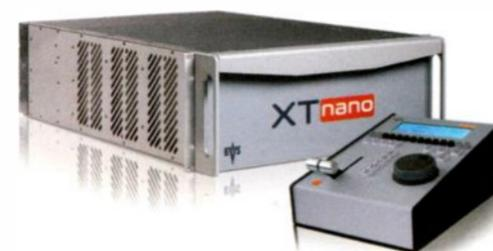
Entry-level replay and live slow-motion server for live broadcasters and OB facilities; housed in a 4RU chassis offering four configurable channels (two cameras IN and two OUT for preview and program control, or three IN and one PGM) and native support of DVCPRO HD and DVCPRO 50; dual Gb/s Ethernet networking provides faster than real-time file transfers.
