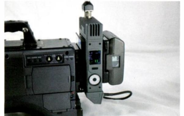
Intended for wireless camera applications, such as sports coverage and electronic news gathering; offers MPEG-4 encoding/decoding, HD, low power consumption and is available in licensed bands and others upon request; rugged machined housing provides durability and thermal characteristics for operation in the harshest of conditions.
