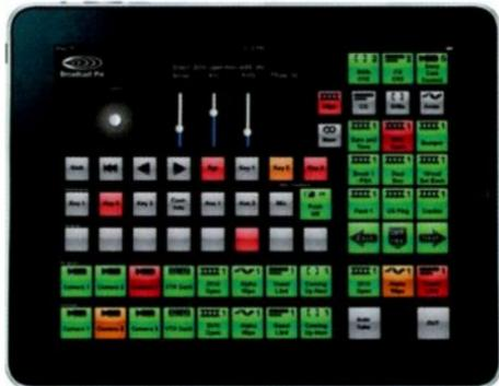
Enables control of any Slate video production system via Apple iPad; facilitates control of every aspect of a video production including switching cameras, adding graphics and clips, controlling robotic cameras and creating special effects; re-creates a classic switcher layout including auto transition and cut buttons as well as eight-input program and preview buses with shift for 16 inputs; adds device controls for the graphics system, clip store, etc.
