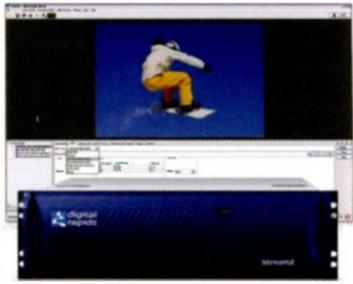
Supports three-screen live and on-demand experiences and file-based workflows by offering simultaneous encoding to multiple formats and devices; new features include integrated segmenting for Apple iPhone delivery, JPEG 2000 encoding and workflow integration, YouTube Content ID fingerprinting support, Microsoft PlayReady digital rights management support and enhanced Microsoft IIS Smooth Streaming.
