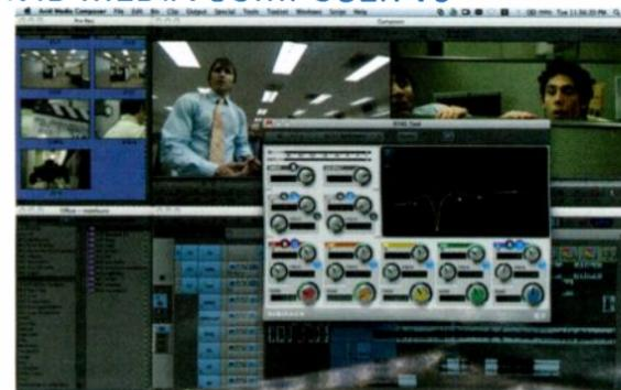
Offers native support for popular industry formats, including RED, QuickTime and Canon XF; features include HD-RGB finishing capabilities, real-time audio effects with support for Real-Time Audio Suite (RTAS) audio plug-ins, and a timeline Smart Tool featuring drag-and-drop audio and video elements.
