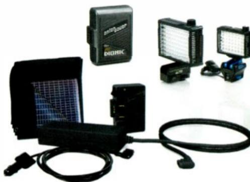
Fully automatic system separates the Gold Mount device from the power supply, allowing the user to simultaneously charge a battery and power a camera; when 75W draw is exceeded, the system automatically stops charging and performs solely as a 150W power supply; when camera is turned off or load is reduced below 75W, the system instantly resumes normal operation; users can operate the system from the AC mains at 100V to 240V AC or 50Hz to 60Hz.
