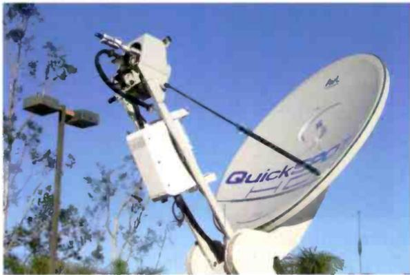
Automated operation sets the antenna up in about five minutes; can be integrated into mid-size SUVs, vans or added to existing ENG vehicles; delivers high-quality video and audio at bandwidth rates as low as 2Mb/s for SD and 6.5Mb/s in HD; can deliver up to 9.98Mb/s uplink data rates; includes mobile office features such as IFB-compatible phone lines and Internet access; modular architecture allows for the integration of additional IP-based components and accommodates future upgrades.
