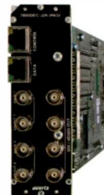
Provides variable JPEG2000 compression rates on ASI or IP; supports pass through of up to two AES groups of embedded audio; card functions are controlled from the card edge or through the VistaLINK interface.
