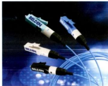
Enables fast, fool-proof, easy fiber termination in the field with no tools required; built-in activator tab performs the fiber splicing and crimping action in one simple motion; users can verify proper connection using an external laser light source, which can be clearly seen through the connector's window, offering immediate termination assurance; available for 900µm LC (OM1, OM2, OM3 and OS2).
