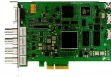
Now includes dual link and 3Gb/s SDI for 4:4:4 quality, and a new hardware downconverter for simultaneous HD and SD playback; connects to SDI, HDMI, component analog, NTSC/PAL and S-video equipment for capture and playback, while instantly switching between SD, HD and 2K.
