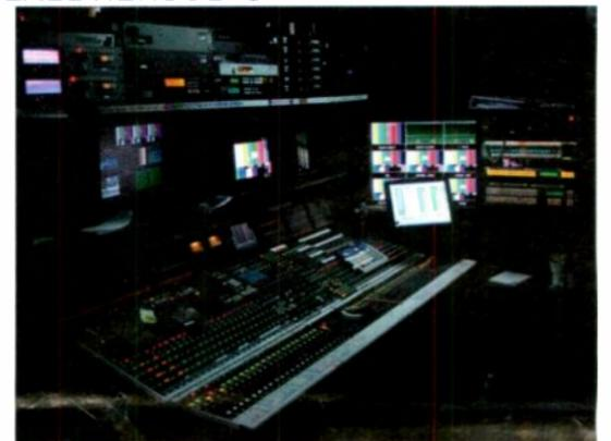
Designed to meet the demand for HD production facilities in hard-to-access production spaces for sports, entertainment and reality TV; features lightweight HD technology, an LCD monitor wall, working positions incorporated into custom equipment racks and optimized rack design and mechanics; can be set up quickly, is flexible and can handle many different types of production requirements.
