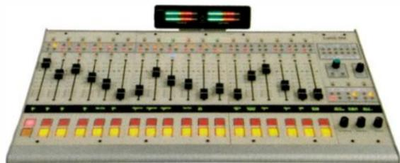
Modular, scalable console provides up to 24 faders; audio sources may be routed as desired to each of the faders; each fader has access to a program bus, three aux busses and cue speaker; bright, wide-angle displays below the faders have room for 16-character source names and support Unicode characters for display of text in multiple languages.
