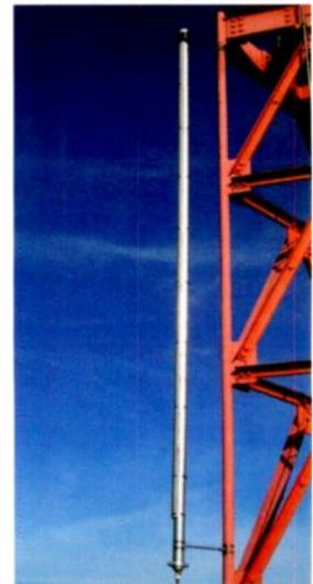
Features horizontally polarized antennas in a number of SD azimuth patterns, with an average power rating of 1.6kW; designed to provide a low weight and windload system for mobile media transmissions, distributed transmission systems and translators; features an eight-bay single module design; provides a single 7/8in input, a 1.5-degree beam tilt and a low-profile slot cover for protection from environment wear and tear.
