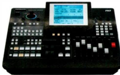
A low-cost HD/SD digital A/V mixer that incorporates a built-in multiviewer display output and combines high-quality video switching and audio mixing features; offers a flexible use interface and supports SD, HD, and 3-D HD formats; supports multiple camera workflows, from production, to corporate A/V projects, to wedding and live events; can switch 3-D HD video.
