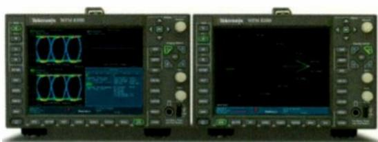
Provide high-quality, real-time, automated 3Gb/s SDI eye pattern display and jitter measurements; feature advances in color grading with new patented Luma Qualified Vector and Spearhead Gamut displays; WFM8300 also provides multi-rate HD/SD-SDI and 3G-SDI color bar and pathological signal generation capabilities.
