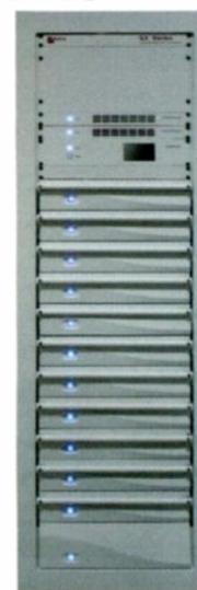
The high-powered, liquid-cooled TV transmitter offers high power density in a small footprint, with N+1 power supplies for reliability, hot-swappable amplifiers for simple maintenance, and a broadband combiner for future upgradeability; available in power levels up to 7kW DVB, and 17kW analog in a single cabinet, with multicabinet configurations available for higher power levels.
