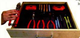
depth. Foam is available in <sup>7</sup>/<sub>8</sub>", 1<sup>1</sup>/<sub>8</sub>" and 2<sup>1</sup>/<sub>4</sub>" depths. It comes in black, white and black on white, which is white foam with one black layer. The dense, rigid foam can be cut with a utility knife, and the multiple layers allow the cut-out to be contoured. The layers are fused together but specially designed to pull apart fairly easily and consistently when cut. **fastcap.com**
