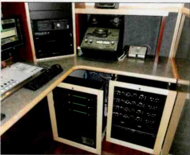
The two under-counter racks are mounted on slides to facilitate equipment access.
