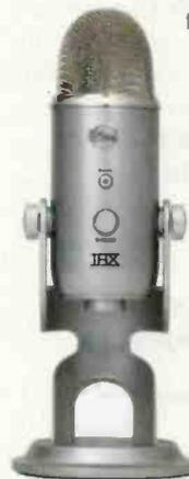
**Yeti:** Yeti is the first THX Certified microphone. It is the first USB mic to offer Blue's premium condenser capsules in a proprietary triple capsule array. It includes four patterns (omni, cardioid, stereo, bidirectional). Yeti has studio quality performance and features, with zero latency, amplified headphone monitoring, microphone mute, and hardware-based gain adjustment. The Yeti's angle
