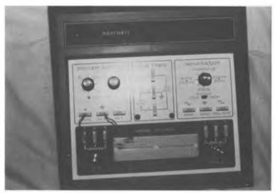
Fig. 1-4. Experimenter's breadboard by Heathkit.
