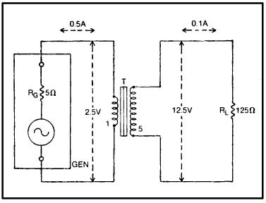
Fig. 2-14. Impedance-matching transformer.
