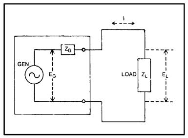
Fig. 2-10. Circuit illustrating an  ${\sf Ac}$  generator feeding a load impedance  $(Z_L).$  Current must flow through both the generator impedance  $(Z_G)$  and the load impedance.
