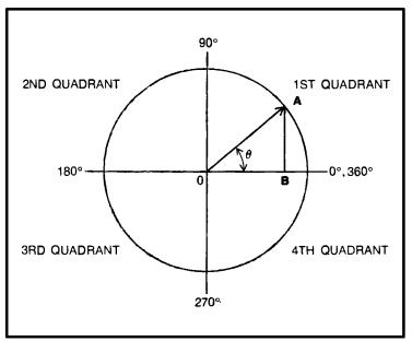
Fig. 1-6. Vector representation of Ac components.
