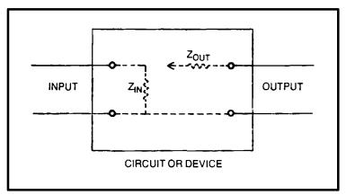
Fig. 2-11. Illustration of a device having both input and output impedance.
