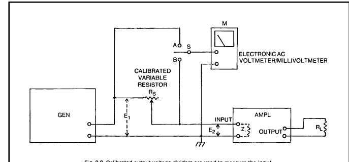
Fig. 3-9. Calibrated output-voltage dividers are used to measure the input impedance of an amplifier.
