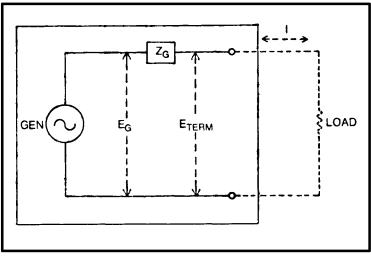
Fig. 2-9. Circuit illustrating impedance ( $Z_G$ ) of an Ac generator.
