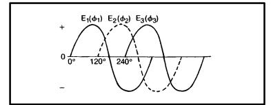
Fig. 1-5. Three-phase voltage. Three equal-amplitude voltages are spaced 120° apart.
