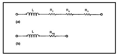
Fig. 4-5. Equivalent circuits of core-type inductors with: (a) losses shown as series-resistant components, and (b) losses simplified to the equivalent resistance.
