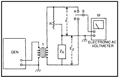
Fig. 3-4. Resistance/balance method of measuring an unknown impedance.
