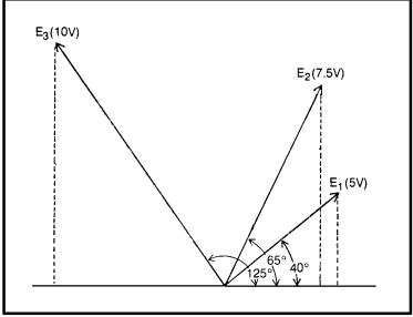
Fig. 1-7. Vector diagram of out-of-phase components.
