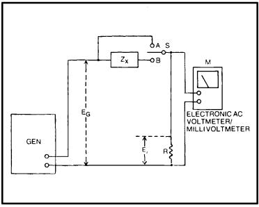
Fig. 3-3. Voltmeter method for measuring an unknown impedance.
