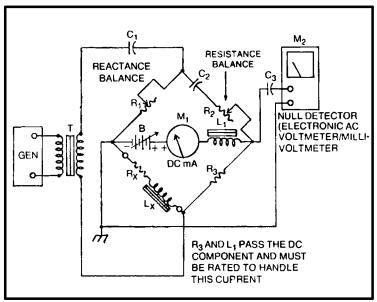
Fig. 3-14. A typical bridge circuit used for choke-coil measurement. The circuit shown is a Hay bridge.
