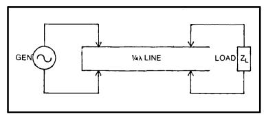
Fig. 2-16. A quarter-wave section of open-line resonant transmission line is short-circuited at one end and used as an RF impedance-matching transformer.
