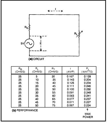
Fig. 2-13. Illustration of impedance matching. The circuit (a) has a variable load resistance connected to a generator. The chart (b) shows the performance of the circuit as the resistance ( $R_U$ ) is varied.
