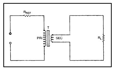
Fig. 2-12. Reflected impedance in the primary of a transformer with resistance  $\rm R_L$  loading the secondary.
