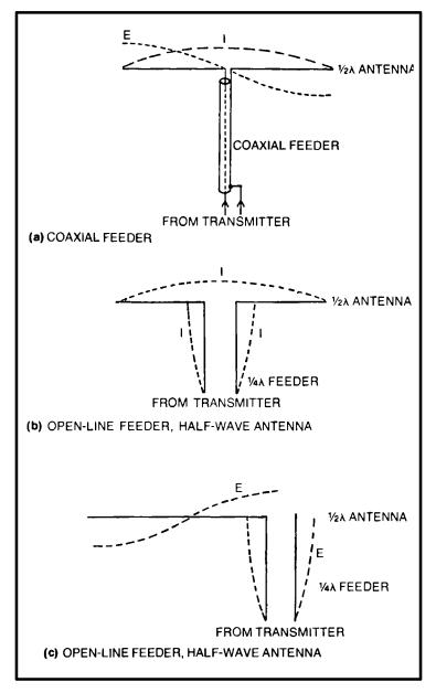
Fig. 2-15. Transmission line feeders used for the maximum transfer of energy from the transmitter to the antenna: (a) a coaxial feeder is connected to the center of a half-wave antenna; (b) a resonant open-line feeder is used to current-feed the center of a half-wave antenna; (c) a resonant open-line feeder is used to voltage-feed a half-wave antenna.
