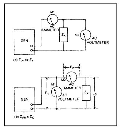
Fig. 3-1. Voltmeter/ammeter method for measuring an unknown impedance: (a) when the impedance of the meter ( $Z_{VM}$ ) is higher than the unknown impedance ( $Z_X$ ); (b) when the impedance of the meter is equal to or less than the unknown impedance
