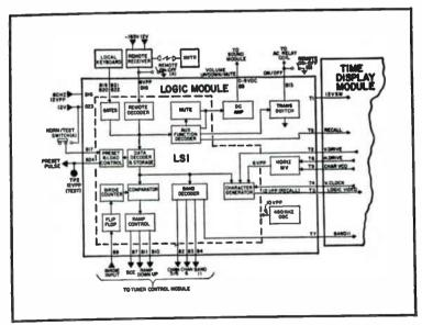
Fig. 2-13. Logic module found in STAR system.
