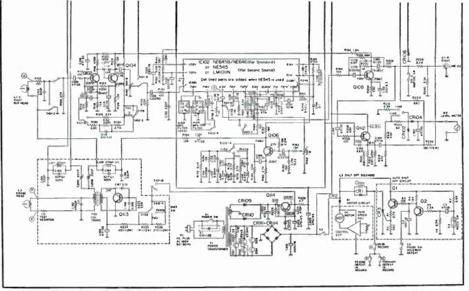
Fig. 7-7. Complete circuit of a cassette play/recorder unit.
