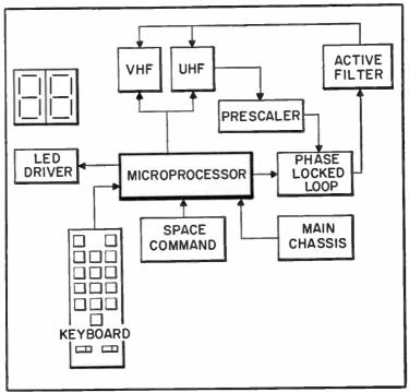
Fig. 1-3. Functional block diagram of direct access system.
