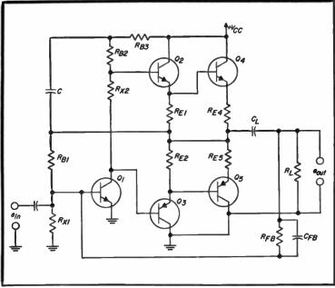
Fig. 5-17. Darlington pairs used in audio output circuit.
