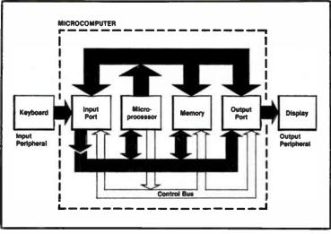
Fig. 12-1. Block diagram of microprocessor system.
