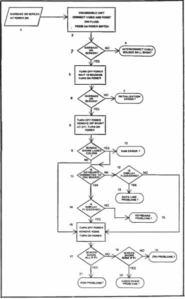
Fig. 12-18. Part removal isolation flowchart.
