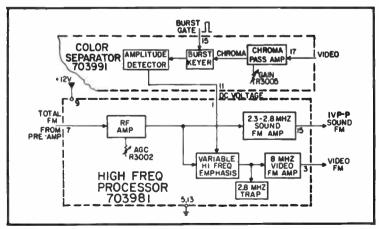
Fig. 11-13. FM signal processing circuit.
