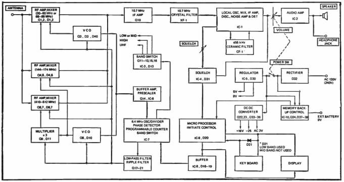
Fig. 8-9. PRO-2008 scanner block diagram.
