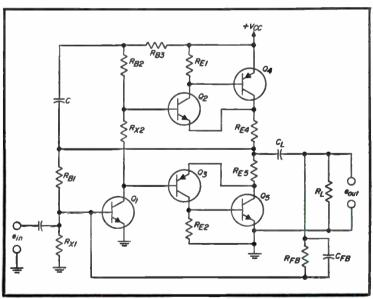
Fig. 5-18. Audio output circuit using complementary pairs.
