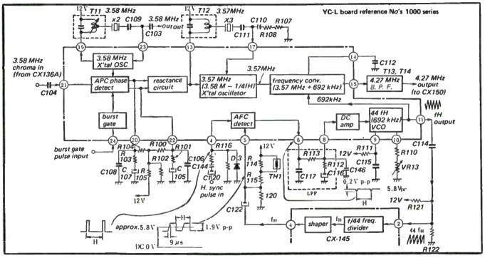
Fig. 10-8. Block diagram of CX137A chip.
