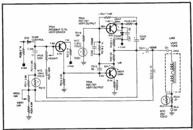
Fig. 4-3. Vertical output and driver circuit.
