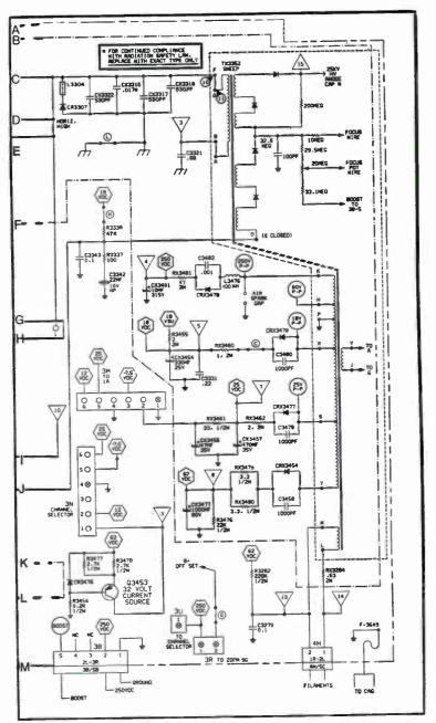
Fig. 3-51. Complete schematic of the 9-160-03 module (continued from page 129).
