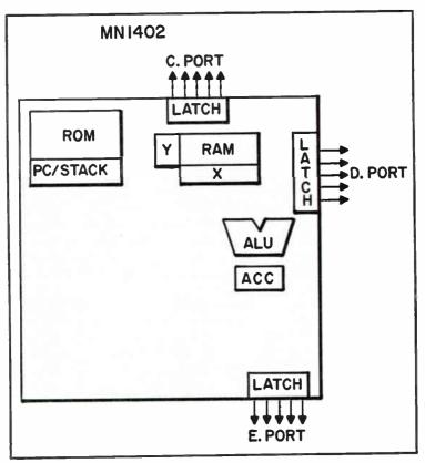
Fig. 1-6. Microprocessor organization diagram.
