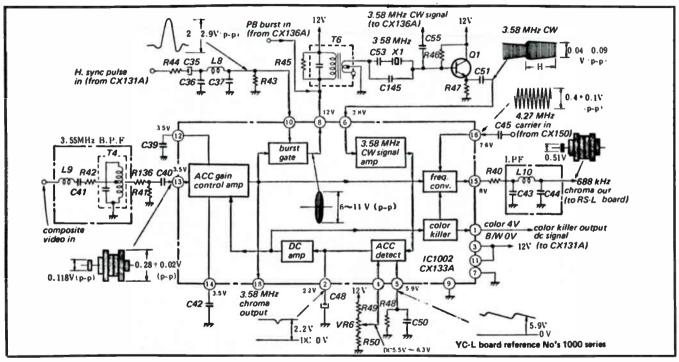
Fig. 10-11. Block diagram of CX133A chip.
