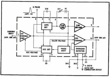
Fig. 3-36. Block diagram of chroma processor module.
