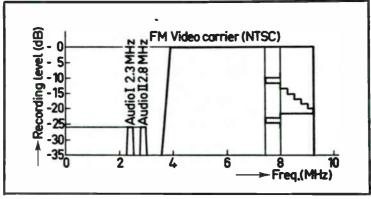
Fig. 11-3. Frequency spectrum of video disc information.
