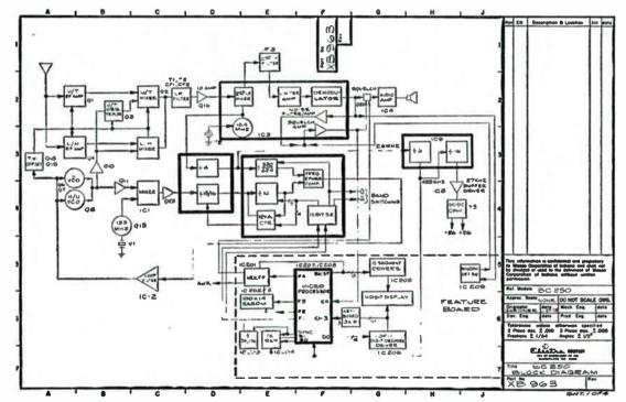
Fig. 8-1. Block diagram of BC 250 BEARCAT programmable scanner.
