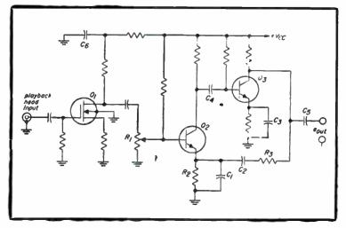
Fig. 7-2. Tape playback pre-amplifier circuit.
