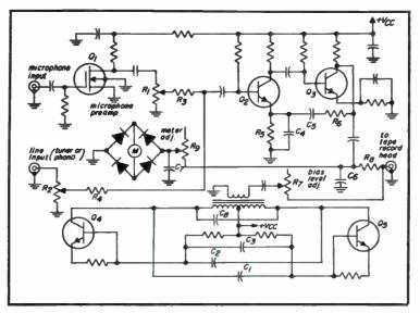
Fig. 7-1. Tape recorder pre-amplifier circuit.
