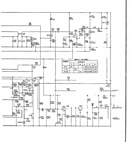
decreases, from the low to high channels, three levels of attenuation are needed. These are provided by voltage-dividing resistors and are switched by the varactor control bandswitch to the base of KQ04. The divider network KR16 and KR17 is used for AFC level correction on the UHF band. KR13 and KR15 are used to attenuate the voltage for high VHF channels, while the collector voltage of KQ02 is used directly on the VHF low band channels.
