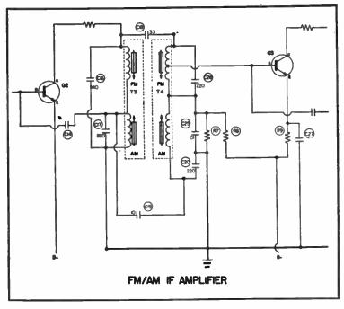
Fig. 5-2. FM/AM IF amplifier circuit.
