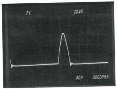
Fig. 3-18B. Horizontal keying pulse.
