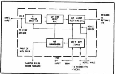
Fig. 3-29. Block diagram of horizontal IC stages.
