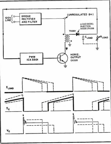
Fig. 3-53. Chopper circuit and waveforms.
