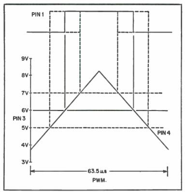
Fig. 3-60. Variations of transfer PWM characteristics.
