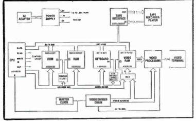
Fig. 12-10. System block diagram of TRS-80.
