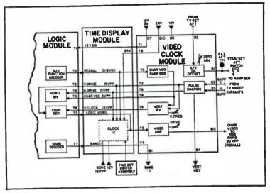
Fig. 2-12. Video clock and time display modules.
