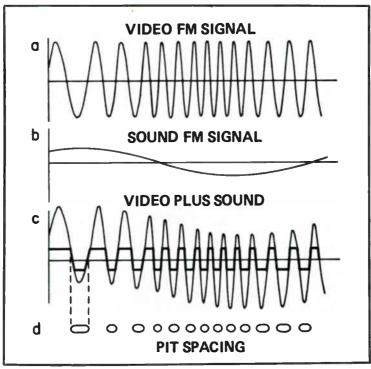
Fig. 11-4. Encoding of disc information.
