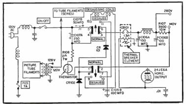
Fig. 3-27. Power supply and degauss circuit.
