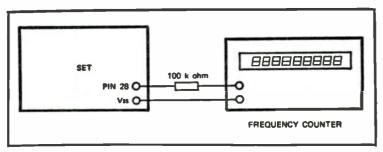
Fig. 6-9. Clock and subcarrier frequency adjustment set-up using a frequency counter.
