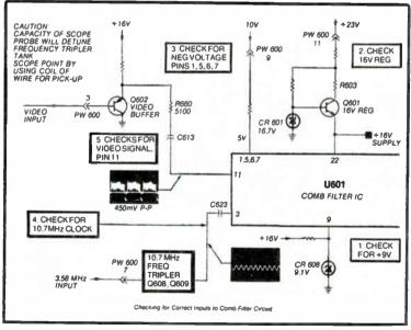
Fig. 3-40. Correct signal inputs of the comb filter.
