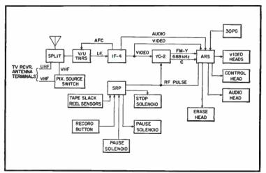
Fig. 10-14. Block diagram of KR9000 units record mode.
