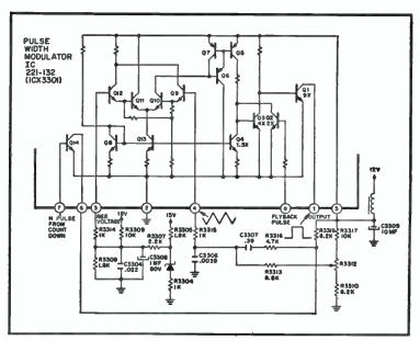
Fig. 3-57. Pulse width modulator IC.
