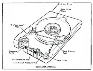
Fig. 7-11. Inside view of an 8-track cartridge.
