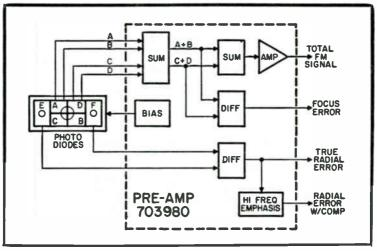
Fig. 11-11. Photo diodes and pre-amp module.
