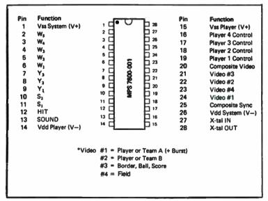
Fig. 6-7. Pin out for MPS-7600-001 game chip.
