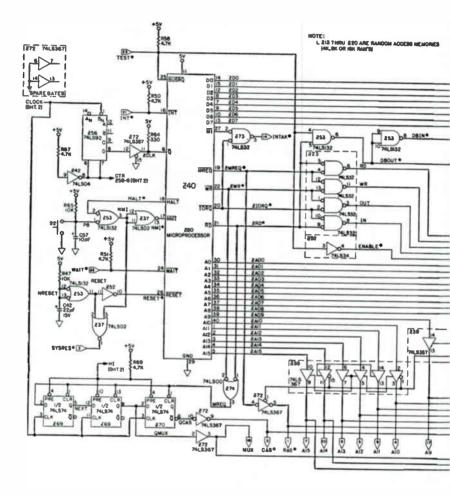
Fig. 12-11. Schematic of TRS-80 (section 1).
