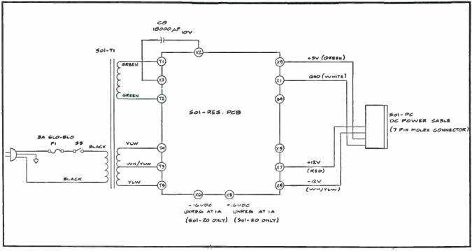
Fig. 12-21. SOL-10 power supply block diagram.
