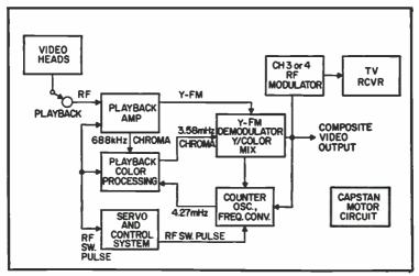
Fig. 10-6. Block diagram of playback mode.
