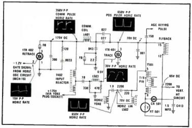
Fig. 3-30. RCA trace and retrace horizontal sweep circuits.
