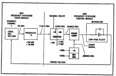
Fig. 1-7. Basic phase-locked loop operation.
