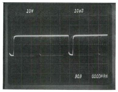
Fig. 3-18D. Horizontal sync pulses.
