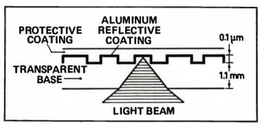
Fig. 11-2. Cross section of one side of a video disc.
