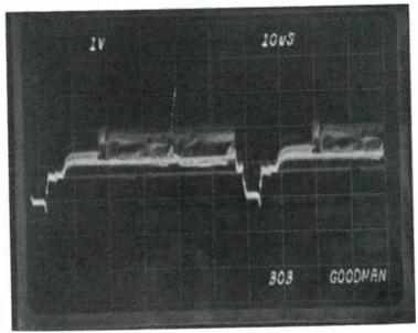
Fig. 3-18C. Composite video signal.
