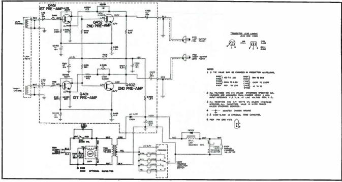
Fig. 7-13. Circuit for 8-track playback unit.
