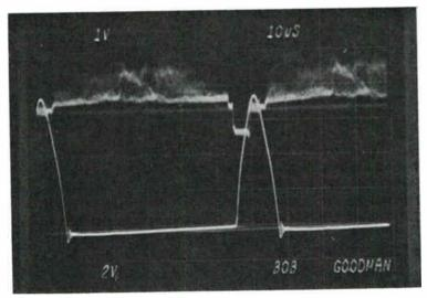
Fig. 3-22. Dual-trace scope showing mis-timed pulse.
