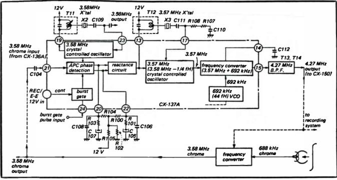
Fig. 10-7. Block diagram of APC circuit.
