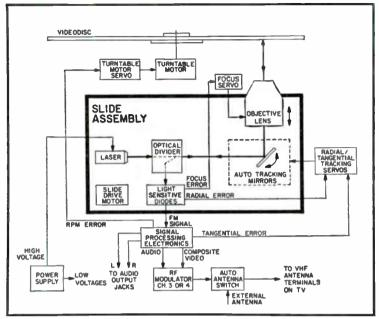
Fig. 11-6. Block diagram of disc player.
