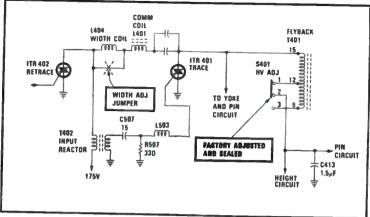
Fig. 3-31. Simplified horizontal deflection circuit.
