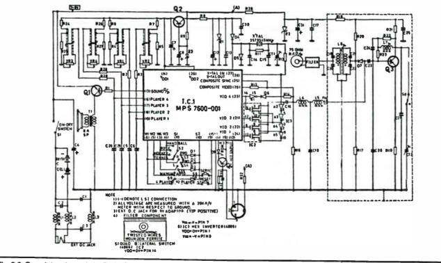
Fig. 6-8. Complete schematic for Radio Shack 60-3057 video game.
