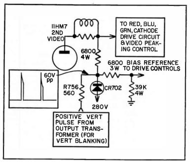
Fig. 3-43. Vertical retrace circuit.
