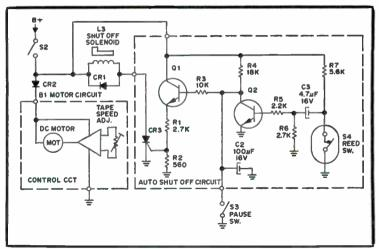
Fig. 7-10. Auto shut-off tape recorder circuit.
