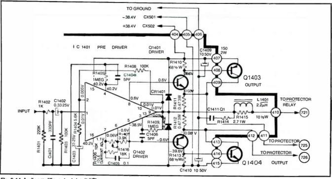
Fig. 5-14. Audio amplifier output circuit (IC).
