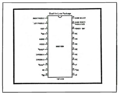
Fig. 6-4. Pin out for model MM57100N IC chip.
