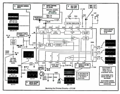
Fig. 3-6. Chroma circuit with check points and waveforms.
