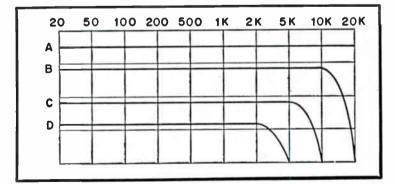
Fig. 7-9. Noise reduction response curve.
