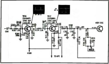
Fig. 4-8. Solid-state sync circuit.
