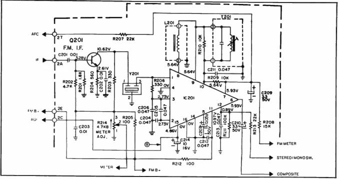
Fig. 5-6. FM IF chip circuit.
