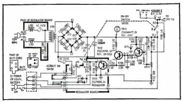
Fig. 4-15. Low voltage power supply.
