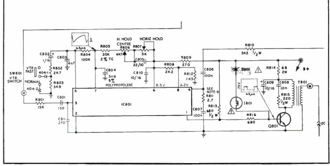
Fig. 4-13. Horizontal oscillator - IC type.
