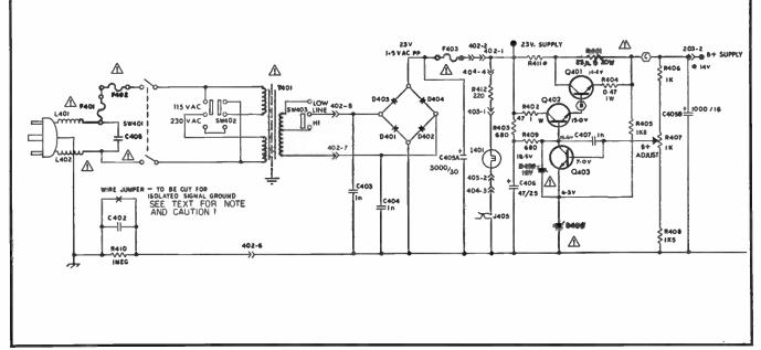
Fig. 4-12. Regulated power supply circuit.
