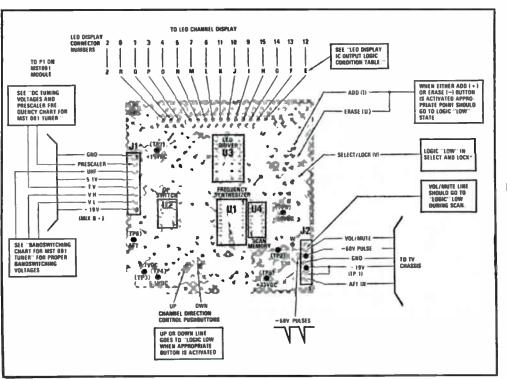
Fig. 1-11. Scan FS control module.
