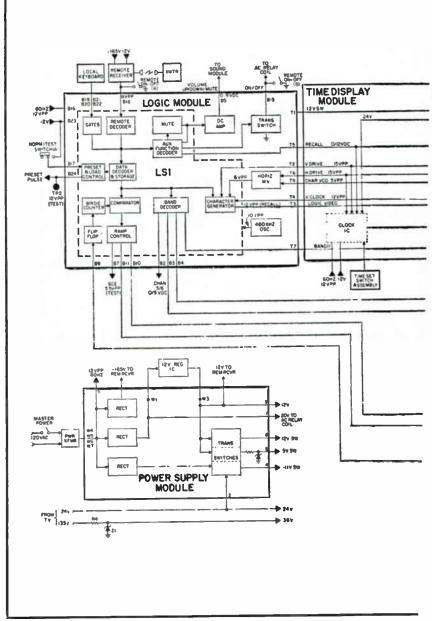
Fig. 2-14. Remote system signal flow block diagram.
