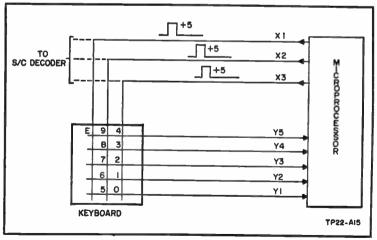
Fig. 1-5. Keyboard scanning block diagram.
