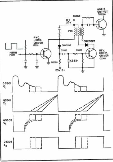
Fig. 3-55. Evolved chopper circuit and waveform.
