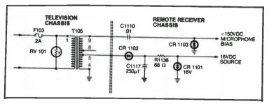
Fig. 2-9. Power supply circuit for remote receiver.
