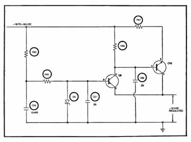
Fig. 5-3. Voltage regulator for stereo receiver.
