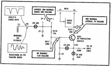
Fig. 3-32. High Voltage protection circuit - RCA CTC 74.
