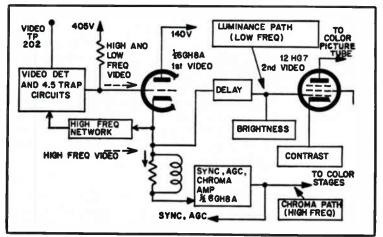
Fig. 3-42. Simplified first video amplifier circuit.
