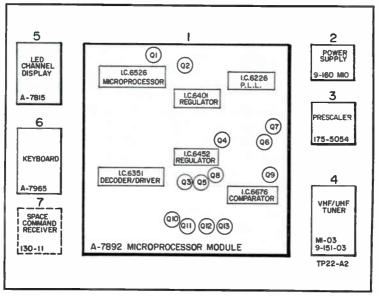
Fig. 1-2. Direct access system block diagram.
