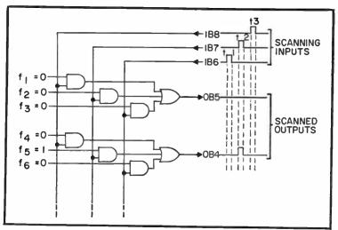
Fig. 2-7. Strobed output logic.
