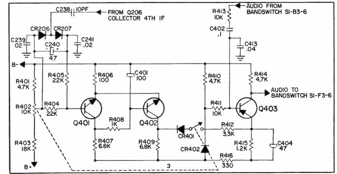
Fig. 9-5. Transistor squelch circuit.
