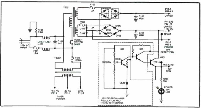
Fig. 10-1. Power supply circuit with +42 volt regulator.
