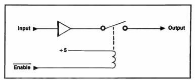
Fig. 12-3. Equivalent Three-State Driver.
