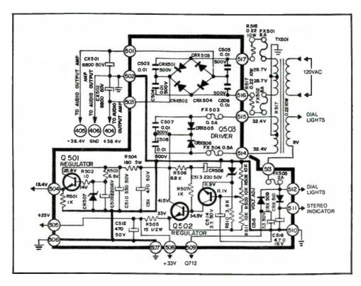
Fig. 5-16. Stereo receiver power supply circuit.
