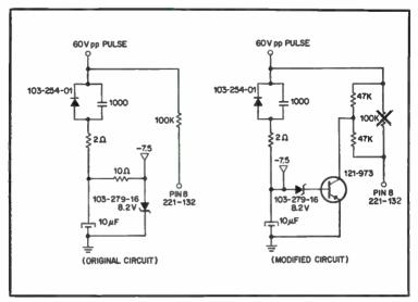
Fig. 3-62. Modification of horizontal output circuit.
