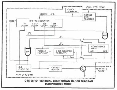
Fig. 3-2. Vertical count-down block diagram.
