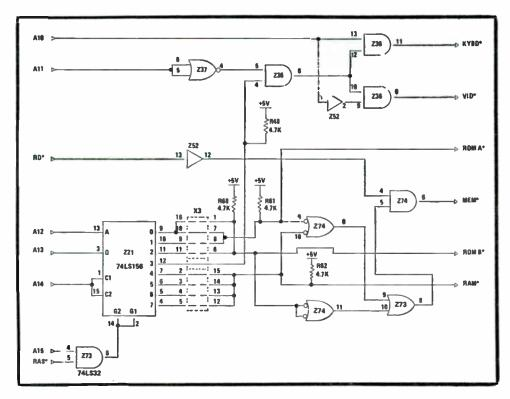
Fig. 12-14. Drawing of address decoder.
