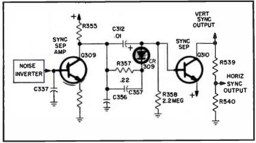
Fig. 3-46. Transistor sync separator circuit.
