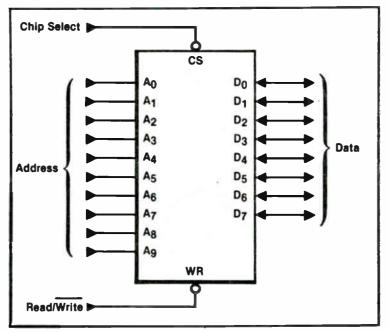
Fig. 12-8. Drawing of a 1K × 8 RAM chip.
