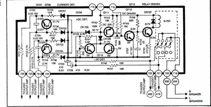
Fig. 5-15. Automatic speaker protection circuit.
