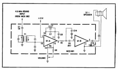
Fig. 3-45B. Simplified schematic MDS 001.
