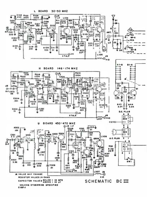
Fig. 8-8. Complete schematic for BEARCAT III crystal scanner.
