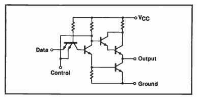
Fig. 12-4. Diagram of three-state driver.
