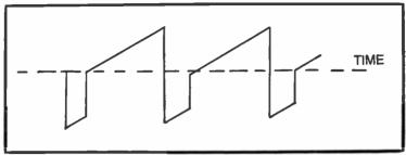
Fig. 3-11. Trapezoidal waveform for the vertical sweep.
