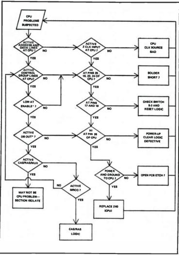
Fig. 12-19. CPU section isolation flowchart.
