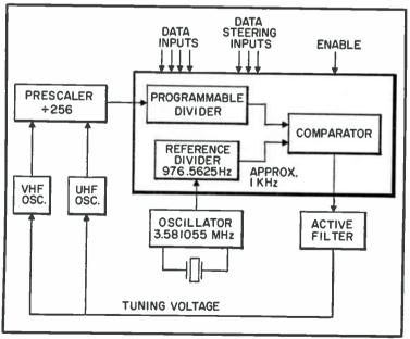
Fig. 1-4. Phase locked-loop block diagram.
