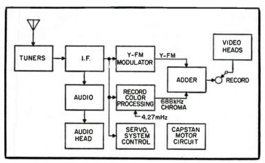
Fig. 10-4. Block diagram of record mode.
