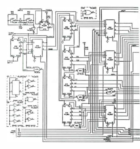
Fig. 12-12. Diagram of TRS-80 (section 2).
