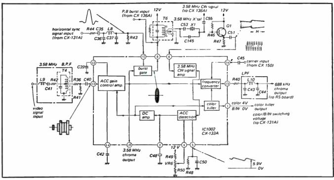
Fig. 10-9. Record chroma signal processing circuit.
