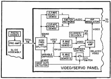
Fig. 11-12. Signal processing block diagram.
