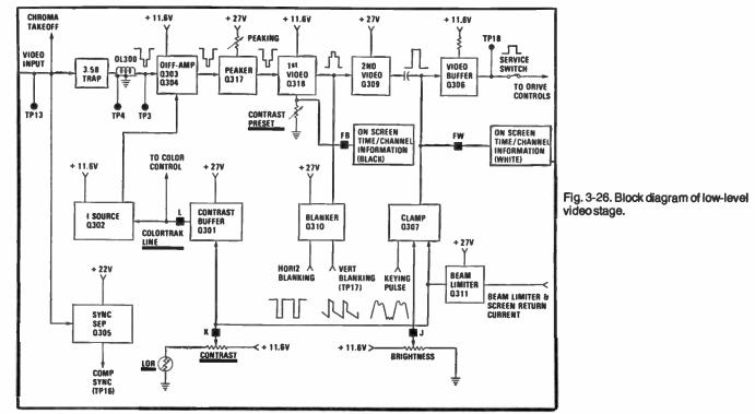
Q301 may be open. Check diode CR306. If this diode is shorted the contrast control will not operate.
