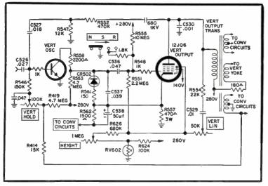
Fig. 3-8. Vertical oscillator and output circuit.
