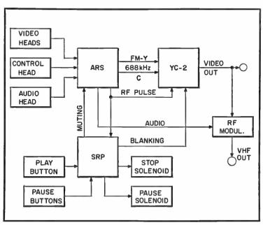
Fig. 10-15. Block diagram of KR9000 units playback mode.
