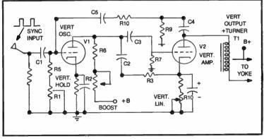
Fig. 3-10. Simplified diagram of a multivibrator.
