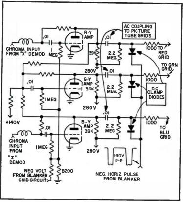
Fig. 3-44. Color difference amplifier circuits.
