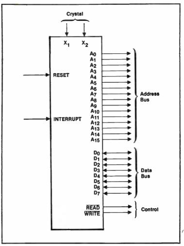
Fig. 12-5. Basic microprocessor signals.
