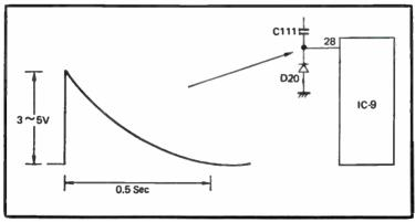
Fig. 8-11. Initializing waveform.
