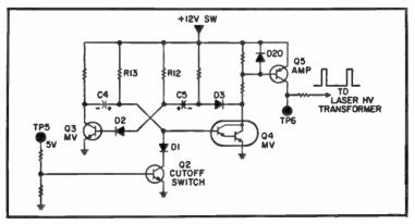
Fig. 11-10. Laser multivibrator circuit.
