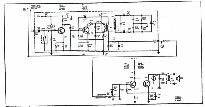
Fig. 4-20. Audio IF and sound output circuits.
