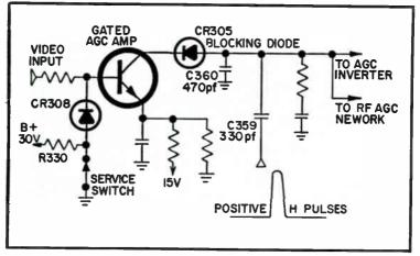
Fig. 3-48. Gated AGC amplifier circuit.
