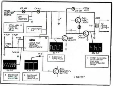
Fig. 3-3. Count-down circuit with waveform checkpoints.
