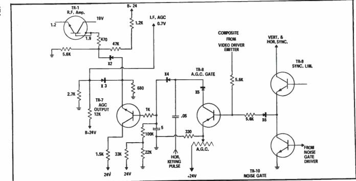
Fig. 4-19. Transistor AGC circuit-gated.
