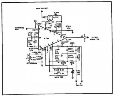
Fig. 5-10. FM Multiplex circuit (chip).
