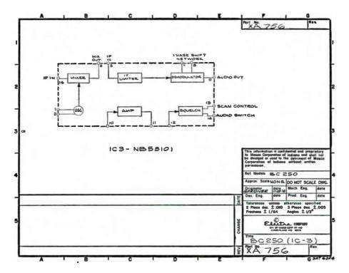
Fig. 8-3. Block diagram of IC3.
