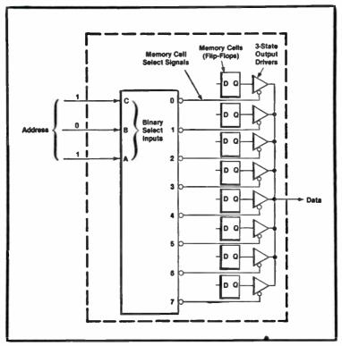
Fig. 12-6. Drawing of eight-bit memory.
