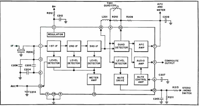
Fig. 5-8. Block diagram of FM IF chip.
