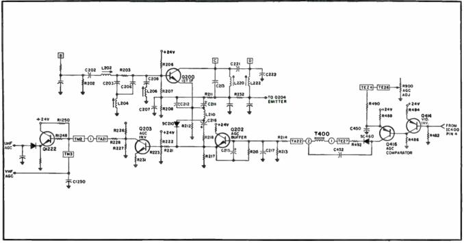
Fig. 3-49. Transistor AGC circuit.
