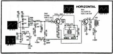
Fig. 4-11 Horizontal oscillator and driver circuit.
