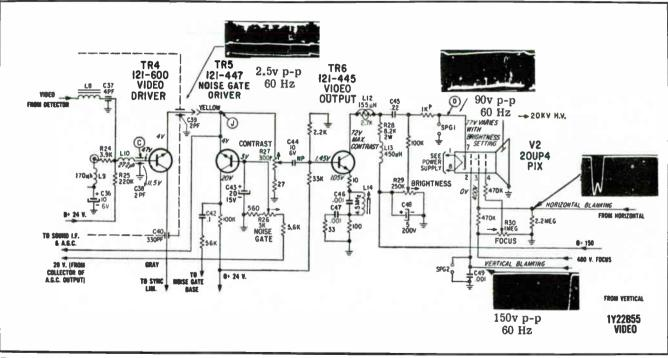
Fig. 4-17. Video amplifier circuit.
