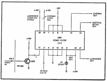
Fig. 3-38. Simplified comb filter diagram.
