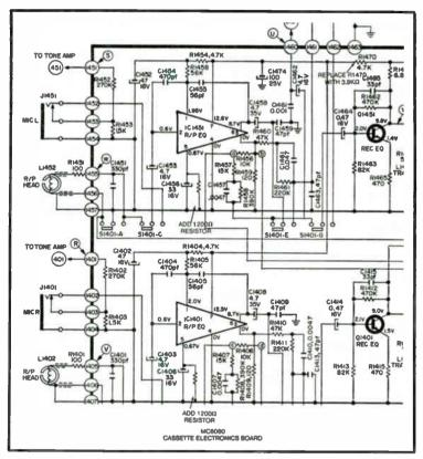
Fig. 7-5. Cassette electronic circuits (stereo).
