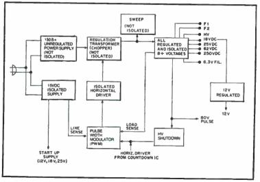
Fig. 3-52. Block diagram of the Electronic Power Supply.
