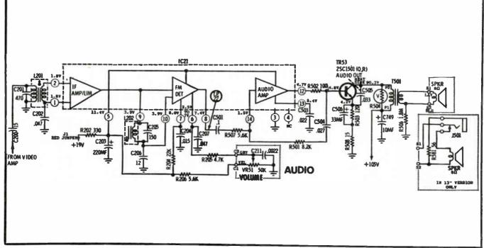
Fig. 4-10. Audio system - IC type.
