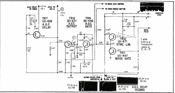
• The AGC gate transistor (TR9) develops a bias proportional to sync tip amplitudes as a gated rectifier. This is fed to the AGC output transistor (TR8) at test point "F" whose emitter is used as follows:
