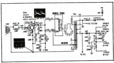
Fig. 4-5. Horizontal sweep output stage.
