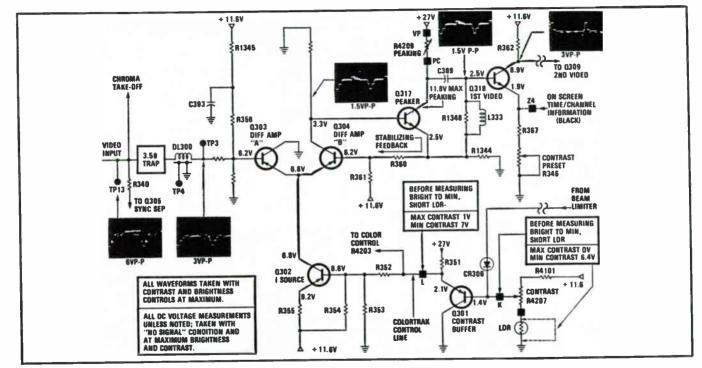
Fig. 3-24. Low-level video stage with check points.
