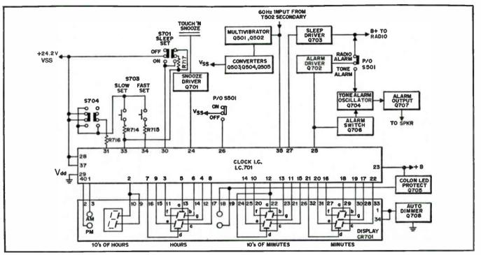
Fig. 9-1. Simplified digital clock readout circuit.
