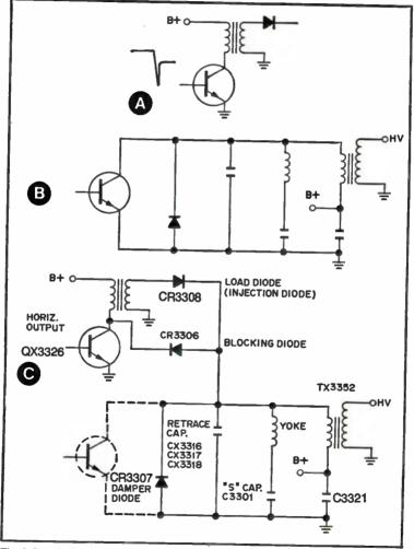
Fig. 3-54A-B-C. Simplified regulator and horizontal output circuit.
