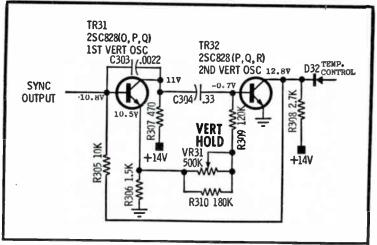
Fig. 4-2. Vertical oscillator and sawformer.
