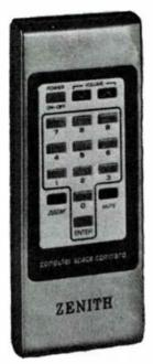
Fig. 2-1. Zenith 2000 remote transmitter.
