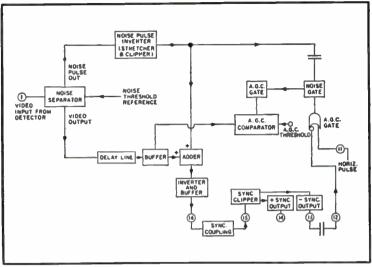
Fig. 3-19. Block diagram of the noise protection circuit.
