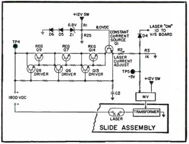
Fig. 11-9. Laser supply regulator circuit.
