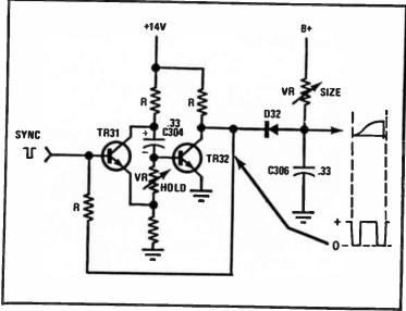
Fig. 4-1. Transistor type vertical oscillator circuit.
