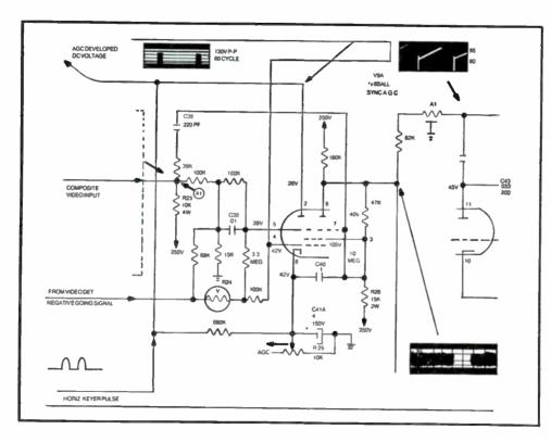
Fig. 3-50. Tube-type sync/AGC circuit.
