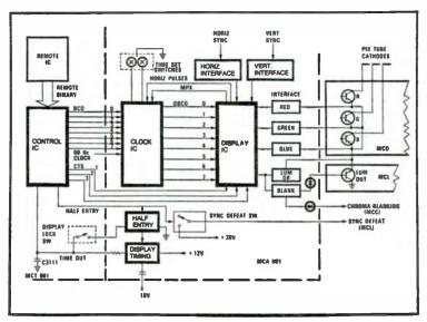
Fig. 9-6. Direct address display system.
