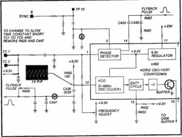
Fig. 3-1. Horizontal count-down block diagram.
