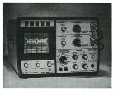
Fig. 5-19. SENCORE model SC60 dual-trace oscilloscope.
