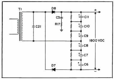
Fig. 11-7. Laser power supply circuit.
