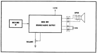
Fig. 3-45A. Block diagram of IC sound circuit.
