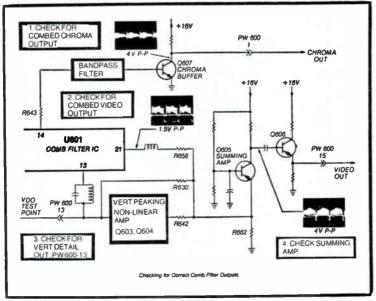
Fig. 3-41. Correct comb filter output signals.
