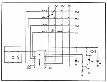
Fig. 2-4. Circuit for 124-14 hand unit.
