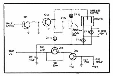
Fig. 9-11. Display timing circuitry.
