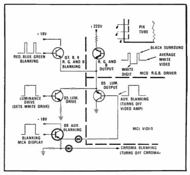
Fig. 9-9. Display - Video Drive for Digit No. 1.
