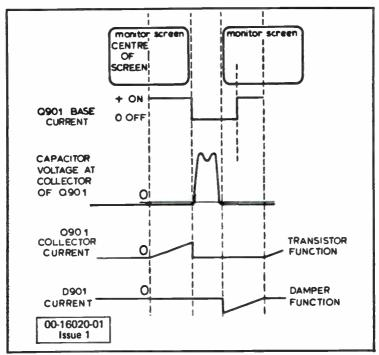
Fig. 4-14. Waveforms for horizontal scan system.
