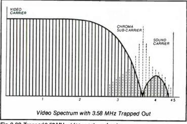
Fig. 3-39. Trapped 3.58 MHz video spectrum drawing.
