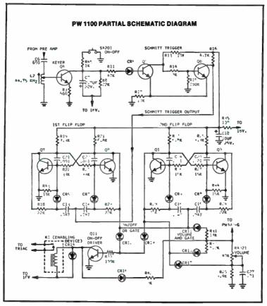
Fig. 2-10. Partial schematic of an RCA remote unit.
