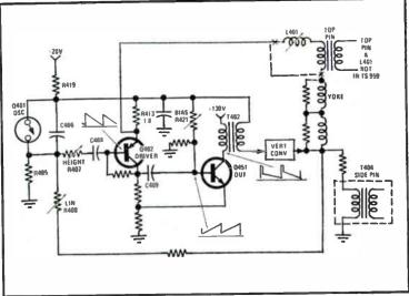
Fig. 3-69. Transistor type vertical sweep circuit.
