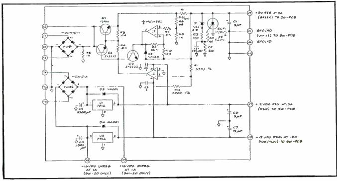
Fig. 12-22. Circuit diagram for SOL-20 power supply.
