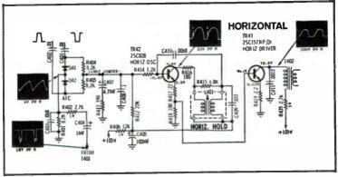
Fig. 4-4. Horizontal AFC and oscillator.
