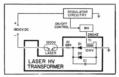
Fig. 11-8. Laser and High Voltage transformer.
