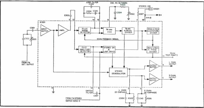
Fig. 9-4. Block diagram of FM multiplex decoder.
