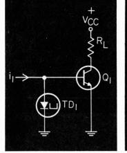
Fig. 1. Widely-used tunnel-diode threshold circuit has the disad-vantage of high hysteresis.
