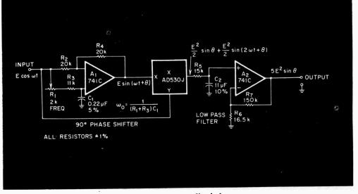
Two IC op-amps and a multiplier form a frequency discriminafor circuit.
