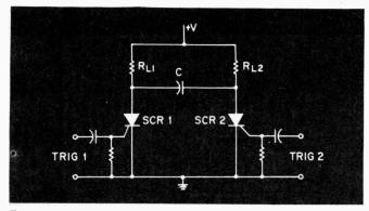
Fig. 1. A conventional SCR flip-flop which has latch-up problems.
