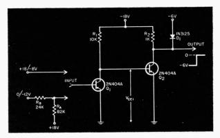
Logical-level couverter with two input circuits for common commercial equipment.
