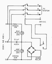
The proper phase rotation is indicated by lamp ABC, which is paralleled with a full-wave bridge and relay circuit to connect the source to the system.
