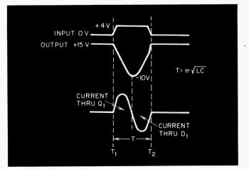
Fig. 2. Typical waveforms for the resonant line driver. During the positive half-cycle current flows through  $Q_{i}$ , and during the negative half cycle it returns via  $D_{\mu}$ .
