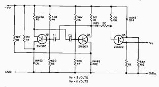
Square wave generator for variable pulse widths and variable interval between pulses.
