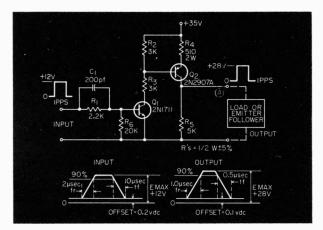
Fig. 1. Single power supply pulse amplifier. Fig. 2. Input and output waveforms.
