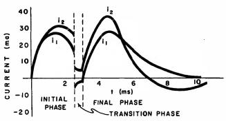
FIG. 2—Current in latching relay coils with 30v input.
