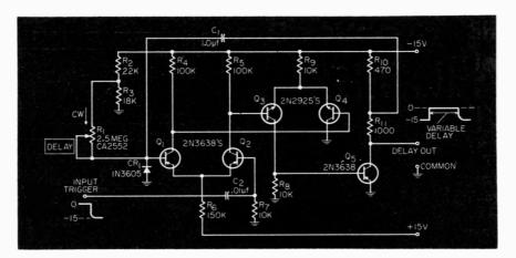
Wide-range, continuously variable delay is set by log-taper pot R<sub>1</sub>.
