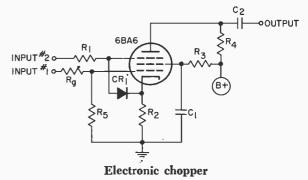
is too much distortion  $R_2$  can be raised, although an adjustment of  $R_4$  may be necessary.
