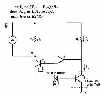
FIG. I—Circuit for measuring dc beta at low current.
