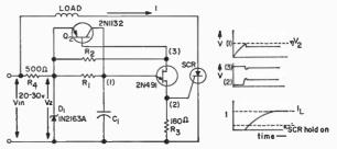
The unijunction latchup circuit for scr's turning on inductive loads and circuit waveforms.
