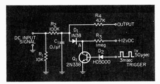
Clearing circuit for R<sub>2</sub>-C<sub>1</sub> integrator network.
