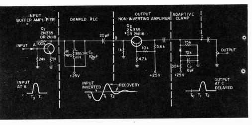
dB. A greater range is possible Fig. 1. With the component values shown, this circuit (positive-input version) provides 6-ms direction so the output is like delay over a 25 to 150-Hz frequency range. The output follows the input over a 30-dB range.
