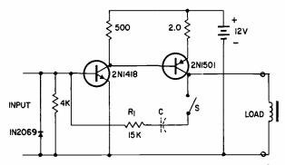
FIG. I—Universal dc amplifier, pulsed relay, pulse stretcher schematic.
