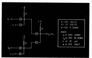
Fig. 2. Common 2-input diode gate.
