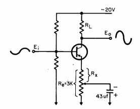
Transistor amplifier stage allows gain to be changed over a large frequency variation without effecting the dc bias.
