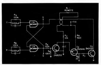
The timing resistor for this resettable one-shot can be several feet away from the circult without allowing noise to fire the circuit.
