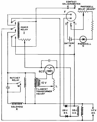
FIG. 2-Solenoid drive circuit for pendulum.
