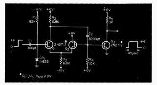
Fig. 2. Improved one-shot output circuit.
