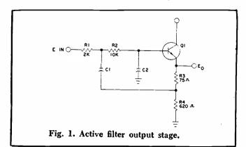
pends on some transistor parameters such as  $r_e$ ,  $\beta$ , and the location of the poles determined by  $R_1C_1$  and  $R_2C_2$ .
