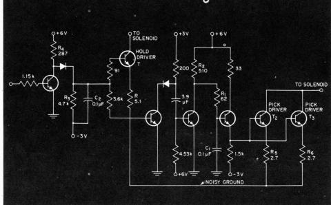
To eliminate transient noise problems, networks R, R, C, R, R, and R, R, C, R, control the switching speed of high-current drivers  $T_{ij}$ ,  $T_{ij}$  and  $T_{ji}$ .
