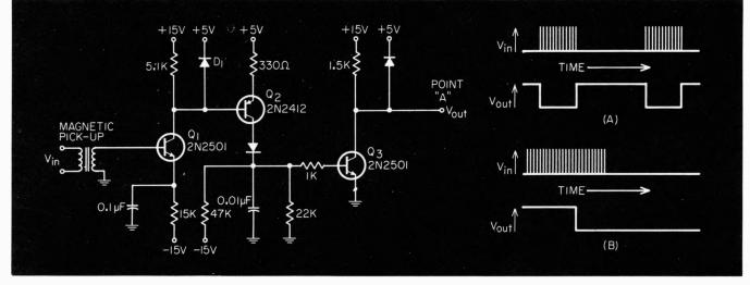
Fig. 1. Basic circuit is a pulse-train detector. If D<sub>1</sub> is returned to point "A", circuit will give an output after counting specified number of pulses.
