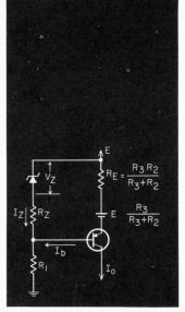
Fig. 2. To simplify the analysis, the circuit of Fig. 1 has been redrawn to show the Thevenin-equivalent generator and impedance in the emitter circuit.
