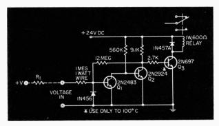
Low-level current-detector Schmitt circuit.
