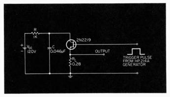
Fig. 1. Switching circuit with transistor driven into second breakdown to give 40-nsec pulses at 30-A peak.
