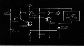
Delay is set by  $R_1C_1$  time constant.
