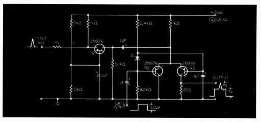
This transmission gate for fast pulses operates in a current-switching mode. The pedestal  $e_p$  on the output pulse is caused by bias current in  $Q_3$ .
