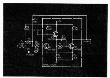
This detector circuit is similar to a Schmitt trigger but buffer amplifier  $Q_i$  is included in the feedback path.
