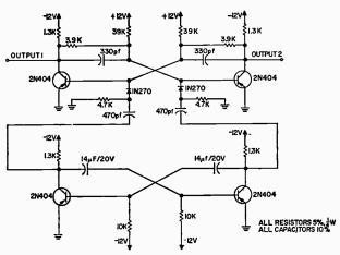
Fig. 2. Symmetrical 5 cps astable multi with flip flop waveform squaring.
