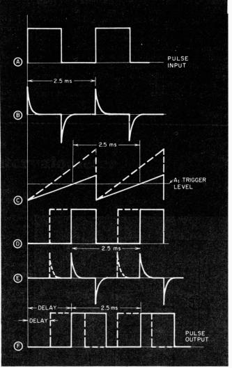
When the input goes positive,  $Q_{s}$  turns on and discharges  $C_{s}$ . Negative excursions are bypassed by  $CR_{I}$ . When the input goes low at the end of the positive excursion, voltage comparator A, senses the low voltage and its output goes low.  $C_{t}$  begins to charge through the variable current source  $(R_1R_2R_2Q_1)$ , which determines the slope of the charging curve.
