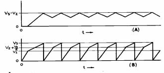
FIG. 2. Output of waveform generator (A) and waveform across C<sub>1</sub> (B)
