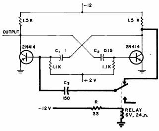
Starter circuit for stalled free-running flip-flop.
