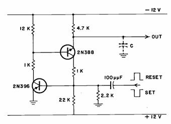
Capacitive load in emitter circuit increases gain.
