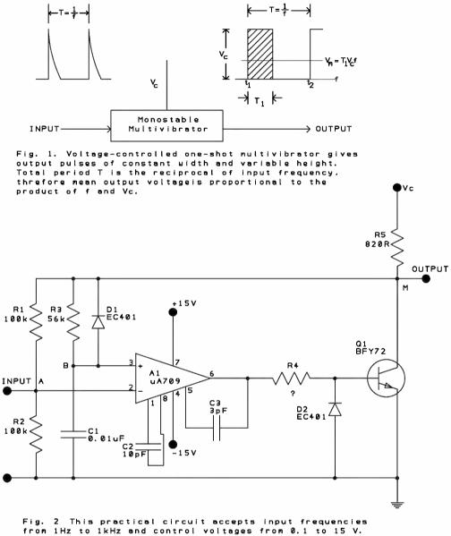
from 1Hz to 1kHz and control voltages from 0.1 to 15 V. Note that voltage balance between points A and B doesn't depend on Vc. Therefore pulse widthdepends only on the values of R3 and C1.
