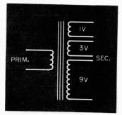
Windings required for transformer giving 1 to 13 V in 1 V steps.
