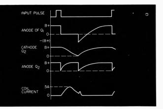
Fig. 2. Typical waveforms for the delay-flop circuit of Fig. 1.
