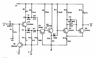
FIG. 1—Circuit of pulse amplitude evaluator.
