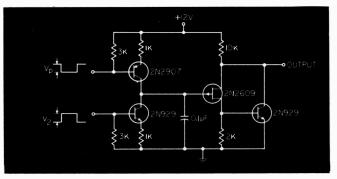
Fig. 2. Simplified pulse integrator with typical component values.
