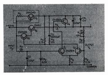
Fig. It In this voltage regulator, the FET constant-current source (inside the dashed rectangle) provides improved regulation, because current through CRi is independent of input and output voltages.
