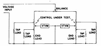
FIG. 2—Final circuit for measuring difference in attenuation between two tandem controls.
