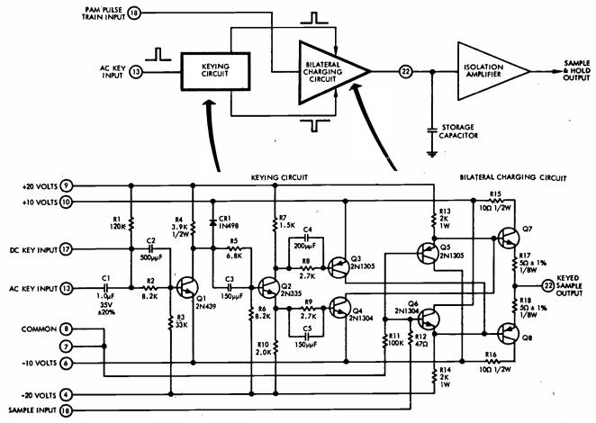
FIG. I—Sample and hold circuit with bilateral charging. Transistor  $Q_7$  is a 2N1304 and  $Q_8$  is a 2N1305. ities, in the order of 200 ma, and essentially all of the current is supplied by the 10-volt supplies. This puts hardly any current requirements on the source and it is effectively used only to catch the voltage on the holding capacitor through a near unity voltage gain, high current gain amplifier.
