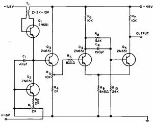
Fig. 1-Rectangular waveform generator.
