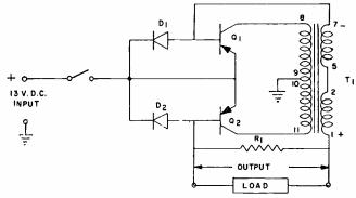
Complete circuit of simple 60-cycle inverter.
