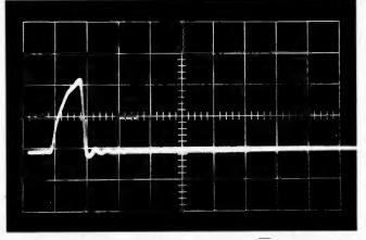
Fig. 2. Typical output waveforms from the Q terminal (top) and the Q terminal (bottom). Vertical scale is 2 V/div and horizontal scale is 100 ns/div.
