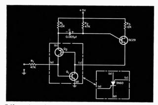
Self-resetting pulse stretcher. Gate turn-off SCR can be used instead of two transistors.
