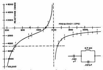
FIG. 4—Network reactance plotted against frequency.
