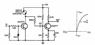
Fig. 1. Dynamic range compressor limits on any negatime imput signal without a saturation level. (left) Fig. 2. The transfer characteristics  $E_{out}/E_{in}$  illustrate cube root proportionality. (right)
