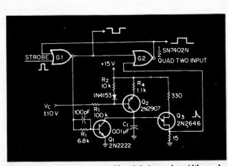
Fig. 1. This one shot is capable of being pulse-width modulated by V. It is capable of high duty cycles and can supply complementary outputs.
