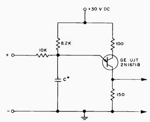
Voltage controlled variable frequency oscillator.
