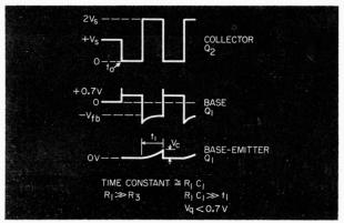
Fig. 2. Waveforms.
