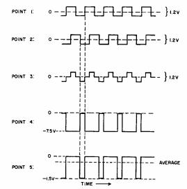
Fig. 2. Waveforms in phase comparator.
