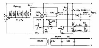
FIG. 2—Circuit of transistor beta checker.
