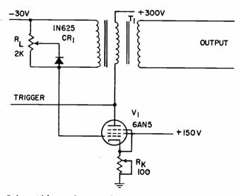
Pulse width can be varied over a range of four to one by adjusting the diode current.
