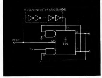
Fig. 1. This simple one-shot uses the propagation delay of cascaded inverters, instead of an RC network, to define its recovery time.
