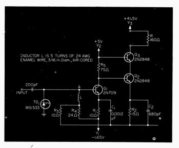
Tunnel diode TD,, in this simple word-line driver, acts as a one-shot to give fast switching speed and adjustable recovery time.
