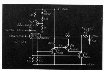
Fast and accurate sample-hold circuit. Matched transistors  $(\mathbf{Q}_1, \mathbf{Q}_2)$  give low offset between the sampled input and held output.
