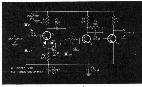
Fig. 1. Signal powered sine-to-square-wave converter schematic.
