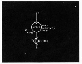
meter. This resistance is neg-voltage to the FET, cutting it ligible compared to the meter off and preventing excessive resistance. When the zener meter current. diode conducts, it applies gate
