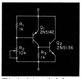
This circuit is particularly useful in the 1- to 3-V range, where conventional zeners have much higher impedance.
