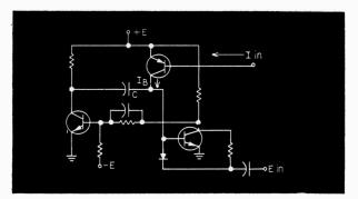
Fig. 1. Limited-range PWM circuit.
