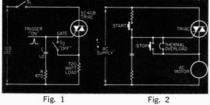
Fig. 1. AC latching switch. Fig. 2. AC motor starter.
