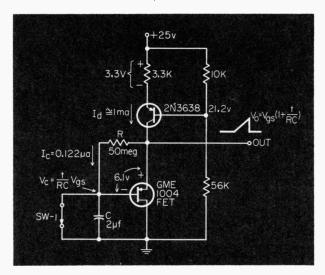
Fig. 2. Ramp generator circuit.
