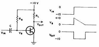
FIG. I—Small noise pulses are amplified in a conventional multivibrator.
