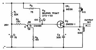
Change of dc input to power supply is accomplished by this low-frequency switching circuit. Adjust R, for best symmetrical waveform at relay contacts (time on-time off).
