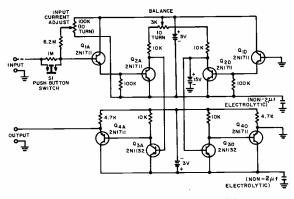
Fig. 2. Practical two-stage preamplifier.
