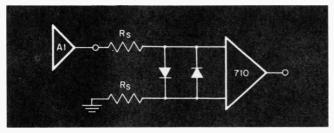
Fig. 1. Usual comparator protection circuit which introduces an error of I aff Rs.
