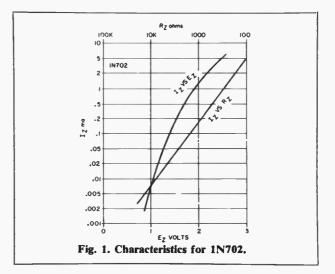
characteristics of the 1N702 are shown in Fig. 1, while Fig. 2 shows a phase-shift oscillator  $(Q_1)$  in which the gain is controlled by coupling a 1N702 zener diode,  $CR_1$ , across the emitter resistor.  $(C_5, C_6, R_7)$  is a non-polar capacitor combination.)
