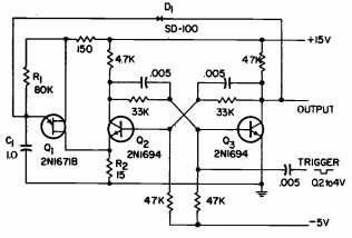
Timing interval of this circuit can be varied from 10 millisec to 0.3 second.
