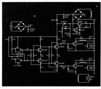
Fig. 2. This improved inverter circuit has an efficiency of about 90 perceut at output frequeucies of 20 KHz or higher. Also, the circuit has good voltage regulation and the frequency doesu't chauge with load curreut.
