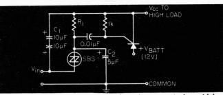
Simple switching circult uses a bilateral trigger device which provides a high input impedance and draws negligible standby current.
