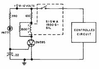
Voltage-limit sensing circuit.
