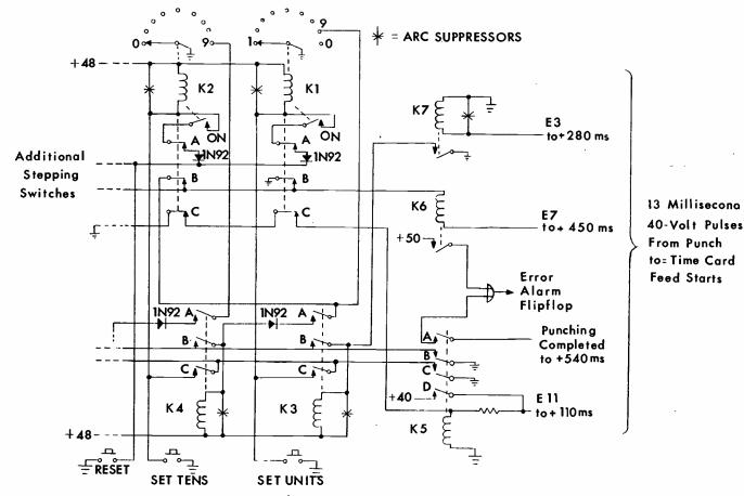
FIG. 1—Counter circuit using stepping switches.
