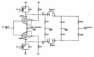
FIG. 2—Circuit of low frequency discriminator.
