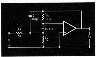
Value of Rc determines the center frequency of this band pass filter. Adjustment has no effect on bandwidth.
