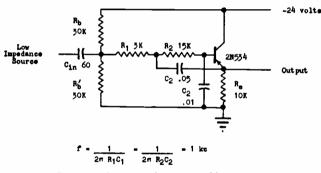
FIG. I—Circuit of active low pass filter.
