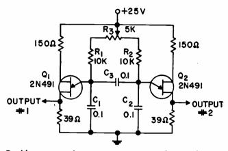
Double-output pulse generator consists of two relaxation oscillators synchronized by capacitance.
