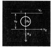
Fig. 2. Basic thermistor sensing circuit. Output  $V_i$  can be used to trigger a breakdown diode, or R, can be replaced by a relay.
