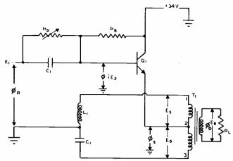
FIG. 2-Suggested values:  $R_{IJ} = 100$ K;  $R_{IJ} = 18$ K;  $C_1 = 1500 \ \mu\mu f$ ;  $C_2 = .047 \ \mu f$ ;  $Q_1 = TI2N1050$ ;  $T_1 = 1:1.4$ , 10 kc;  $L_1 = 2.4$  mh in series.
