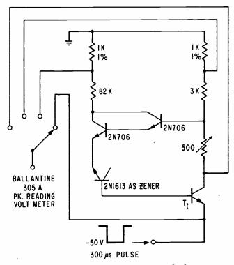
FIG. 2—Pulses permit measurements at higher current.
