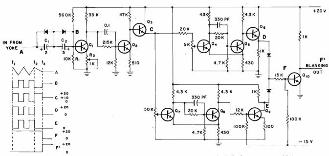
FIG. 2—All transistors of the sweep alarm are type 2N1302 and all diodes are type 1N497.  $R_{21}$ ,  $R_{31}$ ,  $R_{4}$  are Bourns 275 Trimits.
