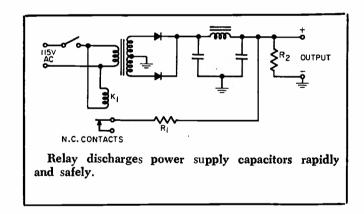
THE RESIDUAL charge on power supply capacitors maintains an output voltage for a considerable time after shutting off the input power. This is objectionable for the testing of computer flip-flop modules, where a zero starting voltage is required.
