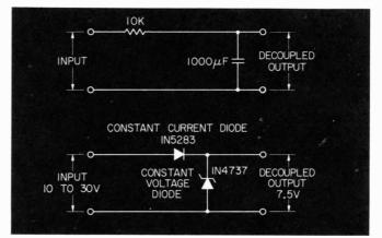
The conventional decoupling circuit at the top uses large components, yet it's not effective at low frequencies; it introduces phase shift and increases the possibility of low-frequency oscillation. The bottom circuit eliminates these problems, offering high attenuation from dc to high frequencies.
