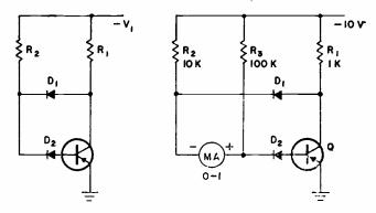
FIG. 1—Antisaturation circuit and Fig. 2 (right) complete circuit of beta tester. A Philips goldbonded Ge OA5 is. used for  $D_1$  and a Philips Si OA200 for  $D_2$ .
