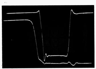
Fig. 2. Typical input (bottom) and output (top) waveforms for the circuit of Fig. 1. Horizontal scale is 10 ns/div. and vertical scale is 1 V/div.
