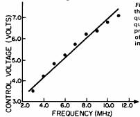
Fig. 2. Linearity is better than 5% of full-scale fre-quency. Above 5 MHz, frequency is approximately proportional to the product of control voltage and timing capacitance.
