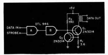
This line-driver circuit offers simplicity with current limiting and signal-return isolation. Any DTL or TTL NAND gates can be used at the input.
