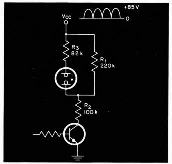
Low-cost, low-power neon indicator drive circuitry.
