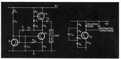
Fig. 1. This self-oscillating vertical-deflection circuit for small-screen black-andwhite TV requires no choke. But it is quite inefficient.
