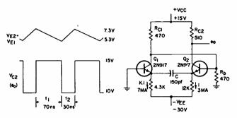
FIG...I—Current switching astable multivibrator and its waveforms.
