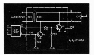
Fig. 1. Electronic audio switch.
