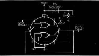
Dual-gate IC, plus external RC network, forms a simple oneshot. Temperature stability can be improved by using a Sensistor as shown.
