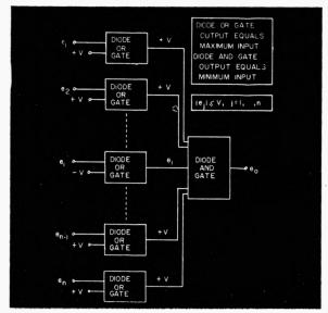
Fig. 1. Analog selection switch. The only gate that switches is the one with -V applied.
