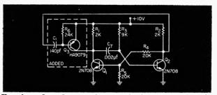
Transistor  $Q_3$  reduces timing capacitot's charging time, increasing the duty cycle.
