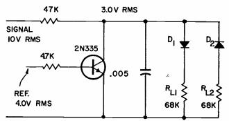
FIG. I—Voltage appears across either of the two load resistors depending upon polarity of input signal.
