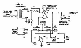
Converter changes 50-17000 cps sine waves to saw-tooth or square waves.
