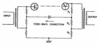
FIG. I—Simplified schematic of bridge feedback amplifier.
