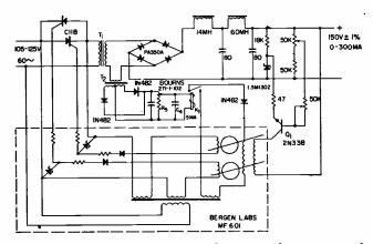
FIG. 2—High-efficiency circuit for 150-volt output and one per cent regulation.
