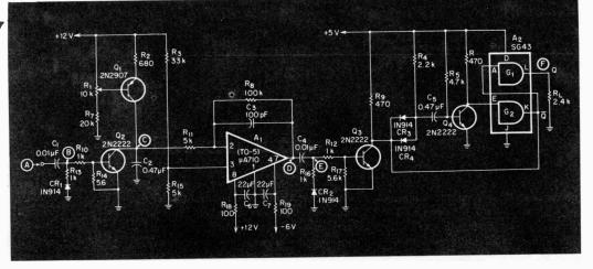
Fig. 1. This circuit provides variable apparent delay for a 400-Hz square wave, but it actually "reconstructs" the square wave.
