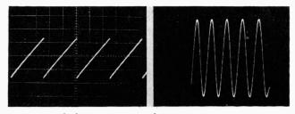
Linearity of the sweep waveform is apparent in Fig. 2, left. Some 10-kc sine waves using the four-layer diode for sweep are shown in Fig. 3, right.
