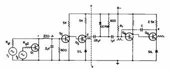
FIG. 2—Circuit to left of dashed line is used for method shown in Fig. 1A, complete circuit is needed for second method, in Fig. 1B. Collector resistor for  $Q_4$  is 2.5K.
