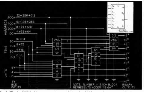
Fig. 1. Simple BCD-to-binary converter uses IC quadruple binary adders to sum the binary equivalents of the parallel BCD inputs.
