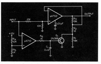
Automatic scaling circuit gives two meter ranges. With values shown here, scales are 1 V and 10 V fsd.
