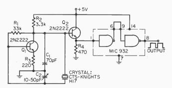
Fig. 1. Simple 1-MHz clock oscillator operates from +5 V supply and gives output levels compatible with digital ICs.
