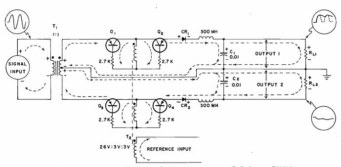
The phase sensor circuit employs Motorola 2N651A transistors. All diodes are IN645A.
