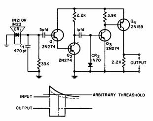
Logarithmic amplifier for radar signals
