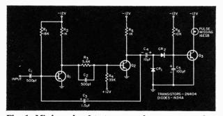
Fig. 1. Missing-pulse detector responds to narrow pulses.
