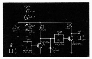
Z-axis modulation circuit.
