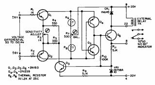
Fig. 1 Voltage comparator.
