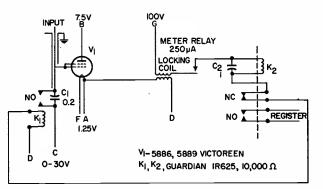
FIG: 1—Circuit of current integrator. Lettered leads connect to power supply leads of Fig. 2.
