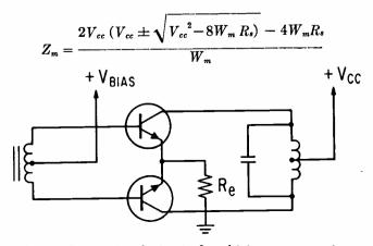
FIG. I-Conventional circuit for driving servo motors.
