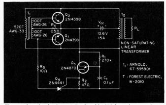
The starting circuit (Q<sub>3</sub> and Q<sub>4</sub>) for this 400-hertz inverter draws negligible quiescent current - thus it doesn't detract from the inverter's efficiency.
