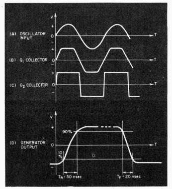
Fig. 2 Typical waveforms at various points in circuit shown in Fig. 1.
