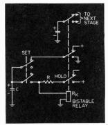
Fig. 1. Bistable relay circuit with capacitor transfer. When used for binary register ap-plications, the "set" contacts shown are part of the bistable relay for the preceeding stage.
