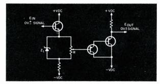
Fig. 1. Basic voltage-control circuit.
