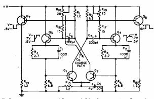
Pulse generator provides variable frequencies from low impedance pulses. All resistors are in kilohms, 10 percent,  $\frac{1}{2}$  w; all transistors are 2N35 or similar: all unmarked capacitors are in picofarads.
