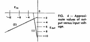
acteristic of this circuit is shown as the crossed line in Fig. 4.
