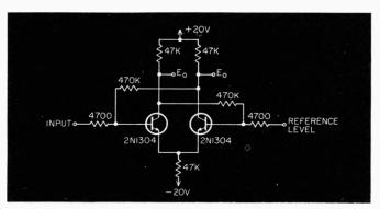
Stable state of this circuit changes when input level crosses the reference level. Output is taken from either collector.
