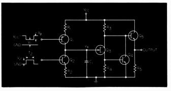
Fig. 1. Constant-current charge and discharge circuit integrates pulses.
