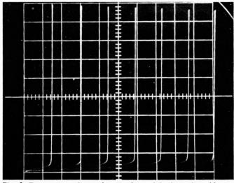
Fig. 2. Zener curves for various settings of R, from 0 to 10 k $\Omega$ . Vertical scale is 2 mA/div, horizontal is 0.5 V/div.
