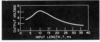
Fig. 2. Typical delay-circuit output as a function of input pulse length
