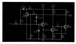
Fig 1. Variable-hysteresis Schmitt trigger.
