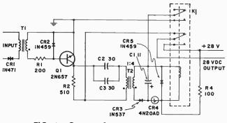
FIG. I—Circuit of integrating amplifier.
