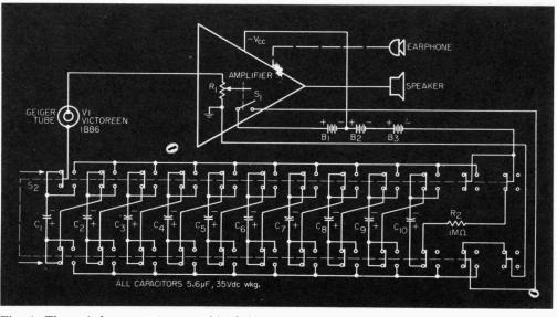
Fig. 1. The switched capacitors in this Geiger-counter circuit provide the high voltage for the Geiger tube.
