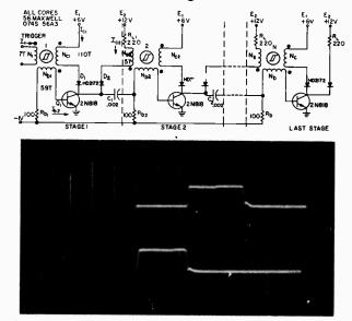
A single trigger pulse is transmitted from stage to stage, saturating each transistor and then turning the transistor off as the induced voltage drops to zero. Adjacent-stage outputs are shown (50 ma/div vert. and 5  $\mu$ sec/div hor).
