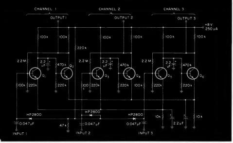
sections. Bias voltages are This 3-input amplitude comparator is based on repetitive 2-transistor sections that lend chosen so that only one input themselves to construction of an n-input comparator. The transistors are 2N4286.
