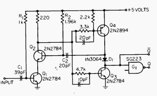
, Fig. 1. The push-pull action of Q3 and Q4, and the unusual trigger circuit (Qi, Ri, Ci), allows this one-shot to generate extremely fast pulses.
