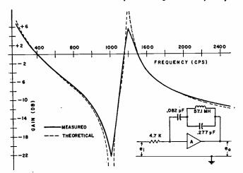
FIG. 5—Theoretical and actual circuit gain.
