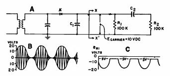
FIG. I—Diode a-m detector and inherent clipping effect.
