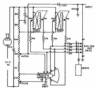
FIG. I—Servo motor is coupled to sine-cosine potentiometer for target bearing indicator.
