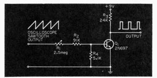
Simple pulse source uses scope output.
