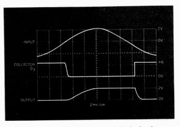
Fig. 2. Typical waveforms for the peak-hold circnit using component values shown in Fig. 1.
