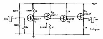
FIG. I—Direct coupling and use of complementary transistors produces pulse amplifier chary of quiescent current.
