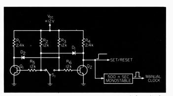
Manual no-bounce pulse generator for testing digital circuits. on the circuit. This is because ates a short pulse each time all input pulses are of the same the switch is pushed. Rise time polarity (positive-going for the of  $Q_1$  determines rise time of circuit shown).
