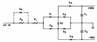
FIG 3-Addition of diode Da permits odjustment of current.
