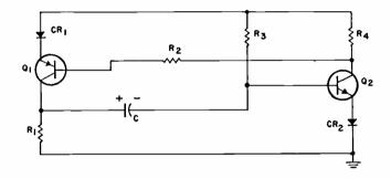
FIG. 1-Circuit of fast recovery monostable multivibrator.
