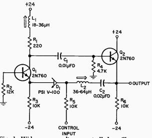
Fig. 1. Wide range, voltage controlled oscillator.
