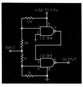
Fig. 1. Universal interface circuit gives +3 volts output with zero input and zero output with positive or negative nonzero inputs.
