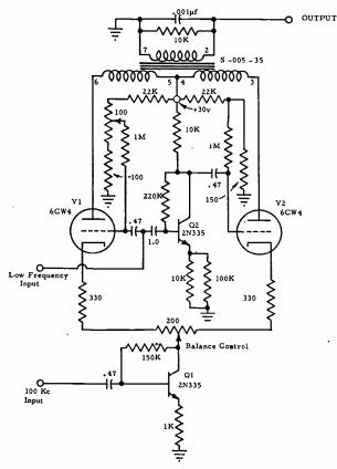
Fig. 1. Hybrid Balanced Modulator for 100 Kc.
