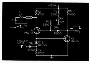
Opposite polarity transistors allow fast recovery with broad width control.
