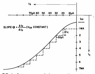
FIG. I—Beta curve on which tester is designed.
