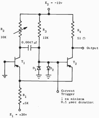
FIG. 1—Current switching monostable multivibrator uses two IN266G silicon diodes and two 2N384 transistors.
