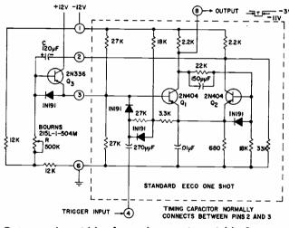
Output pulse width of one-shot mv is variable from one second to one minute.
