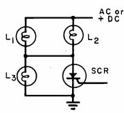
Fig. 1. Basic inversion circuit for incandescent lamp readout.
