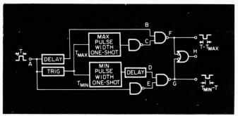
Fig. 1. Pulse-width discriminator in block-diagram form.
