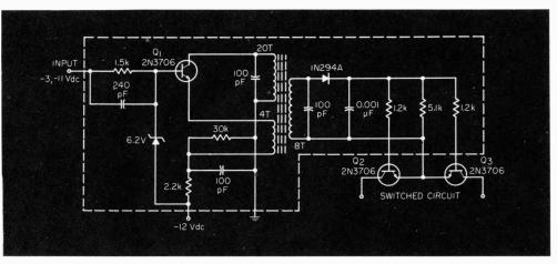
Solid-state switch driver replaces conventional relays.
