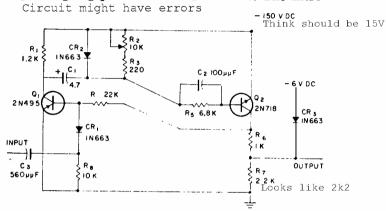
Neither transistor of this monostable multivibrator conducts until an input pulse is applied.
