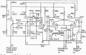
Pulse width modulator circuit.
