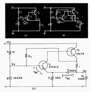
Fig. 1. Two-transistor voltage regulator; a. without feedback; b. with positive feedback; c. with positive feedback and temperature compensation.
