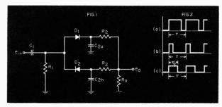
Fig. 1. Square-wave symmetry detector. Fig. 2. Typical rectangular waveforms.
