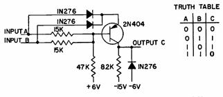
FIG. I—Transistor conducts when inputs are different levels.
