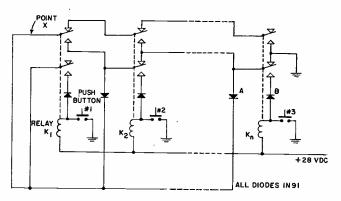
FIG. I—Diodes permit clearing other relays when one pushbutton is pressed.
