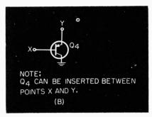
Fig. 2. Oscillator doubles as power driver with extra driver transformer. Power capabilities can be increased by adding transistor as shown in 2b.
