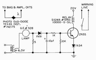
Fig. 1 Photocell lamp burnout warning circuit.
