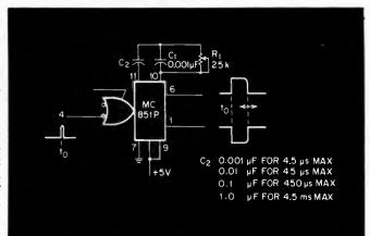
ommended range of external put pulse are better than 100 A simple modification of the MC851P monostable extends out**a** put pulse widths from 4.5  $\mu$ s to 4.5 ms.
