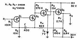
Gain of the high-impedance input amplifier is 13 and output impedance is 20 ohms. Frequency response ranges from 0.5 cycle to 20 kc.
