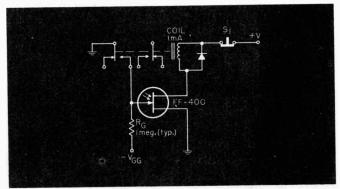
Photosensitive FET gives light-activated latching relay.
