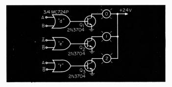
Fig. 2. A decoder circuit can use the remaining three gates of a quadruple dual-input IC. With the transistors shown here, the circuit will drive loads of up to 250 mA.
