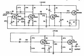
Wide range of input voltage is handled by this agc amplifier.
