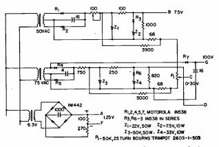
FIG. 2—Rectifiers R3 and R6 each consist of three in series.
