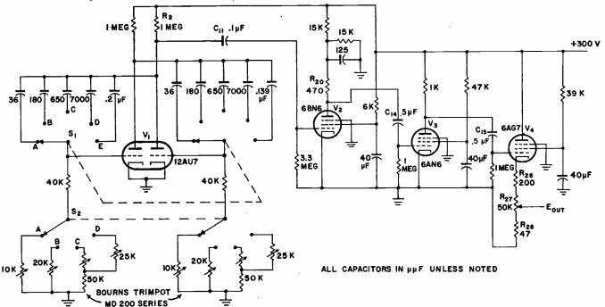
FIG. I—Test generator using gated-beam concept.
