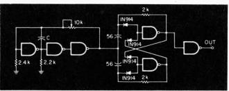
A single IC is used to form a wide range, buffered, square-wave generator.
