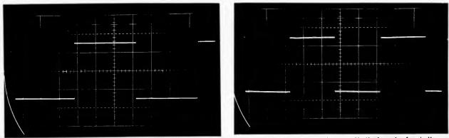
Fig. 2. Output waveform is excellent over a wide frequency range, as shown in these scope pictures. Vertical scale for both waveforms is 1 V/cm. Frequencies are 30 Hz (left) and 100 kHz (right). Horizontal scales are 5 ms/cm and 2 µs/cm respectively.
