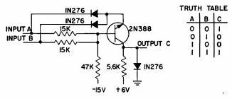
FIG. 2—Logic circuit for use with an npn transistor.
