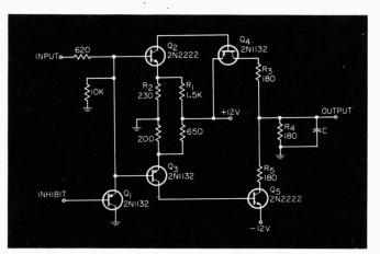
Positive pulses at input give  $\pm 6$  V balanced pulses at output. If inhibit terminal is grounded, output is held at -6 V.
