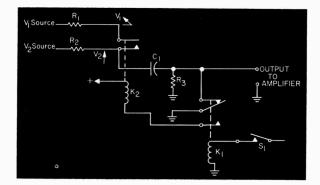
Fig. 1. Voltage comparator circuit.
