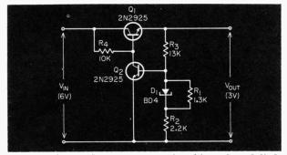
Fig. 2. Series regulated power supply with backward-diode reference.
