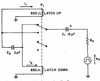
FIG. I—Magnetic latching relay flip-flop.
