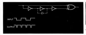
Fig. 2. Changing the output NAND to an exclusive OR converts OR gates enables the designer are available in both TTL and the circuit to a frequency doubler.
