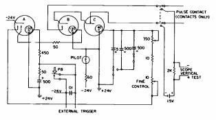
Circuit produces pulses from 10 microsec to 200 msec in length.
