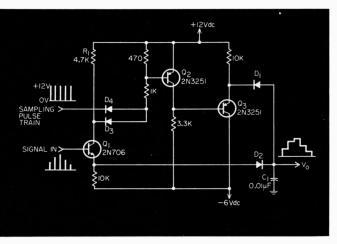
collector voltage of  $Q_i$  drops Sample-and-hold circuit in which a new signal level is sensed below +12 V because of the only when a sampling pulse arrives at the other input.
