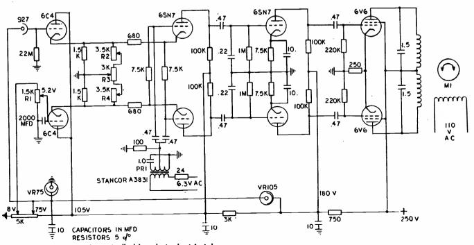
Low cost servo system is controlled by photoelectric tube.
