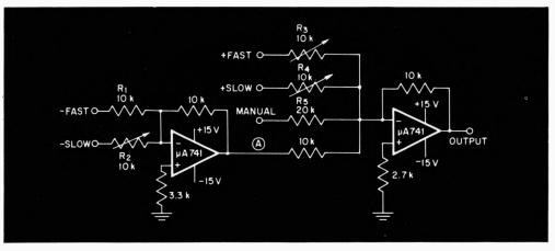
This circuit interfaces between digital or bipolar analog signals and a bi-directional servo.
