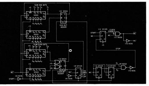
lows us to achieve an add time Fig. 2. Practical circuit for an 8-bit split serial adder.
