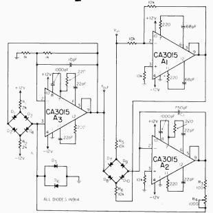
Fig. 1. IC op amps simplify the design of this VCO which gives a triangular wave at the output of  $A_2$  and a square wave at the output of A<sub>3</sub>.
