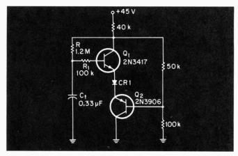
Fig. 3. Another modification of Fig. 1 allows one to generate very low frequencies but sacrifices temperature stability.
