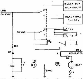
FIG. I—Circuit for switching voltages from an industrial test line.
