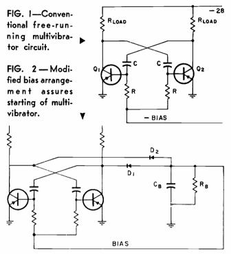
shown in Fig. 1. On initial turn on, or if in use with test equipment, both capacitors are switched simultaneously, and conditions may arise in which both  $Q_1$  and  $Q_2$  will be fully conducting. (Amount of saturation is determined by R and the negative bias voltage.) With both  $Q_1$  and  $Q_2$  saturated, their incremental gain is low. Loop gain may not be sufficient to ensure oscillation.
