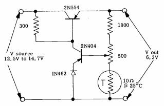
Fig. 1 Low cost transistor voltage regulator.
