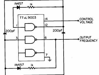
Fig. 1. High-frequency VCO uses cross-coupled IC gates. TTL logic allows oscillation frequencies of 25 MHz or higher.
