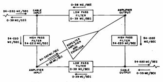
FIG. 1-Modified repeater station.
