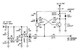
Circuit of transistor time delay switch.
