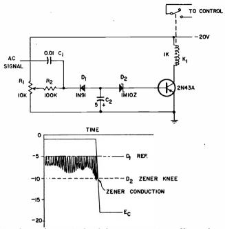
Level switch circuit (top) has snap action effect when ac signal goes over zener conduction point (bottom).
