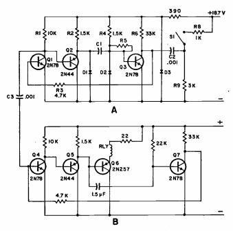
FIG. 2-Complete circuit of transistorized intervalometer.
