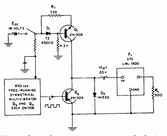
FIG. I—Circuit for generating constant amplitude sine waves.
