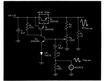
Modification of a conventional dc series regulator yields a lowimpedance, high-output audio source.
