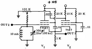
Resistive degeneration allows isolation of the tank circuit from the driving tube while eliminating all grid current from the tank.
