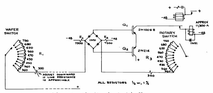
FIG. 2—Remote rotary switch steps to ntatch resistor values at control position.
