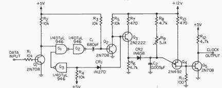
Clock resynchronizer consists of a UJT osillator (Q4) triggered by a one-shot multivibrator (Q2, G1, G2 and G3).
