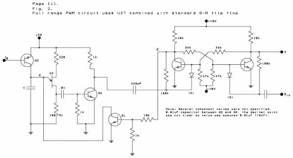
Fig. 2. Full-range PWM circuit uses UJT combined with standard S-R flip flop.
