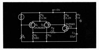
Time-delayed Schmitt trigger with photocell as sensor.
