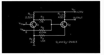
Variable Schmitt trigger, amplitude comparator in which V<sub>B</sub> controls trigger level or is compared with  $V_{TA}$ . Comparison of calculated and experimental triggering points (below).
