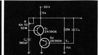
Fig. 2. One modification of Fig. 1 permits a very wide frequency range.
