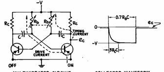
MULTIVIBRATOR CIRCUIT COLLECTOR WAVEFORM FIG. I—Classical multivibrator circuit and its output waveform.
