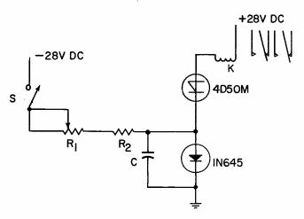
FIG. 1—Simple time delay circuit uses four-layer diode.
