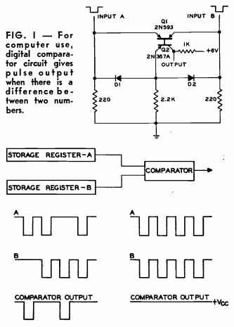
FIG. 2—Output waveforms when two numbers are equal or unequal.
