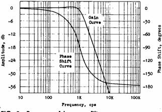
FIG. 2-Response of low pass filter.
