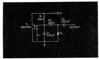
Fig. 1. This amplitude-modulated rf noise generator serves as a handy receiver tester.
