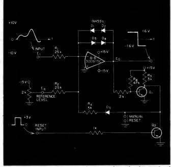
This op-amp comparator latches up when the input signal exceeds the reference.
