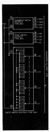
Fig. 2. Typical manual-i n p u t circuit using thumbwheel switches.
