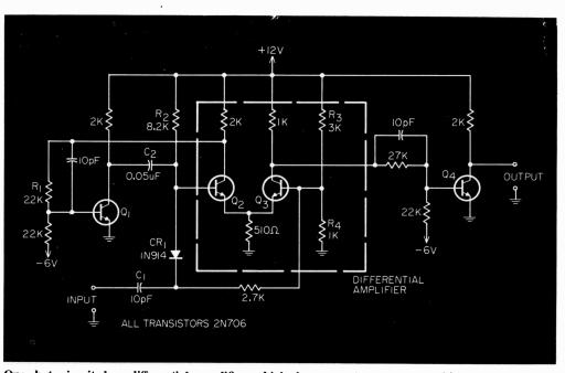
One-shot circuit has differential amplifier which improves temperature stability.
