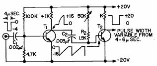
Variable-pulse-width generator provides very high duty cycle.
