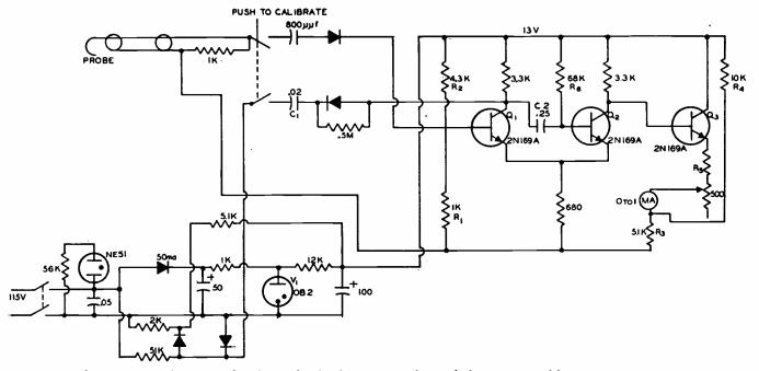
FIG I—Tachometer couples to high-voltage lead of engine with quick-disconnect cable.
