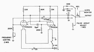
FIG. 1—Portable generator provides pulses up to 900,000 per minute.
