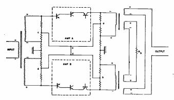
FIG. 3—Failure-proof amplifier showing common feedback connection.
