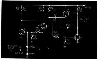
Addition of  $Q_{a}$ ,  $R_{c}$  and  $R_{c}$  to a conventional monostable multivibrator raises the noise immunity without affecting input sensitivity.
