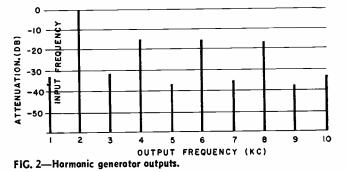
of 1 kc. At 2 kc, the conversion gain was 0.76 and at 4 kc, it was 0.14. That is, the conversion gain was approximately 3 times the maximum gain of a rectifier multiplier. At the second harmonic, an insertion loss of only 3 db makes an amplifier not essential except where large amounts of power are required. The output at other harmonics is of in-
