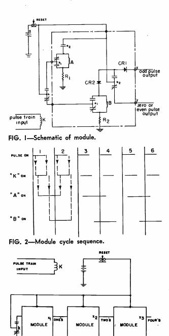
FIG. 3-Three-stage binary counter.
