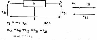
FIG. I—Three-terminal network provides 180-deg phase shift.
