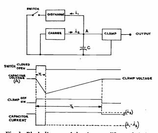
Fig. 1. Block diagram of the time amplifier and timing waveforms.
