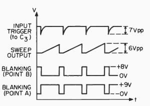
Fig. 2. Typical waveforms for the circuit of Fig. 1. The amplitude of the linear ramp output is unaffected by variations in sweep duration.
