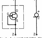
Fig. 1. A current-regulator diode behaves like an unbiased n-channel FET. The device is normally represented by the symbol shown right.
