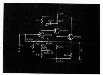
Low-noise preamplifier for low-capacitance transducer.
