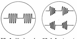
FIG. 2—Waveform of pulsed signal output when feedback is correct.
