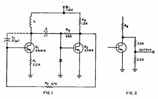
Fig. 1. A stable low-frequency oscillator.
