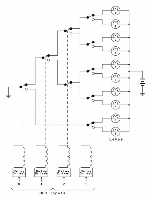
Fig. 1. Relay BCD-to-decimal converter.
