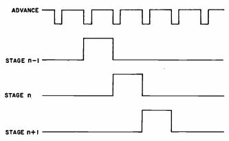
FIG. 2—Outputs of adjacent stages are shown with reference to the advance or shift pulses.
