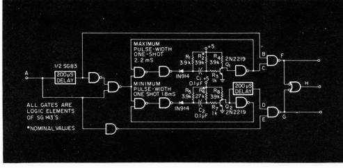
cision pulse generator and trimming  $R_s$  to adjust the Maximum - Pulse - Width One - Shot until a pulse just appears at point H. The minimum allowable pulse width is similarly calibrated by applying 1.8-ms pulses at point A and trimming  $R_s$  to adjust the Minimum-Pulse-Width One-Shot until a pulse appears at point H.
