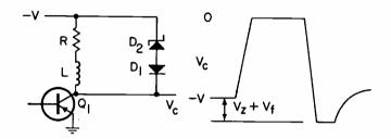
Fig. I—Circuit with controlled fall time.
