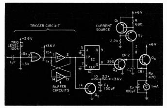
Fig. 1. The direct-reading period-meter circuit uses a Motorola MC779P as well as discretes.
