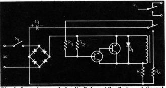
Fig. 2. In an improved circuit,  $C_1$  is rapidly discharged through  $R_{i}$ . Darlington connection gives increased gain and further reduces the size of  $C_{I}$ . A bridge rectifier allows ac operation.
