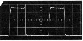
Fig. 4. Output waveform for the circuit shown in Fig. 3. Vertical scale is 1 V/cm and horizontal scale is 50 ns/cm.
