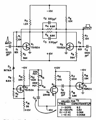
FIG. I—Blanking pulse generator.
