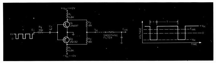
Fig. 1. Duty-cycle of input signal determines the output voltage of this discriminator.
