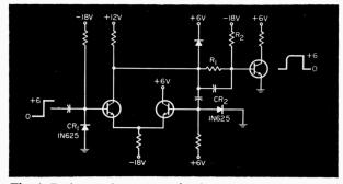
Fig. 1. Basic one-shot output circuit.
