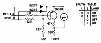
FIG. 3—Neon lamp glows when inputs are at same level. In all three circuits, logic 1 = 0 volts (ground) and logic 0 = -6 volts.
