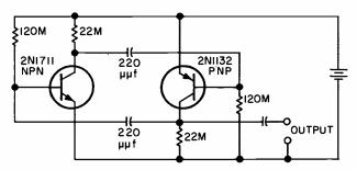
Fig. 1 Multivibrator having extremely low power consumption.
