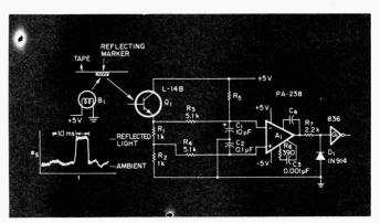
A phototransistor, op amp and DTL gate are used to construct an optical end-of-tape sensor.
