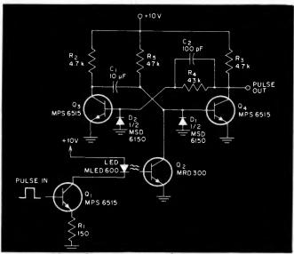
ms output pulse with an ampli- A monostable multi serves as a pulse stretcher, driven by a The base of  $Q_3$  is held to tude from  $V_{CE(S,T)}$  to  $V_{CC}$ . In phototransistor which is triggered by light coupled from a LED.
