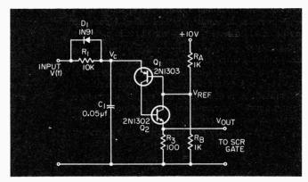
Data-pulse discriminating trigger circuit.
