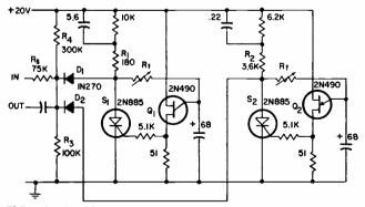
FIG. 1—In the time variant attenuator, Bourns type 3250L-1-502 pots are used to vary the timing of the unijunction circuits. The silicon controlled switches are miniature units made by Solid State Products.
