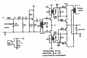
FIG 2—Circuit of pulse demodulator with pulse reference.
