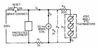
Fig. 1. PTC thermistors used to trip 50 a contact at limiting temperature.
