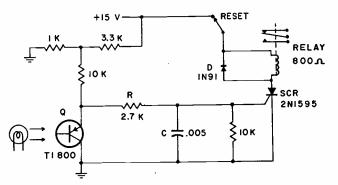
FIG. 1—Phototransistor controls silicon controlled rectifier operated relay.
