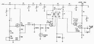
FIG. 9—Circuit of ignition noise simulator.
