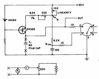
Test circuit at bottom is substituted for  $C_1$  during adjustment of linearity control of ramp generator.
