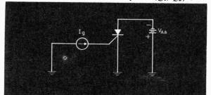
Fig. 1. SCR bias for linear amplification.
