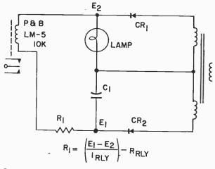
Circuit for indicating lamp failure of photoelectric system.
