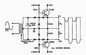
Fig. 3. Practical circuit for 500-kc-to-1-mc operation.
