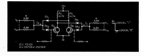
Modified flip flop is set or reset when all input signals are low.
