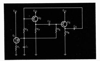
Fig. 1. Basic astable multivibrator circuit.
