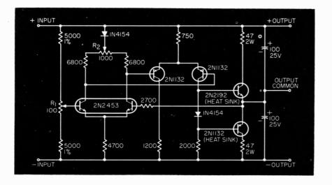
The initial adjustment of the circuit is made by comparing the output voltage with a precision voltage divider connected between the positive and negative inputs. Potentiometer  $R_1$  is adjusted to balance the output voltage and potentiometer  $R_2$  is adjusted to give good tracking of the output voltage with a precision voltage divider convoltage.
