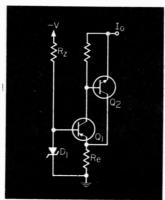
Fig. 2. Temperature drift can be minimized by matching the TCs of  $D_1$  and  $Q_1$ 's  $V_{bs}$ . There is little internal temperature rise in  $Q_p$ , because  $Q_s$ handles the bulk of the load current.
