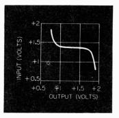
Fig. 2. Input-output transfer characteristic for the circuit of Fig. 1.
