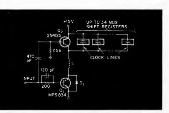
Circuit designers often need Complementary emitter-fol- Fig. 1. In this unusual clock-line driver, inductor L forms a to connect a large number of lowers are commonly used as series-resonant circuit together with the load capacitance.
