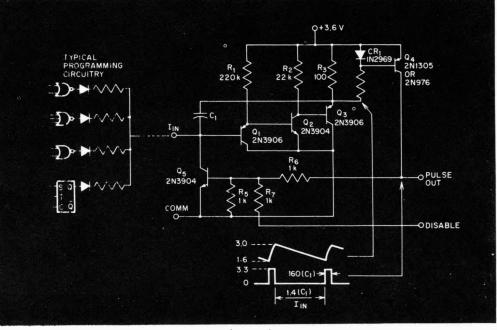
This timing generator, operating at RTL levels, can be current programmed over a wide range.
