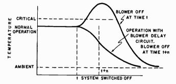
FIG. I—Temperature versus time for a typical system at shutdown.
