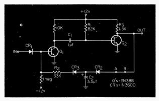
Fig. 3. Frequency-divider circuit.
