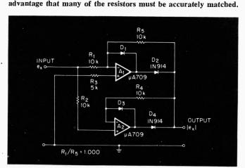
Fig. 2. In this improved circuit only one pair of resistors (R, and R<sub>s</sub>) is critical.
