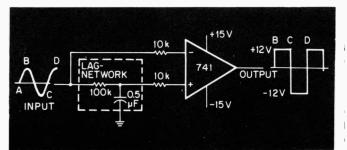
High and low output levels indicate changes in slope of an input signal, regardless of input level over a wide range.
