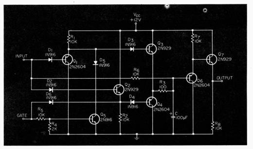
off. The push-pull pair  $Q_s$  Fig. 1. Basic circuit of gated low-pass filter with two alternaand  $Q_{\perp}$  alternately charge and tive time constants. Removing  $R_{\sigma}$  gives a sample-hold circuit.
