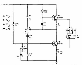
FIG I—Two-transistor circuit provides choice of four different wave shapes.
