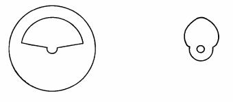
STATOR PLATE ROTOR PLATE FIG 4—Configuration of capacitor plates.
