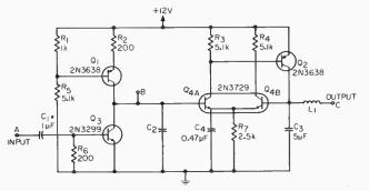
Fig. 1. In this simple D/A converter, Q1 generates a ramp voltage across C2. Duration and height of the ramp are controlled by the input signal which turns on  $Q_3$  to discharge the capacitor.
