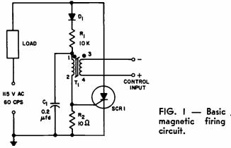
ative half cycle of the ac line so that the scr will be fired on the following positive half cycle.
