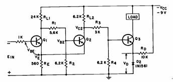
FIG. 3-Basic circuit of transistor switch.
