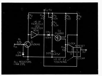
Fig. 1. Delayed-action data receiver inhibits noise in logic systems. Input stage  $Q_i$  is designed to interface with a Data-phone.
