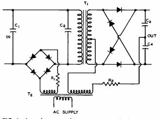
FIG I—Impedance-matching circuit uses diode chopper and synchronous demodulator.
