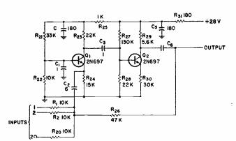
Up to 20 inputs can be handled by grouping amplifier.
