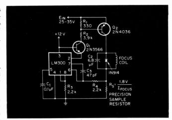
In this precision focus-current regulator, the focus coil and the IC regulator are fed from separate voltage sources. Thus the unregulated input voltage can exceed the allowable maximum for the IC.
