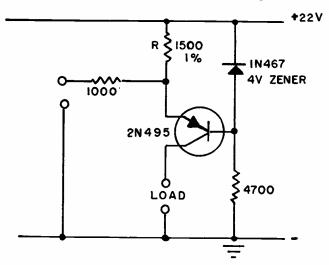
FIG. 1—Constant-current generator is temperature compensated.
