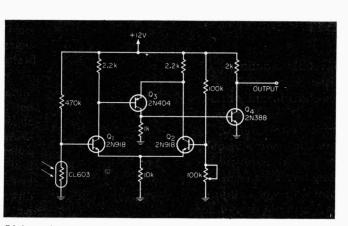
Light-activated switching circuit uses a resistive photocell.
