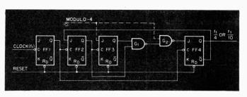
This is a modulo-10 counter when a "1" signal is applied to the "Modulo-4" input, and a modulo-4 counter when a "O" is applied there.
