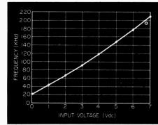
Fig. 1. Crosscoupled NOR gate provides sensitive low-cost VCO.
