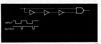
Fig. 1. This is the circuit of a transition detector using IC logic gates.
