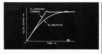
Fig. 1. This graph shows the transient response of the differential amplifier with and without the constant-current load.
