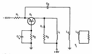
Blocking oscillator provides even duty cycle.
