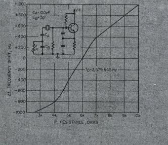
circuit of the basic crystal oscillator without FET control. Oscillation frequency is given by Eq. 1.
