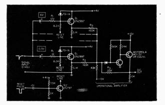
Tunnel-diode pulse-height discriminator.
