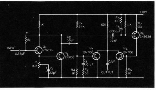
Differentiating circuit gives increased gaiu at high frequencies to compensate for loss of brightness in CRT.
