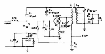
FIG. I — Frequency-modulated oscillator and slope detector provide high-gain dc amplifier.
