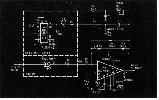
This oscillator generates a choice of four low-frequency tone bursts under direct digital control. Tones are turned on or off rapidly, with no transients.
