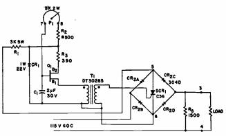
FIG. 1—Full-wave output is provided with one unijunction trigger and one controlled rectifier.
