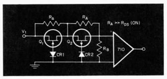
to be less than the input and Fig. 2. New comparator protection circuit extends differential and input voltage ranges while maintaining accuracy.
