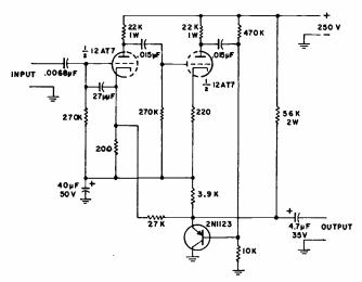
FIG. I—Hybrid amplifier has gain of 95 from 1 kc to 50 kc.
