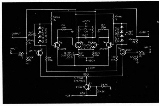
Direct-coupled differential amplifier provides 400-V output swing.
