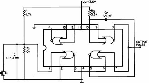
Fig. 1. Because swtich S<sub>i</sub> is shunted by C<sub>i</sub> and has one side grounded, noise generated by the switch is normally below the threshold of the IC. The circuit generates output pulses from 1  $\mu$ s to 80 ms, wide
