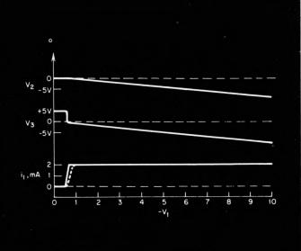
Fig. 3. Voltage-current relationships for a test circuit in which a negative-going ramp replaces the pulse generator and a meter and power supply replace the IC.
