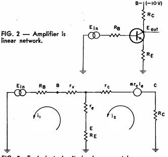
FIG. 3—Equivalent circuit showing current loops.
