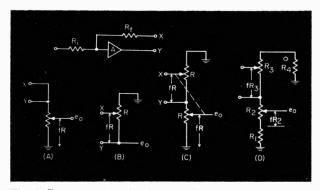
Fig. 1. Four methods of gain control. Method shown in 1d is most practical method for control from zero to infinity.
