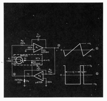
pinching off the source-gate junction. The time constant during this part of the cycle is  $(R_1 + R_2) C_1$ .  $C_1$  charges until the output of  $A_i$  reaches the positive trip level of the Schmitt trigger. When this
