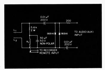
The circuit starts a tape recorder when a telephone receiver is lifted to make a call or receive one. The relay is a Sigma 65F1A -24 Vdc or equivalent.
