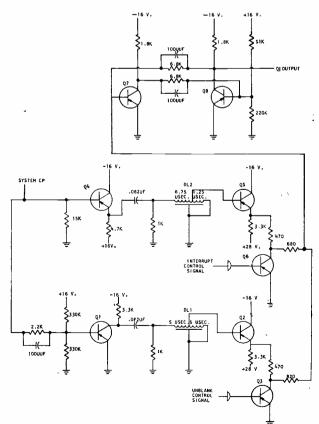
Fig. 1B. Transistorized circuit produces square wave output.
