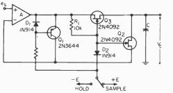
Fig. 2. Modified circuit overcomes the problem of FET "on" resistance, by placing FETs inside feedback loop. Capacitor then sees a much lower source resistance.
