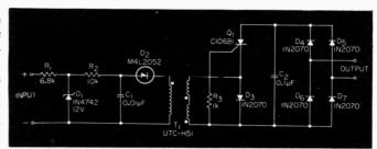
Fig. 1. Simple voltage sensor with threshold voltage determined by four layer diode  $D_{i}$ . The pulse transformer isolates the sensing circuit from the load circuit.
