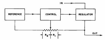
FIG. 1-Conventional two-transistor regulator.
