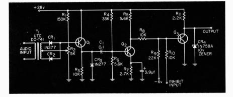
Zero-crossing detector with adjustable output interval.
