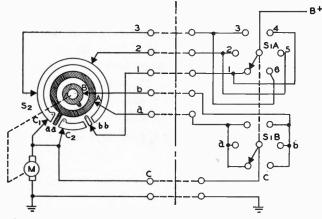
FIG. 2—Contact ring assembly.
