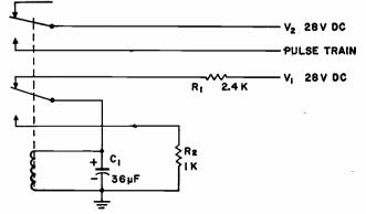
FIG. 1 — A Sigma 8000 G or equivalent is used in the intervalometer.
