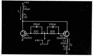
Fig. 1. Fast-riso current switching circuit.
