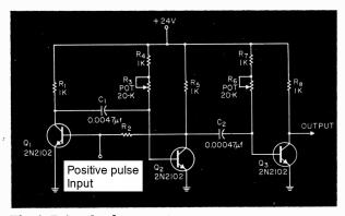
Fig. 1. Delayed pulse generator.
