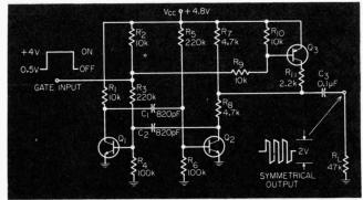
Fig. 2. This improved keyed multivibrator overcomes the level-shift problem. Added transistor  $Q_j$  restores the output dc level to the mean value when the gate signal is low.
