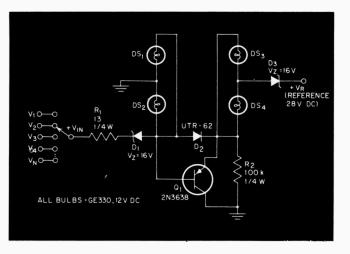
Fig. 1. Simple go-no-go indicator monitors circuit continuity of electronic systems.
