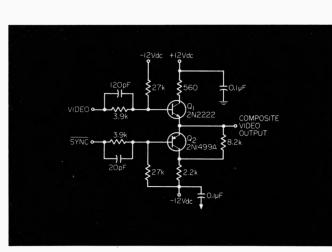
Low-cost vldeo amplifier is compatible with IC logic and EIA standard displays. Frequency response is flat within 1 dB over 20-MHz bandwidth.
