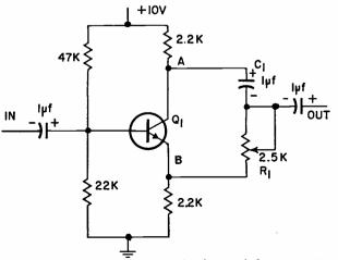
FIG. I—Simple transistorized phase shifter, 0-180 deg. continuous.
