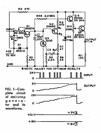
twenty seconds. Unijunction transistor  $Q_2$  triggers at a fixed value of emitter voltage. The point at which  $Q_2$  triggers is fixed by the voltage across zener diode  $D_2$ .
