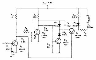
Voltage doubling technique provides fast current rise to drive inductive load.
