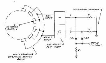
FIG. I—Synchronizer eliminates noise problems in highspeed switching.
