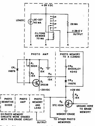
Diode CR<sub>1</sub> is a conventional silicon type with paint removed to allow light to reach junction.
