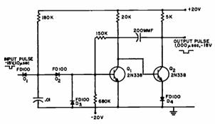
Monostable circuit with less than zero recovery time.
