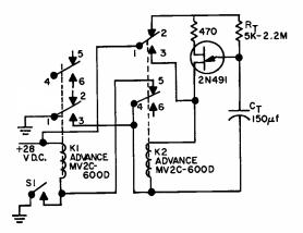
The time interval is determined by the  $R_T$ - $C_T$  charging circuit, which fires the unijunction transistor.
