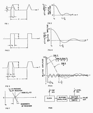
This wave shape has a spectral distribution of the form  $(\sin x/x)$   $(\sin y/y)$  where  $x = n\pi t_1/T$ and  $y = n\pi (t_1 + t_o/T)$ . A plot of this function in x and y is shown in Fig. 6.
