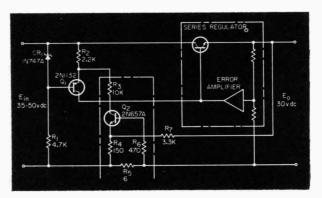
Fig. 1. Low-power overload protection circuit.
