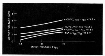
Fig. 2. Offset voltage versus input voltage as a function of supply voltage and temperature.
