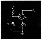
Fig. 1. A conventional grounded-base current source has the disadvantage of poor temperature stability.
