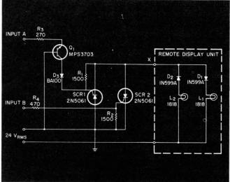
Low-cost plastic semiconductors are used in circuit that minimizes the number of drive lines required for remote lamp display.
