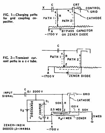
FIG. 3-Circuit designed for protecting grid of c-r tube.
