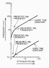
Fig. 2. Frequency response of filter with short time constant (gate grounded) and long time constant (gate open).
