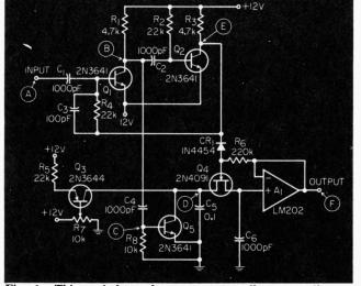
Fig. 1. This period-to-voltage converter allows sampling at rates approaching the input frequency, but without introducing excessive ripple.
