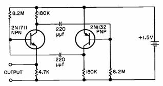
Fig. 2 Multivibrator with low output impedance.
