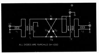
Double-balanced mixer uses hot-carrier diodes. Inductors L<sub>1</sub> and L<sub>2</sub> balance the transformers primaries with respect to ground.
