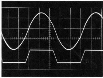
Fig. 2. Waveforms at the output of A (top, 5 V/div) and at the output of  $A_2$  (20 V/div).
