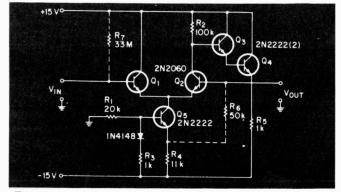
Fig. 1.  $R_4$  and  $R_6$  give the basic follower circuit unity gain, infinite input Z and/or zero input current. Actual gain is 0.9997 V/V.
