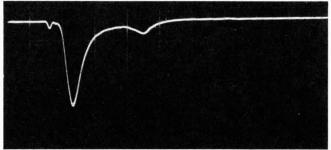
Fig. 3. The Q output of the flip-flop. (same scale as Fig. 2.)
