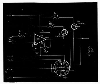
A dual-voltage translator, controlled by DTL or TTL levels, controls the FETs which select the feedback resistance that determines the gain of the op amp. Applied to pin 8 or 2 of the translator, logic low turns on and logic high inhibits a FET.
