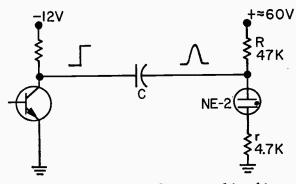
Small voltage changes are adequate to drive this neon readout.
