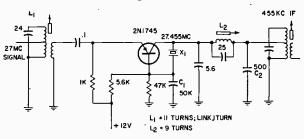
FIG. 4—Mixer-oscillator combination C.
