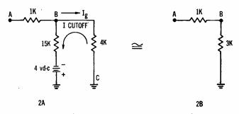
FIG. 2—Equivalent circuit of amplifier before firing.
