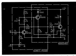
Schmitt trigger,  $(Q_1, Q_2)$  and monostable multi  $(Q_2, Q_3)$ .
