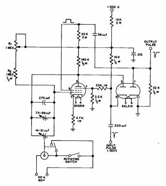
FIG 3—Circuit for simulating acceleration.
