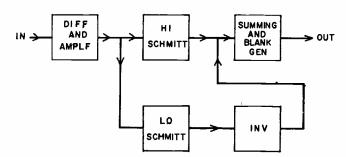
FIG. I—Block diagram of sweep alarm system.
