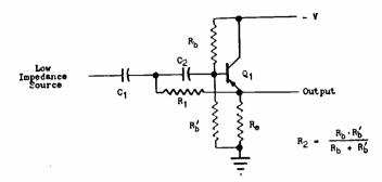
FIG. 3—Active high pass filter.
