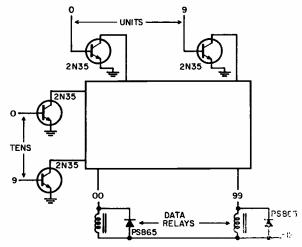
Fig. 1. Basic form of XY code converter.
