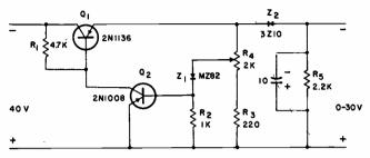
FIG. 2-Simple regulator provides zero to 30 volts autput.
