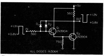
Fig. 1. Diode feedback in this inverter circuit keeps the transistors in the active region (avoiding saturation and cutoff).
