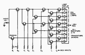
Fig. 2. Transistor BCD-to-decimal converter.
