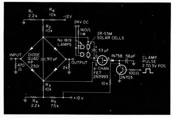
In this unusual gate circuit, a Schottky-diode bridge is switched by a FET. Two illuminated solar-cells provide a floating lowimpedance bias source.
