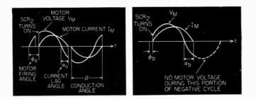
Fig. 2 a (left) In this example, the firing angle  $\phi$  is greater than the current-lag angle  $\alpha$  so single-cycling is not a problem.
