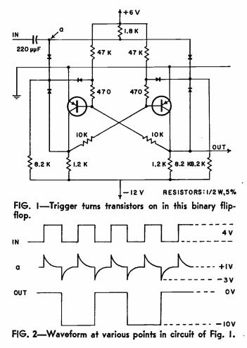
Trigger current is designed into the circuit. The trigger impulse only has to lower point a below ground for a small period. (0.05 to 0.3 microsecond depending on transistors). Triggering operation and steering is very efficient, because the "off" transistor turns on.
