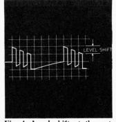
Fig. 1. Level shift at the outof conventional keyed put multivibrators causes distortion when the load is ac coupled.
