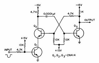
Fig. 1-Circuit for triggering from any-shaped input signal.
