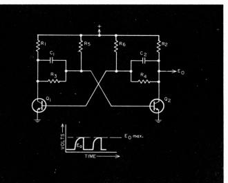
Fig. 1. Basic flip flop rise time is limited by time constants of  $R_2 C_2 \cdots$
