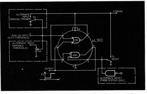
meter as shown in the figure. This versatile latch circuit has many threshold-sensing applications. Alternative connections are The circuit also eliminates shown inside the dashed boxes.
