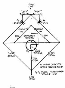
Fig. 1. Simple triac bridge controls direction of rotation of capacitor-type motor.
