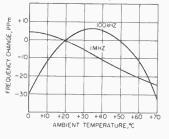
Fig. 3. Frequency varies less than  $\pm$  30 ppm over the temperature range to +70°C. Stability is determined primarily by the crystal.
