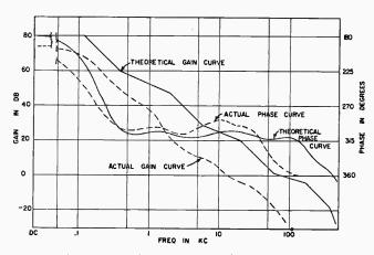
FIG. 3—Phase-gain characteristic of operational amplifier.
