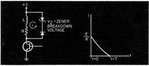
Fig. 2. Voltage protection with diode and zeuer with current decay curve.
