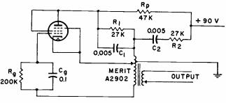
FIG. I—Plate-tuned RC oscillator circuit for 1000 cps.
