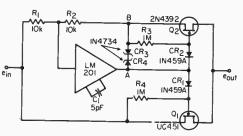
Fig. 1. Unusual linear full-wave Unusual rectifier uses fewer expensive components than other circuits having equal performance
