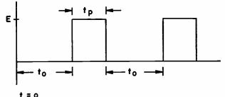
Fig. 2. Output waveshape shows on and off times.
