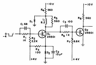
FIG. I—Ringing type of pulse generator.
