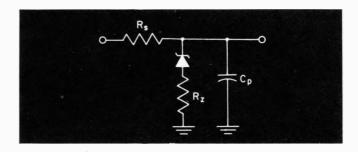
Fig. 1a. Basic circuit of zener shunted by decoupling capacitor used to filter out conducted interference.
