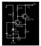
Fig. 3. In this practical circuit, the emitter resistance can be adjusted to set the load current. The zener is bypassed to minimize noise.
