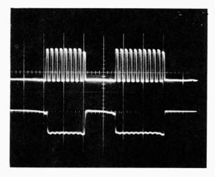
Fig. 2. Typical output (top) and input (bottom) waveforms for a 5-MHz gated oscillator. Horizontal scale is 1  $\mu {\rm s}/$  div. Vertical scales are 2 V/div (top) and 5 V/div (bottom).
