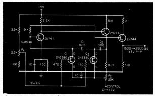
Fig. 1. Voltage-controlled oscillator using FETs.
