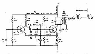
Diode provides small duty cycle of pulsed audio oscillator.
