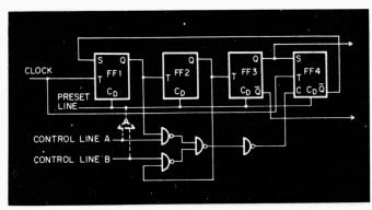
Fig. 1. Circuit for divide-by-8 or -10 and for unambiguous divide-by-9 if the dashed-line gate is added.
