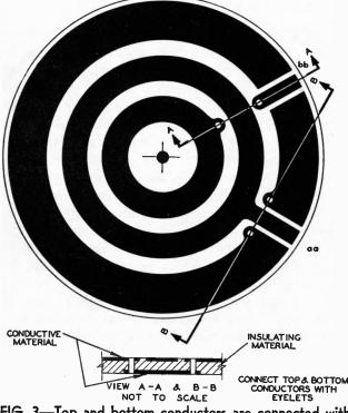
FIG. 3—Top and bottom conductors are connected with evelets.
