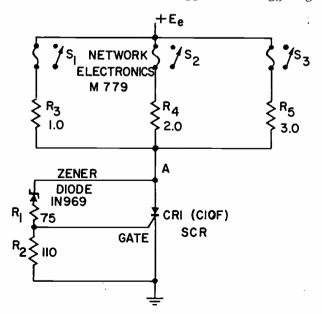
FIG. I—Voltage sensitive trigger circuit initiates sequenced time delays.
