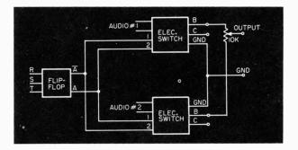
Fig. 2. Two-channel audio switch.
