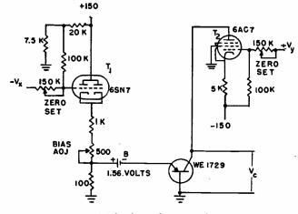
FIG. 2—Multiplier schematic diagram.
