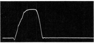
Fig. 2. The Q output of the flip-flop. (Vert. = 1.0 V/cm, horiz. = 50 ns/cm, Vcc = 4.0 V.)
