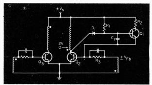
Fig. 1. DC to dc one-shot starting circuit.
