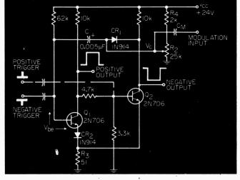
Fig. 1. This voltage-controlled monostable can be pulse-width modulated over a 100-to-1 range without change in amplitude or sensitivity.
