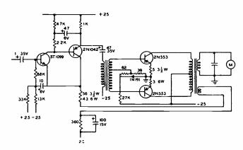
FIG. 1—Motor driver amplifier circuit was developed for the Radan-500 system.
