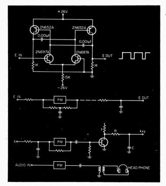
Fig. 1. Basic pulse-width modulator circuit.
