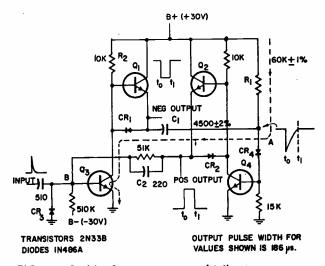
FIG. I—Stable fast-recovery multivibrator.
