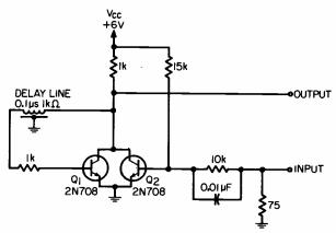
Fig. 1 Simple delay-line oscillator has the advantage that output clock signal always starts in phase with the input gate signal.
