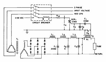
the ratio of secondary turns to primary turns of  $T_2$ , or N2E/N1. This pulse is coupled through capacitor  $C_1$  to the gate of silicon controlled rectifier  $SCR_1$ . The voltage,  $V_3$ , applied between the gate and cathode of  $SCR_1$  is determined by the following equation;  $V_3 = C_1/(C1 + C_2) \cdot N_2/N_1 \cdot E$ .
