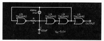
Fig. 3. Practical circuit for 4-MHz pulse generator, using quad 2-input gate. Spare input to the first gate can be used for stop/start control.
