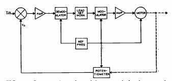
FIG. I—Servo using demodulator and lead network. stabilization.
