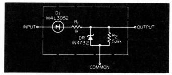
Simple, three-terminal active filter works like a Schmitt trigger, yet needs no external dc supply.
