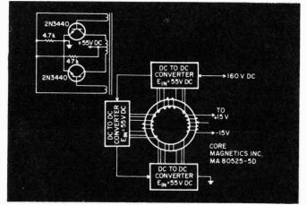
A novel cascade scheme eliminates high-voltage transistors in this dc-to-dc converter.
