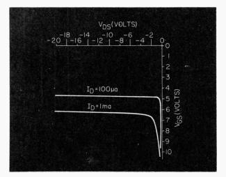
Fig. 1. Typical characteristics for MOS FET type 1004.
