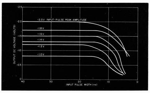
Fig. 2. When an input pulse lasts longer than about 10 ns, the output dc is proportional only to pulse-peak amplitude.
