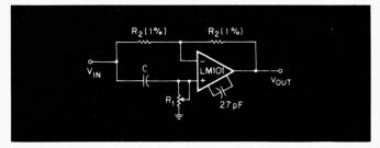
This IC-phase shifter produces 0 to 180° with a constantamplitude output.
