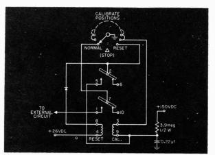
Normal-calibrate mode switching circuit.
