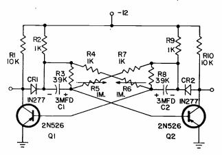
Fig. 1. Modified astable multivibrator.
