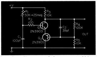
Relaxation oscillator composed of ramp generator driving a trigger circuit.
