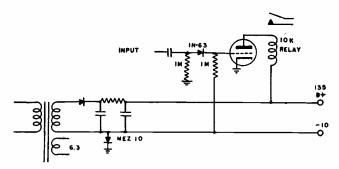
FIG. 1-Zener diode provides ground return for bios supply.
