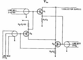
Three transmission lines are matched using emitter follower circuits.
