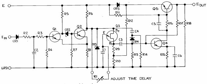
FIG. I—Circuit of solid state variable time delay relay.
