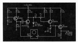
Unijunction transistor serves as relaxation oscillatnr at horizontal sweep frequency.
