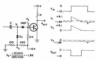
FIG. 2—Noise rejection provided by one diode in this circuit can be adjusted to a desired level.
