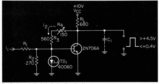
Fig. 3. Improved threshold circuit with adjustable hysteresis. The magnitude of current iz determines whether the circuit hysteresis is positive, zero or negative.
