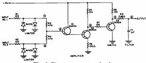
Fig. 1. Phase comparator circuit.
