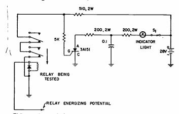
FIG. I—Lamp lights if any relay contact opens for 0.1 microsecond.
