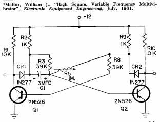
Fig. 2. Converted circuit of Fig. 1 to monostable multivibrator operation.
