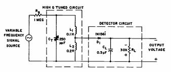
FIG. I—Resonant circuit and detector for feeding to transistor.
