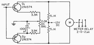
Rate circuit triggers relay on rapid input voltage changes.
