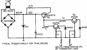
foolproof. Simultaneous triac rent in the main winding is triggering, or a shorted triac, will stall the motor — which ed. then draws about two-thirds of its normal running current. triac minimize the possibility With the specified motor, cur- of unwanted dV/dt triggering. rent in the capacitor winding The values depend on the inranges from 500 mA rms at ductance and back emf of the idling speed, down to 300 mA particular motor used.1 With
