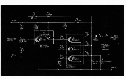
Current sink absorbs 3-A reverse current. Clamping voltage is adjustable over the range 5-15 V.
