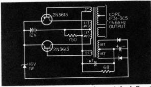
Battery converter-regulator uses extra control winding to bias converter transistors.
