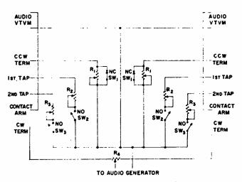
FIG. I—Basic circuit for measuring tracking of stereo controls.
