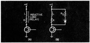
Fig. 1. Inductive load switching circuit (1a) and kickback protection circuit (1z).
