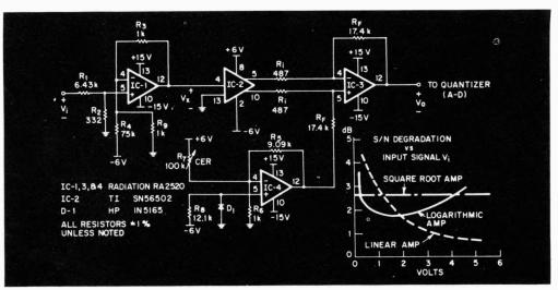
This non-linear amplifier, made with IC op amps, synthesizes  $Vo = 2.5 Log_{10} (V_i + 1).$
