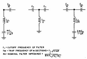
FIG. 5—High pass filter design equations.
