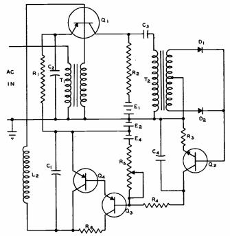
FIG. 3—Complete circuit contains amplifier for the difference signal.
