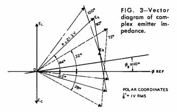
is possible by adjustment of  $R_D$  in shunt with  $C_1$ . At precisely a phase shift of 90 degrees, this value was 21 kilohms.
