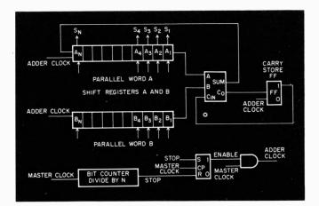
Fig. 1. Block diagram of a conventional serial adder.
