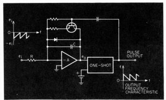
One-shot multivibrator, in trigger generator circuit, provides pulses which discharge capacitor in feedback circuit of operational amplifier. Output frequency is swept linearly by the innut voltage.
