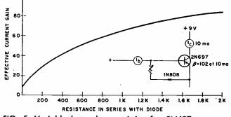
FIG. 5-Variable beta characteristic of a 2N697.
