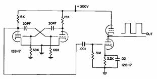
Stacked triodes provide constant output impedance.
