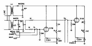
Circuit of vibration test monitor for components.
