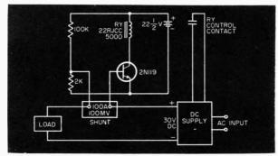
Single-transistor short-circuit detector.
