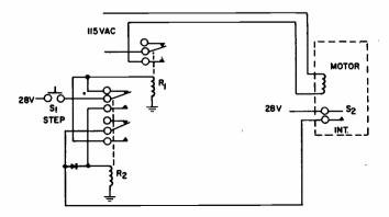
Circuit for step control of motor-driven switch.
