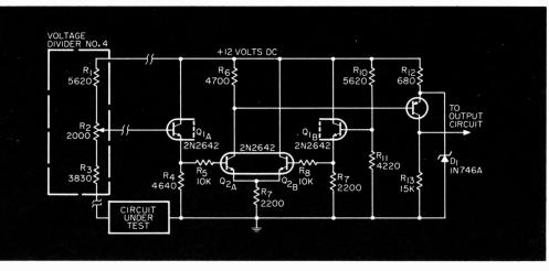
detector,  $Q_3$ . The detector reference voltage level is held constant by zener diode  $D_1$ . When the resistance under test is greater than the nominal value, the output at the collector of  $Q_3$  is a positive voltage. If it is less than nominal, the output is ground.
