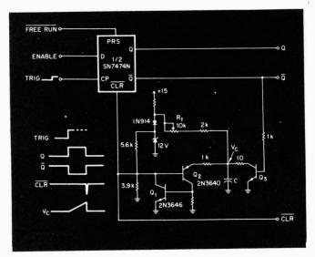
This highly stable circuit can be used as a one-shot, variable pulse delay or oscillator.
