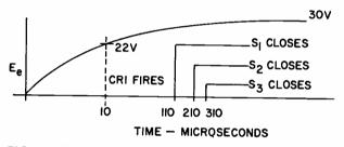
FIG. 2—Timing sequence as applied voltage,  $E_{\rm e_1}$  builds up.  $CR_1$  fires after 10 msec.  $S_{11}$   $S_2$  and  $S_3$  close at 100 msec intervals thereafter.
