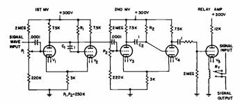
FIG. 1—Sampling circuit using two cathode-coupled multivibrators.
