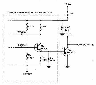
FIG. 2—Multivibrator and Q<sub>2</sub> coupling.
