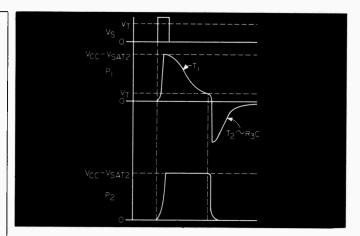
Fig. 3. Typical voltage waveforms for the circuit of Fig. 2. operating in the one-shot mode.
