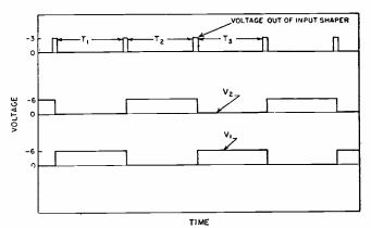
FIG. 2—Waveforms in frequency measuring circuits.
