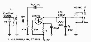
FIG. 3—Mixer-oscillator combination B.
