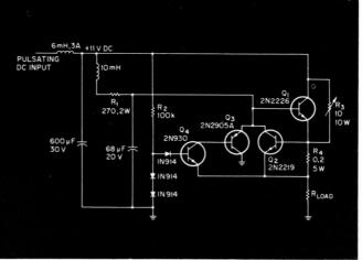
Though protected against short circuits, this current limiter will deliver momentary high current to uncharged capacitors or cold filameuts.
