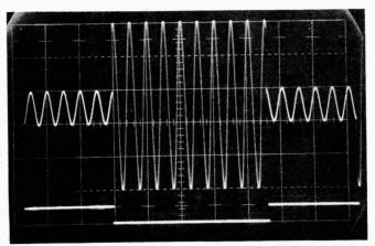
Fig. 2. Output voltage variation as a function of the digital control signal. Analog output voltage scale is 1 V/cm and the digital input voltage scale is 10 V/cm. The time scale is 200  $\mu s/cm$ .
