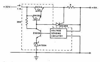
Transistor protection circuit for regulated power supply.
