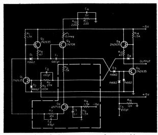
Added transistor Q<sub>6</sub> increases range of monostable.
