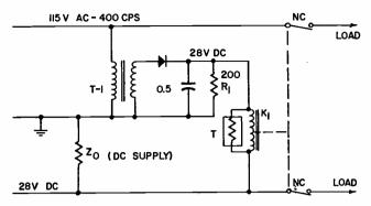
Differential relay circuit provides over and under voltage protection.
