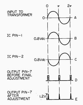
Fig 2. Timing diagram shows how the output pulse coincides with the zero-axis crossing. Width of the output pulse depends on the initial bias voltage.
