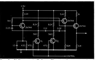
Fig. 2. Voltage-controlled oscillator using conventiona! transistors in place of FETs.
