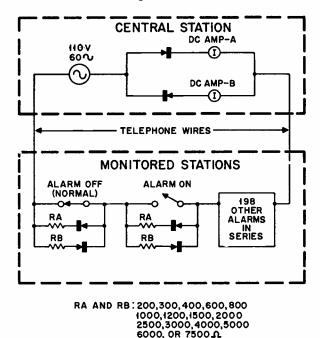
FIC. 1—Use of diodes at central station and monitored stations allows detection of the one of 200 that is in the alarm state.
