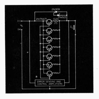
SCR protection for seven paralleled power transistors.
