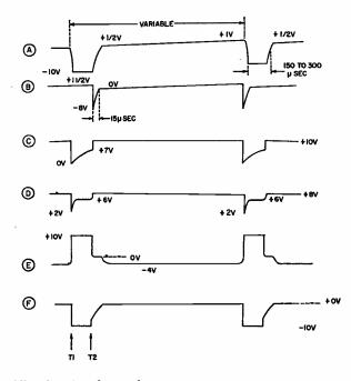
Fig. 2. Waveforms for DC-to-Frequency converter.
