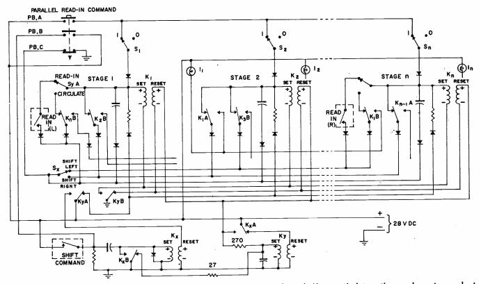
In the shift register, all A and B normally open contacts of relays  $K_I$  through  $K_n$  are tied together and go to readout indicators  $I_I$  through  $I_n$ . Capacitors are 8  $\mu$ f and diodes are 1N537. Unmarked resistors are 250-ohm, 5-watt.
