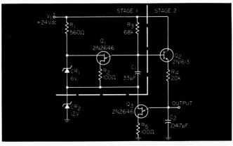
Fig. 1. Simple sweep-frequency generator consists of two cascaded unijunction oscillators.
