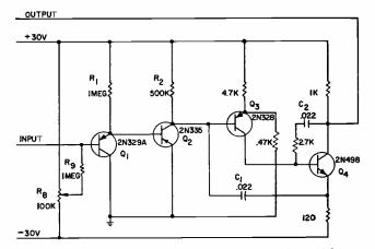
Schematic of simplified transistor operational amplifier.
