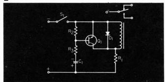
Fig. 1. In this simple time-delay circuit, transistor  $Q_1$  reduces the size of capacitor  $C_i$  needed for a given time delay. But this circuit has slow reset because  $C_i$  must discharge through the resistors and the relay coil.
