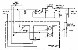
FIG. I—High-efficiency power supply for low-voltage applications.
