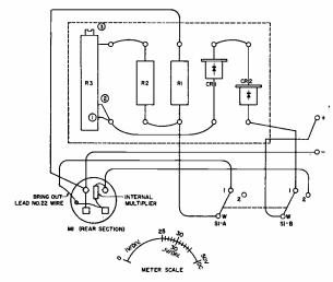
Fig. 2. Rear view of dual range voltmeter.
