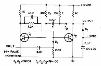
FIG. 1—Monostable multivibrator circuit designed for fast turnoff.
