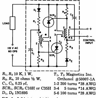
FIG. 2-Solid state ac latching relay.
