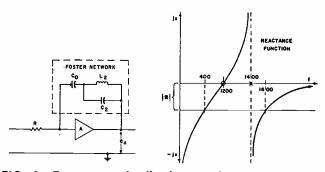
FIG. 2—Foster type feedback network.
