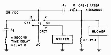
FIG. 2—Blower delay switching circuit.
