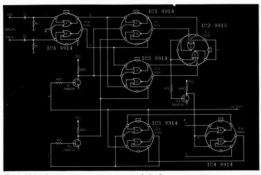
Fig. 1. Digital frequency comparator uses no tuned circuits.
