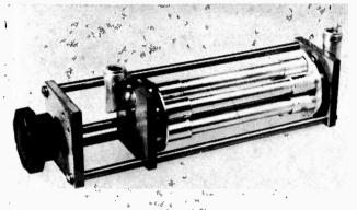
FIG. 2—Filters are combined with pull-turn-push coaxial switch.
