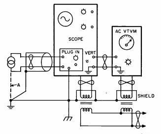
For preferred low level signal measurement: isolation power transformers, short twisted shielded cables, and single point grounding are emphasized.
