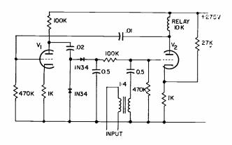
FIG. I—A 10-mv rms 60-cps signal to this sensitive amplifier energizes the relay.
