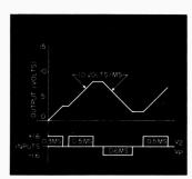
Fig. 3. Typical output waveform for the circuit shown in Fig. 2. Note that charge and discharge time constants are both 10 V/ms.
