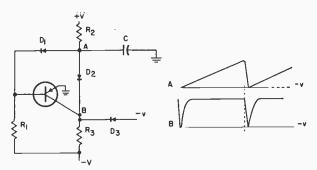
Single-transistor generator employs germanium diodes at  $D_1$  and  $D_3$ , and a silicon type at  $D_2$ . Waveforms shown occur at points A and B.
