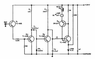
Fig. 1-Detector for giving visual alarm when pulse skips.
