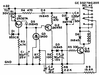
FIG. 2—Repeat cycle timer results by revising basic circuit shown in Fig. I.
