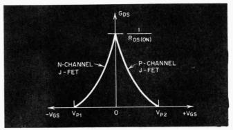
Fig. 3. Graph of FET conductance versus comparison points.
