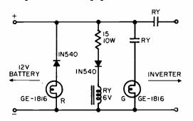
Control protects transistorized inverters from being incorrectly polarized.
