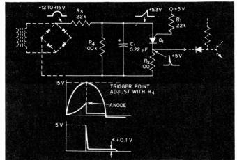
This simple and inexpensive circuit provides a reliable syuc pulse from the 60-Hz power line.
