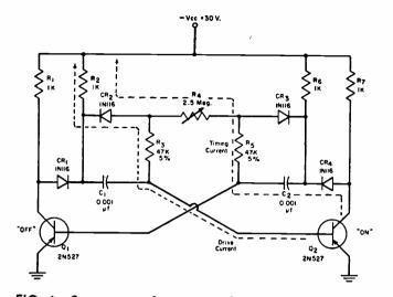
FIG. I—Squareness of 1670 at 4 kc is provided by circuit composed of two audio transistors and four diodes.
