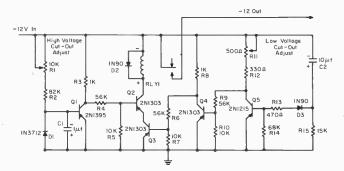
High-low voltage cutoff circuit. Tunnel diode  $D_i$  senses high voltage and thyristor  $Q_i$  senses low voltage.
