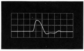
Fig. 2. Typical output pulse for the circuit shown in Fig. 1. Horizontal scale is 20 nsec/div and vertical scale is 5/div (18 A/div).
