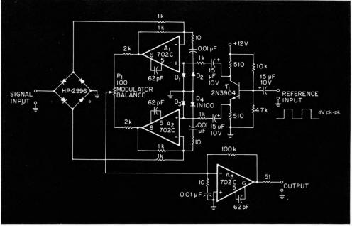
IC op amps obviate transformers and extend the frequency range of this ring modulator.
