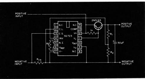
Positive high-efficiency regulator uses an external pnp transistor. Minimum  $V_{in} \equiv V_{out} + 0.5 \text{ V} \equiv R_{cs} I_{L^*}$  Output = 7 to 37 V. er biasing for the rest of the as a brute-force stabilizer. circuitry.
