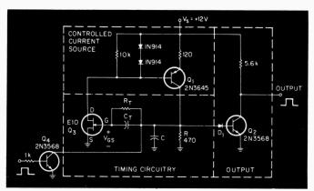
In this unusual one-shot, transistor  $Q_{i}$  and capacitor C isolate the timing circuitry from transients on the dc line.
