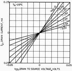
Fig. 1. For small val∪es of Vos, the 2N5163 FET behaves like a resistor with value determined by Vos.
