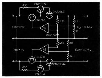
Fig. 2. Complete dual 15-volt power supply for IC op amps has protection circuits in each line.
