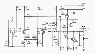
Fig. 2. Stabilized phase-shift oscillator.
