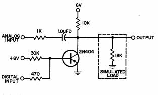
ANALOG INPUT 8cps TO 650KC WITH  $V_P < 12V$ OV-SWITCH CLOSED DIGITAL INPUT 6v-SWITCH OPEN
