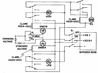
Go-no go voltage comparator circuit. Transistors mu& be mounted on heat sink.
