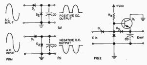
Fig. 1. Basic clamping circuits.
