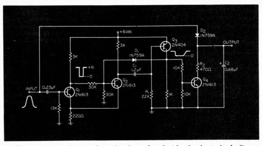
Fig. 1. Simple circuit holds the peak voltage of a short-duration input signal. Storage period is determined by the value of  $C_{r}$ .
