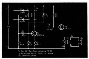
Differential-voltage or current alarm circuit.
