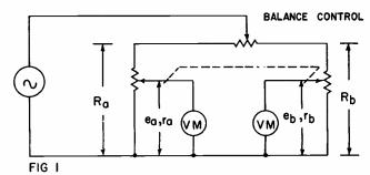
Two methods of checking tracking of dual pots.
