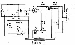
the necessary voltages for operation of the amplifier. This circuit configuration may be used for either ac or dc signal inputs.
