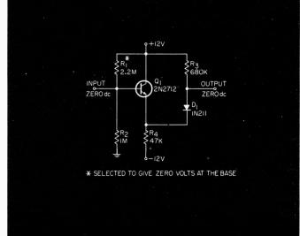
minimizes drift due to varia- Modified emitter follower has equal dc levels at input and outtions in power-supply voltage. put. Offset due to  $V_{BE}$  is eliminated by diode  $D_{I}$ .
