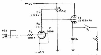
FIG. 1-Circuit of voltage controlled high voltage switch.
