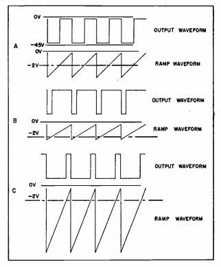
Fig. 2-Waveforms showing how output wave varies with amplitude of ramp voltage (setting of  $R_s$ ). At A, symmetrical wave results. See text for conditions that cause waveforms at B and C.
