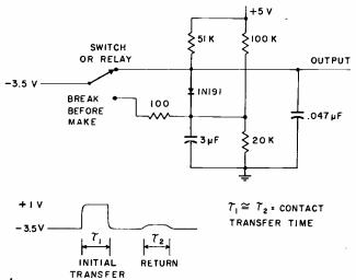
FIG. I—Pulse generator is driven by switch transient.
