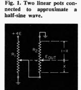
greater than  $R_1$  (i.e.  $R_2$  does not load  $R_1$ ), it can be shown that  $E_{out} = 4X(1 - X)E$ , where X is the fraction rotated by the wipers. This parabolic function approximates onehalf of a sine wave with a maximum error of 0.056E at 21 deg and 159 deg, as may be seen in Fig. 2.
