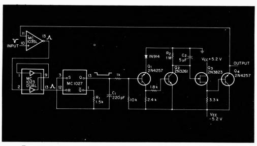
Fig. 1. This circuit responds to the peak amplitude of narrow pulses and is insensitive to their widths.
