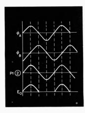
Fig. 1. Phase relationships of tacho output signals and corresponding outputs from the circuit of Fig. 2.
