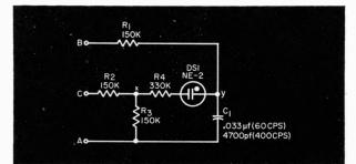
Fig. 1. Phase indicator circuit.
