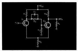
Fig. 2. Conventional Schmitt trigger circuit.
