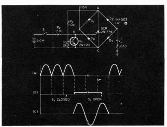
Fig. 1. Schematic and waveforms of zero-crossing solid-state switch.
