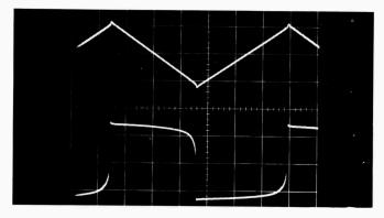
$$T = (3) \frac{C_{1}(V_{T_{1}} - V_{T_{2}}) (R_{5} + R_{6})}{V_{in} - E_{0}}$$
