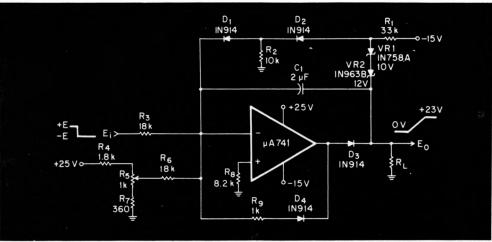
Two diodes and two zeners clamp this integrator's output to below the op amp's saturation voltage, making for fast recovery. All resistors are 5%, 1/4-W carbon comps.
