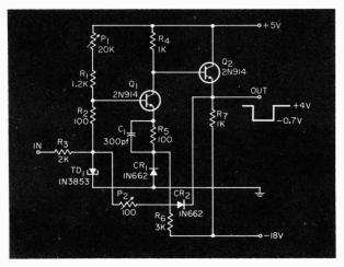
Fig. 1. Tunnel-diode discriminator using dc amplifier.
