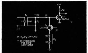
Fig. 1. Current amplitude detection circuit.
