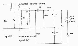
Drop of 25 volts in primary circuit actuates neon lamp.
