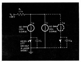
Automatic lamp back-up circuit using 4 layer diodes.
