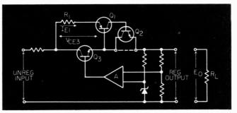
Fig. 1. Simple overvoltage-protection circuit  $(R_p, Q_p, Q)$  can be added to any conventional series regulator.
