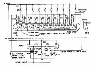
FIG. I-Reset and MBS tube circuit.
