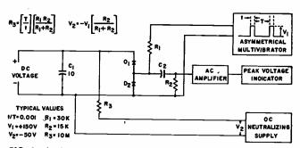
FIG. 1—A dc impedance level of 5 megohms is achieved with values shown. Design formulas shown for  $R_3$  and  $V_2$  can be improved upon, for greater accuracy.
