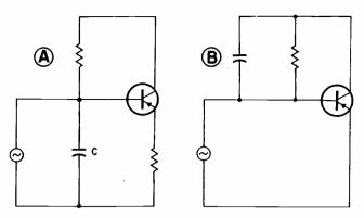
FIG. I—Equivalent circuits for inductive (A) and capacitive (B) transistor circuits.
