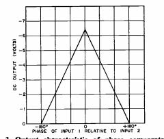
Fig. 3. Output characteristic of phase comparator.
