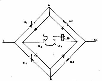
FIG. 1—Bridge circuit used to detect signal for activation of rotary switch.
