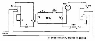
FIG. I—Circuit of relay under test is isolated from monitor circuit.
