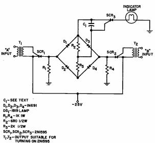
Fig. 3-Anti-Coincidence Detector.
