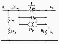
FIG. 2—Transistor equivalent circuit.
