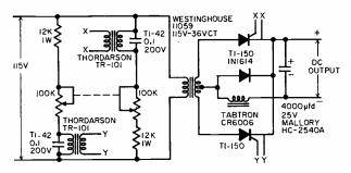
Power supply uses an scr thus enabling the output dc voltage to be varied without changing the input ac voltage.
