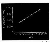
Fig. 3. Output frequency of the second stage is a linear function of the emitter voltage of Q2.
