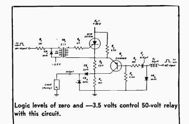
data processing system. A 50-volt relay (internally connected to ground) of this unit was to be operated by logic levels of -3.5 volts and 0 volt.
