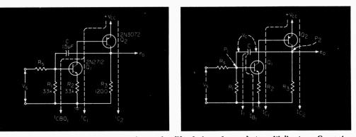
Fig. 1. (left) Complementary transistors simplify design of one-shot multivibrator. Current flow paths are shown for the quiescent "off" state. Fig. 2. (right) One-shot circuit redrawn to show current flow after triggering. With modification of component values, the same basic circuit becomes a free-running multivibrator.
