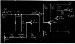
Fig. 1. Electronically-adjustable monostable.
