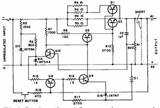
FIG. 1—Transistors  $Q_{\scriptscriptstyle 8}$  and  $Q_{\scriptscriptstyle 9}$  protect the power supply until the circuit is reset.
