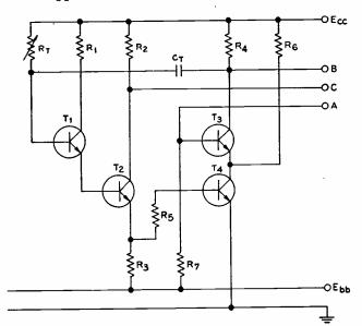
FIG. 1—Ohmic values of resistors follow:  $R_1$  and  $R_5$ -100;  $R_2$  -2700;  $R_8$ ,  $R_4$  and  $R_6$  -4700;  $R_7$  -100K. All transistors are 2N388 and  $E_{cc}$  is -22v, and  $E_{bb}$  is -6v.
