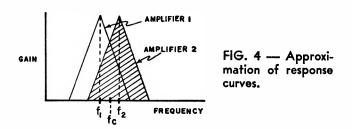
inator given in Fig. 3. Assuming equal gains and attenuation rates in the interval  $f_1 \leq f_c \leq f_2$ , a close approximation to the response curves, as shown in Fig. 4, can be obtained.
