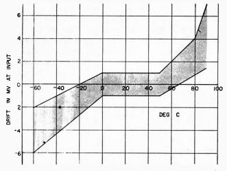
FIG. I—Temperature-drift range of operational amplifier.
