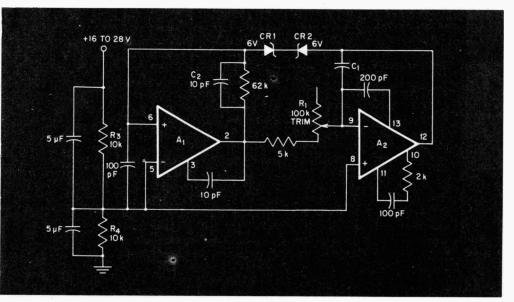
limited only by the observer's Circuit diagram of a wide-range triangle/square-wave generator.
