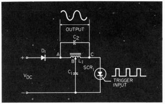
The SCR is the only active device in this circuit. Efficiency is better than 90%.
