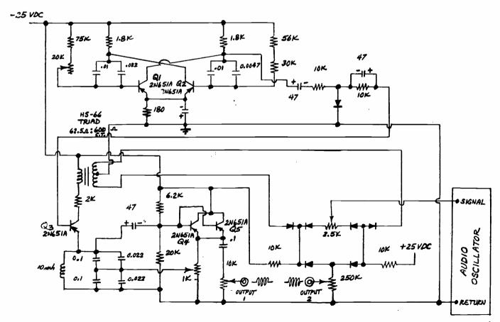
FIG. I—All diodes are IN645A and all transistors are Motorola 2N65IA. Type 236S-I-203 Bourns Trimpot was used for the 20K pot at top left, 224S-I-252 for the 2.5K pot, and 224S-I-102 for the IK pot at Q
