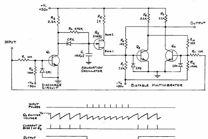
Pulse detection uses unijunction transistor as relaxation oscillator.
