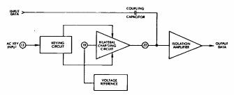
FIG. 2—Bilateral charging circuit used in dc restoration.
