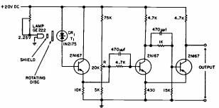
Fig. 2-Circuit Incorporating Photo-Diode Pickoff
