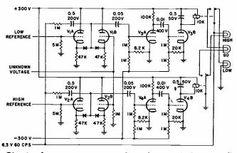
Circuit of go no-go vacuum-tube voltmeter. Tubes are all type 12AX7, diodes 1N69.
