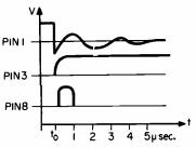
Fig. 2. Switch bounce at pin 1 has no effect on the inverted signal at pin 3. This signal then triggers the one-shot circuit to give a 1-µs output pulse at pin 8.
