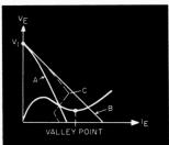
Fig. 2. Characteristic curves for basic and modified relaxation oscillator circuits.
