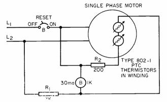
Fig. 4. PTC used with a single-phase motor.
