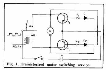
Assume the relay is pulled in at position B when the circuit is in operation. This places -v volts on one side of dc motor, M, and heavily forward-biases transistor  $T_1$ . As a result V-V<sub>sat</sub> goes to the other side of the motor. The preceding causes the motor to rotate in one direction. When the relay drops out to position A,  $T_2$  turns on, reversing the polarity at the motor and the direction of rotation.
