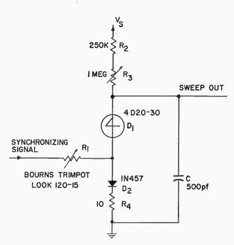
FIG. I—Resistors of the synchronous sweep circuit are noninductive types.
