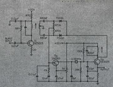
Fig. 6. Complete phase-locked oscillator loop. The FET presents a high input impedance to the output of the phase detector.
