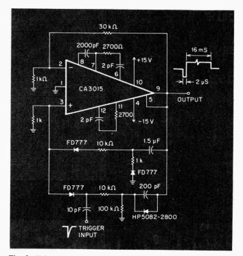
Fig. 2. This practical version of the bipolar multivibrator gives a  $2-\mu s$  negative pulse and a 16 ms positive pulse.
