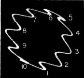
Fig. 448. Crown-wheel pattern for  $f_u/f_s = 10$ . Count the spikes on one side of the wheel only.
