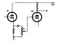
distortion. To accomplish this, dc amplifiers are required. Such amplifiers are liable to drift, especially if the overall gain is high. Drift may be minimized by a symmetrically designed amplifier and careful matching of the two halves.
