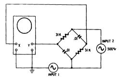
Fig. 447. Circuit used for generating crown-wheel patterns for frequency measurements.
