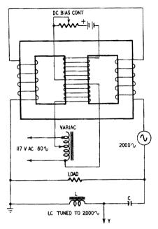
Fig. 636. Magnetic modulator for modulating a 2,000-cycle voltage by 60 cycles.
