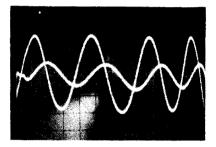
Fig. 407. Two sine waves in quadrature.  $\phi \equiv 0$ . The peak of one wave occurs simultaneously with the zero base point of the other.
