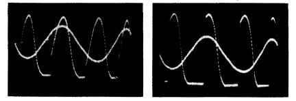
Figs. 7114 to 7117 incl. Working cycle of the gas tubes of Fig. 7113 for different settings of phasing control R (no input filter capacitor). A 60-cycle reference voltage is displayed simultaneously. The double waveforms were obtained by using an electronic switch. Fig. 7114 (upper left). 220-volt output. Fig. 7115 (upper right). 160volt output. Fig. 7116 (lower left). 100-volt output. Fig. 7117 (lower right). 22-volt output.
