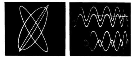
Fig. 523 (left). Phasing ellipses obtained with the constant-amplitude phasing circuit of Fig. 522. R and C as in Fig. 518. Fig. 524 (right). Phasing conditions for two different values of R. Simultaneous viewing is obtained by using an electronic switch. Upper waveform:  $R \equiv 1,000$  ohms; lower waveform:  $R \equiv 100,000$  ohms.
