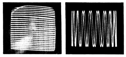
Fig. 248 (left). Television type raster sweep has low frequency ratio to make individual lines clearly visible. Fig. 249 (right). Sine-wave sweep leads to an illegible pattern.
