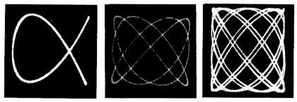
Fig. 426 (left). Another aspect of  $f_y/f_x = 3/2$ . Fig. 427 (center).  $f_y/f_x = 4/3$ . Fig. 428 (right).  $f_y/f_x = 8/7$ .
