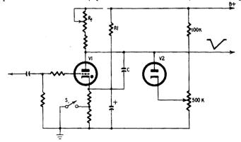
Fig. 239. Triggered time-base generator is made free running by closing switch S.
