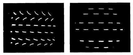
Fig. 1013 (left). Square wave is differentiated by trace shifting in an incorrectly operating dc amplifier. Fig. 1014 (right). Correctly operating amplifier, no differentiation.
