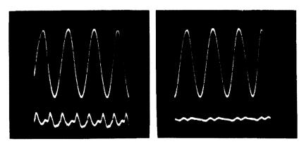
as shown in Fig. 817, operating at about 400 cycles. This twin-Tee must be carefully matched for efficient cancellation of the fundamental. High-grade components must be used for stability. As the exact absorption frequency is unimportant, it is best to select four resistors and four capacitors of about 40,000 ohms and .01  $\mu$ f, respectively, on a bridge to get them matched at 1% or better. These components are then assembled on a bakelite board, and the whole
