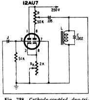
Fig. 738. Cathode-coupled duo-triode oscillator.
