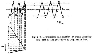
waves during one sweep time (Fig. 216). The corresponding geometrical plotting is indicated in Fig. 217. It is important to understand well the mechanism of pattern generation by two rightangled deflecting forces, this being one of the fundamentals of oscilloscopy.
