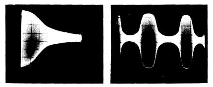
Fig. 792 (left). Nonlinear modulation characteristic (trapezoidal waveform) due to incorrect adjustment of tube voltages. Fig. 793 (right). The modulation waveform (corresponding to the trapezoid shown at the left) illustrates the flattening of the positive and negative modulation peaks.
