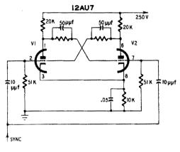
Fig. 774. Multivibrator-derived scale-of-two circuit.
