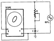
Fig. 518. Simple resistance-capacitance phasing circuit.
