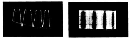
Fig. 1008 (left). 120 cps hum modulation of the CRT grid. Fig. 1009 (right). Hum modulation of the CRT grid showing display of a higher frequency.
