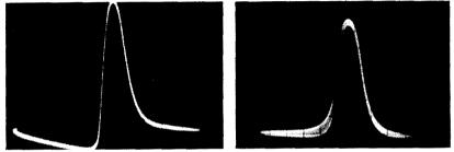
rig. 851 (lett). Base-line distortion resulting from connecting scope input to point C of Fig. 829. Fig. 852 (right). Superimposed rf component appears when the scope is connected to point B.
