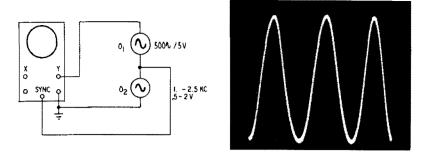
Fig. 501 (left). Circuit used for synthesizing waves containing predetermined amounts of harmonic distortion. Fig. 502 (right). 10% second harmonic is hardly discernible. Note the slight spreading of the trace.
