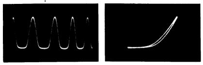
Fig. 706 (left). Flattening of the negative peaks indicates excessive bias voltage. Fig. 707 (right). Characteristic shows condition of plate-current cutoff due to high bias.
