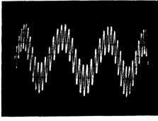
Fig. 775. Linearly superimposed voltages, no modulation.
