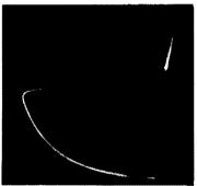
Fig. 763. P1/G1 characteristic of the multivibrator.
