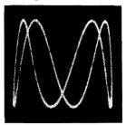
and that its losses are not negligible. Adjusting R for equal length results in the oscillogram of Fig. 418. Now the reactance equals the resistance, or  $2\pi$ fL = R. As R = 2,400 ohms, L = R/ $2\pi$ f = 2,400/ $2\pi$ 60 = 6.35 henries.
