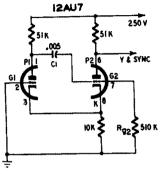
Fig. 764. Cathode-coupled multivibrator.
