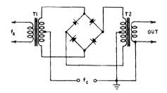
Fig. 780. Bridge modulator circuit.
