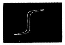
depending upon the direction (increasing or decreasing) of the variation of H. That explains the loop-shaped aspect of the B/H characteristic.
