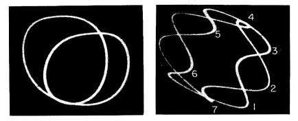
Fig. 451 (left).  $f_u/f_s = 1/2$ . One tooth for two revolutions. Fig. 452 (right).  $f_u/f_s = 7/2$ . Seven teeth, two traces.
