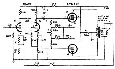
Fig. 824. Conventional class-A push-pull audio amplifier.
