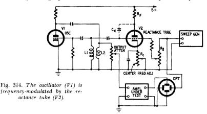
horizontally. Using a scope to display such curves, a graph-type two-dimensional representation can be obtained by linking the generator frequency control with the horizontal deflection device of the scope in a manner to correlate each point of the X axis on the screen to a definite frequency. This can be carried out by the motor-driven device illustrated in Fig. 313, effectively used some 20 years ago.
