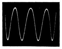
Fig. 757. Waveform produced by the transistor phase-shift oscillator.
