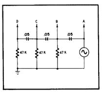
As the usable phasing introduced by a simple R-C section is often insufficient, cascaded sections such as shown in Fig. 529 are sometimes used, for instance, in phase-shift oscillators. The input voltage A is compared with the voltage at B, C and D by an electronic switch (upper, center and lower traces respectively, Fig. 530). The larger amplitude identifies the input voltage. Though the overall phasing introduced is about  $120^{\circ}$  the loss of ampli-
