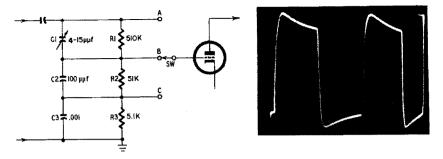
Fig. 209 (left). Frequency-compensated input attenuator. Fig. 210 (right). Overcompensation of attenuator due to excessive capacitance of C1.
