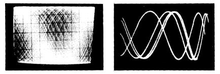
Fig. 230 (left). Insufficient sync results in a blurred oscillogram. Fig. 231 (right). Erratic time-base generator triggering due to insufficient sync signal causes highly unstable trace.
