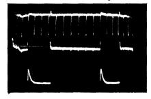
Fig. 772. Multivibrator frequency division. Sync pulses are shown above and collector voltage below.
