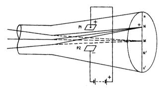
Fig. 103. Electrostatic deflection of the electron beam.
