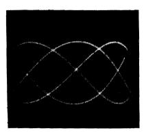
return stroke. To display 6 cycles, the time base has to run at 1/6 of the signal frequency. Calling  $f_y$  the signal frequency and  $f_x$  the sweep frequency, we have here  $f_y/f_x = 6$ .
