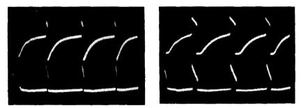
Fig. 243 (lett). Above: grid voltage of V2; below: voltage across R<sub>g</sub>. Fig. 244 (right). Same as Fig. 243, but the time constant of R1C1 is different.
