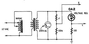
Fig. 644. Circuit for obtaining curves of VR tubes.
