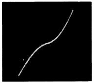
Fig. 642. Characteristic of a nonlinear thyrite resistor (varistor).
