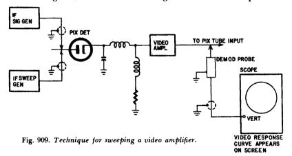
method of sweeping a video amplifier because the response of the picture detector peaking coils is taken into account. A demodulator probe is used at the video amplifier output. This gives a standard demodulated response on the scope screen.
