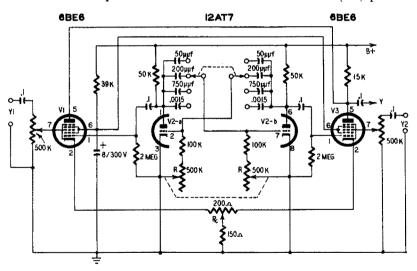
Fig. 302. Electronic switch of the multivibrator type.
