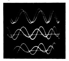
Fig. 530. Comparison of phasing conditions between points A and B (top), C (center) and D (bottom) of Fig. 529.
