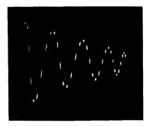
is 1/100,000 sec, or 10 µsec, and this then corresponds to the interval between the two vertical lines. Similarly, timing intervals of 1 and 100 µsec are obtained using circuits tuned to 1 mc and 10 kc respectively.
