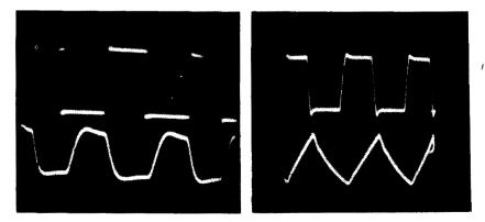
phase shift of low-frequency components. A distinct improvement is obtained by inverse feedback, for some low-frequency components, while attenuated, are still present. They disappeared entirely when eliminating the feedback loop. A very slight improvement is noted at 100 cycles (Fig. 803).
