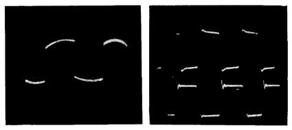
Fig. 808 (left). Rounded tops indicate low-frequency boost. The test frequency was 180-cycles. Fig. 809 (right). Overshoot (upper trace) caused by shunting the transformer primary with a capacitor; ringing (lower trace) produced by shorting the feedback resistor.
