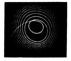
Fig. 255. This is an example of the type of spiral sweep that can be obtained with the circuit illustrated in Fig. 254. This shows the extent to which the base line of the sweep can be lengthened.
