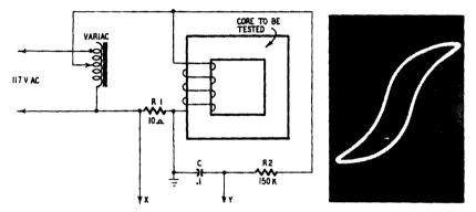
Fig. 628 (left). Practical circuit for tracing B/H curves. Fig. 629 (right). Typical B/H curve for silicon iron.
