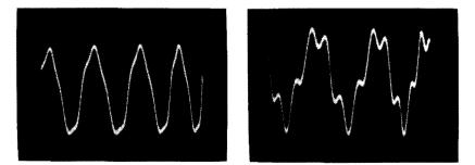
Fig. 515 (left). 10% fourth harmonic creates a clearly visible amount of distortion. This is typical of low levels of the higher-order harmonics. Fig. 516 (right). 30% fourth harmonic. Note the lack of symmetry due to the even-harmonic distortion.
