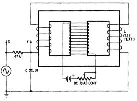
Fig. 638. Determination of the inductance variation of a saturable reactor.
