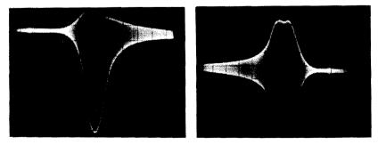
insufficient time constant of R3-C3 at 60 cycles, connection to point C results in the broken base line of Fig. 851, making skirt observation somewhat difficult. An rf residue appears if the scope is connected to point B (Fig. 852).
