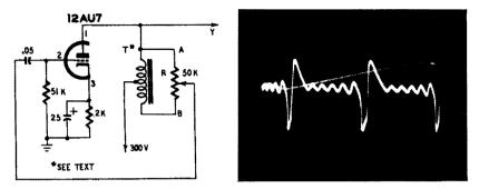
Fig. 726 (left). With this circuit arrangement, a variable in-phase or out-of-phase signal can be returned from the output to the input. Fig. 727 (right). Waveform obtained through the use of the circuit in Fig. 726. The amount of feedback was small.
