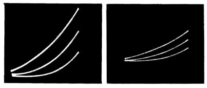
Fig. 611 (left),  $I_p/E_g$  curves of a 12AX7. Plate voltages used were 300, 250 and 200. Fig. 612 (right). Characteristic curves of the 12AX7 with a plate load of .05 megohm.
