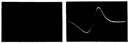
Fig. 858 (left). Assymetric S-curve displayed by single-trace method. Fig. 859 (right). Approximately symmetric S-curve with acceptable linearity.
