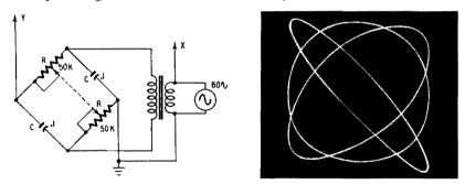
Fig. 525 (left). Phasing bridge using a dual control. Fig. 526 (right). Phasing ellipses obtained with the bridge of Fig. 525.
