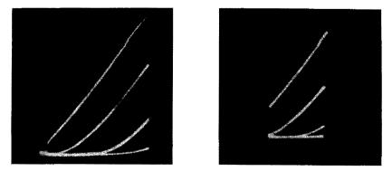
Fig. 619 (left).  $I_p/E_g$  characteristics of a 12AX7 for bias voltages from 0 (top) to -3 volts (bottom). Fig. 620 (right). Reducing the sweep voltage results in incomplete curves.
