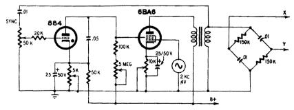
Fig. 254. Spiral time-base generator for demonstration purposes.
