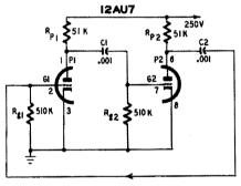
Fig. 759. Multivibrator is a closed-loop two-stage amplifier.
