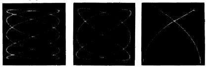
Fig. 438 (left).  $f_y/f_x \equiv 2/5$ . Compare this with the photo shown in Fig. 435. Fig. 439 (center).  $f_y/f_x \equiv 2/3$ . Compare with Fig. 425. Fig. 440 (right).  $f_y/f_x \equiv 2$ . The waveform of  $f_y$  is triangular.
