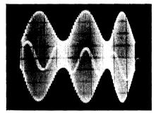
Fig. 637. The pattern of the modulated voltage obtained.
