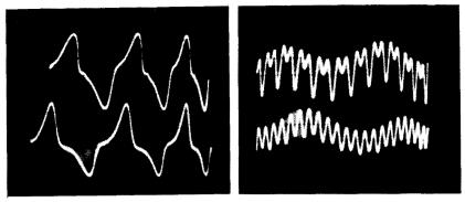
Fig. 826 (left). Low-frequency distortion at 20 cycles is nearly the same with (above) and without (below) negative feedback. Fig. 827 (right). Voltage across R1 in Fig. 824 for unbalanced (above) and balanced (below) push-pull output.
