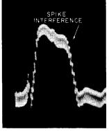
Fig. 905. Spike interference from the horizontal sweep circuit.
