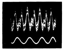
affair is inserted between the amplifier output and the scope amplifier. The scope is switched to external sync, and the sync input is connected to the signal source to secure locking-in on the fundamental after cancelling it on the scope input.
