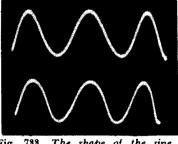
Fig. 733. The shape of the sine wave (above) is improved by the introduction of negative feedback (below).
