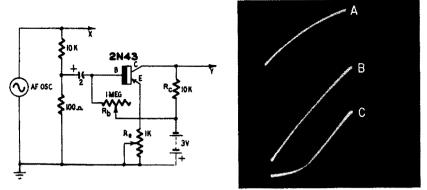
Fig. 715 (left). An experimental transistor amplifier. Fig. 716 (right). Commonemitter transistor amplifier output characteristics. The curves are for different values of base resistor.
