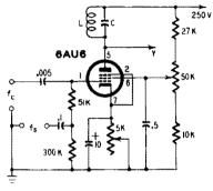
Fig. 785. Pentode modulator with signal and carrier voltages injected into the control grid.
