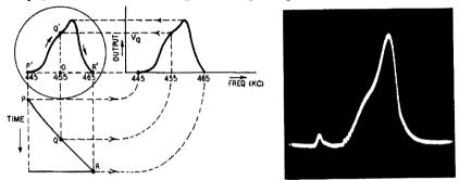
Fig. 315 (left). Generation of a single-trace response curve pattern. Fig. 316 (right). Oscillogram of an assymmetric single-trace pattern.
