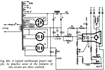
tubes are necessary but, as the cathode of Vl is grounded, this tube may conveniently be connected to the common amplifier heater supply.
