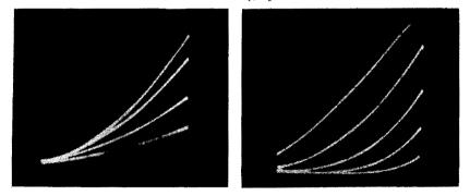
ing two 1N89 germanium diodes of the same batch resulted in the clearly spread characteristics shown in Fig. 606; the higher-sloped curve indicates the more efficient unit. Testing these diodes for forward current, the vom gave readings of 45 and 200 ohms, respectively, on a low-resistance scale (readings of forward resistance on high-resistance scales are meaningless).
