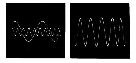
Fig. 465 (left). Frequency ratio of 10 to 2 or 5 to 1. Fig. 466 (right). Time base running at 1/6 of signal frequency.  $f_y/f_x = 6$ .
