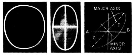
Fig. 412 (left). Quadrature voltages ( $\phi = 90^{\circ}$  or 270°). The applied voltages are of equal amplitude. Fig. 413 (center). Quadrature voltages of unequal amplitudes. The principal axis of the ellipse can be either vertical or horizontal. Fig. 414 (right). Tilted ellipse showing intermediate phase angle ( $\phi = 42^{\circ}$ ).
