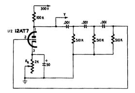
Fig. 740. Simple phase-shift oscillator using resistance-capacitance-coupled sections.
