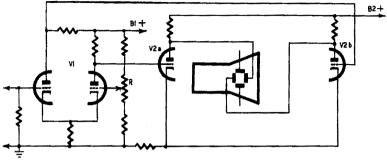
Fig. 206. Push-pull dc amplifier featuring two long-tailed pairs.
