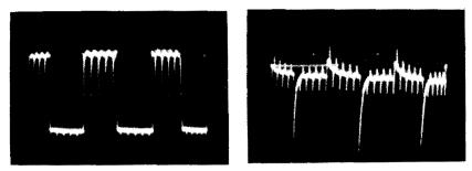
Fig. 550 (left). Waveform produced by mixing a 500-cycle square wave and 5,000-cycle pulses. Fig 551 (right). Waveform produced by mixing pulses of 500 and 5,000 cycles.
