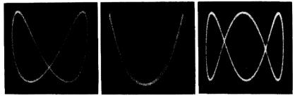
Fig. 419 (left). Lissajous figure where  $f_y/f_x = 2$ . Fig. 420 (center).  $f_y/f_x = 2$ . The two loops are superimposed, but are nevertheless counted. Fig. 421 (right).  $f_y/f_x = 3$ .
