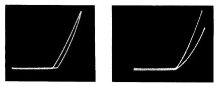
Fig. 605 (left). Phase shift produces a looped characteristic. Fig. 606 (right). Spread of characteristics of diodes from the same production run.
