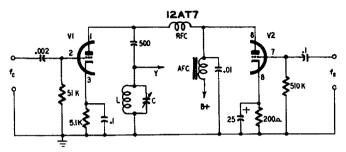
Fig. 7100. Technique for obtaining plate modulation. The audio cnoke is common to the plate circuits of both tubes.
