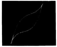
Fig. 641. Hysteresis loop of barium titanate capacitor.
