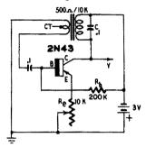
Fig. 745. Transistor oscillator circuit.
