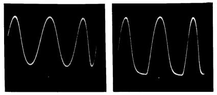
Fig. 832 (left). Detected signal at point A (junction of R1 and R2) in Fig. 829. Note absence of rf carrier. Fig. 833 (right). Demodulation distortion as a result of too high a value of diode load resistance (R1 in Fig. 829).
