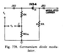
ing signal (frequency,  $f_s$ ). By impressing a low-frequency on a high-frequency wave, it can be transmitted by a radio link. At the receiving end of the link, the wanted information is extracted from the carrier by a process called demodulation or detection.
