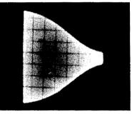
Fig. 799. Modulation characteristic (trapezoid) obtained with the circuit of Fig. 798. The percentage of modulation is 78%.
