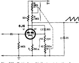
Fig. 240. Typical multivibrator type time-base generator.
