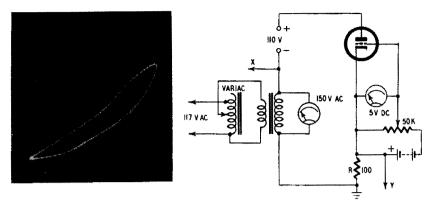
Fig. 617 (left). Looped characteristic due to phase shift. Fig. 618 (right). Circuit used for producing the  $I_n/E_a$  characteristics of triodes.
