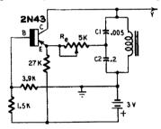
Fig. 753. Transistor oscillator using a two-terminal inductor.
