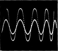
Differentiation of traces is also possible by varying the on-off ratio of the amplifiers, making one trace a bit fainter than the other. This is obtained by choosing unequal grid resistors in the multivibrator circuit.
