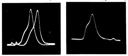
Fig. 319 (left). Single-trace pattern incorrectly phased. The two traces can be made to coincide by the proper use of a phasing network. Fig. 320 (right). Single-trace pattern blanked to avoid trace superimposition problems.
