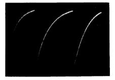
The voltage built up across a charging capacitor, however, is not proportional to time because of the exponential nature of the charging characteristic (Fig. 221). The charging current becomes lower and lower as the voltage across C approaches the voltage E of the charging power supply, resulting in a nonlinear sawtooth waveform as in Fig. 222.
