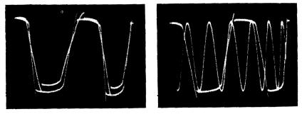
Fig. 330 (left). The clipped-wave amplitude is fairly independent of the input voltage. Outputs are shown for 80 and 150 volt rms inputs. Fig. 331 (right). Method of comparing the amplitude of the clipped calibrating voltage to the size of the unknown sine wave.
