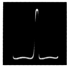
Fig. 921. Gating pulse at the screen grid of the burst amplifier tube.
