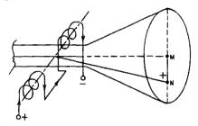
makes magnetic deflection of high-voltage tubes comparatively easy. Having no internal deflection system to align, television tubes are cheaper than comparable oscilloscope tubes and deflection coils may easily be operated at some fixed frequency.
