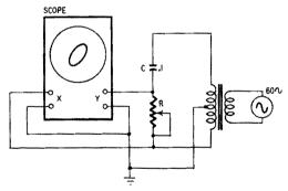
Fig. 522. Constant-amplitude phasing circuit using a tapped transformer.
