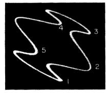
Fig. 449 (left),  $f_u/f_s = 5$ . Fig. 450 (right),  $f_u/f_s = 3$ .
