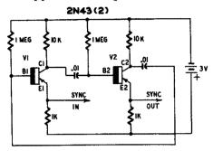
Fig. 768. Transistor multivibrator.
