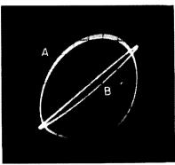
amplifier, while application of inverse feedback resulted in the flattened ellipse (B). Omission of capacitor C6 of the feedback loop (Fig. 801) reduced even this low phase shift to about zero.
