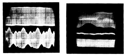
Fig. 822 (left). Intermodulation patterns: with negative feedback (upper trace); without feedback (lower trace). Fig. 823 (right). Push-pull amplifier intermodulation patterns: without feedback (upper trace); with feedback (lower trace).
