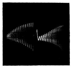
Fig. 256. Waveform of spiral sweep voltage of Fig. 255.
