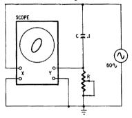
Fig. 520. Resistance-capacitance phasing circuit.
