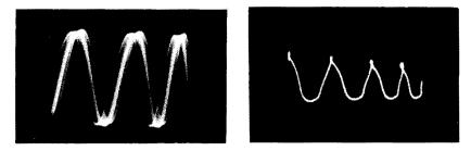
Fig. 1003 (left). Effect of a stray magnetic field on a higher-frequency sine wave. Fig. 1004 (right). Deflection produced by an external magnetic field on an unshielded CRT.
