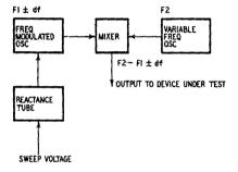
Fig. 325. Block diagram of a multiplerange sweep generator based on the bfo principle.
