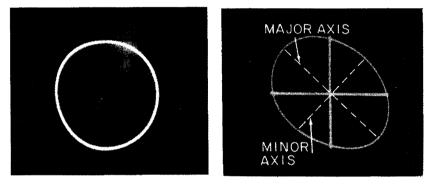
Fig. 417 (left). When a capacitor of negligible loss at the line frequency is substituted for Z in Fig. 416, a circle is obtained. Fig. 418 (right). Oscillogram used for measuring the inductance and resistance of a filter choke.
