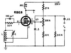
Fig. 791. Modulated high-frequency oscillator using a pentagrid tube.
