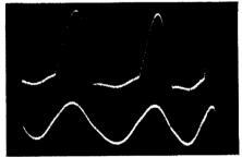
Fig. 7103. The upper trace (with the input filter capacitor omitted) shows the output of the half-wave rectifier of Fig. 7102. The lower waveform is a 60-cycle reference voltage.
