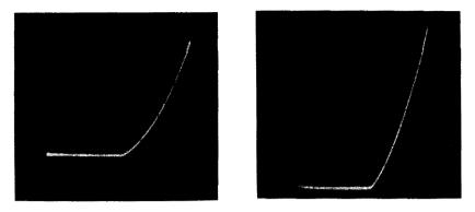
Fig. 608 (left). Characteristic of a 5V4-G rectifier tube. Fig. 609 (right). Characteristic of one section of a 6AL5 duo-diode. Note that there is no reverse current in vacuum tube diodes.
