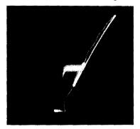
Fig. 749.  $E_c/E_b$  characteristic of the blocking oscillator.
