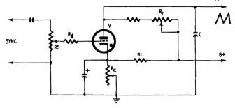
Fig. 223. Typical gas-triode time-base generator circuit.
