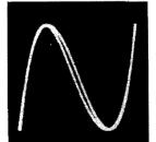
Fig. 422 (left).  $f_y/f_x = 3$ . Phase relationship differs from that of Fig. 421. Fig. 423 (right).  $f_y/f_x = 4$ .
