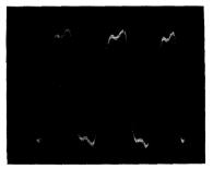
Fig. 510. 20% third harmonic. Due to different phasing, the distortion seems more severe. Note the definite symmetry of the flattened tops.
