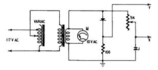
Fig. 602. Circuit used for tracing diode characteristics.
