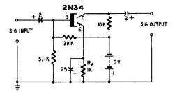
Fig. 721 (left). Effect of presence (A) and absence (B) of emitter bypass capacitor. Fig. 722 (right). Transistor amplifier circuit is stabilized when base bias voltage is obtained from a voltage divider.
