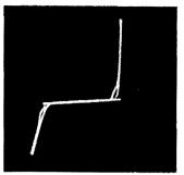
Fig. 645. Characteristic curves of an OA2 voltage-regulator tube.
