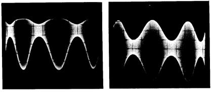
Fig. 830 (left). Clipped modulated rf wave at point D in Fig. 829 showing detection prior to filtering. Fig. 831 (right). Removing the diode detector (V2 in Fig. 829) results in reproduction of the signal generator output without demodulation.
