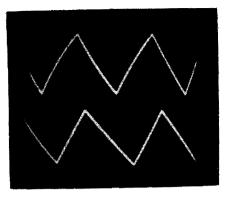
components. Decreasing R or C (that is, reducing the time constant RC) results in suppression of the lower-frequency components, thus emphasizing the "rapid" components. Mathematically speaking, this corresponds to a differentiation of the function represented by the waveform.
