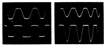
Fig. 532 (left). Square wave obtained with the diode clipper. The input voltages were 2 volts rms (above) and 10 (below). Fig. 533 (right). Clipped waveforms produced by using one diode only.
