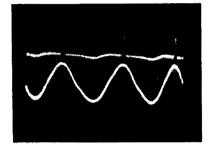
Fig. 7106. The charging current flows only during a small part of each cycle. The lower waveform is the reference voltage.
