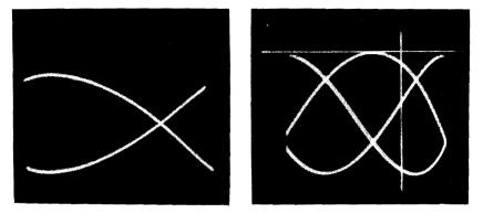
Fig. 467 (left). Time base running at twice the signal frequency.  $f_y/f_x = 1/2$ . Fig. 468 (right).  $f_y/f_x = 2/3$ . There are two complete loops tangent to the horizontal line and three traces crossing the vertical line.
