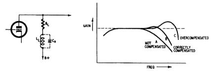
Fig. 204 (left). Peaking coil  $L_L$  extends the high-frequency response of a resistancecoupled amplifier. Fig. 205 (right). Effect of peaking on the high-frequency response of a resistance-coupled amplifier.
