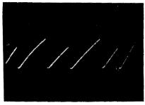
Fig. 236. Sawtooth voltage producing sweeps of different lengths.
