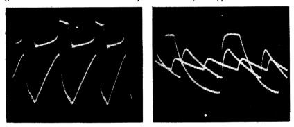
Fig. 246 (left). Above: grid voltage of blocking oscillator; below: sweep voltage across C1. Fig. 247 (right). Decreasing amplitude and increasing frequency result from increasing R1.
