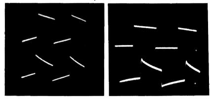
Fig. 806 (left). 10,000-cycle square wave. Fig. 807 (right). 20,000-cycle square wave. (These are the illustrations at the bottom of the page.)
