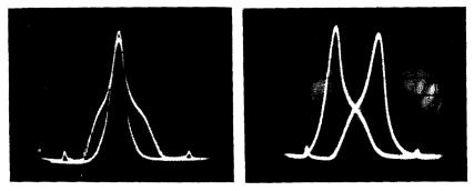
As it may be troublesome to manage an exact superposition of both traces, blanking is often preferred; that is, suppression of one of the traces by a suitably phased voltage applied to the C-R tube's control grid. Such a "blanked" single trace is shown in Fig. 320, the blanking voltage being derived from one X-deflection plate.
