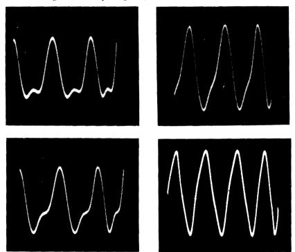
Fig. 507 (left). 10% second harmonic as in Fig. 505, but phased differently. Fig. 508 (right). 10% third harmonic. Note the symmetry of odd-harmonic distortion.
