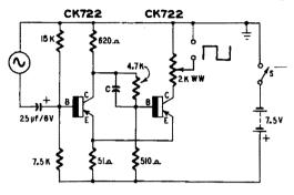
Fig. 537. Transistor version of the Schmitt trigger circuit.
