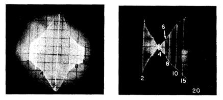
Fig. 327 (left). Resonance curve of L-C circuit covering 200 to 1,000 cycles. Fig. 328 (right). Transmission curve of twin-Tee circuit between 200 and 2,000 cycles. Note the null at 400 cycles.
