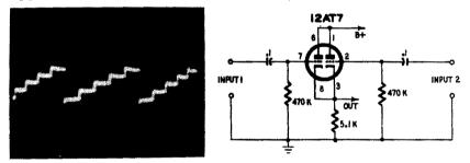
Fig. 548 (left). Staircase wave produced by two sawtooth waves. Fig. 549 (right). Simple mixer for the production of complex waveforms
