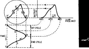
Fig. 317 (left). Generation of a single-trace pattern using a sine-wave sweep. The spot runs the curve in both directions. Fig 318 (right). Single-trace pattern, sine-wave sweep.
