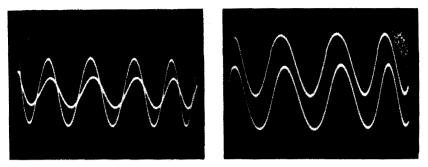
Fig. 310 (left). Oscillogram obtained with an electronic switch of the counter type. Note the neat traces and the absence of switching transients. Fig. 311 (right). Same as Fig. 310; the traces are separated.
