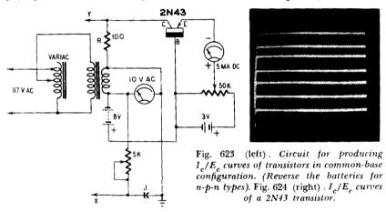
or breakdown may be experienced. The amplitude of the "signal" is sufficient for direct deflection of the C-R tube, and no phasing device is necessary.
