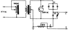
Fig. 640. Circuit for tracing the hysteresis loop of the nonlinear dielectric capacitor C1.
