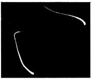
Fig. 762. P1/P2 characteristic of the multivibrator.
