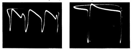
Fig. 728 (left). Increasing the amount of positive feedback reinforces the pulses. Fig. 729 (right). A large amount of feedback produces typical blocking oscillator operation.
