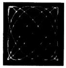
Fig. 429 (left).  $f_y/f_x = 6/5$ . Fig. 430 (right).  $f_y/f_x = 5/4$ .
