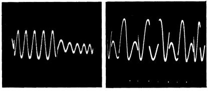
Fig. 303 (left). Successive operation of two channels of the electronic switch. Note the presence of switching transients (descending peak at the beginning of the low amplitude trace). Fig. 304 (right). If the switching frequency is a multiple of the sweep frequency an illegible pattern results.
