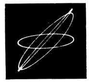
Fig. 519. Phasing ellipses obtained with R = 1,000, 10,-000 and 100,000 ohms (in the circuit of Fig. 518).
