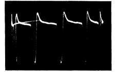
Fig. 744. Waveform of Fig. 743 when proper synchronization is used.
