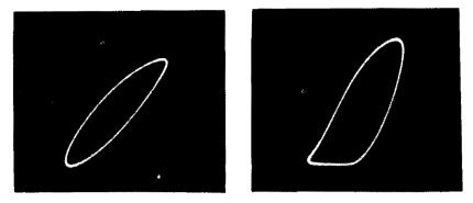
Fig. 835 (upper left). Lissajous pattern (modulated input vs detected output) showing correct detection. Fig. 836 (upper right). Increasing the value of the diode load resistor R1 (in Fig. 829) results in distortion. Compare this with Fig. 833. Fig. 837 (lower left). Connecting the scope to point B (in Fig. 829) shows the presence of rf in the detected wave. Fig. 838 (lower right). Selectivity curve (double trace). Frequency correct; some skirt dissymmetry.
