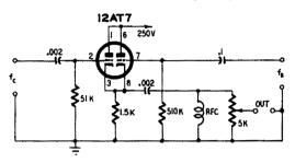
Fig. 798. Cathode-coupled modulator devised by by the author.
