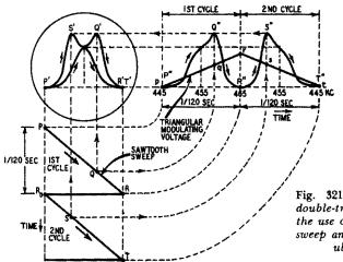
Fig. 321. Generation of a double-trace pattern through the use of a sawtooth-shaped sweep and a triangular modulating voltage.
