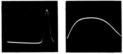
Fig. 845 (upper left).Single trace. Incorrect sweep frequency shifts the trace. Fig. 846 (upper right). Sweep width too low. Only the top of the curve appears. Fig. 847 (lower left). Sweep width is too high. No detail is visible on the curve. Fig. 848 (lower right). Instability on the low-frequency side of the curve.
