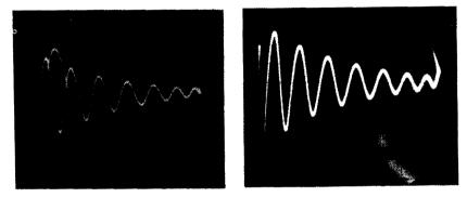
Fig. 333 (left). Oscillogram of the damped timing oscillation which starts at the end of the linear sweep. Fig. 334 (right). Return-trace blanking eliminates the confusing first part of the calibrated wave. If the return trace time is short compared to sweep time, blanking is not required.
