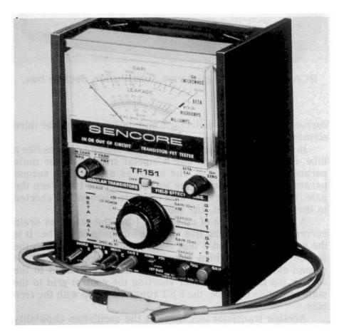
Sencore Model TF151 transistor tester designed to check bi-polar and field-effect transistors.
