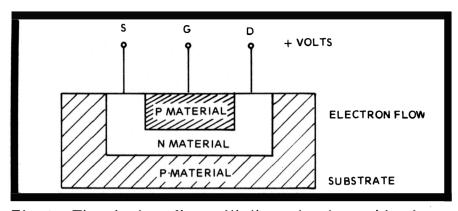
Fig. 71. The electron flow with the gate at zero bias is an important parameter, IDSS.
