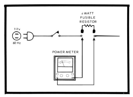
Fig. 23. A good power meter can test the exact current that an electronic unit draws to verify fuse capability.
