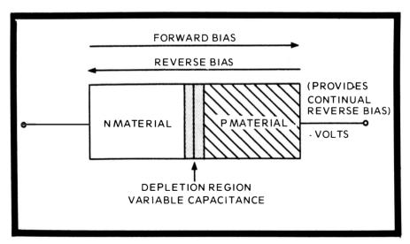
Fig. 80. A varicap diode is operated only with reverse bias. During forward bias there is no variable capacitance.
