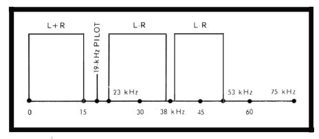
Fig. 22. The stereo multiplex transmission covers a large part of the available 75-kHz allowable bandwidth.
