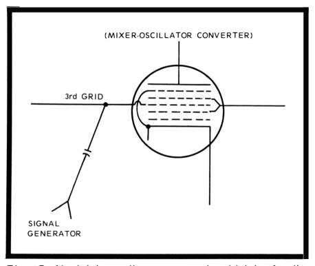
Fig. 2B. Most tube radios use a pentagrid tube for the mixer oscillator function.
