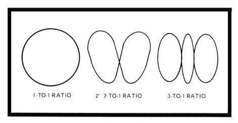
Fig. E. A Lissajous figure scope display reveals the ratio between the input voltage frequencies.
