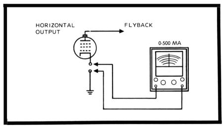
Fig. 25. The color TV horizontal output cathode current is a critical test with a 0-500 milliammeter.
