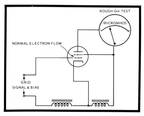
Fig. G. Some commercial testers actually provide a rough Gm test with this basic circuit.
