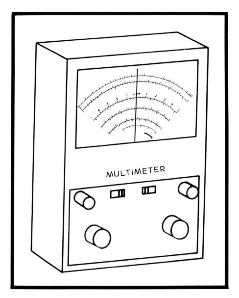
Fig. 87. Most multimeters have a zero-center scale. In some cases, it's very useful.
