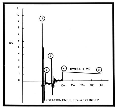
Fig. 111. Typical waveform across the ignition coil primary.
