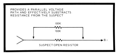
Fig. 82. By installing a known good resistor across another resistor, they form a parallel circuit and subtract if the original resistor is OK.
