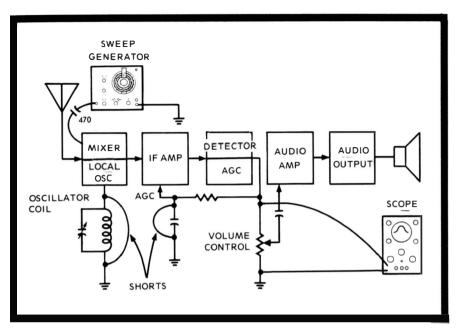
Fig. 2A. A sweep generator and an oscilloscope provide an exact method for AM peak alignment.
