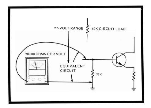
Fig. 86. Using a 20,000 ohms-per-volt VOM in the 2.5-volt range is like putting 50K across the circuit.
