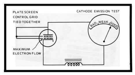
Fig. F. Most tube testers simply measure cathode emission. It follows that other characteristics probably are good if the cathode emission is good.
