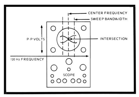
Fig. 12C. A trick to achieve closer discriminator alignment is to double the scope's horizontal frequency.
