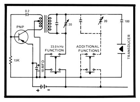
Fig. 89. The transmitted wave can be in the audio range. It is produced by a transducer which creates sound waves in the air.
