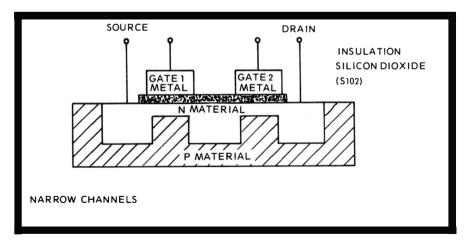
Fig. 69. A metal oxide semiconductor FET (MOSFET) is so named because of the oxide dielectric insulation.
