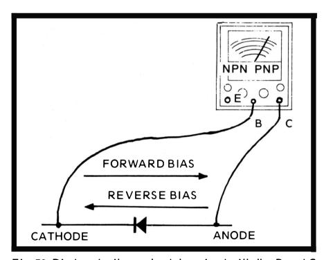
Fig. 78. Diode polarity can be determined with the B and C transistor tester leads. Forward bias will deflect the needle.
