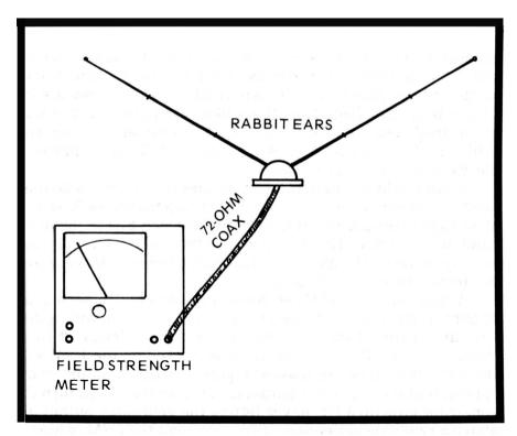
Fig. 50. To conduct a satisfactory signal strength survey test, ordinary "rabbit ears" can be used.
