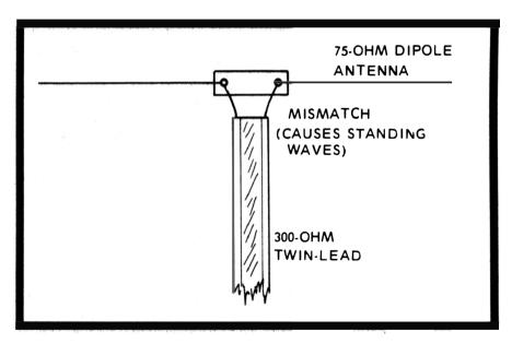
Fig. 52. Standing waves are caused by impedance "bumps" in mismatched antenna components.
