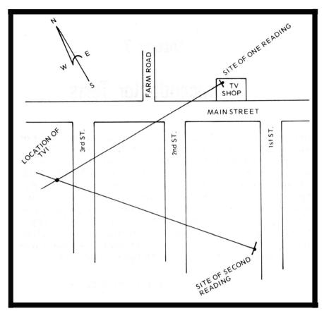
Fig. 57. Triangulation of a TVI source leads to its indentification and then to the eventual riddance of it.
