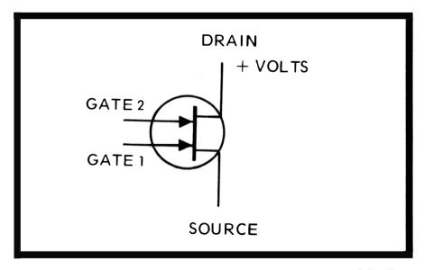
Fig. 70. The schematic diagram of a dual-gate MOSFET, N-channel type.
