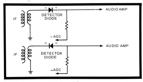
Fig. 11. You can tell if the AGC is positive or negative by observing the polarity of the diode attached into the AGC.
