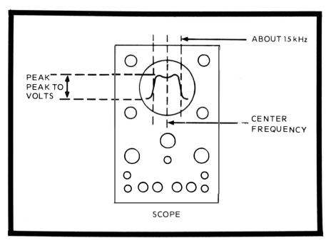
Fig. 3B. The typical AM broadband response curve is 15 kHz wide and approaches a square wave.
