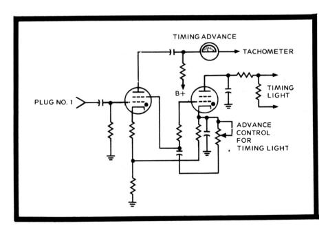
Fig. 115. A typical timing light circuit receives an input pulse every time the rotor fires the number one spark plug.
