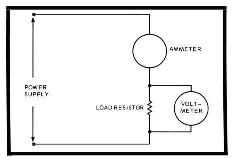
Fig. B. An ammeter in series with the load measures the amperage drawn by the load. An ammeter in shunt with a load measures the voltage across the load and, in effect, is a voltmeter.
