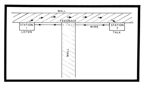
Fig. 103. During intercom installation, stay away from common walls to avoid unwanted feedback.
