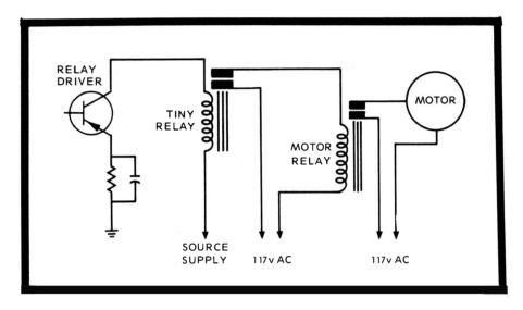
Fig. 109. Typically, a motor relay in a garage door opener is a heavy duty type. It's operated by a tiny circuit relay.
