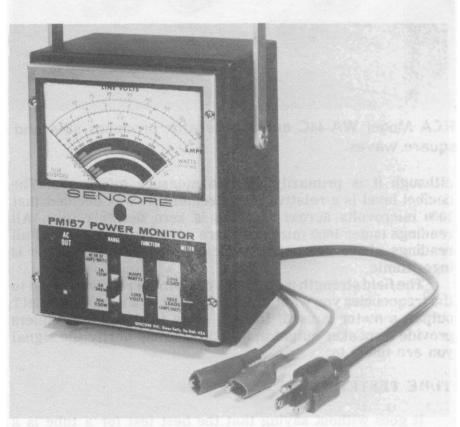
Sencore PM157 power monitor measures line voltage, current and watts.
