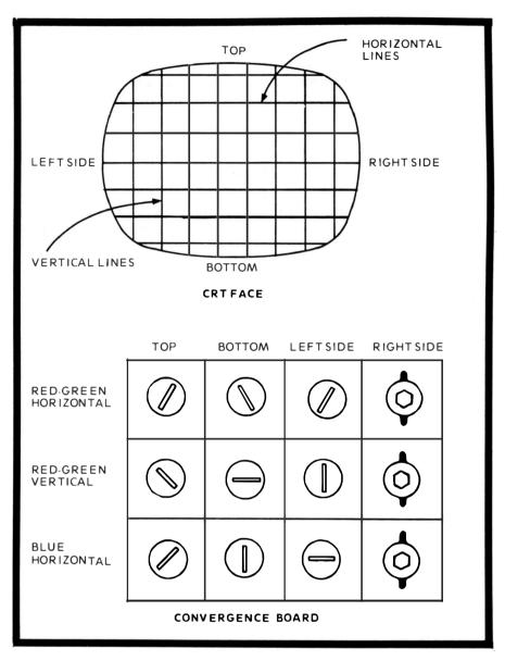
Fig. 29. The twelve adjustments on the convergence board and the crosshatch from a color generator are used in convergence adjustments.
