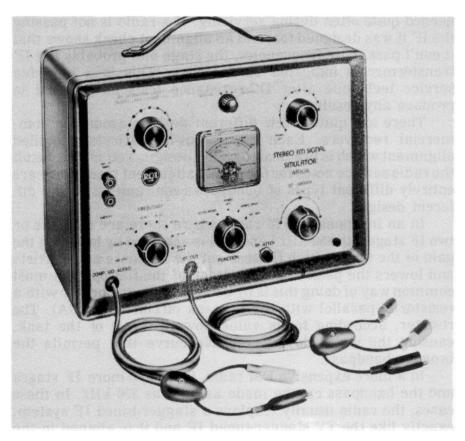
Stereo signal generator, RCA Model WR-52A.
