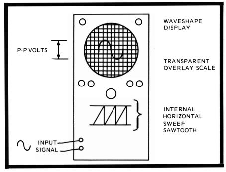
Fig. D. A scope displays circuit waveforms and the amplitude in p-p volts when calibrated.
