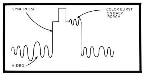
Fig. 30. The composite TV signal has about eight "rings" of color burst on the horizontal sync "back porch."
