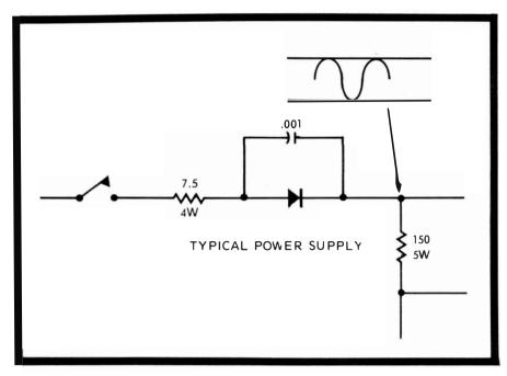
Fig. 85. Ripple voltage is usually too low to cause trouble, but it's useful to have the capability to test it.
