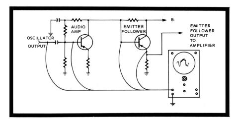
Fig. 98. A scope can be used to trace through the organ circuitry, since it only has to follow the oscillator signal.
