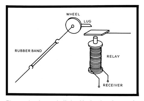
Fig. 93. A relay controlled rubberband motor can be slowly unwound by repeated movement of the relay.
