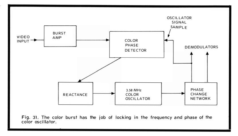
oscillator voltage. If the voltage does not increase, the burst amplifier is causing the trouble. When the voltage does rise, the burst amplifier is cleared. While you are there, adjust the burst transformer for maximum voltage, which correctly aligns the transformer.
