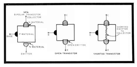
Fig. 61. A transistor breaks down by opening, shorting or leaking. A transistor tester quickly reveals the condition.
