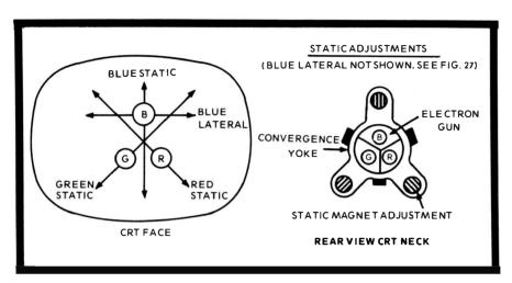
Fig. 28. The blue lateral, red, geeen and blue statics are all adjusted to achieve convergence at screen center.
