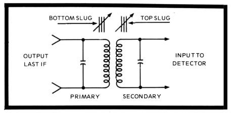
Fig. 1B. The top slug is the secondary and the bottom slug is the primary in a typical IF transformer.
