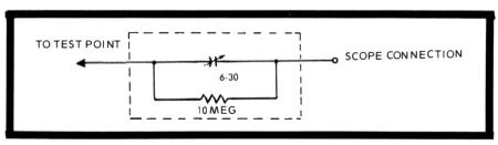
Fig. 41. A typical high-impedance probe isolates the scope from the circuit under test and reduces any loading.
