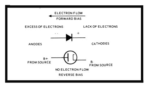
Fig. 77. Diode polarities can be confusing since they are marked positive on the cathode and negative on the anode.
