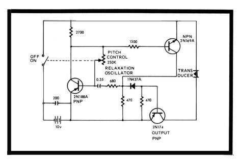
Fig. 101. Electronic vocal chords have been devised using this Bell Lab oscillator circuit and transducer.
