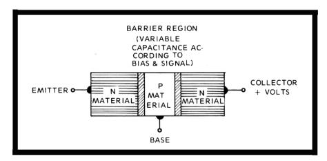
Fig. 67. A bipolar transistor has a depletion region or barrier region between the material junctions.
