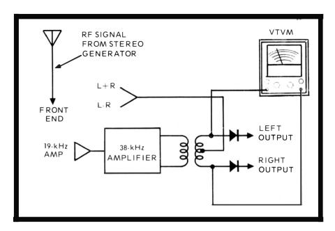
Fig. 21. Multiplex alignment requires a stereo generator input and a VTVM indicating device.
