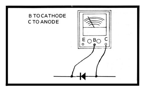
Fig. 79. Diodes can be tested out of circuit by attaching to B and C tester leads.
