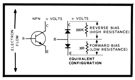
Fig. 60. The bipolar transistor has characteristics similar to two diodes connected back to back.
