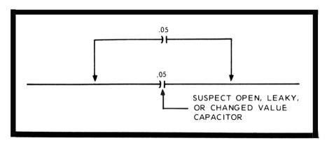
Fig. 83. By installing a known good capacitor across another capacitor values add.
