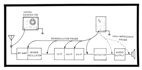
Fig. 38. Signal tracing through a receiver is easy when you have a scope, generator and correct probes.
