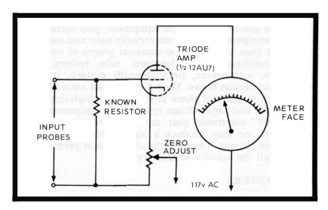
Fig. A. When a triode tube in a VTVM has a voltage input, it causes a proportional change in the ammeter reading in its plate circuit. The triode has a large input impedance so circuits under test are not loaded down.
