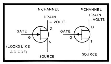
Fig. 65. Depletion-type FET schematic representation. The arrow points at N and away from P.
