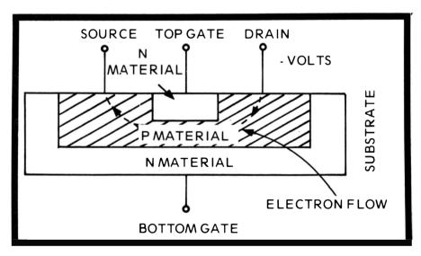
Fig. 64. In a P-channel FET, the electron flow is from drain to source. The gate serves as a valve.
