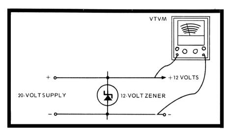
Fig. 81. A zener diode can be tested by installing it in a test circuit, with cathode toward the positive voltage.
