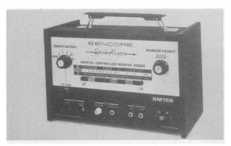
Marker generator, Sencore Model SM158, provides signals for TV IF, chroma and RF alignment.
