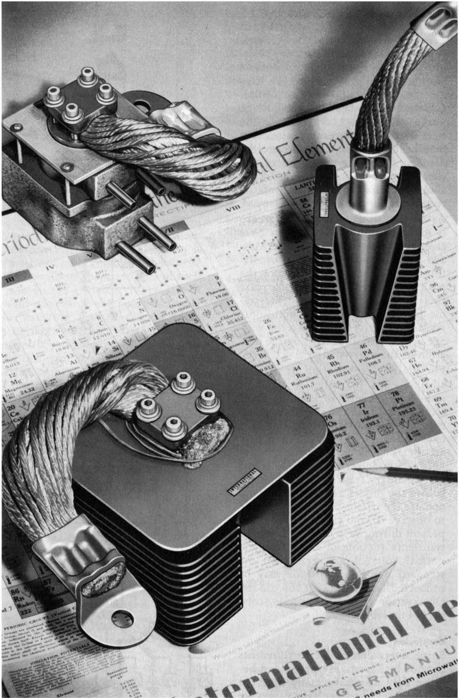
Fig. 2. Representative collection of germanium power rectifiers. Forced air-cooled units shown are rated from 330 amp to 500 amp half wave. The liquid-cooled unit at upper left is rated 667 amp (half wave) up to 66 v r.m.s. input.
