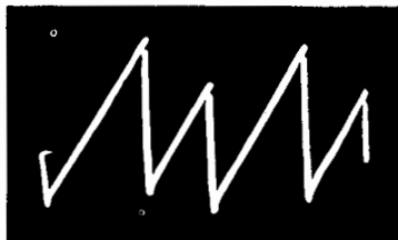
(B) Sawtooth signal developed at second section.
