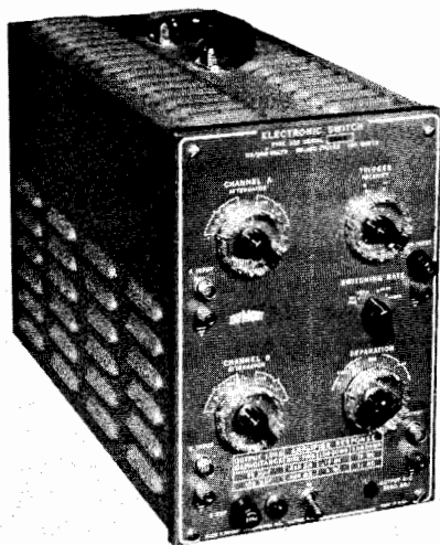
Fig. 7-20. The DuMont Model 330 electronic switch. (Courtesy of Allen B. DuMont Laboratories, Inc.)
