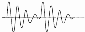
Fig. 3-11. A train of damped sine waves applied to the RC network of Fig. 3-9 will produce a spiral trace.
