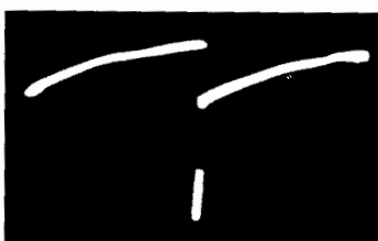
Fig. 12-7. Vertical deflection waveform from vertical output stage.
