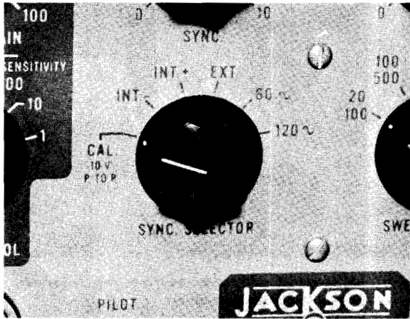
Fig. 6-3. Sync selector includes CAL position for internal calibrating voltage.
