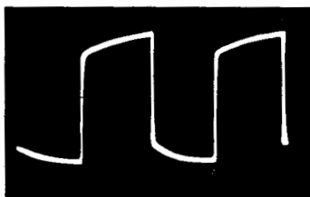
Fig. 10-4. Effect of bass boost on square wave signal.
