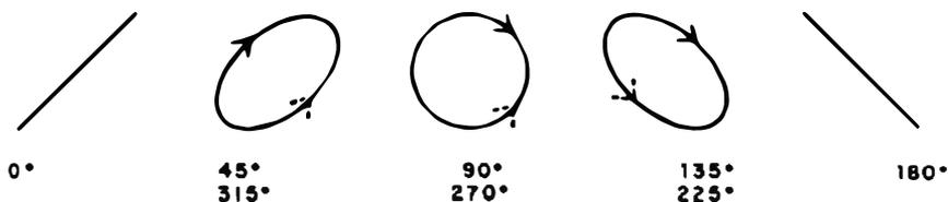
Fig. 2-47. Lissajous patterns show phase difference between two sine waves.
