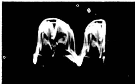
Fig. 5-6. Negative-going noise-gate signal applied to point F.
