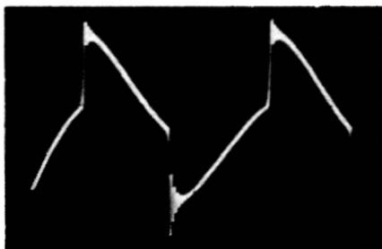
**Fig. 4-29. Differentiation, ringing, and overshoot in a reproduced square wave.**
