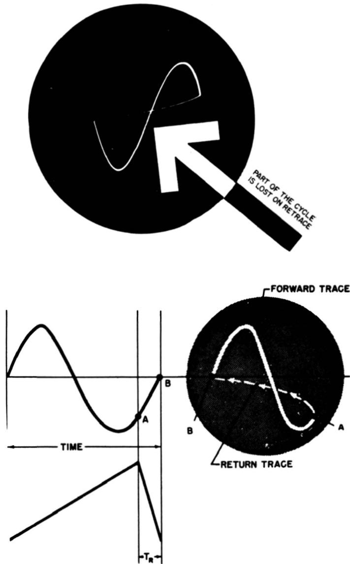
Fig. 2-13. Detail of a single-cycle display.
