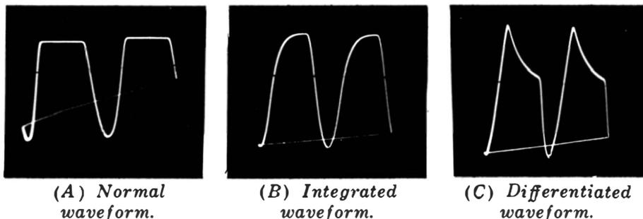
Fig. 4-24. Hybrid sine and square waves.
