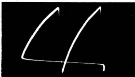
Fig. 6-4. Normal sawtooth waveform from horizontal-oscillator circuit.
