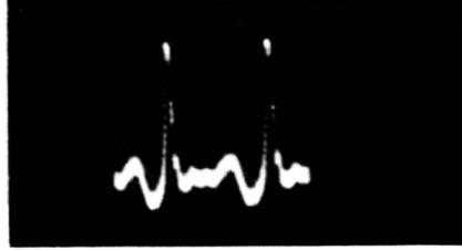
(B) Distorted waveform, using demodulator probe.
