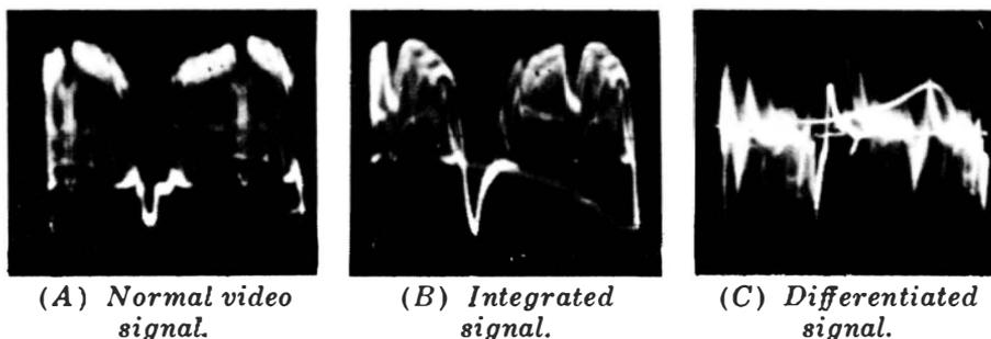
Fig. 4-23. Normal and abnormal video waveforms in Fig. 4-21.
