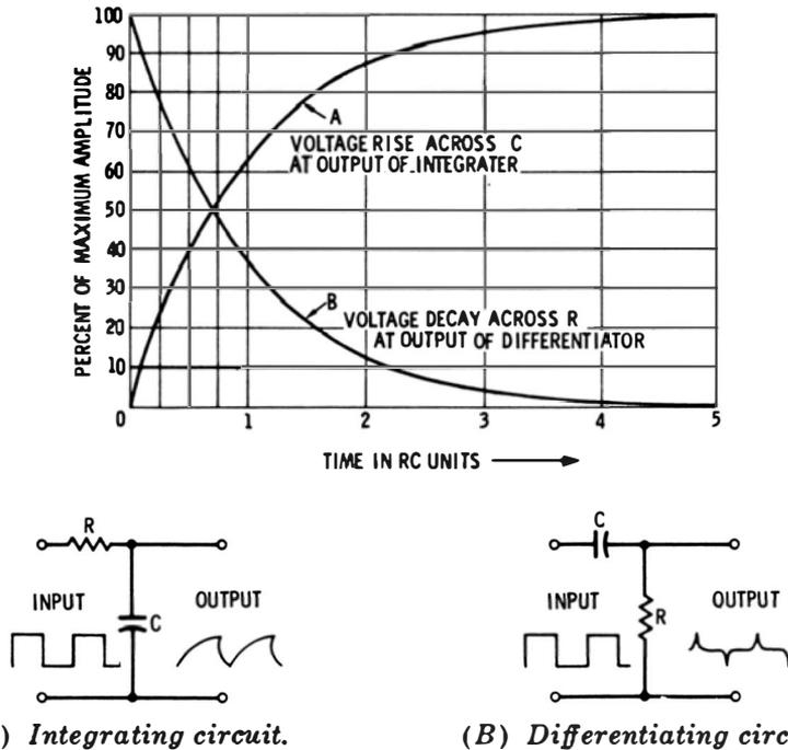
Fig. 1-8. Universal r-c time-constant chart showing the effects of integrating and differentiating circuits on a square-wave input.
