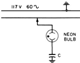
Fig. 3-24. Capacitor provides return path.
