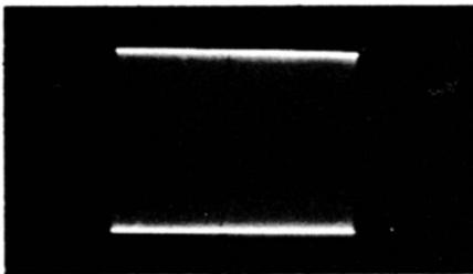
**Fig. 2-11. Waveform appears as a blur on the screen when horizontal-sweep rate is too low.**
