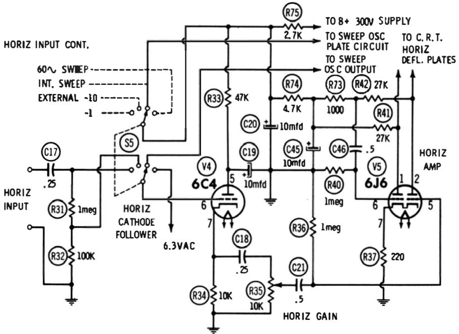
Fig. 2-24. Typical horizontal-amplifier circuit.
