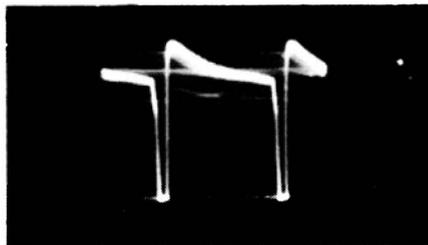
Fig. 6-19. Mixed pulse and sawtooth waveform.
