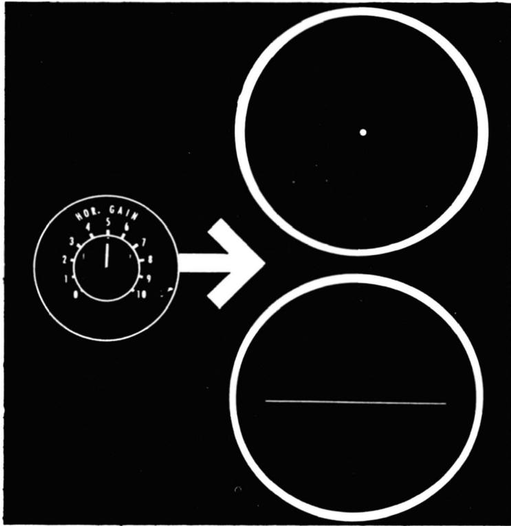
Fig. 2-7. Action of horizontal-gain control.
