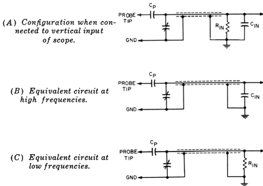
**Fig. 3-15. High-voltage capacitance-divider probe and its load circuit.**
