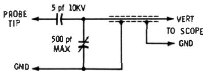
Fig. 3-13. Typical high-voltage capacitance-divider probe.
