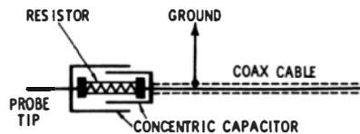
very little distortion. For example, a square wave or pulse with a rise time of 0.02 microsecond passes through a lab-type probe with practically no overshoot or ringing.
