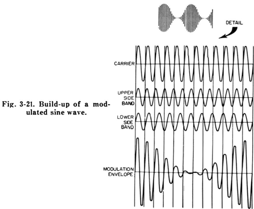
Fig. 3-21. Build-up of a modulated sine wave.
