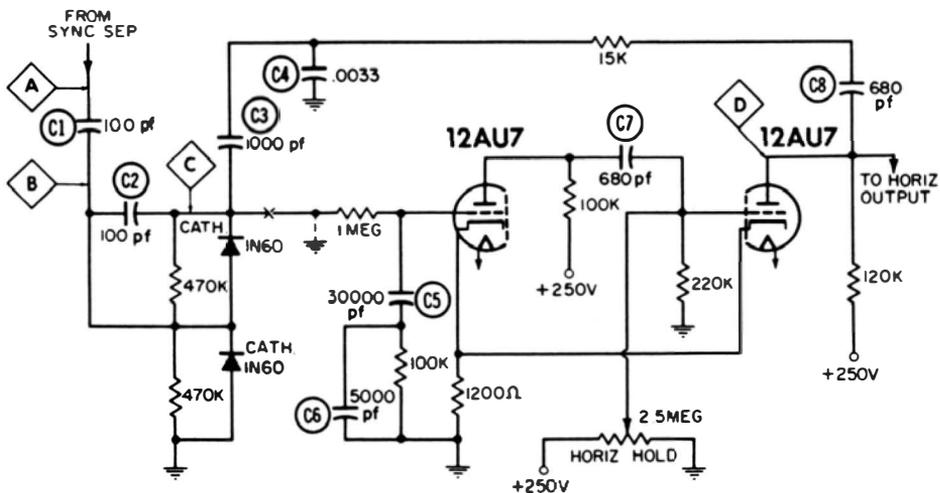
Fig. 6-1. Typical horizontal-oscillator and -afc configuration.
