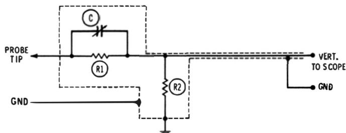
Fig. 3-3. Low-capacitance probe.
