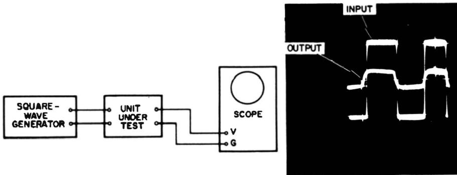
Fig. 2-52. Result of a typical square-wave test.
