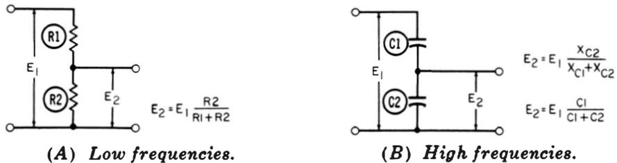
Fig. 2-19. Voltage dividers for low and high frequencies.
