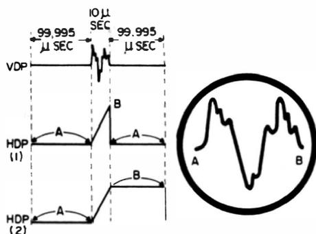
Fig. 2-40. Sweep-magnifier action — suitable for repetitive waveforms only.
