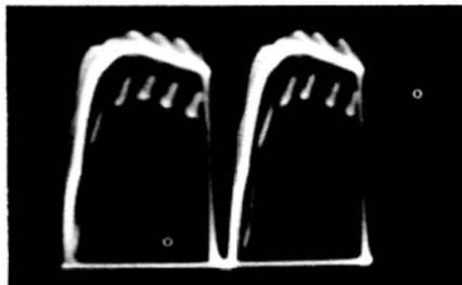
Fig. 6-9. Waveform at point B when C4 is open.
