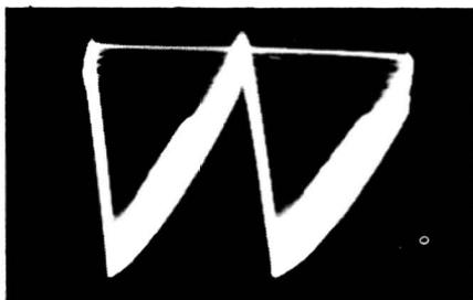
Fig. 6-6. Waveform at point B when C1 is open.
