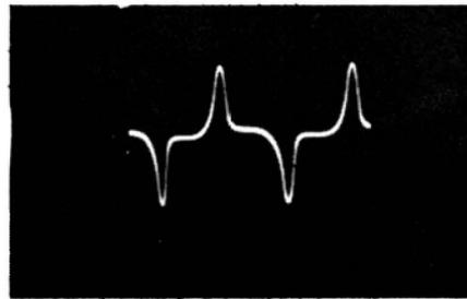
Fig. 10-6. Pulse current without a sine-wave component.
