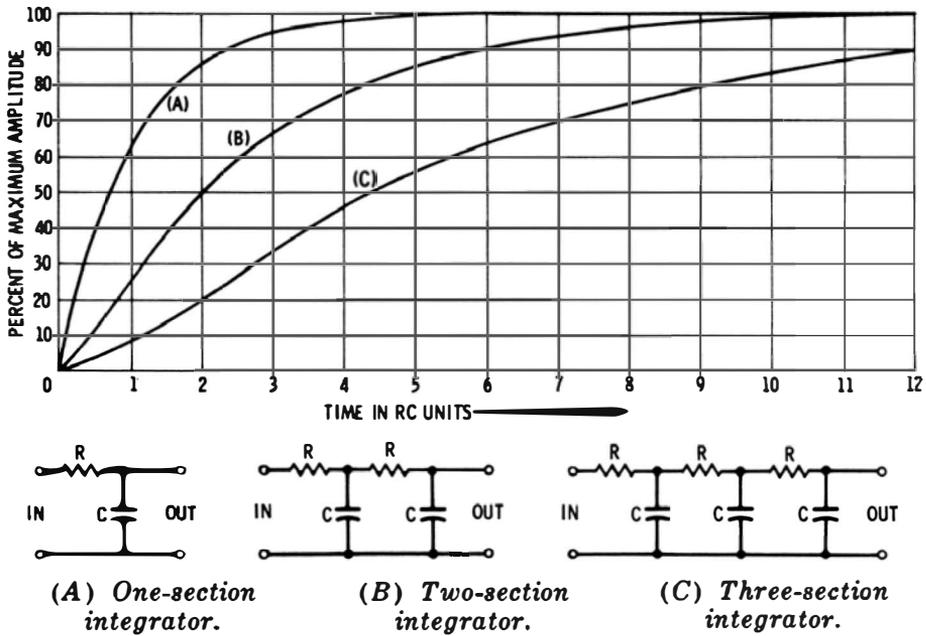
Fig. 1-9. Universal time-constant chart for one-section, two-section, and three-section integrator circuits.
