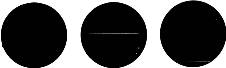
(A) +10 volts applied to vertical input. (B) 0 volts applied to vertical input. (C) -10 volts applied to vertical input.
