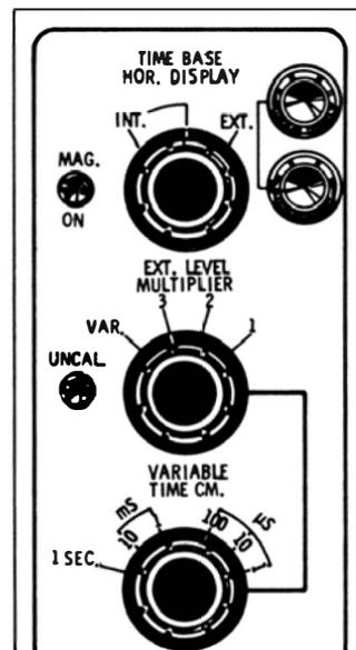
likewise increased 500 times, the waveform detail appears clearly, as illustrated in Figs. 2-42B and C. Similarly, a pulse, square-wave, or video signal can be expanded for analysis of detail.
