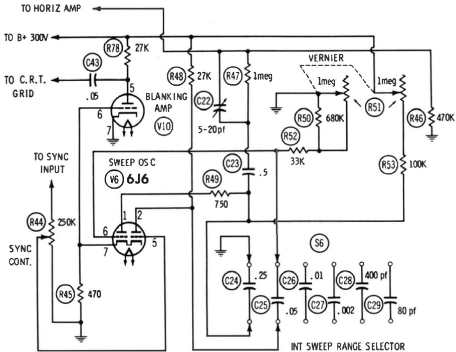
Fig. 2-25. Typical sawtooth-sweep oscillator and blanking amplifier.
