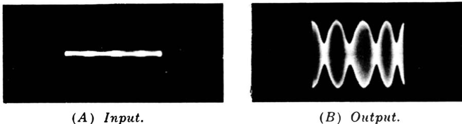
Fig. 11-3. Basic gain displays.
