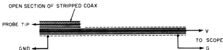
Fig. 7-10. Special high-voltage capacitance-divider probe.
