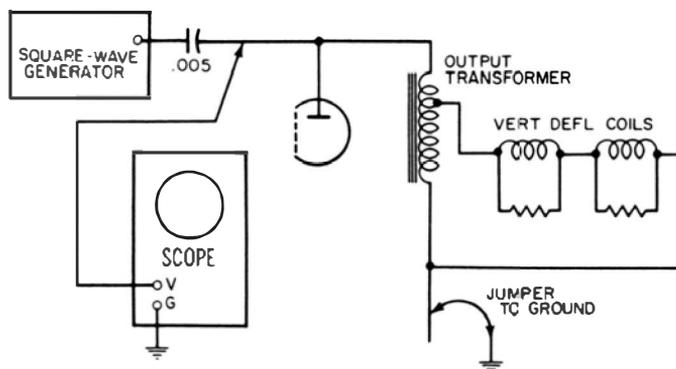
Fig. 8-11. Test setup for shorted turns.
