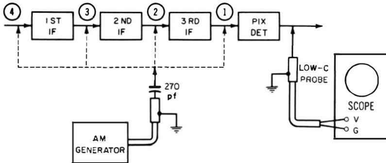
Fig. 4-18. Stage-gain test setup.
