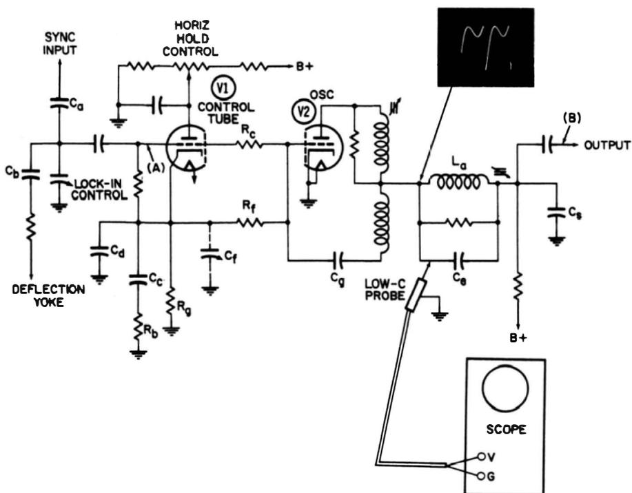
Fig. 6-15. Signal check of Synchroguide ringing-coil adjustment.
