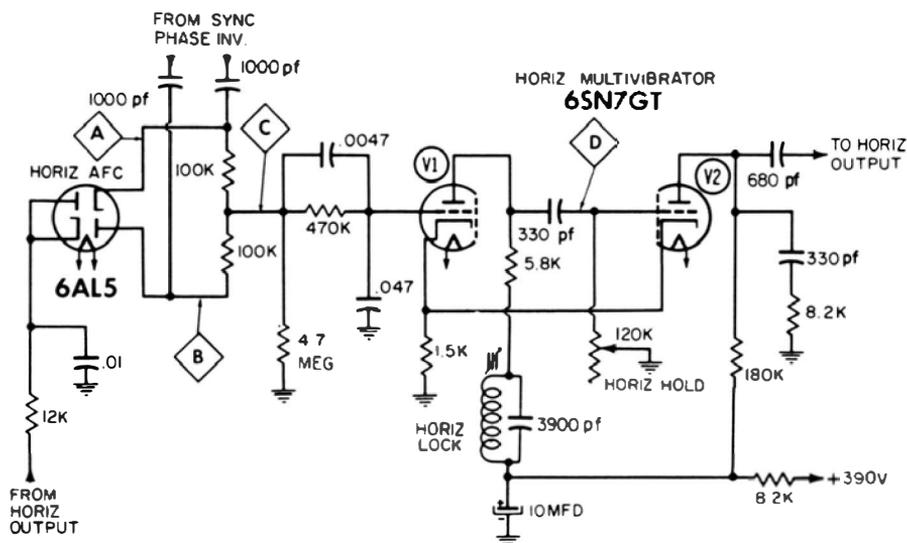
Fig. 6-17. Multivibrator with ringing coil.
