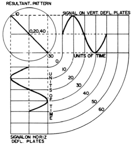
harmonics in the 60-Hz voltage to the vertical or horizontal amplifier, or both, a perfect circle cannot be obtained. Irregularities are seen instead.
