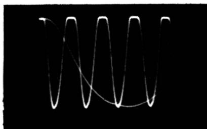
Fig. 12-8. Severe even-harmonic distortion of a sine wave.
