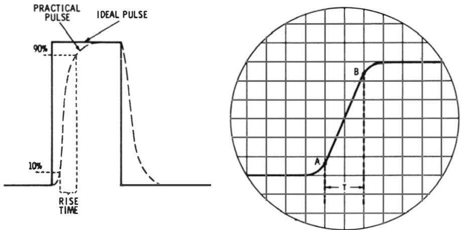
(A) Rise time is measured from the 10 percent point to the 90 percent point on the leading edge of the pulse.
