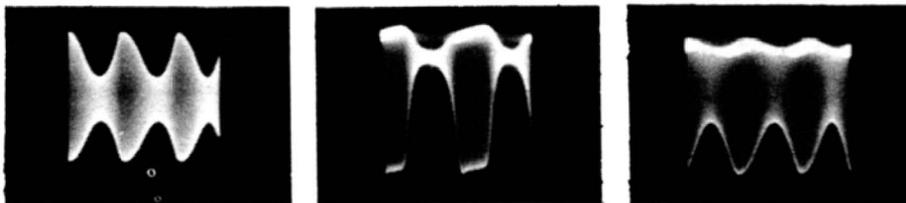
Fig. 9-7. Distorted outputs from an a-m generator.
