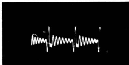
(B) *Breakdown in high-voltage winding.*
