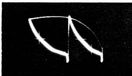
speeds up, and the picture cannot be locked. The increased oscillator frequency causes additional cycles to appear in the pattern when the scope is deflected at a 30-Hz rate. Leakage in C3 has much the same effect as capacitance loss because the negative d-c grid bias is bled to ground.
