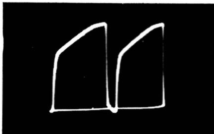
Fig. 6-12. Normal output waveform from horizontal oscillator.
