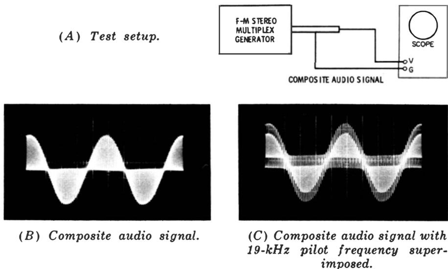
**Fig. 11-10. Multiplex generator output check.**
