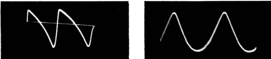
Fig. 10-4. Typical waveforms at filter input.
