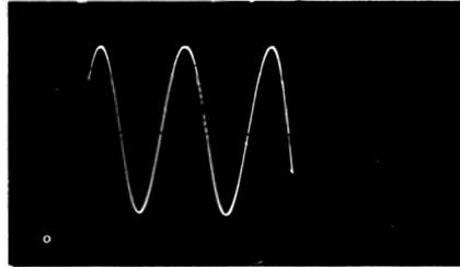
Fig. 4-4. An a-m generator displays a sine-wave signal.
