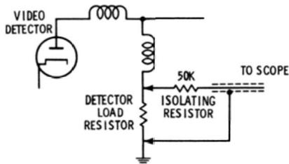
position (if the marker is on the steep side of a curve) is displaced. On the other extreme, broad markers result when the time constant is too short. In general, a 50-K resistor with a conventional coaxial cable gives a good response in sweep-alignment work.
