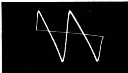
Fig. 6-18. Comparison sawtooth from the sweep circuit.
