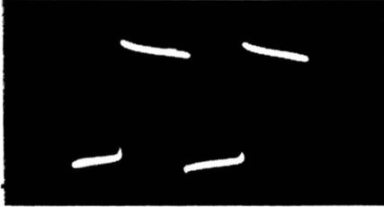
**Fig. 12-11.** Tilt in top of square wave is caused by low-frequency attenuation and phase shift.
