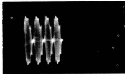
Fig. 11-6. Envelope changes with receiver tuning due to incidental f-m.
