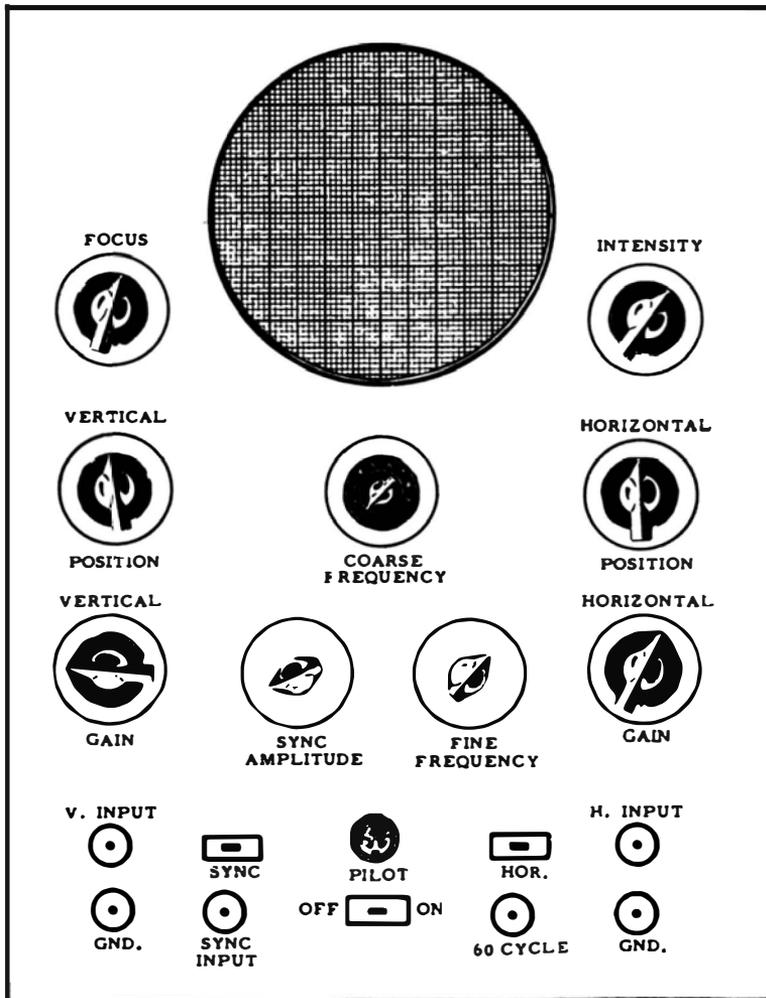
Fig. 2-1. Typical panel layout for a simple oscilloscope.
