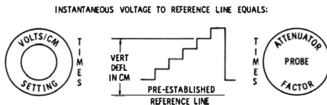
**Fig. 3-7. Reading the instantaneous voltage at a point along a waveform.**
