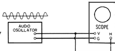
Fig. 12-1. Check of scope linearity
