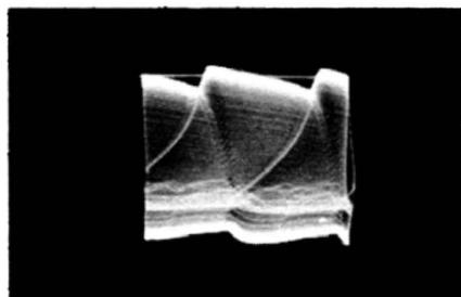
Fig. 6-10. Waveform at point B when C5 is open.
