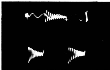
**Fig. 12-15. Severe ringing occurring in square-wave test.**
