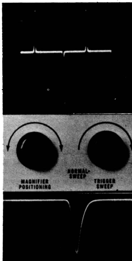
In Fig. 2-39, when the "Trigger-Sweep" control is turned completely to the left, the cut-off bias is removed from the sawtooth oscillator, and ordinary sawtooth deflection takes place. By advancing the horizontal-gain control to maximum, a certain amount of horizontal expansion is possible when ordinary sawtooth deflection is used. However, the obtainable expansion is considerably less than when triggered sweep is used.
