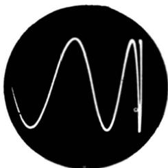
Fig. 2-27. Severe horizontal nonlinearity.
