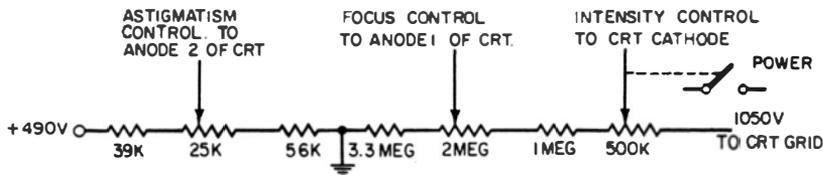
Fig. 2-5. Focus and intensity functions.
