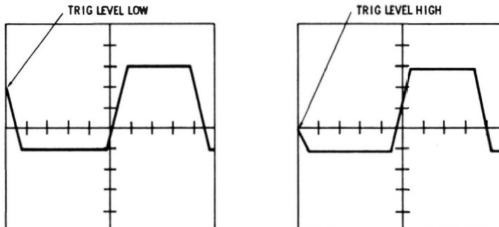
**Fig. 2-46. This waveform is being triggered along its negative slope (falling interval).**
