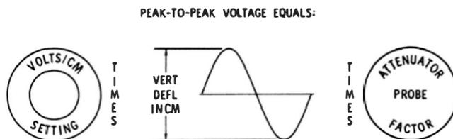
**Fig. 3-6. Reading peak-to-peak voltage from vertical-gain control setting.**
