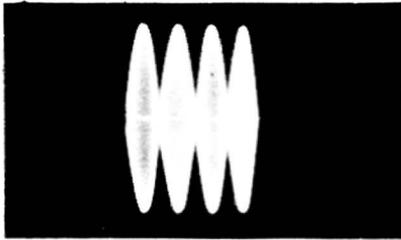
(A) Output waveform from a-m generator.
