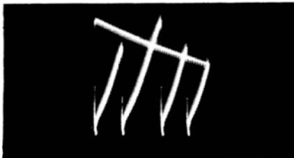
**Fig. 10-8. Alternate peaks of the signal have different heights.**
