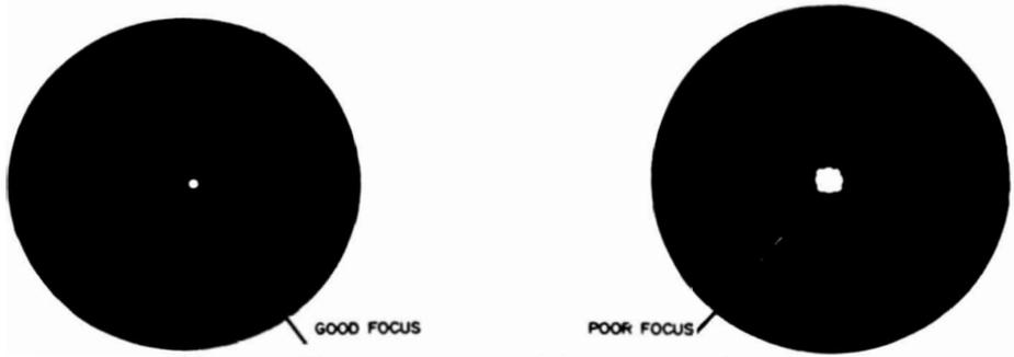
Fig. 2-4. Action of focus control.
