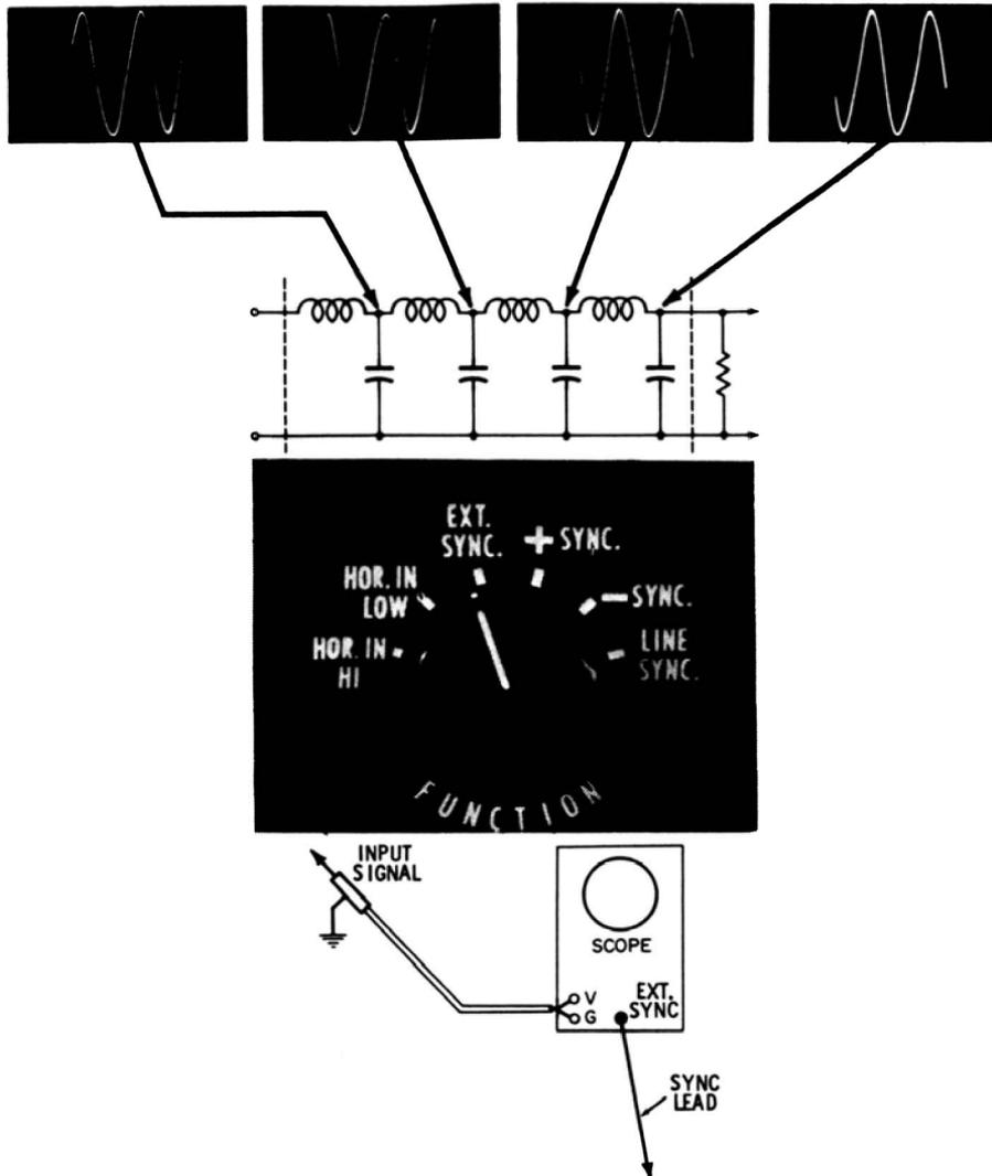
Fig. 2-38. External sync is used when checking out a generator delay line.
