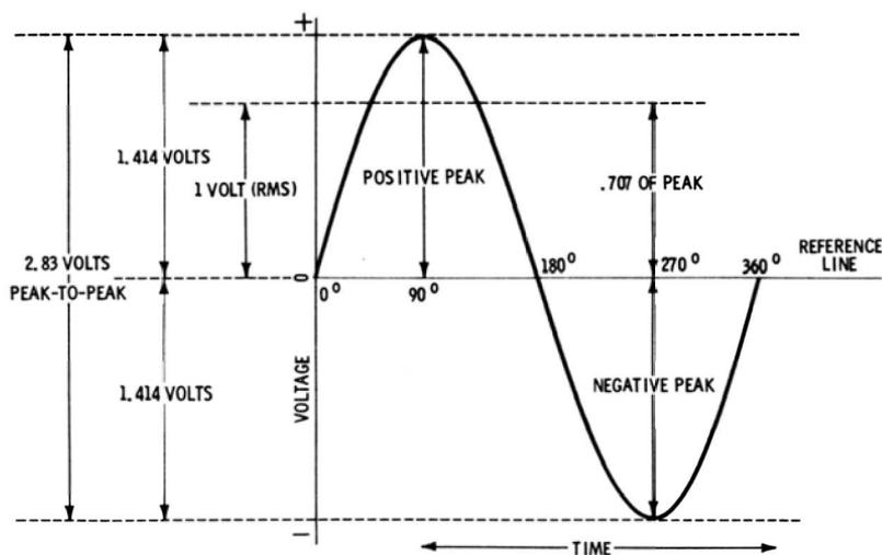
Fig. 1-1. The fundamental sine wave.
