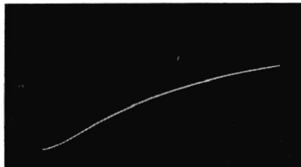
**Fig. 1-13. Square-wave response of a 2-1 unsymmetrical two-section integrator.**
