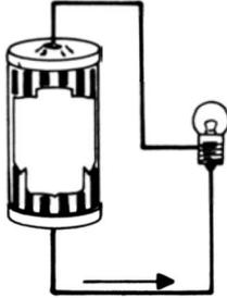
Fig. 3-23. If one of the leads is omitted, the lamp does not light.
