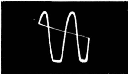
Fig. 9-10. Negative peak clipping of the audio signal.
