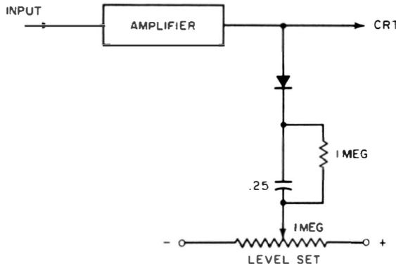
Fig. 5-10. Circuit for automatic centering.
