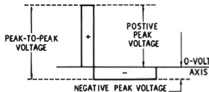
Fig. 2-33. Pulse-waveform voltages.
