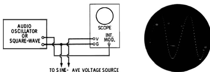
Fig. 2-29. Instantaneous voltages "marked" and timed by intensity modulation of the scope.
