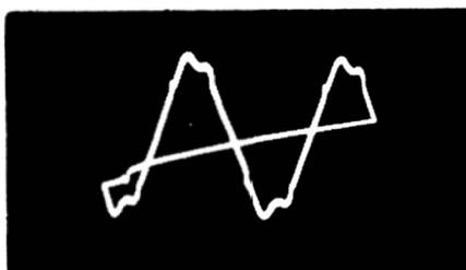
The stray-field pattern disappears if the probe or leads are connected across a resistor, capacitor, or inductor. Appearance of the stray-field pattern on open circuit is due to the high input impedance and high sensitivity of the scope. Stray fields are a source of very high impedance voltages. When the input impedance to the scope is reduced by connecting the input leads or probe across a component, stray fields induce a negligible voltage into the leads.
