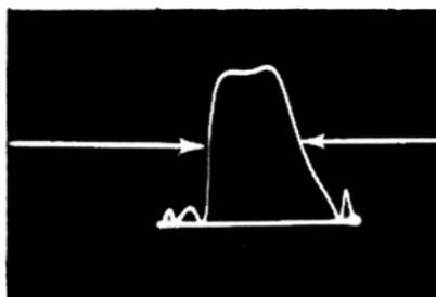
**Fig. 4-10.** Bandwidth is measured between the 6-db points.
