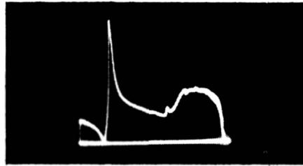
pattern will again change rapidly. Because the i-f response curve is so sharply peaked (Fig. 4-11), a small change in stray capacitance shifts the ringing frequency considerably. Regeneration is also responsive to signal-level (agc bias) changes. The reason for this dependency is that the sharpness of the peak depends greatly on the amount of i-f signal being fed back. When the i-f gain is reduced, less i-f voltage
