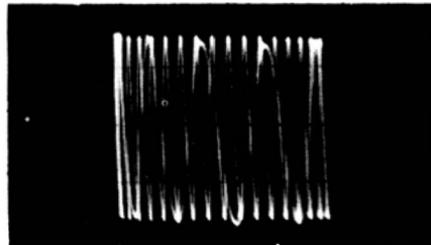
Fig. 11-5. The unmodulated output from the signal generator.
