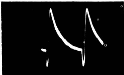
Fig. 6-8. Waveform at point B when C3 is open.
