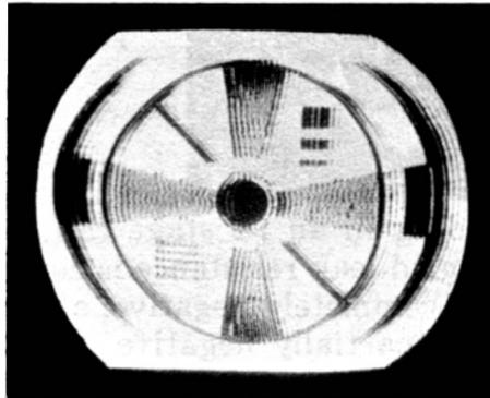
**Fig. 4-12. Distortion caused by i-f regeneration.** is fed back. This reduces the amplitude of the peak and increases the bandwidth.
