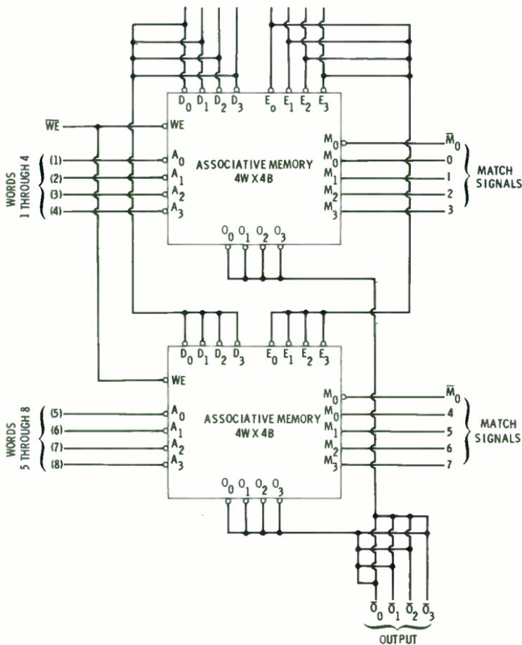
Fig. 9-12. Diagram for expanding word length.
