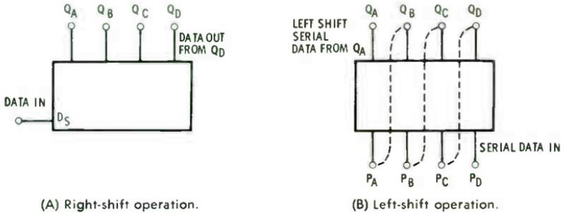
Fig. 5-6. Operational method of Fig. 5-5.
