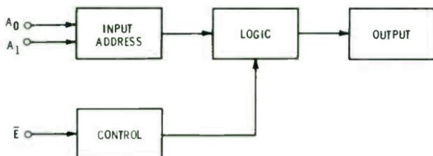
Fig. 3-2. Basic functions of a decoder circuit.
