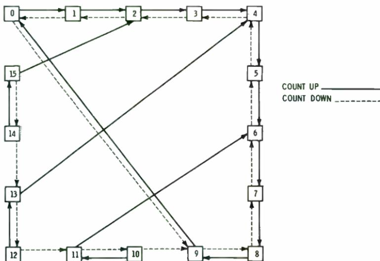
Fig. 6-18. State diagram of count sequence for Fig. 6-16.
