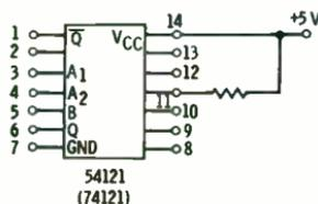
(C) Pulse width stabilizing circuit added.
