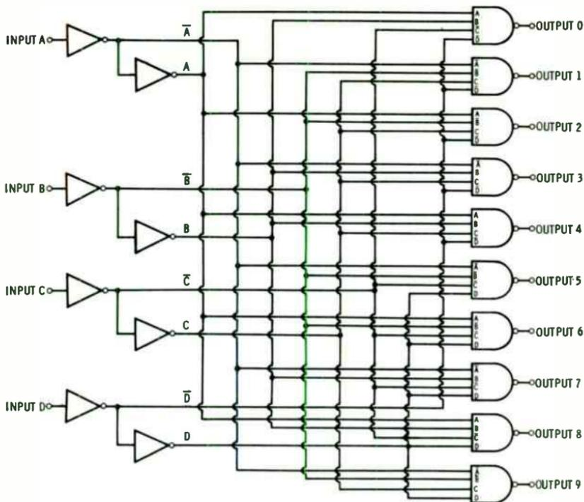
Fig. 3-6. Excess-3-to-decimal decoder functional block diagram.
