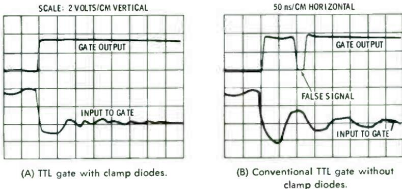
Fig. 11-3. Effect of input clamping diodes.
