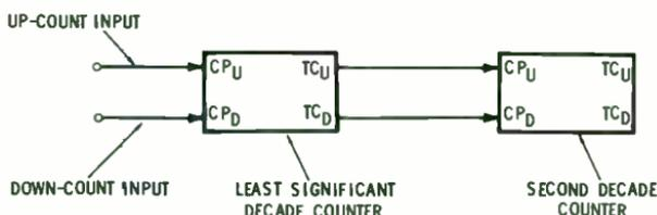
Fig. 6-19. Decade counters in tandem operation.
