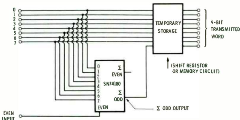
Fig. 8-4. Circuit for adding parity bit.
