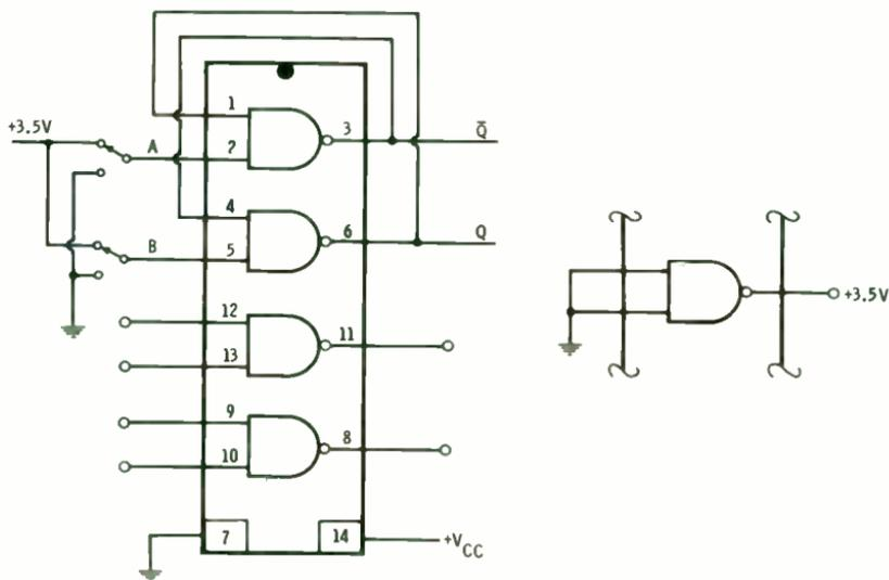
(A) Circuit using a type 7400 IC.
