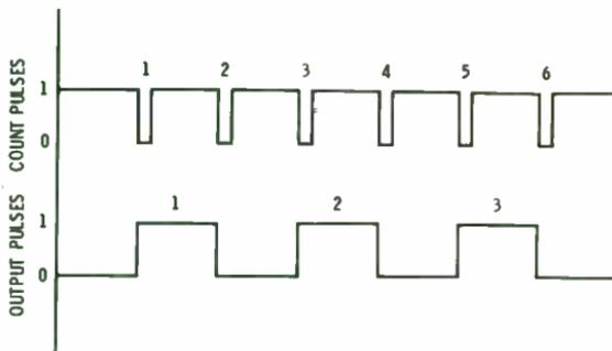
(C) Input/output waveforms.
