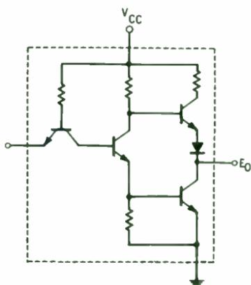
Fig. 1-7. One-input NAND gate inverter.
