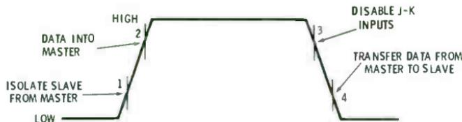
Fig. 2-18. Clock waveform for Fig. 2-16.
