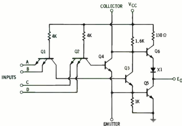
Fig. 1-12. An expandable 2-wide 2-input AND-OR-Invert gate.
