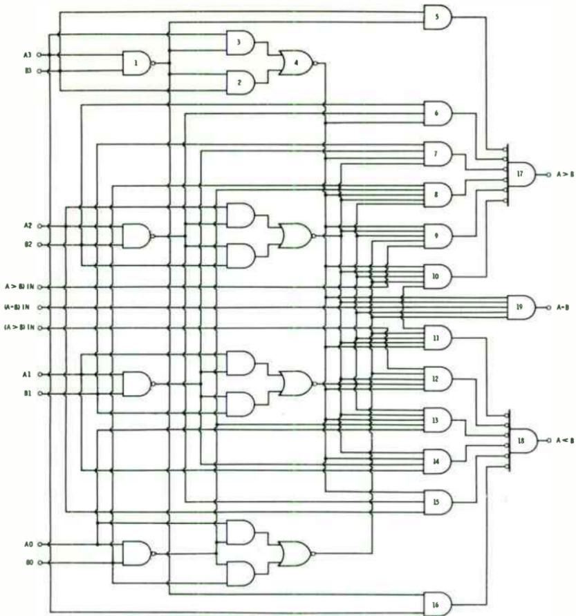
Fig. 7-9. Four-bit magnitude comparator.
