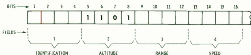
Fig. 9-9. Possible organization of a digital word for an aircraft monitoring system.
