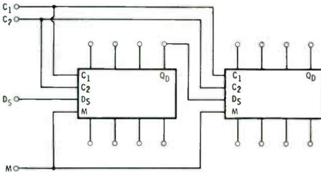
Fig. 5-7. Registers connected to provide expanded output.
