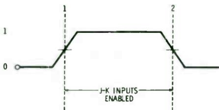
Fig. 2-24. Clock waveform for Fig. 2-22.
