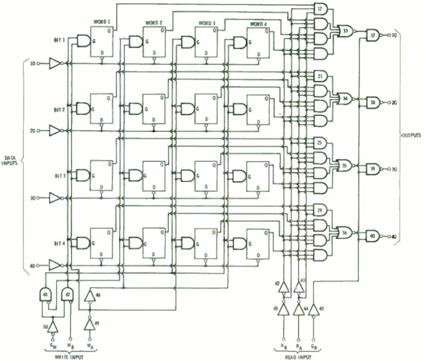
Fig. 9-5. Functional block diagram for a Register File.
