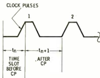
(D) Clock pulse waveform.
