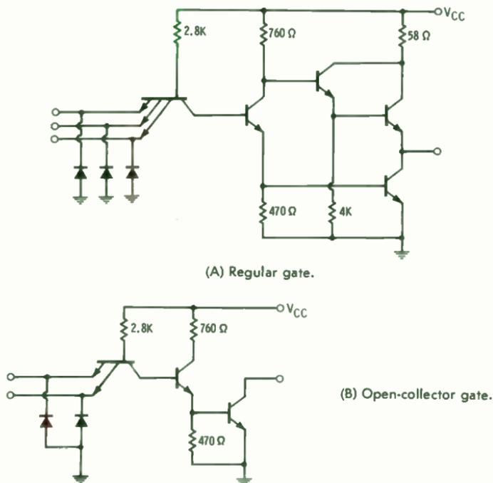
Fig. 11-2. High-speed TTL NAND gate.
