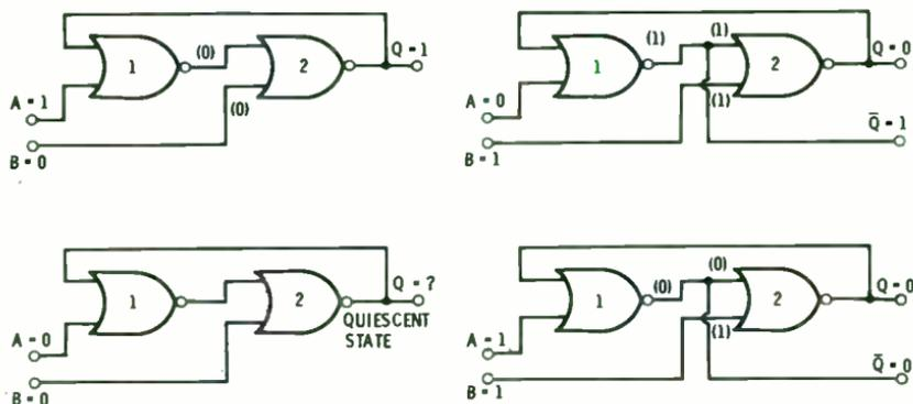
Fig. 2-6. Different input/output conditions for Fig. 2-5A.
