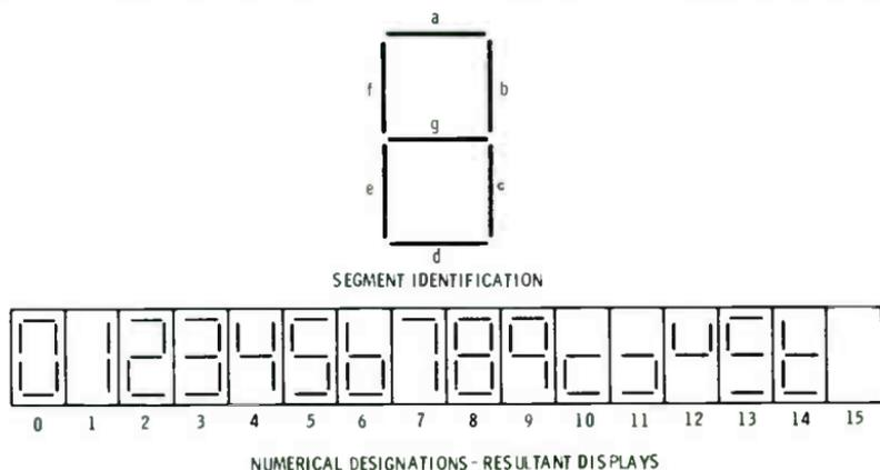
Fig. 3-10. Seven-segment indicator tube.
