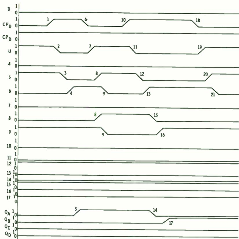
Fig. 6-14. Waveforms showing operational sequence of gates in Fig. 6-12.
