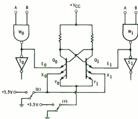
Fig. 9-2. Schematic of a storage flip-flop.
