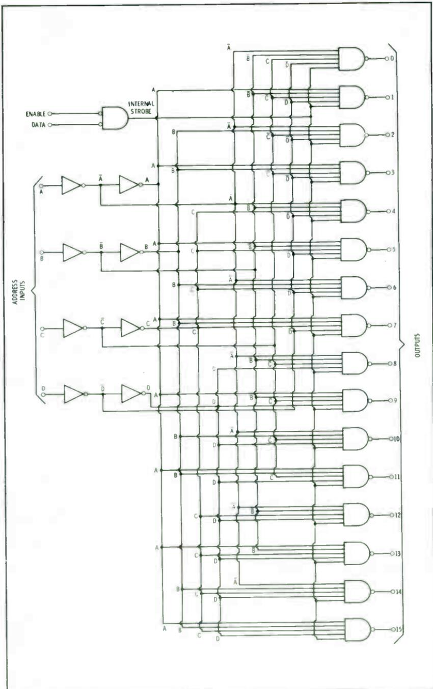
Fig. 12-3. Decoder/demultiplexer logic diagram (type SN74154).
