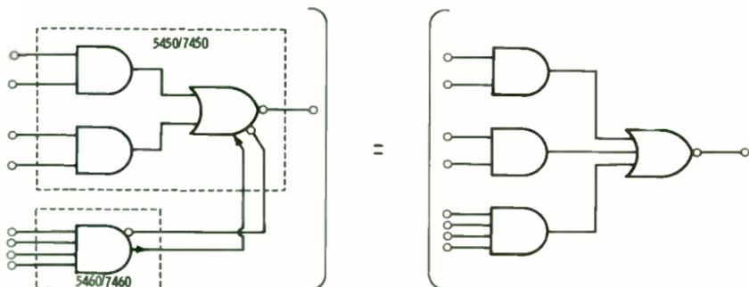
Fig. 1-15. Diagram for expandable gate with expander.
