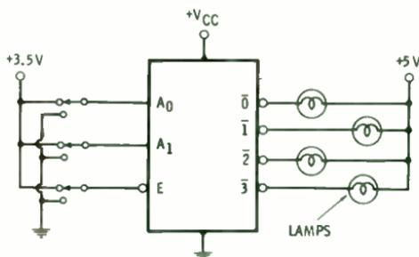
Fig. 3-4. Typical decoder circuit configuration.
