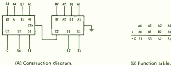
Fig. 7-5. Four-bit addition using two 2-bit adders.
