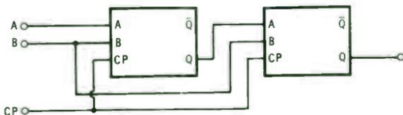
Fig. 5-2. Using two ICs in tandem operation.
