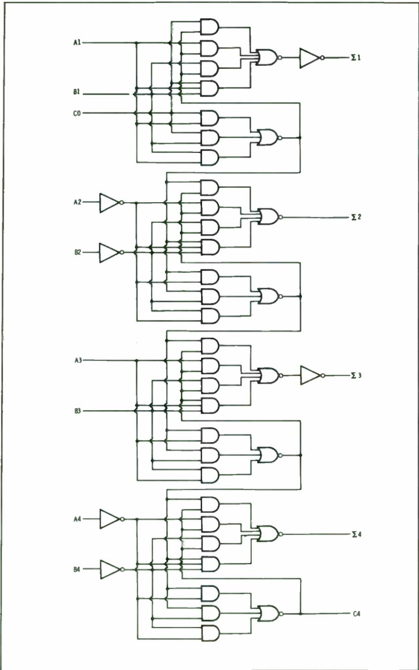
Fig. 7-6. Four-bit adder logic diagram.
