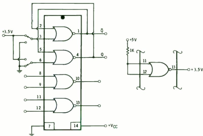
(A) Circuit using a type 7402 IC.
