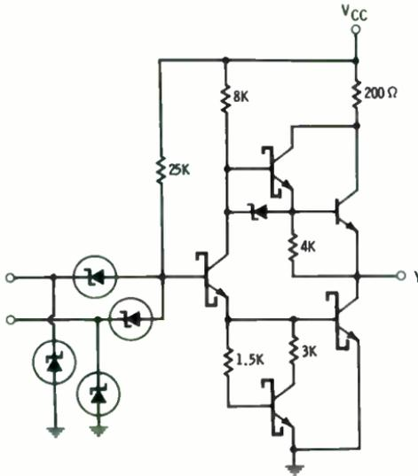
Fig. 11-8. Low-power Schottky TTL gate with totem pole output.
