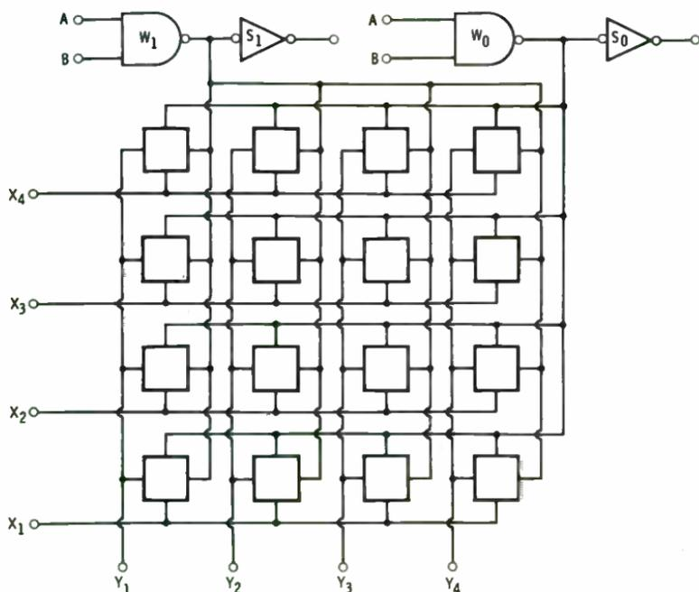
Fig. 9-3. Typical connection diagram of a RAM.
