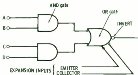
Fig. 1-13. Block diagram for an expandable gate.
