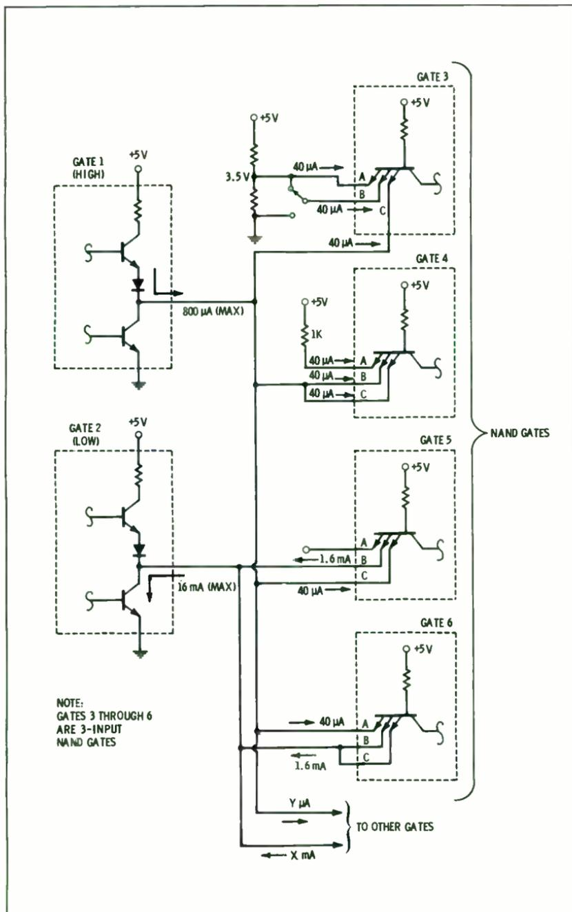
Fig. 1-16. Gate-to-gate loading conditions.
