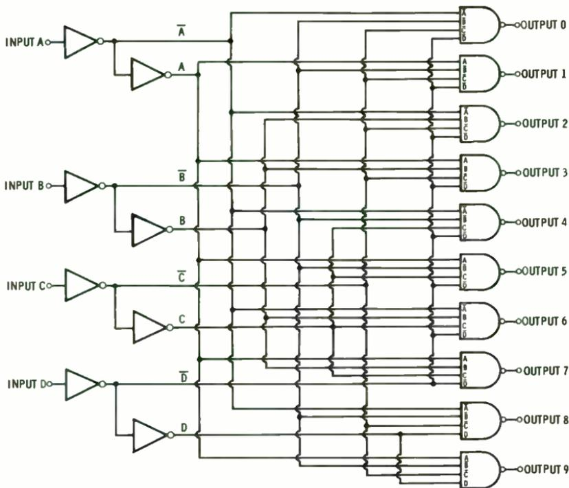
Fig. 3-5. Functional block diagram for a BCD-to-decimal decoder.
