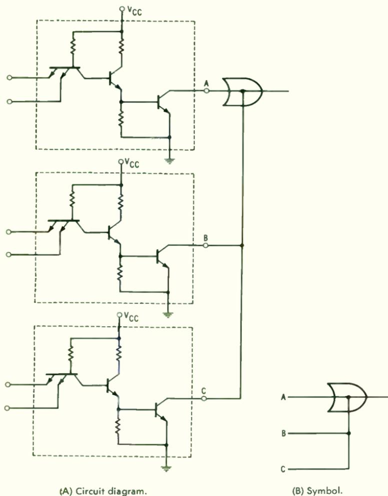
Fig. 1-10. A wired-OR circuit.
