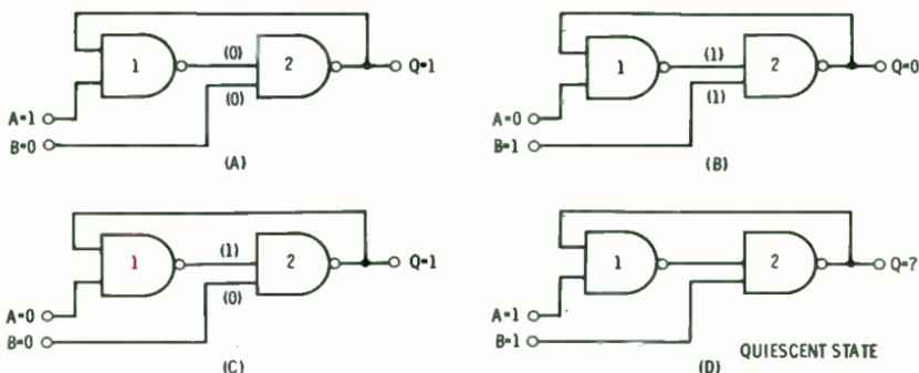
Fig. 2-2. Different input/output conditions for Fig. 2-1A.
