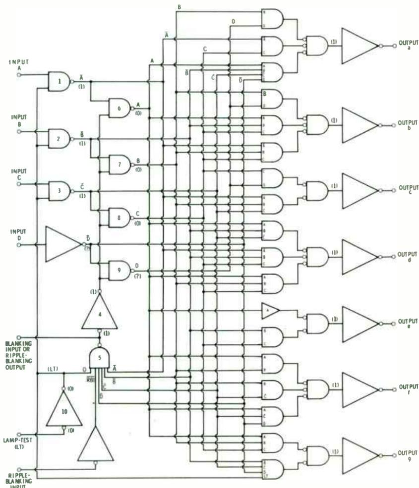
Fig. 3-14. Block diagram of circuitry having provision to test for indicator lamp failure.
