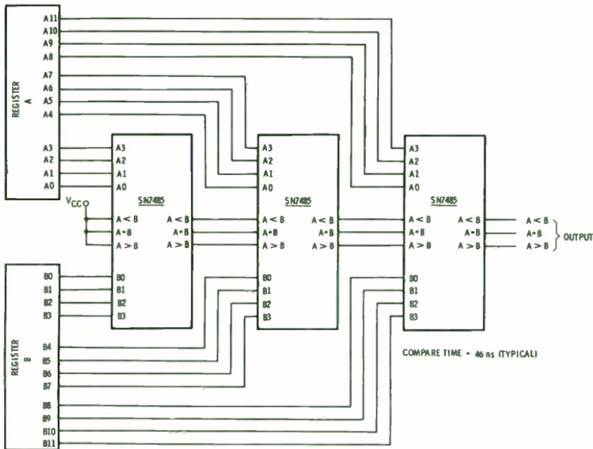
Fig. 7-11. Cascaded comparators.
