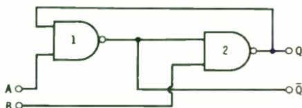
Fig. 2-3. Negative output— $\bar{Q}$ .
