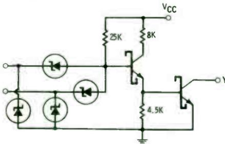
Fig. 11-9. Low-power Schottky TTL gate with open-collector output.
