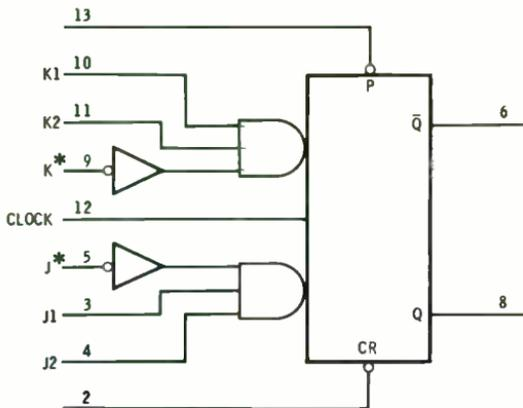
Fig. 2-21. Edge-triggered J-K Master-Slave flip-flop with inverted inputs.
