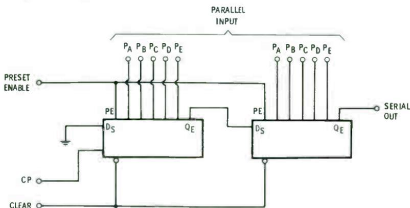
Fig. 5-4. Shift registers connected for tandem operation.
