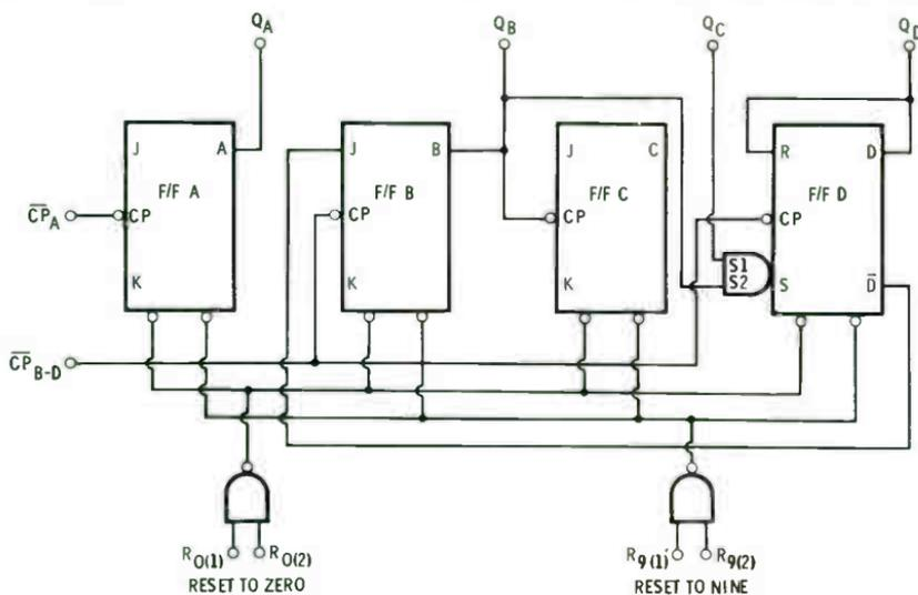
Fig. 6-8. Block diagram for a decade counter.
