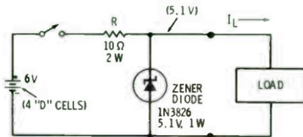
Fig. C-1. Schematic of 5-volt power supply for TTL circuits.
