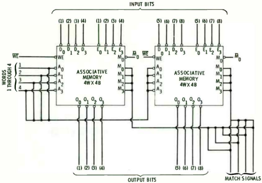
Fig. 9-13. Diagram for expanding bit length.
