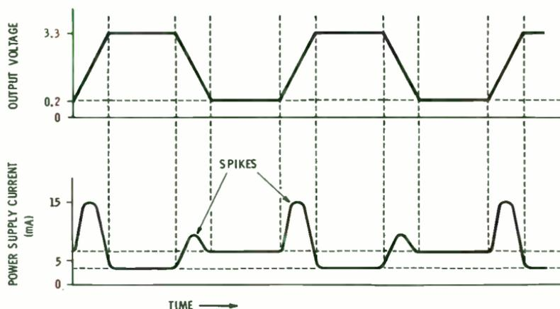
Fig. 1-3. Gate current spikes during changes of gate output.
