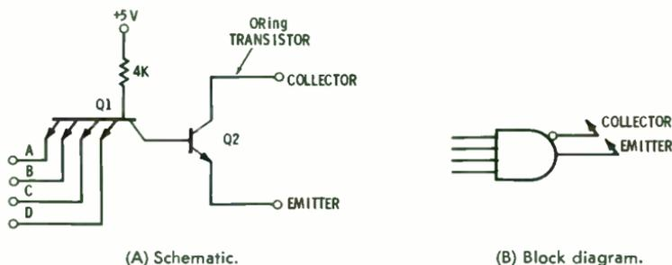
Fig. 1-14. Four-input expander.
