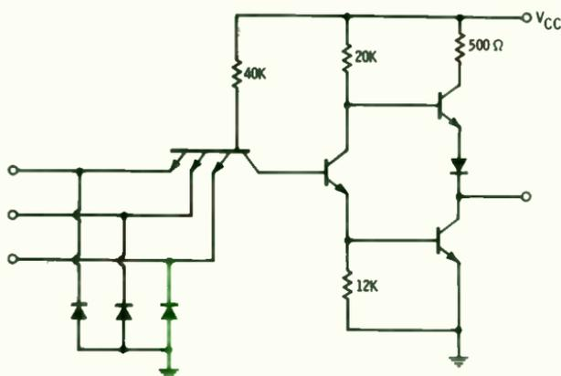
Fig. 11-4. Low-power TTL NAND gate.
