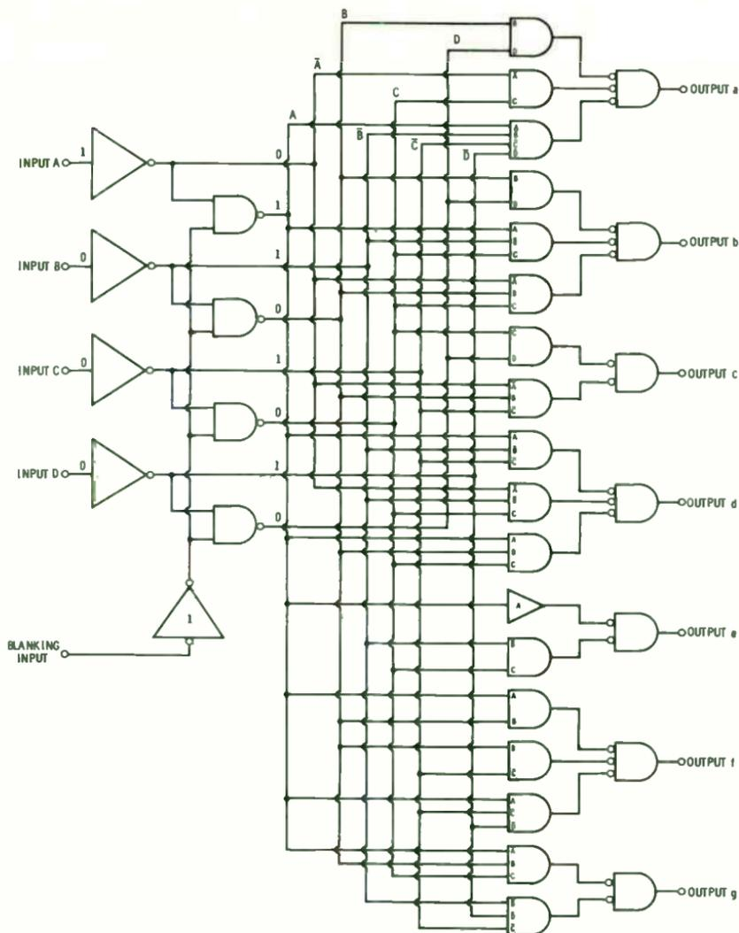
Fig. 3-11. Block diagram for typical IC used to drive indicator tubes.
