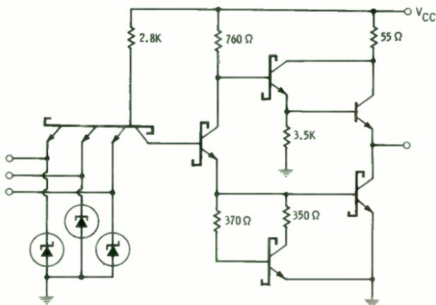
Fig. 11-7. Schottky-clamped TTL gate.
