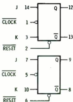
Fig. 2-19. Block symbol for SN5473/SN7473.
