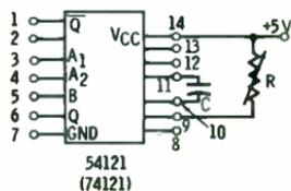
(B) Addition of R-C timing circuit.
