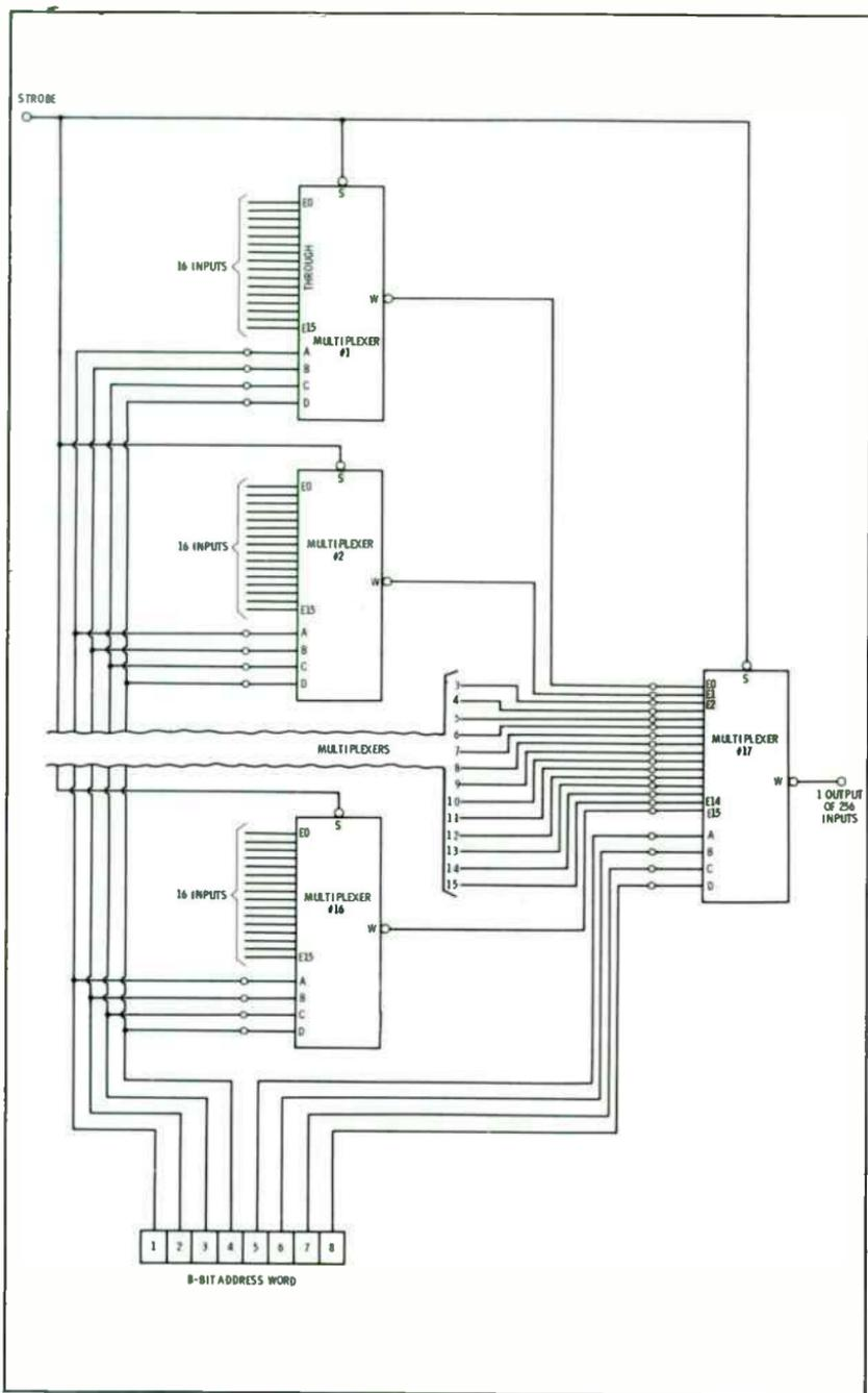
Fig. 4-2. Using multiple devices to increase input capability.
