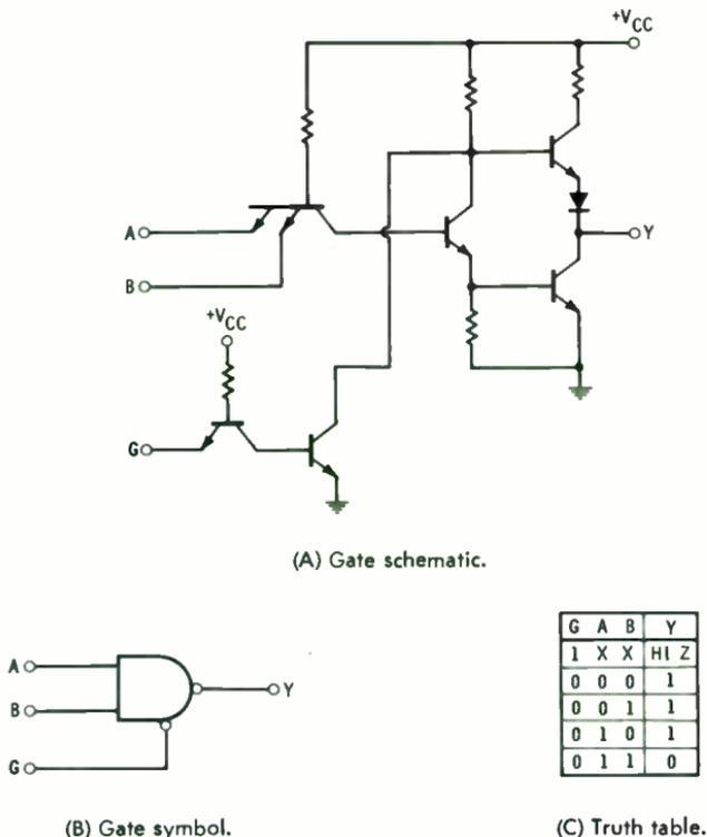
Fig. 11-10. Tri-State logic gate.
