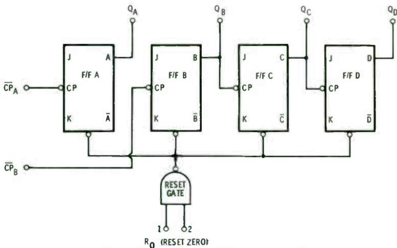
Fig. 6-1. Block diagram for a 4-bit binary counter.
