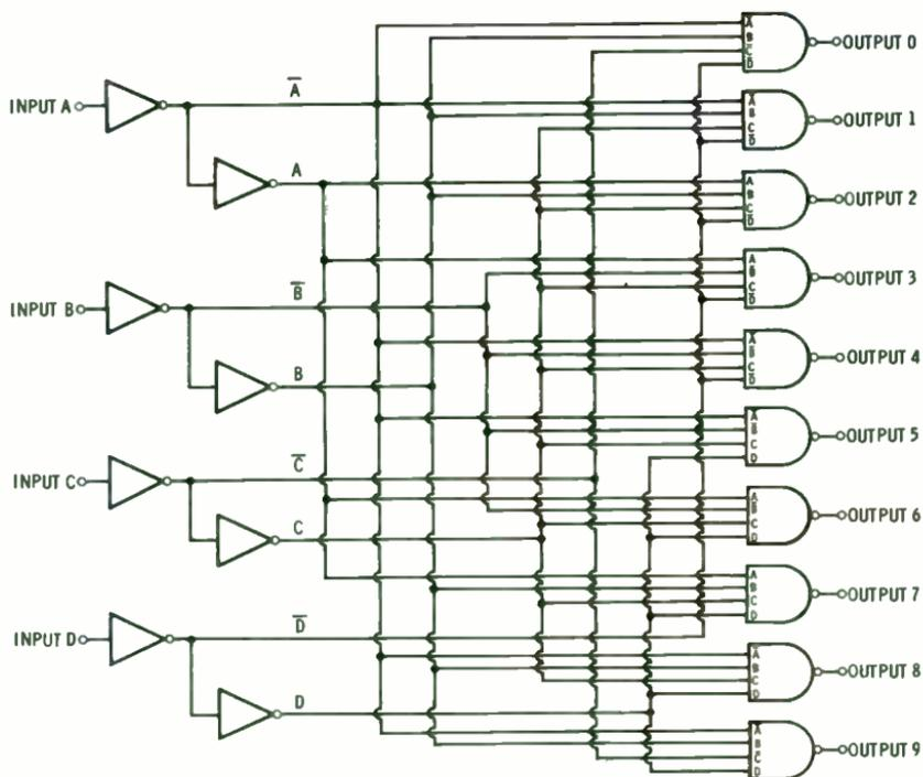
Fig. 3-7. Excess-3-Gray-to-decimal decoder functional block diagram.
