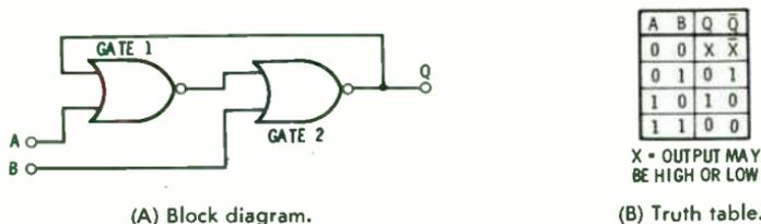
Fig. 2-5. A NOR-gate flip-flop.
