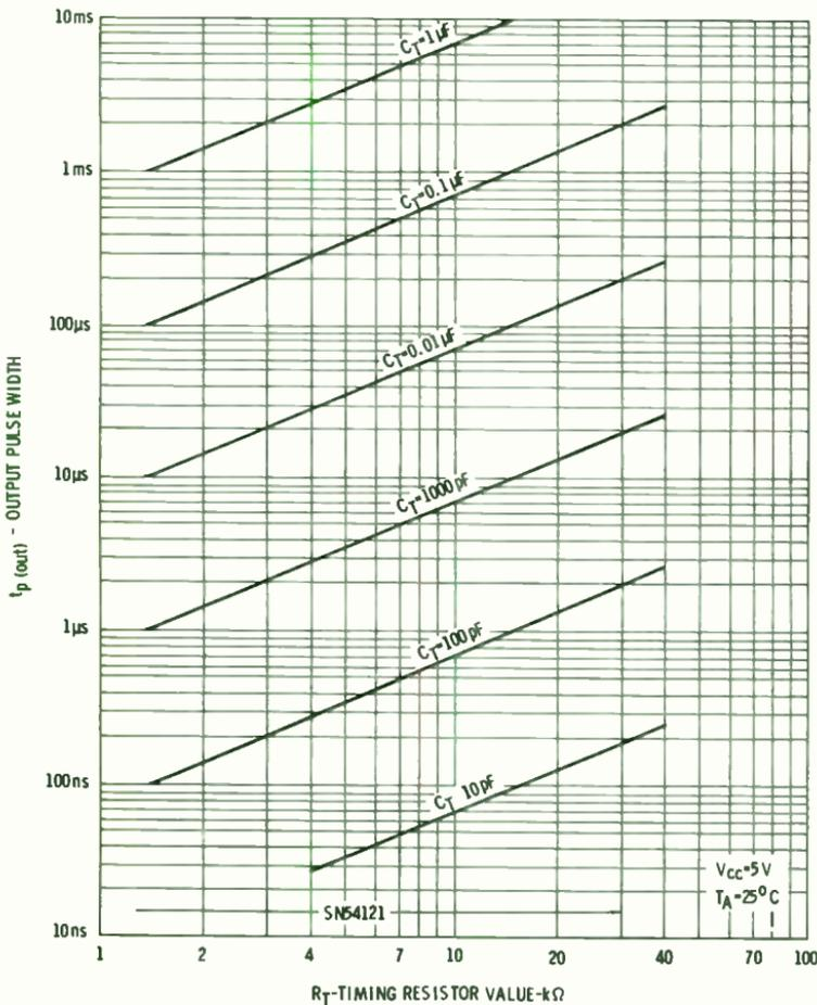
Fig. 10-3. Typical characteristics.
