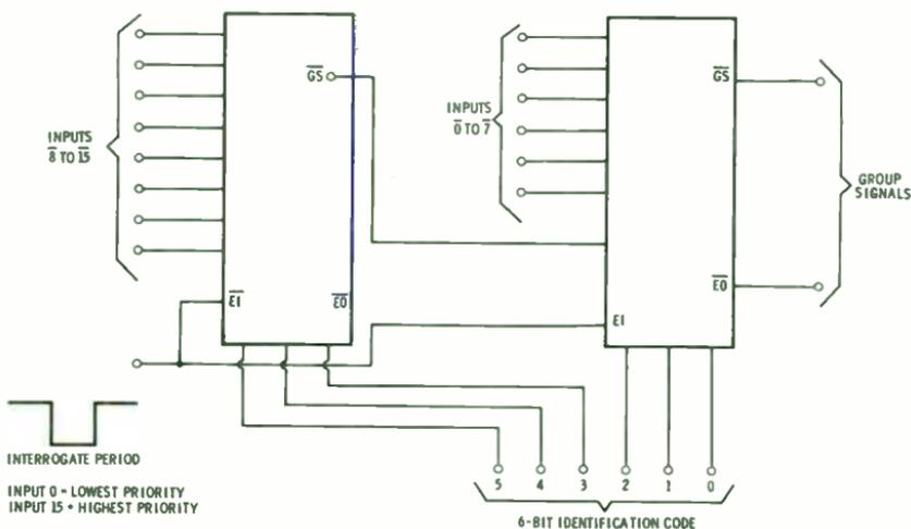
Fig. 8-7. Diagram for expanded encoder operation.
