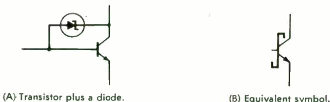
Fig. 11-6. Schottky-barrier diode-clamped transistor.
