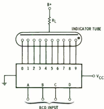
Fig. 3-9. Block symbol for a BCD decoder with direct-drive capability.
