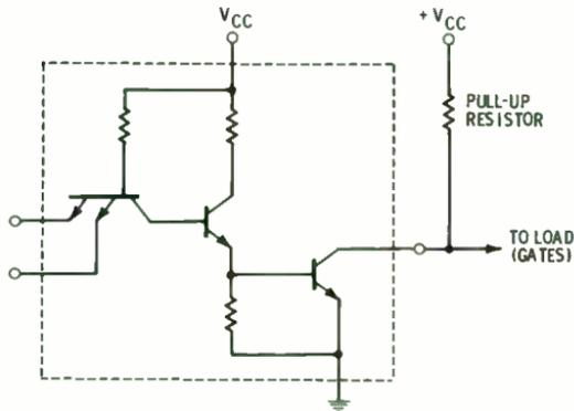
Fig. 1-11. Open-collector gate with pull-up resistor.
