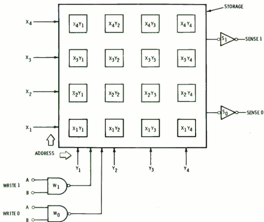
Fig. 9-1. RAM storage arrangement diagram.
