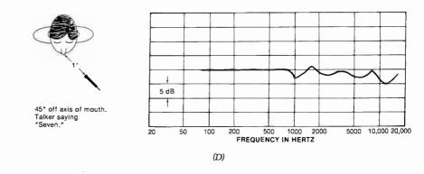
(Fig. B-12B and C). Thus, a flat-response omnidirectional microphone placed close to the mouth produces only minor coloration.
