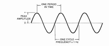
Fig. 1-5. Graph of waveform showing amplitude vs. time.
