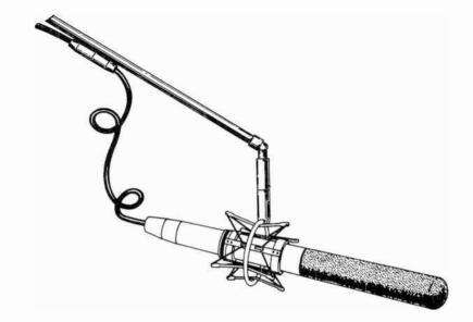
Fig. 9-17. Short, flexible cable helps isolate the microphone from noises and vibration.
