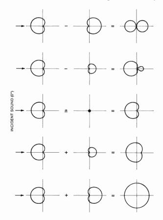
Fig. 3-8. Variety of polar patterns that may result from combining the output of two cardioids back to back. polarizing voltages, making a continuous mixture possible between pressure and pressure-gradient polar-response characteristics.
