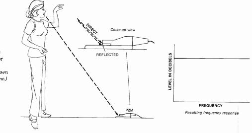
Fig. 6-19. Pressure Zone Microphone or PZM system. (Courtesy of Crown International, Inc.)
