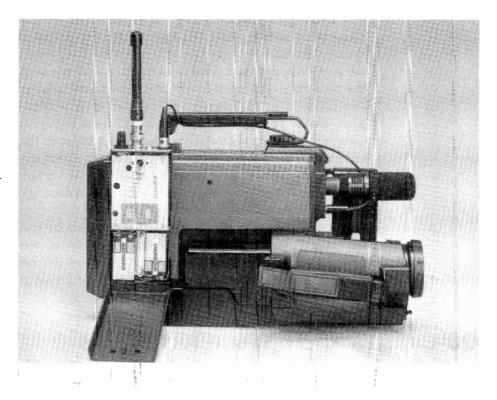
Fig. 9-11. Magnavox portacam/Swintek Mark QOC combination. (Courtesy of Swintek Relecommunications Division)
