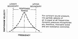
Fig. 2-2. Frequency responses for typical dynamic microphone.
