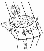
of feedback. This method often produces a brittle or mid-range-heavy tone that may improve with experimentation with microphone placement and equalization.
