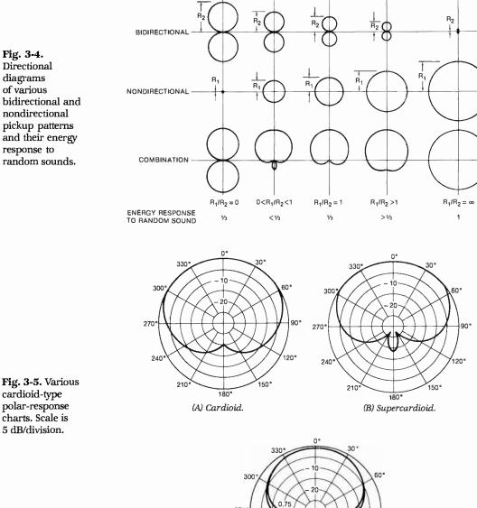
Fig. 3-5. Various cardioid-type polar-response charts. Scale is 5 dB/division.
