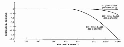
Fig. 4-1. Effect of various cable lengths upon frequency response (cable capacitance: 22 pF/foot).
