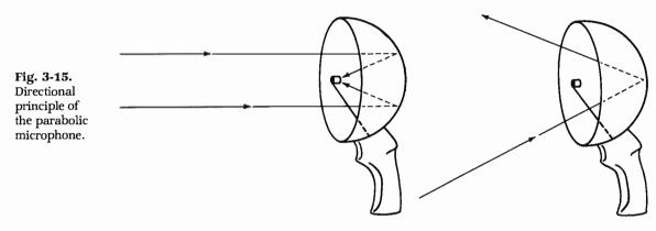
(A) On-axis signals are focused at the microphone.
