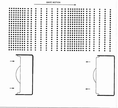
Fig. 1-6. Diaphragm displacement with sound motion.
