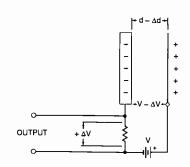
Fig. 2-12. As a sound wave decreases a condenser element's spacing by  $\Delta d$ , the capacitance increases by  $\Delta C$ . Conversely, the voltage across the plates falls by  $\Delta V$ .
