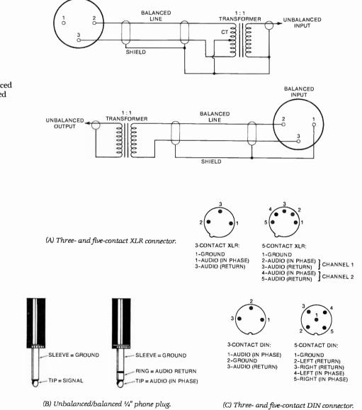
Fig. 4-5. Transformer connections between balanced and unbalanced equipment.
