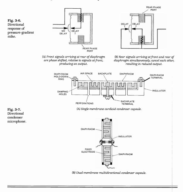
diaphragm) is created by admitting some acoustic energy to the rear of the diaphragm. This is accomplished by drilling perforations completely through the backplate beside the damping holes. These perforations are designed as an acoustic labyrinth such that any sound wave that impinges directly on the rear of the diaphragm will be 180° out of phase with respect to sound waves at the front of the diaphragm plate.
