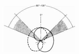
The hypercardioid X/Y pair is similar to the cardioid pair, except the included angle is typically narrower in order to preserve a solid center image (Fig. 7-10). The increased reach of the hypercardioid allows a more distant placement for a given direct-to-reverberant sound ratio. With their small reverse-polarity lobes, the hypercardioid pair is often a good compromise between the cardioid and the Blumlein X/Y technique.
