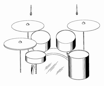
Fig. 8-19. Typical stereo overhead mike positioning.
