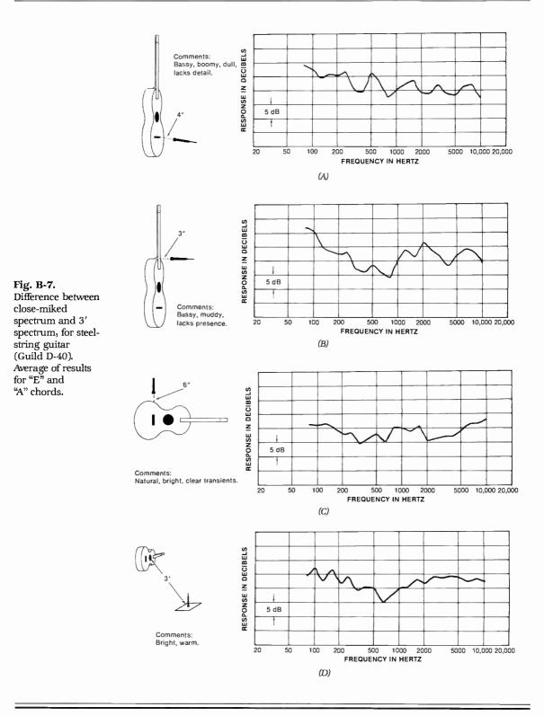
and lacking in presence—perhaps due to low-frequency masking of higher frequencies. With another guitar, the presence range may well be audible.
