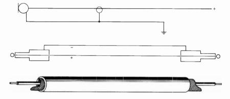
Fig. 4-3. Unbalanced microphone circuit.
