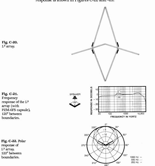
October 1983. The frequency response is shown in Figure C-21 and the polar response is shown in Figures C-22 and -23.
