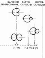
sound source than an omnidirectional microphone while maintaining an equivalent direct-to-reverberant ratio and/or feedback threshold. For example, a cardioid microphone can be placed at a distance 1.7 times that of an equivalent omnidirectional microphone and maintain the same ratio of direct-to-reverberant pickup.
