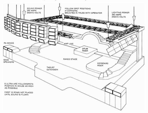
Fig. 10-6. Typical large-scale reinforcement system.
