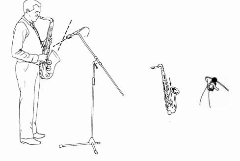
**Fig. 8-7.** Typical mike positioning for saxophone.
