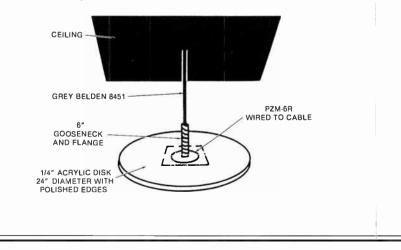
Fig. C-4. Circular boundary to be hung over choir sections.
