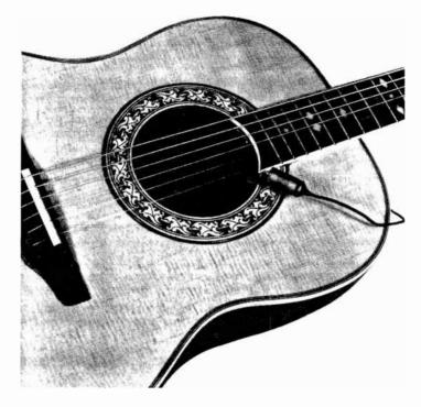
Fig. B-6. Clip microphone near guitar's sound hole.
