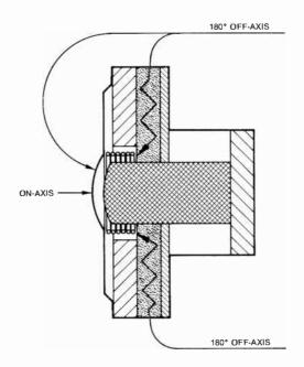
Fig. 2-3. Frequency response of a moving-coil microphone: (1) damped resonance of the vibrating system (2, 3, 4) resonance of additional air pockets.
