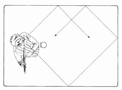
Although close miking offers several advantages, a microphone should be placed only as close to the source as is necessary, not as close as is possible.
