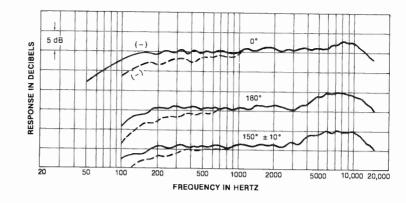
dioid microphone that displays a strong peak within its operating range may receive too much energy at that peak frequency from the off-axis stage monitors or audience loudspeakers. This might cause feedback at that frequency.
