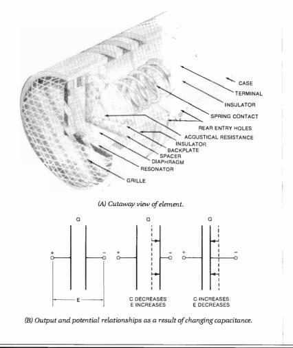
Fig. 2-10. Details of a condenser capsule. (Courtesy of Shure Brothers, Inc.)
