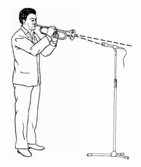
**Fig. 8-4.** Typical mike positioning for single trumpet.
