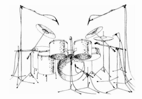
Fig. A-3. Drum set miked with carefully placed array of omnidirectional microphones.
