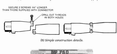
(C) Commercially available microphone line attenuator.
