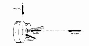
The Effects of Boundary Interference at Close Distances As with distant microphone techniques, the effects of phase cancellations as a result of reflections from nearby boundaries may affect the quality of a signal pickup at close working distances.
