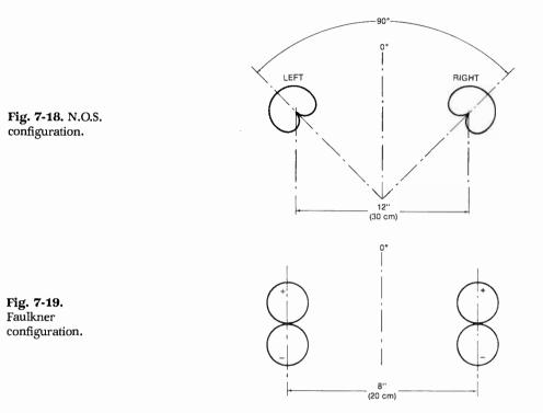
time (phase) differences resulting from the spacing between the microphones. Additionally, Faulkner recommends that the microphone pair be placed further back from the sound source than is common with other coincident techniques; this provides a more natural balance between the direct and reverberant sounds.
