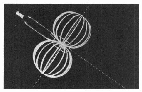
Fig. 3-3. Bidirectional microphone. (Courtesy of Sennheiser Electronic Corporation (N.Y.))
