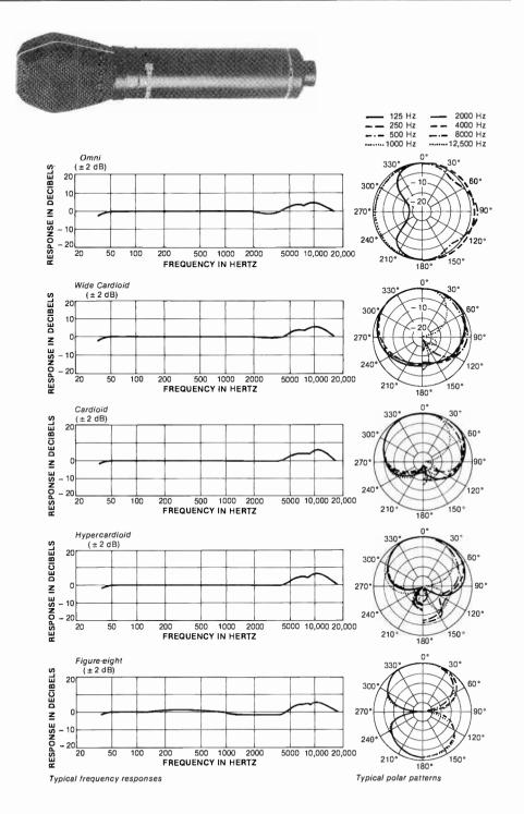
Fig. D-16. Beyer Dynamic MC 740 N(C) P48. (Courtesy of Beyer Dynamic, Inc.)
