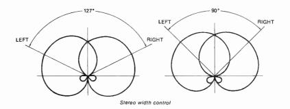
Fig. 9-3. The Sanken CMS-7 MS stereo microphone. (Courtesy of Sanken/Pan Communications, Inc.)
