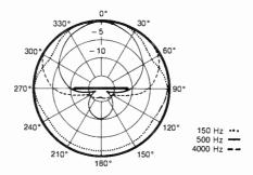
With multiple boundaries, the shape of the pickup pattern approximates the shape of the boundary assembly. For example, a V-shaped boundary produces a polar pattern with a lobe whose sides are defined by the sides of the "V." Note, however, that the polar pattern varies with frequency.
