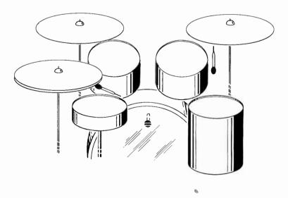
Fig. 8-45. Drums miked with three microphones. (Courtesy of Crown International, Inc.)
