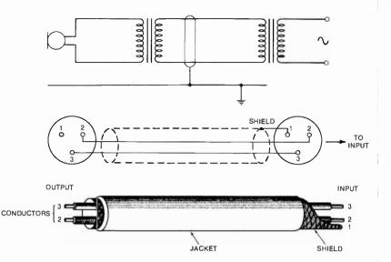
Fig. 4-4. The balanced microphone circuit.
