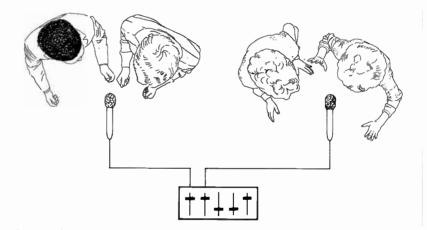
When individual control is necessary or if feedback is a problem, each individual sound source may be given its own microphone (Fig. 8-3). If the ensemble is out of balance at the time of recording, this approach enables a proper balance to be restored in the mixdown phase.
