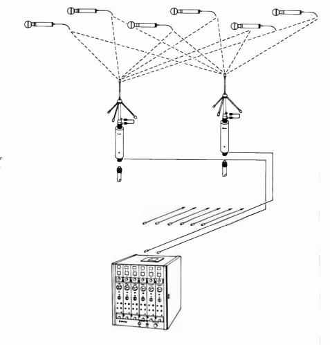
Fig. 9-10. Sony UHF 6-channel diversity reception system. (Courtesy of Sony Corporation of America)
