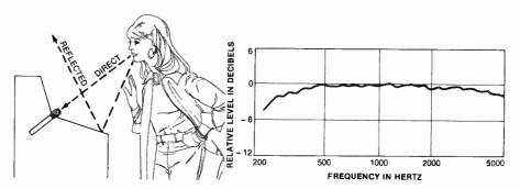
(B) Effects of flush-mounted pickup.
