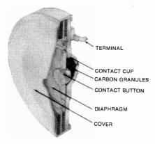
Fig. 2-20. Carbon microphone. (Courtesy of Shure Brothers, Inc.)
