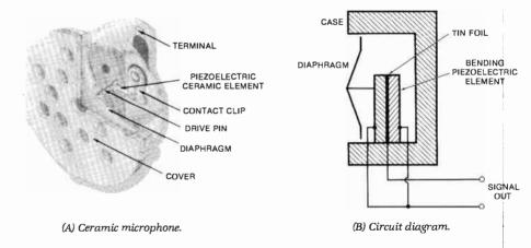
Prior to 1960, Rochelle salt crystals were used as the generating element, but these proved to be unstable with changes in humidity or heat. Since this time, they have been replaced by newer ceramic materials that are more sistant to environmental extremes.
