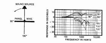
Below 94 Hz, the response is a constant 6 dB below the upper midfrequency level. Note that there is a response shelf, not a roll-off.
