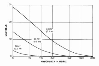
To compensate for this effect, a low-frequency roll-off filter is often provided to restore the bass response to a flat and natural sounding balance. This filter is most often a selective switch located on the body of the microphone (Fig. 3-21).
