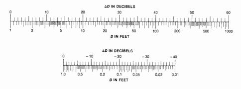
Fig. 10-1. Inversesquare graph showing changes in decibel level  $\Delta D$ over distance D.
