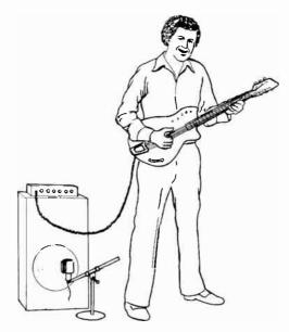
Fig. 8-34. Typical microphone placement for bass guitar.
