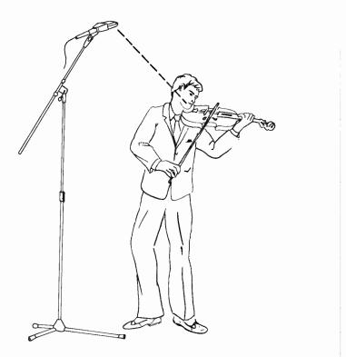
**Fig. 8-23.** Typical pickup placement of violin.
