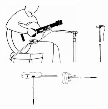
Fig. B-1. Various microphone positions for acoustic guitar.
