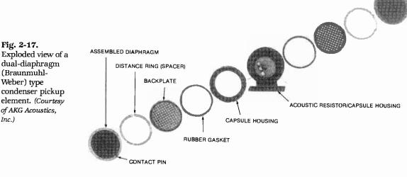
Basically, this system consists of the equivalent of two back-to-back cardioid capsules (Fig. 2-18A), with each diaphragm acting as part of a pressure-gradient capsule. The opposing diaphragms, in combination with the phase-shift port holes, combine to create an effective 180° phase shift relative to the on-axis angle, producing a dual-cardioid system within a single housing. This gives the user a choice of several polar patterns (Fig. 2-18B),
