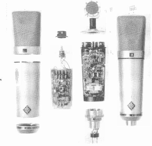
Fig. 2-9. Detail of the Neumann U-89 condenser microphone. (Courtesy of Gotham Audio Corporation)
