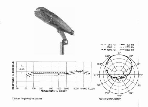
Fig. D-6. Sennheiser MD 421. (Courtesy of Sennheiser Electronic Corporation [N.Y.])
