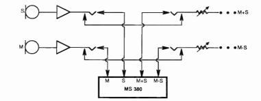
Fig. 7-15. MS-38 active M/S Matrix patch loop.
