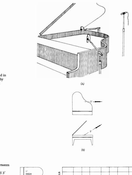
Fig. B-9. Microphone positions used in pickup of baby grand piano.
