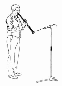
Playing technique affects the harmonic content of the instrument, which generally runs up to 8 kHz and is extended by breath noises that take the range to a peak between 12 to 13 kHz.
