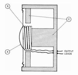
Fig. 2-1. Movingcoil microphone.
