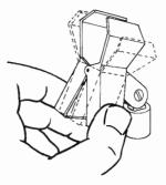
The dual microphone mount (Fig. 5-13) can be used to place two microphones on one stand or mount to ensure reliable coverage of a speech or multimedia event. Such mounts are also available for use with the lavaliere-type tie-clip microphone.
