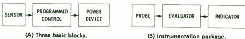
**Fig. 9-1. Basic control and instrumentation functions.**
