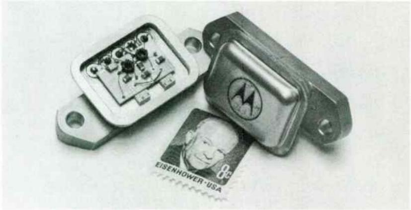
(A) IC showing external toroid coils.
