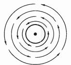
Fig. 9-5. The magnetic lines of force form in a counterclockwise direction around a conductor when the current is moving toward the observer.
