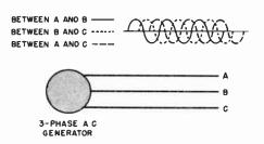
Fig. 11-50. A three-phase generator cannected to three line wires. The valtage and current will rise and fall in the three line wires in time relation to each other as shown. intensity at the same time.
