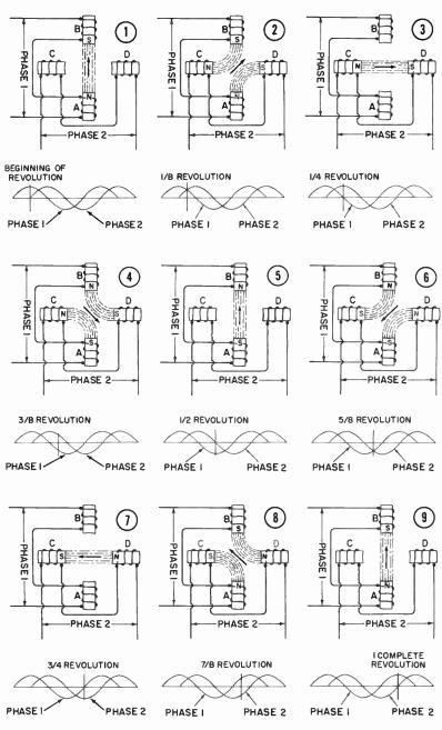
Fig. 13-9. Showing how a two phose current con produce o rotating mognetic field.
