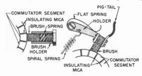
Fig. 12-23. How the brushes rest on the commutator. The brushes are held firmly against the commutator by spring tension. The individual segments of the commutator are separated from each other by insulating mica.
