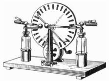
Fig. 3-15. A Wimshurst induction static machine. 3-15, may be purchased from physics apparatus firms. They give a high electric potential, and a constant stream of sparks jump the air gap between terminal knobs. Such a machine is much better than the electrophorus for lecture table demonstrations and for charging Leyden jars and capacitors.
