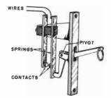
Fig. 14-5. A switch which could be used with a pull cord.
