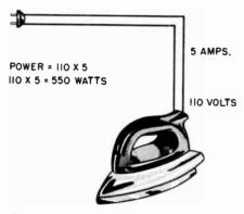
Fig. 10-10. How to figure the power used by an iron when the voltage and current are known.
