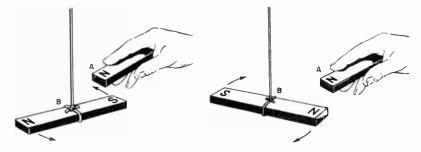
Fig. 8-4. The north pole of one magnet will attract the south pole of another magnet.
