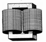
Fig. 11-21. How the coils are placed on a care-type transformer.
