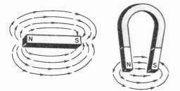
Fig. 8-10. The lines of force seem to travel in curved lines.
