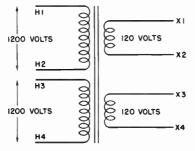
Fig. 11-43. A transformer with two high-voltage and two low-voltage windings.
