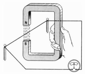
Fig. 11-27. Moving the magnet while the conductor is stationary will also induce a voltage within the conductor.
