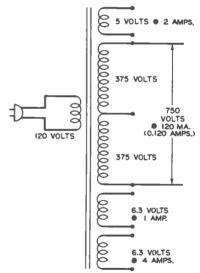
Fig. 11-53. Diagram of a typical radio power supply transformer showing primary and secondary windings.
