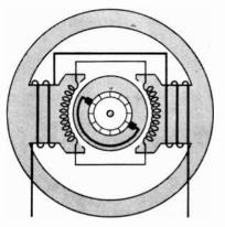
Fig. 13-27. The armature will rotate when the brushes are in this position.
