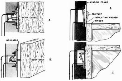
Fig. 14-12. A plunger-type door Fig. 14-13. A switch for use on winswitch. dows in an alarm system.
