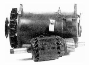
Fig. 12-28. An automobile generator. This is a common type of DC generator.
