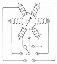
Fig. 13-7. A simple method to show how a rotating magnetic field can be produced.
