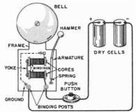
Fig. 14-18. Wiring details of a singlestroke bell.
