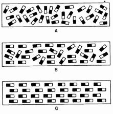
Fig. 8-18. How the molecules line up under the influence of magnetism.
