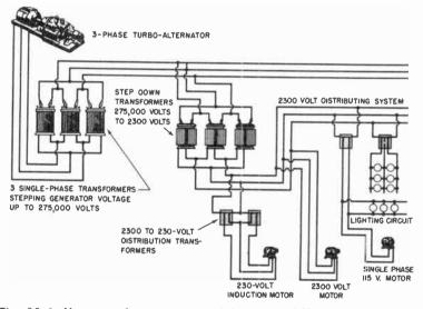
Fig. 11-4. How transformers are used for many different purposes in a transmission and a distribution system.
