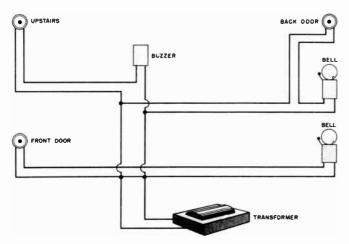
Fig. 14-23. A typical door bell signal system used in a better home.
