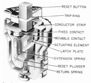
Fig. 5-17. A cross-sectional view of a mini-breaker shawing its internal construction. (Caurtesy of Mechanical Products Inc.)
