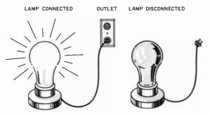
Fig. 4-3. A complete metollic path must be provided for the passage of electricity.
