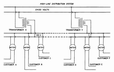
Fig. 11-41. How two tronsformers can be connected to supply power to a group of customers.
