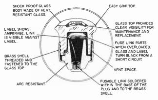
Fig. 5-1. Cross-sectional view of a fuse plug showing its various parts.
