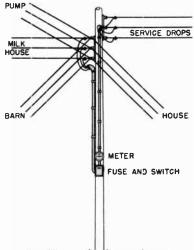
Fig. 15-5. The main fuse and main switch are often located on the meter pole.
