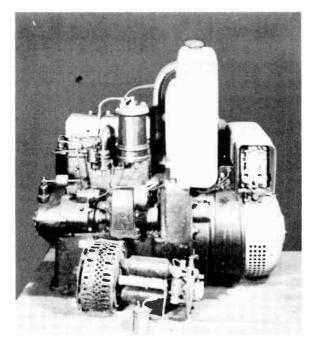
Fig. 13-1. A 110 volt alternator of the type that is sometimes used on farms.
