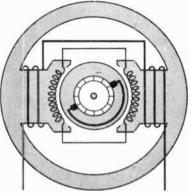
Fig. 13-28. When the brushes are in this position, the armature will rotate in the opposite direction to that of Fig. 13-27.
