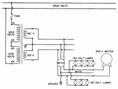
Fig. 11-47. The manner in which this type of transformer is most often used.
