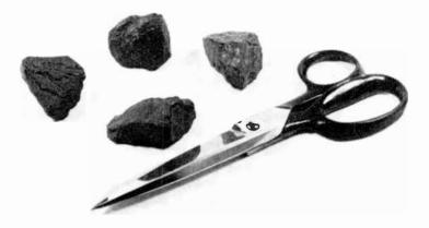
Fig. 8-1. Lodestones, the original natural magnets.
