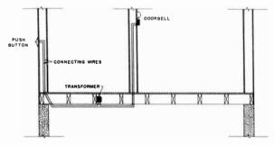
Fig. 14-3. How the wires are run to connect a door bell with its push-button control.
