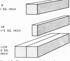
Fig. 6-2. The resistance is inversely proportional to the cross-section area of the conductor.
