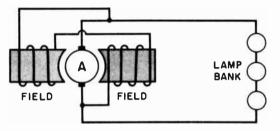
Fig. 12-26. Electrical circuits in a shunt generator. The field cails here are connected directly to the full autput voltage of the generator.
