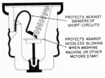
Fig. 5-4. Interiar cross-sectian view of a Fusetron fuse. (Caurtesy af Bussmann Mfg. Company.)
