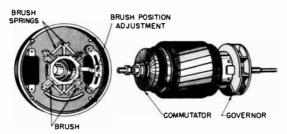
Fig. 13-30. The cammutator of a repulsion-induction matar with the brushes and brush shifting mechanism.
