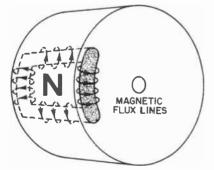
Fig. 13-13. How a current, induced in a short-circuited inductor of a squirrel cage rotor produces a magnetic field about itself.
