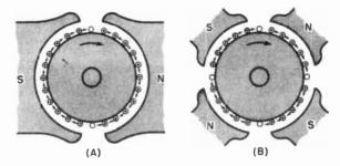
Fig. 12-20. Armatures used with a two-pole magnetic field and a four-pole magnetic field. The north and south poles of the magnets alternate around the armature.
