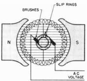
Fig. 13-2. How slip rings are used to pick up the current from a two-pole alternator.
