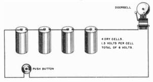
Fig. 14-1. A simple signal circuit powered from dry-cell battery.
