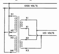
Fig. 11-4S. Both primary windings and both secondary windings connected in parallel.
