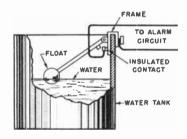
Fig. 14-15. A "Float" switch for controlling the level of water in a tank.
