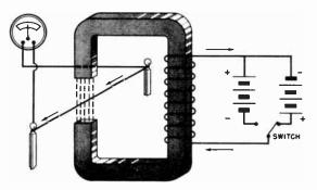
Fig. 11-29. If the current through the coil is reversed, the voltage induced in the wire in the gap will be reversed.
