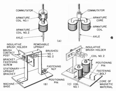
Fig. 12-2. Parts or components of an experimental direct-current generator.
