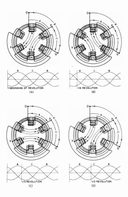
Fig. 13-16. How the rotating magnetic field shifts
