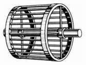
Fig. 13-10. An elementary squirrel cage rotor.
