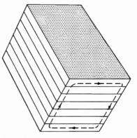
Fig. 11-8. Slicing (laminating) a steel core into thin sections (sheets) reduces the eddy currents materially.
