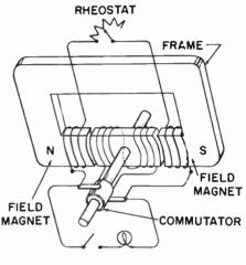
Fig. 12-7. Self-excited shunt-wound DC generator.
