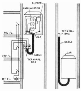
Fig. 14-33. How an annunciator system would operate in an elevator.
