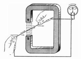
Fig. 11-25. Moving a conductor across magnetic lines of force at right angles to them induces a voltage in the conductor.
