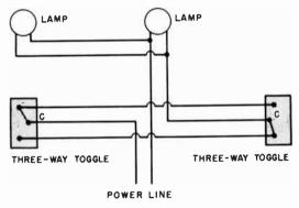
Fig. 14-36. How two three-way toggle switches can be used to control two lamps from two different positions.
