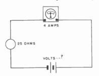
Fig. 7-2. When the current and the resistance in a series circuit are known, it is a simple matter to figure the voltage.
