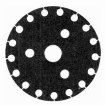
Fig. 13-11. A rotor punching for use in the rotor of an induction motor.
