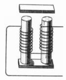
Fig. 14-16. Basic construction of an electromagnet.
