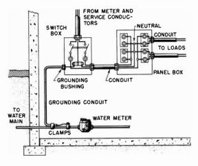
Fig. 15-21. A practical method of grounding an electrical system.
