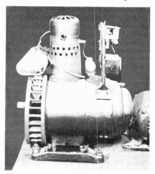
Fig. 12-29. A 32-volt electric generating plant intended for home use in remote areas where commercial power is not available.
