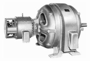
Fig. 4-21. Two generators mounted on the same shaft. The small generator supplies the exciting current for the fields of the larger generator. (Courtesy of Allis-Chalmers Mfg. Co.)
