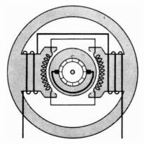
Fig. 13-26. There is no current flow through the armature (rotor) of a repulsion motor if the brushes are in the position shown.
