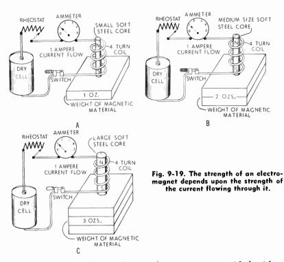
For illustration let us take an electromagnet provided with a core made of a poor grade of iron (Fig. 9-20A). Let us assume further that the magnet coil has four turns of wire for its winding with one ampere of current passing through it. Let us also assume that this electromagnet illustrated will lift a soft steel weight of just one ounce.
