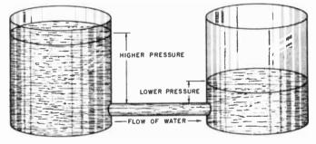
Fig. 4-17. Water will flow through the connecting pipe because of the difference in pressure at the bottom of the two tanks. This is similar to the difference of potential which often exists in electrical circuits.
