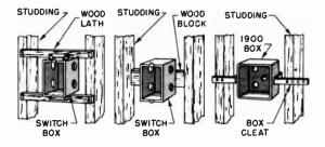
Fig. 15-36. Methods of mourting switch boxes.
