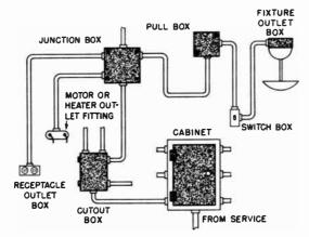
Fig. 15-24. How rigid conduit is run from one box to another in an electrical wiring system.
