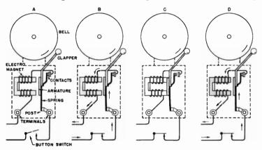
Fig. 14-17. How a vibrating bell works.
