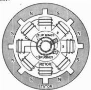
Fig. 13-18. The ratar and statar of a synchronous matar.
