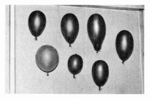
Fig. 3-2. A static charge imparted to the rubber balloons causes them to be attracted to a dry wall.
