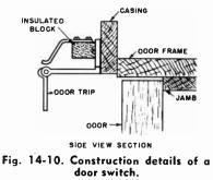
The constructional details of such switches varv widelv: however, there are two requirements that must be met by all. It is essential that the contacts of the switch do not close when the door is closed and that they make contact with each other only when the door is open. Some are designed to maintain contact
