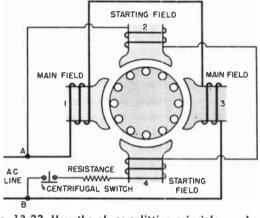
Fig. 13-22. How the phase-splitting principle can be applied to a single-phase motor.
