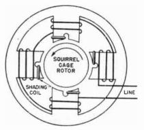
Fig. 13-31. A shaded-pole motor.
