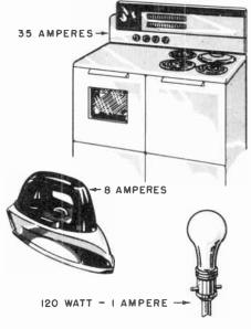
Fig. 4-11. A 120-watt lamp uses about 1 ampere of current, a pressing iron uses from about 7 amperes to about 9 amperes, and an electric range may use as much as 35 amperes.
