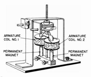
Fig. 12-4. A permanent-magnet type of experimental direct-current generator.
