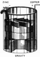
Fig. 4-18. A "crow's foot" electric cell such as was once widely used in telegraph work.
