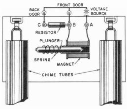
Fig. 14-20. How a door chime works.
