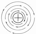
Fig. 9-7. The magnetic lines of force form in a clockwise direction when the direction of current flow is away from the observer.
