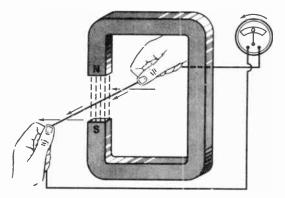
Fig. 11-26. Moving the conductor in the opposite direction induces a voltage with an opposite polarity.
