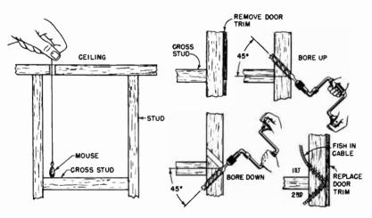
Fig. 15-30. How obstructions within o woll con be locoted. Fig. 15-31. Bypassing on obstruction without seriously morring the woll.
