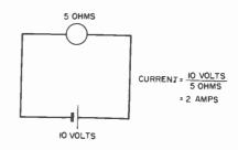
Fig. 7-1. A simple series circuit.
