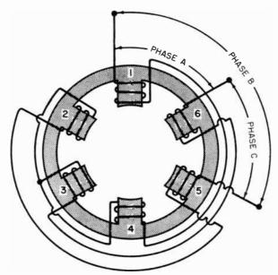
Fig. 13-14. The windings of a three-phase field, showing how the lead wires from the windings are brought out.
