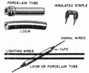
Fig. 14-22. An insulated staple, loom, and porcelain tube.
