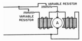
Fig. 12-31. Direct-current shunt motors can be controlled by inserting variable resistance in either the armature circuit or in the field circuit. Many shunt motors use variable resistances in both circuits to obtain even greater control than either alone can give.
