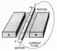
Fig. 12-11. A current will flow in the conductor when it becomes a complete circuit.
