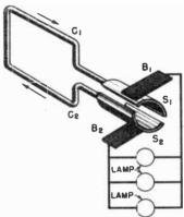
Fig. 12-15. A commutator, consisting of two or more segments, con be used to tap the current inside the rotating loop.
