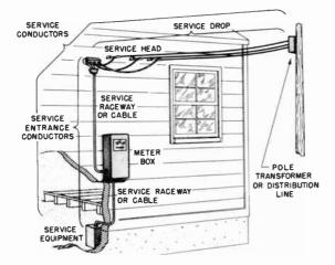
Fig. 15-2. The principal parts of an electrical service entronce.
