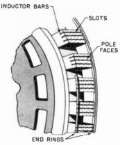
Fig. 13-19. How the squirrel-cage bars used to start the motor are imbedded in the faces of the poles on the rotor of a synchronous motor.
