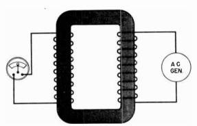
Fig. 11-30. By connecting the first coil to a source of AC voltage, we can cause the magnetic lines of force in the iron to keep continually moving, and continually inducing a voltage in the second coil.
