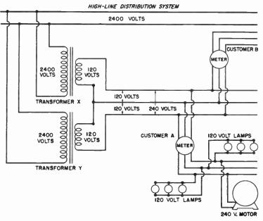
Fig. 11-42. How two transformers can be connected to a distribution system to supply power for a three-wire Edison system.
