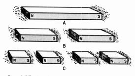
Fig. 8-17. Breaking a magnet results in the formation of new magnets which assume polarities as shown.
