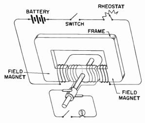
Fig. 12-6. Elementary separately-excited direct-current generator.
