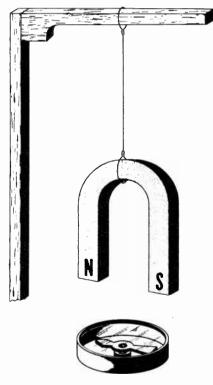
Fig. 13-6. An elementary demonstration to show the principle of a rotating magnetic field.
