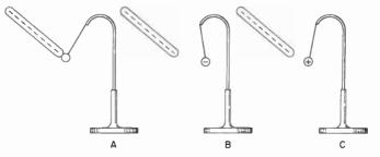
Fig. 3-3. Placing a charge on a pith ball electroscope. Electric charges may be identified and their forces of attraction and repulsion observed.
