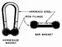
Fig. 8-6. The iron filings show where the lines of magnetic force exist.
