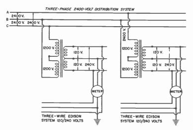
Fig. 11-51. How three-wire Edison-system power can be tapped off individual phases of the three-phase pawer distributian system. Pawer far use in the Edison system can be tapped off the distribution system between any two of the three wires.
