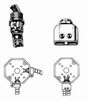
Fig. 15-26. Connectors used with armored cable and how they are used.
