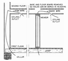
Fig. 15-29. It is often possible to fish armored cable through wall spaces without making holes in the wall or removing baseboard.
