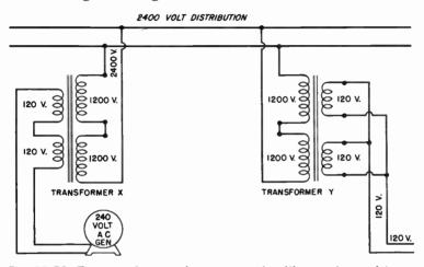
Fig. 11-52. Two transformers that are exactly alike can be used in two different and apposite manners.
