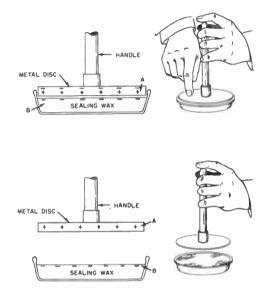
Fig. 3-14. The charges on an electrophorus.
