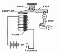
Fig. 14-31. Operating details of an annunciator drap.
