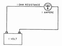
Fig. 6-6. One volt will force one ampere through one ohm of resistance.
