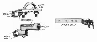
Fig. 15-22. Types of ground clamps and straps.
