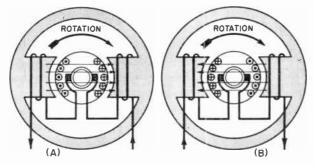
Fig. 13-33. The relationship between the direction of rotation of a series motor and the flow of current through the motor circuits.
