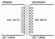
Fig. 11-32. If the secondary has the same number of turns as the primary, it will also have the same voltage.
