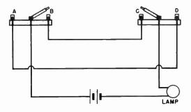
Fig. 14-35. How two single-pole double-throw knife switches can be connected to control a lamp from either of two positions.
