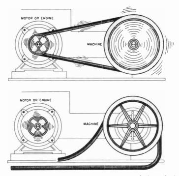
Fig. 4-14. An electric circuit must have a complete round-trip conductive path. This is just as necessary as it is to have a complete unbroken belt connecting the motor with the machine it is driving.
