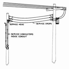
Fig. 15-6. The location of the service conductors, the service drops, and the service head in an overhead service to a meter pole.
