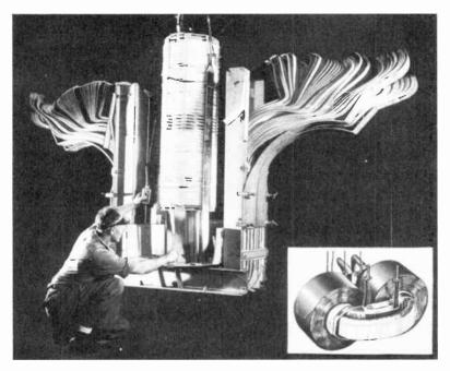
Fig. 11-13. A power transformer being assembled from a precut, preformed core of laminated steel strips. A small Spiracore transformer is shown in the insert.
