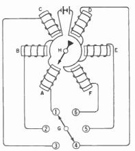
Fig. 13-8. This is a modified arrangement of Fig. 13-7 to show the principle of a rotating magnetic field.
