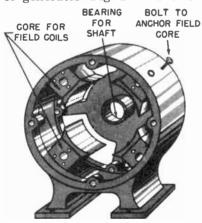
Fig. 12-21. The end bells and field cores are mounted on the frame. The bearings in the end bells receive the shaft on which the armature rotates.
