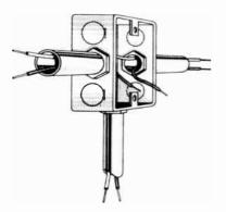
Fig. 15-23. How a junction box is used to make a connection to a branch circuit enclosed with rigid conduit.
