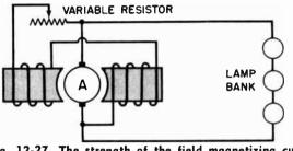
Fig. 12-27. The strength of the field magnetizing current in a shunt generator can easily be controlled by inserting a variable resistor in the field circuit.
