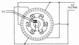
Fig. 13-4. A six-pole alternator with the armature wound on the stator, or frame, of the machine.
