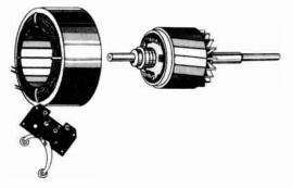
Fig. 13-23. The stator, rotor, and switch of a resistancestart induction motor.
