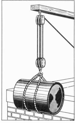
Fig. 10-5. Raising a barrel of apples into a loft involves the lifting of a specific weight a specific distance.
