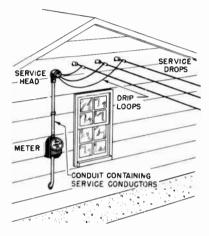
Fig. 15-8. The location of a meter on the side of a building when a meter pole is not used.
