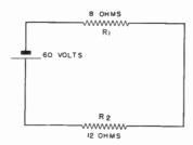
TOTAL RESISTANCE = 12 + 8 = 20 OHMS TOTAL CURRENT =  $\frac{60}{20}$  = 3 AMPERES VOLTAGE OROP ACROSS RI = 8 x 3 = 24 VOLTS VOLTAGE OROP ACROSS R2 =  $12 \times 3 = 36$  VOLTS TOTAL VOLTAGE OROP = 24 + 36 = 60 VOLTS
