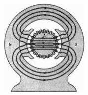
Fig. 12-19. The magnetic circuit of a generator or motor. The armature, the field cores, and the frame are all made of iron. The iron provides a low reluctance path for the magnetism.
