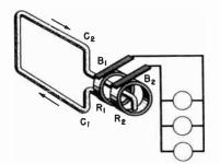
Fig. 12-14. Opening the loop and connecting the two ends of the conductor to slip rings make it possible to tap the current within the loop.
