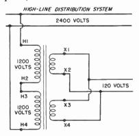
Fig. 11-46. The high-voltage windings are connected in series to serve as the primary for connection to 2400 volts. The low-voltage secondary windings are connected in parallel.
