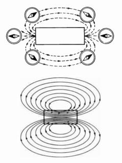
Fig. 8-11. The lines of force assume direction in the manner shown.
