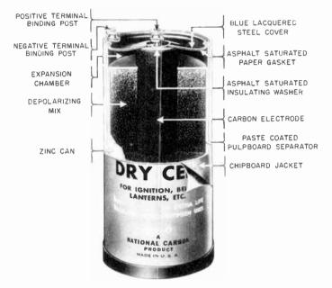
Fig. 4-19. A cut-away view of a dry cell. This is a primary electric cell. (Courtesy of National Carbon Co.)
