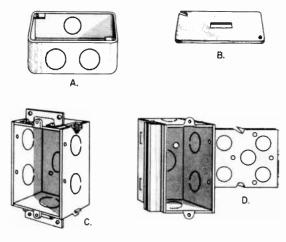
Fig. 15-33. "Switch boxes" used to enclose switches and convenience outlets.
