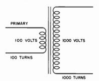
Fig. 11-34. If there are ten times as many turns on the secondary as on the primary, the voltage across the secondary will be ten times that across the primary.
