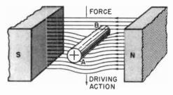
Fig. 12-10. A voltage is induced in a conductor when it is moved through a magnetic field.
