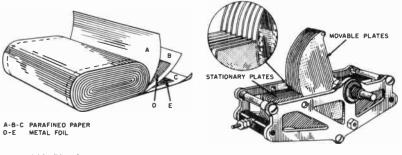
(A) Fixed paper capacitor. (B) Variable plate capacitor. Fig. 3-17. Construction of two types of copacitors.
