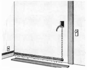
Fig. 15-39. How armored cable can be used for making an electrical extension without damaging the visible plaster.
