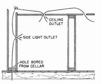
Fig. 15-27. Armored cable can be run from box to box. It can be easily fished through the hollow spaces within the walls and above the ceiling.
