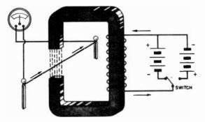
Fig. 11-28. During the instant a magnetic field is building up across the gap in the iron, the moving magnetic lines of force will induce a voltage in the conductor.
