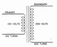
Fig. 11-33. If the secondary has twice as many turns as the primary, the secondary valtage will be twice as great as the primary valtage.
