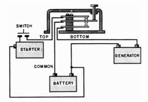
Fig. 14-8. How the principle of the two-contact switch can be applied to the automatic control of an automabile electric system.
