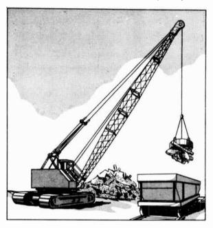
Fig. 9-15. Electromagnets are used to handle scrap iron.
