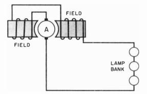
Fig. 12-25. Electrical circuit in a series generator. Note how the field coils obtain their exciting currents.
