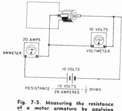
of a motor armature by applying Ohm's law to the measured current and voltage.
