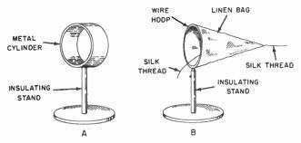
Fig. 3-10. A static charge is entirely on the outside surface of a metal cylinder or tube.
