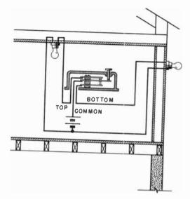
Fig. 14-7. How two lamps can be controlled from a single two-contact switch.
