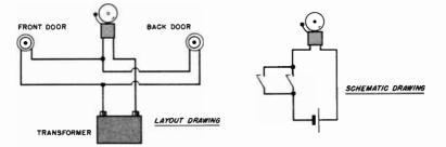
Fig. 14-24. A door bell controlled by two pushbuttons.
