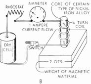
Fig. 9-21. The magnetic permeability (conductivity) of the core of an electromagnet depends not only upon the material of which it is made but also upon its size or cross-sectional area.
