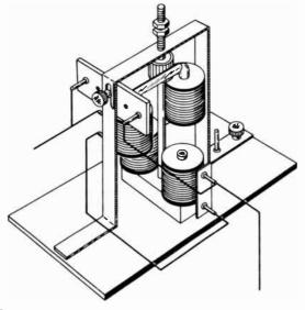
Fig. 12-3. The experimental direct-current generator as-' sembled ready for operation.
