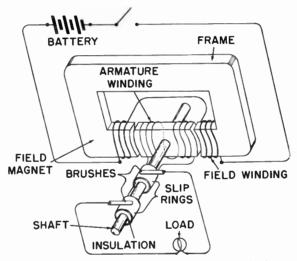
Fig. 12-S. Simple type of elementary (alternator) alternating-current generator.
