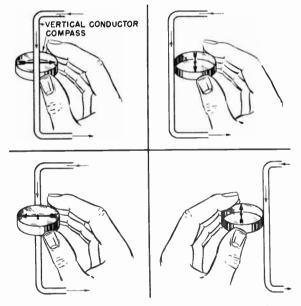
Fig. 9-1. The presence of a magnetic field around a conductor carrying an electric current can be detected by using a compass.
