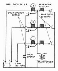
Fig. 14-27. A signal system commonly used in apartments.
