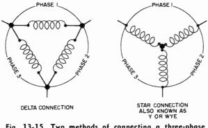
Fig. 13-15. Two methods of connecting a three-phase motor stator winding.
