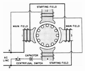
Fig. 13-25. The circuit of a capacitor-start motor, showing how the capacitor is connected in the starting winding circuit.
