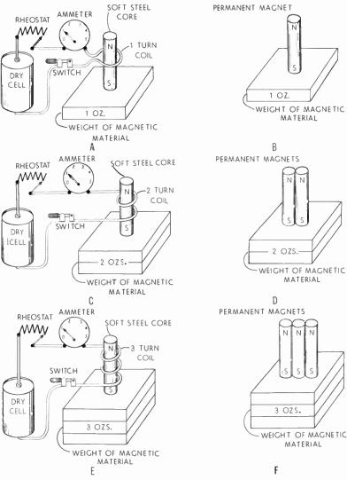
Fig. 9-18. Showing the relation of the magnetic strength of a solenoid to the number of turns in its winding.
