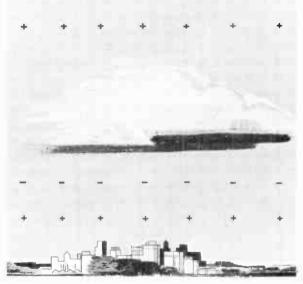
Fig. 3-18. During fair weather the earth's surface may be negatively charged, but it becomes positively charged by induction when a negative cloud passes over. (Courtesy of Westinghous Mfg. Corp.)
