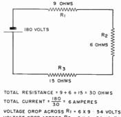
VOLTAGE OROP ACROSS R2 = 6 x 6 = 36 VOLTS VOLTAGE OROP ACROSS R3 = 6 x 15 = 90 VOLTS TOTAL VOLTAGE DROP = 54 + 36 + 90 = 180 VOLTS
