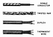
Fig. 14-21. Types of door-bell wire.
