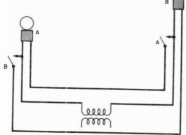
Fig. 14-25. A return-call system circuit.
