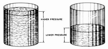
Fig. 4-16. There will be different amounts of pressure at the bottom of the two tanks because the level of water is higher in one than in the other.
