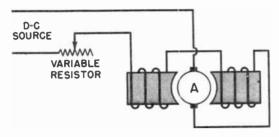
Fig. 12-30. A DC series motor can be controlled by inserting resistance in the circuits leading to the motor. The voltage drop across the resistance tends to reduce the voltage to the motor, thus slowing its speed.
