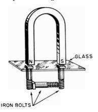
Fig. 8-20. There is no insulation for magnetism.
