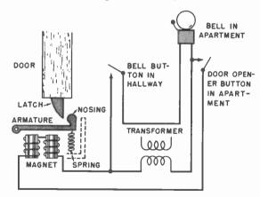
Fig. 14-28. Operating details of a door opener.
