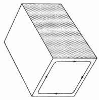
Fig. 11-7. Eddy currents are set up in a solid core through which alternating magnetic lines of force are passing.
