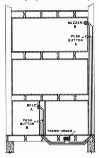
Fig. 14-26. The method of wiring a return-call system.
