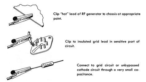
Fig. 11-9. RF (or marker) generator signal may be injected by being loosely coupled to receiver circuits.
