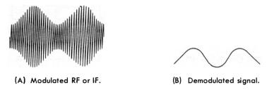
Fig. 12-2. Response patterns obtained in signal tracina an AM radio receiver.
