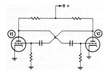
Fig. 3-7. Basic multivibrator circuit.
