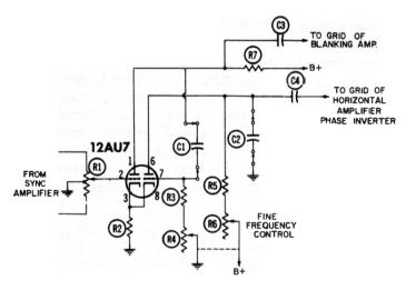
Fig. 3-12. Multivibrator sweep generator used in Simpson Model 466 HANDISCOPE.
