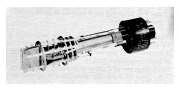
Fig. 1-4. Electron gun of cathode-ray tube.
