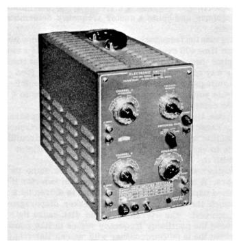
Fig. 7-20. The DuMont Model 330 electronic switch. (Courtesy of Allen B. DuMont Laboratories, Inc.)
