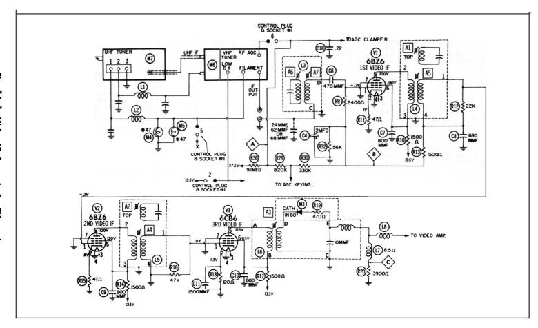
Fig. 11-1. Video IF channel of a TV receiver.
