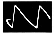
(A) Input signal to phase detector.
