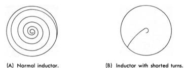
Fig. 7-11. Test waveforms obtained with Doss probe.
