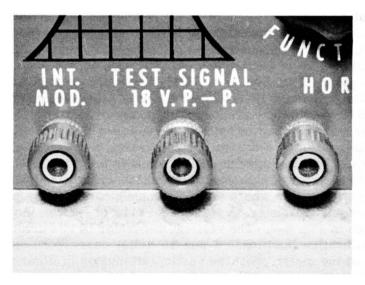
Fig. 6-1. Source of calibration voltage located on front panel of oscilloscope.
