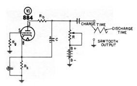
Fig. 3-4. Basic Thyratron sawtooth oscillator.
