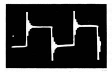
Fig. 10-7. Moderate ringing induced by application of square waves.
