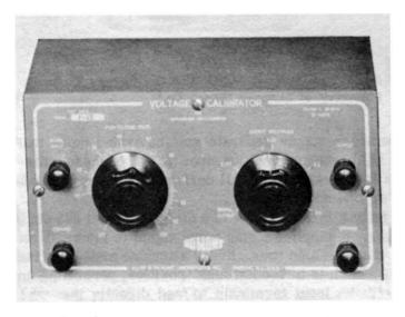
Fig. 7-12C. Dumont Type 264-B voltage callbrator.
