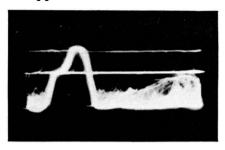
Fig. 8-8. Response showing effect of added input capacitance.
