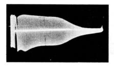
Fig. 10-10A. Response curve with generator connected directly to wide-band oscilloscope.
