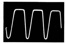
Fig. 12-14A. Triode operating characteristic with large signal overload.
