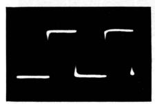
Fig. 10-1. A 1-kc square wave applied directly to the oscilloscope input.
