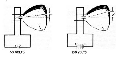
Fig. 1-7. The amount of deflection is directly proportional to the voltage applied to the plates.
