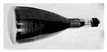
Fig. 1-3. Modern 5-inch cathode-ray tube.
