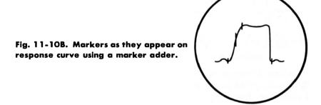
Since the sweep signals for the receiver response curve and marker adder are both taken from the same sweep generator, the marker will appear at its proper location when combined with the response curve. The marker signal does not pass through the receiver circuits and, therefore, is not attenuated by the trap circuits or amplified at peak response frequencies. The marker remains at the same amplitude on the oscilloscope screen as it is tuned across the entire response curve.
