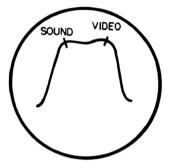
Fig. 11-12. Idealized tuner response curve.
