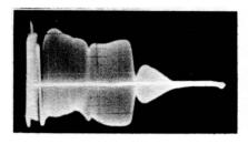
Fig. 10-12. Normal response of video amplifier.
