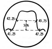
When the receiver is aligned for reception of normal strength TV signals, RF and video IF stages should be maintained at the same bias level that would be obtained with signals of this strength. In some amplifiers, the over-all response may change as the operating bias is changed. Therefore, to insure best response during actual reception, the receiver is aligned with normal operating bias. This also helps avoid adjustment of any stage to an overload condition.
