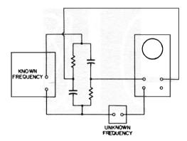
Fig. 9-4. Unknown frequency superimposed on circular trace resulting in crown wheel pattern.
