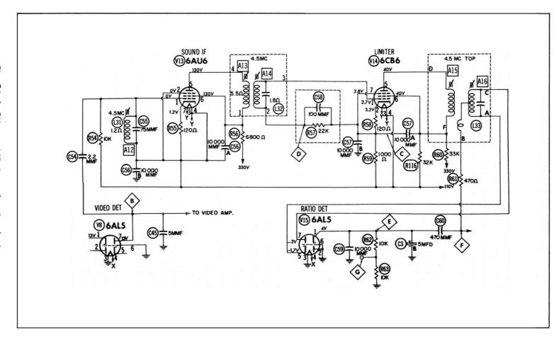
Fig. 11-6. FM sound IF channel and ratio detector.
