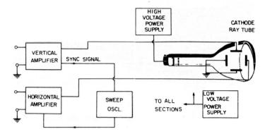
Fig. 1-2. Simplified block diagram of general-purpose oscilloscope.
