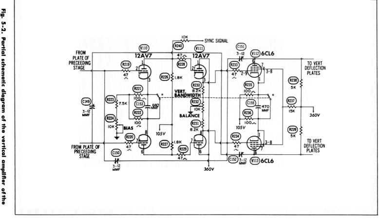
Fig. 5-2. Partial schematic diagram Hickok Model 770 oscilloscope. of the vertical amplifier
