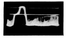
Fig. 8-7. Oscilloscope response using amplifier of 2-megacycle bandwidth.
