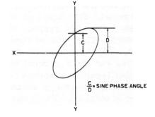
manner: Find the value of the sine by the preceding method. Locate this value and corresponding angle in the sine table. An angle between 0 and 90 degrees will be given, which should then be subtracted from 180 degrees for the final correct value.
