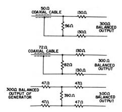
Fig. 11-5. Sweep generator attenuator pads.
