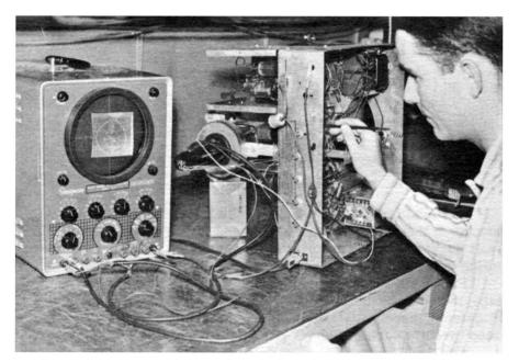
Fig. 7-9. "Plc-Probe" and scope together substitute for picture tube.
