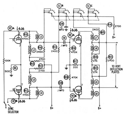
Fig. 5-1. Partial schematic diagram of the vertical amplifier of the Jackson Model CRO-2 oscilloscope.
