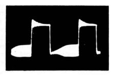
Fig. 10-8. Instability shown by continuous oscillation when square wave is applied.
