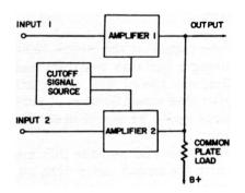
Fig. 7-16. Block diagram of an electronic-switch circuit.
