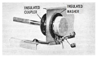
Fig. 2-6. One method of insulating between a control and the chassis.
