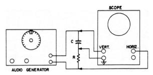
Fig. 3-8. Circuit for producing a circular trace, using one sine wave audio generator.
