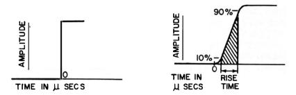
Fig. 5-6. Diagram illustrating rise time.
