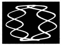
Fig. 9-5. 6 to 1 crown wheel pattern.
