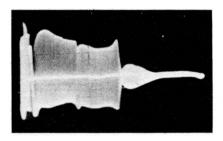
Fig. 10-18. Effect of stray capacity on high-frequency response.
