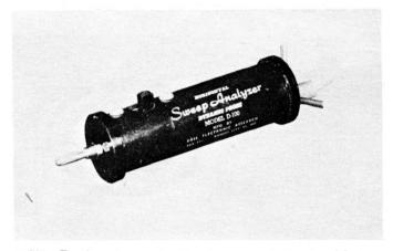
Fig. 7-10. Doss sweep analyzer, Model D-100, for use with an oscilloscope.
