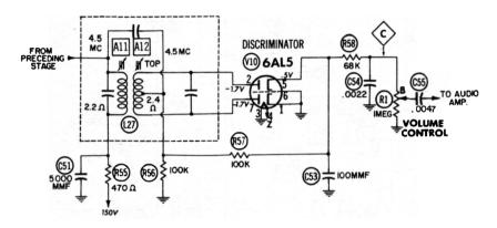
Fig. 11-7. Typical FM discriminator circuit.
