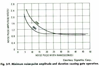
The curve of Fig. 3-9 is typical of the relation between the amplitude and duration of pulses causing a gate to operate. The 8400 gate is of the diode-transistor logic (DTL) type and is slower than the 8800 TTL gate. For pulses of the same amplitude the slower gate requires longer pulses for false operation. Pulses of any duration below 0.8 volt do not cause operation.
