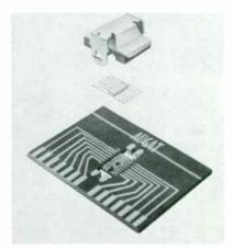
(C) Test board and socket for 14-pin flatpack integrated circuits.
