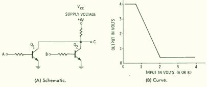
Fig. 3-2. Schematic and input-output curve for one kind of gate.
