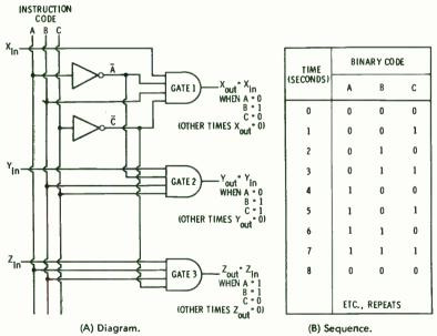
Fig. 4-4. Logic subsystem which passes three signals according to coded instructions.
