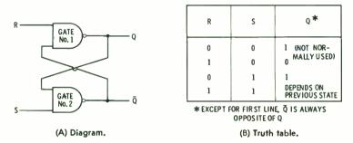
Fig. 5-1. R-S flip-flop using NAND gates.
