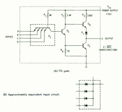
Fig. 6-6. Four-input TTL gate (TI Type SN7420).
