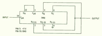
Fig. 8-14. The 7490 connected to divide-by-six.
