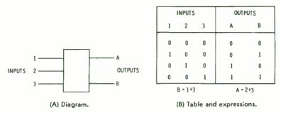
Fig. 4-22. Block diagram, truth table, and Boolean expressions for simple encoder.
