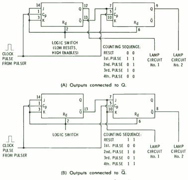
Fig. 8-12. Synchronous counters from the 7473.
