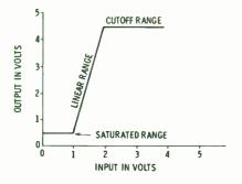
Fig. 3-1. Typical transistor amplifier inputoutput relation.
