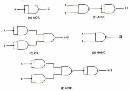
Fig. 4-30. Logic functions using only NAND gates.
