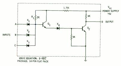
Fig. 6-5. Typical DTL gate (Fairchild DTµL 962).
