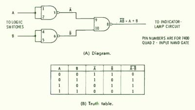
Fig. 8-8. An OR gate constructed from NAND gates.
