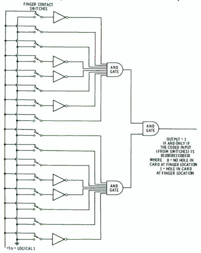
Fig. 4-5. Circuit producing logical 1 output for one 16-bit code.
