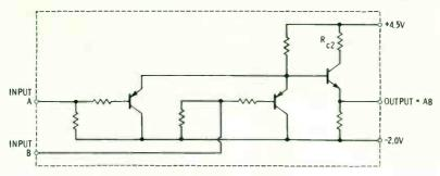
(A) Typical CTL two-input gate.
