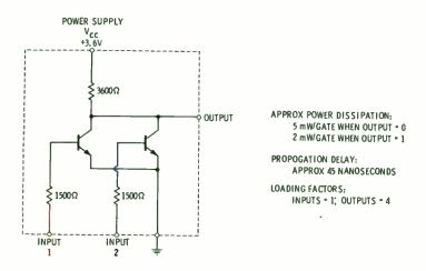
Fig. 6-4. Low-power RTL logic (Motorola MC 717P).
