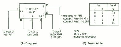
Fig. 8-10. Connections for studying the J-K flip-flop.
