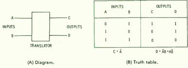
Fig. 4-19. Translator block diagram and truth table.
