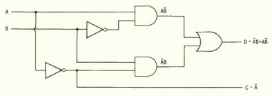
Fig. 4-20. Logic diagram for simple translator.
