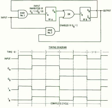
(B) With additional gates two R-S-T flip-flops can count to 3 and return to starting count (divide by 3).
