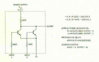
Fig. 6-3. Typical RTL gate (Motorola Type MC 724P).
