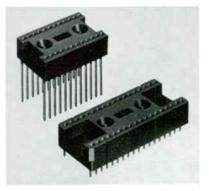
(B) 24-pin socket with wire-wrap terminals and 36-pin socket for printed boards.
