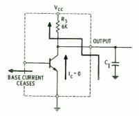
(A) Low transistor resistance permits capacitor voltage to fall quickly.
