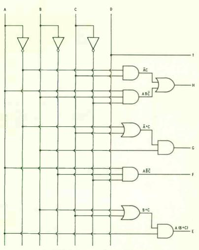
Fig. 4-21. Logic diagram for binary-to-BCD translator.
