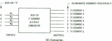
Fig. 4-26. ROM used as a converter from BCD to 7-segment readout code.
