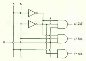
Fig. 4-11. Three-pole transfer switch using electronic gates.
