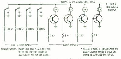
Fig. 8-4. Logic switch and lamp circuits.
