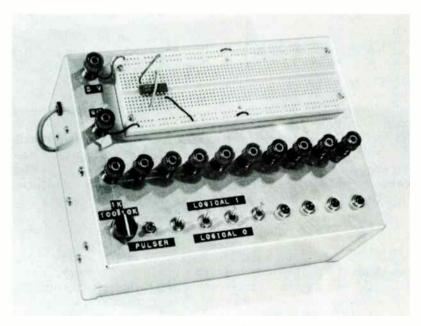
Fig. 8-1. Logic demonstrator/breadboarder.
