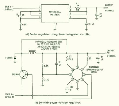
Fig. 7-5. Logic-circuit regulated power supplies.
