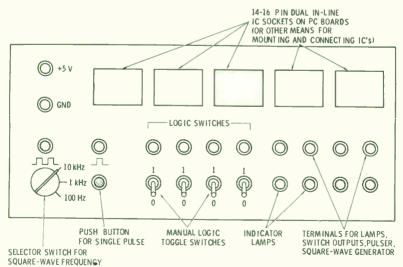
Fig. 8-2. Typical panel layout for logic demonstrator/breadboarder.
