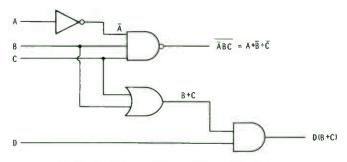
Fig. 3-4. Logic diagram showing interconnected gates.
