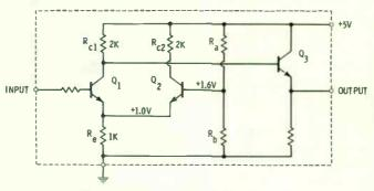
Fig. 6-8. Basic emitter-coupled logic circuit.
