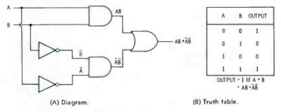
Fig. 4-15. Two-bit comparator.
