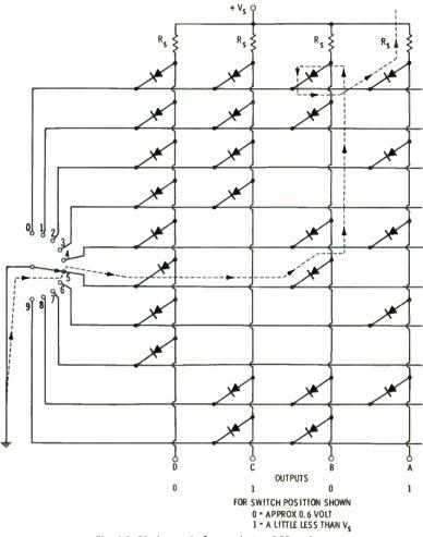
Fig. 6-2. Diode matrix for producing BCD code.
