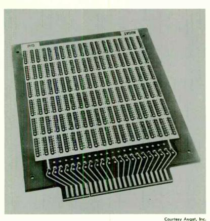
Fig. 7-1. Digital IC breadboard.
