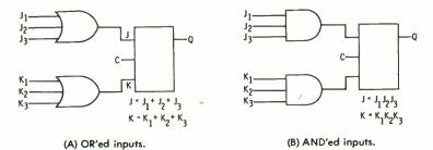
Fig. 5-9. J-K flip-flops with multiple inputs.
