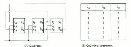
Fig. 5-11. Divide-by-5 parallel counter.
