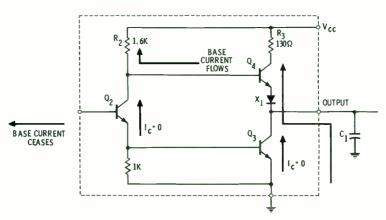
(C) C1 charges through active pull-up transistor when output goes high.
