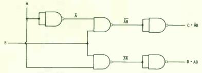
Fig. 4-28. Two-pole transfer switch using NAND gates.
