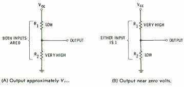
Fig. 6-11. Dc equivalent circuit of complementary MOS gate.
