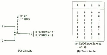
Fig. 4-8. Two-pole selector switch with truth table and Boolean expressions.
