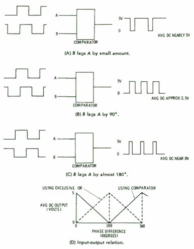
Fig. 4-18. Phase detector using comparator.
