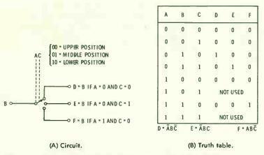
Fig. 4-10. Three switch positions represented by two-bit code.
