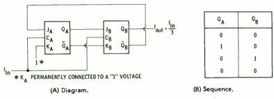
Fig. 5-10. Divide-by-3 parallel counter using J-K flip-flops.
