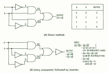
Fig. 4-17. Two methods of performing the exclusive-OR function.
