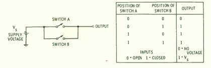
Fig. 2-1. OR logic circuit using switches.
