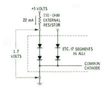
Fig. 8-15. Representation of an LED segment.
