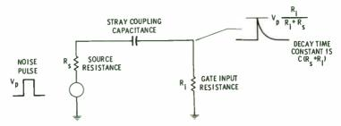
Fig. 3-8. Equivalent circuit for capacitively coupled noise pulses.
