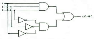
Fig. 4-16. Three-bit comparator.
