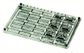
Courtesy Andresen Enterprises, Inc. Fig. 7-3. Logic-circuit breadboard.
