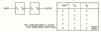
(A) Without additional gates two R-S-T flip-flops count to 4 (divide by 4).
