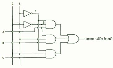
Fig. 4-14. Three-pole selector switch using gates.
