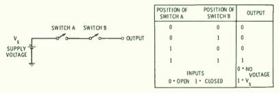
Fig. 2-2. AND circuit using switches.
