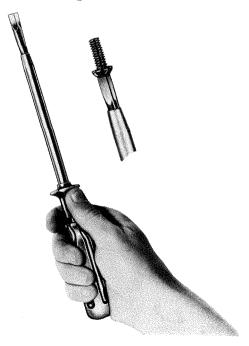
Fig. 1-8. Screw holding screwdriver.
