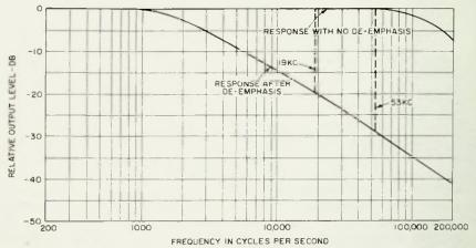
Fig. 3-10. Effect of de-emphasis on multiplex frequencies.
