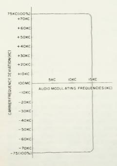
Fig. 2-1. Frequency distribution for FM station at 100 mc.
