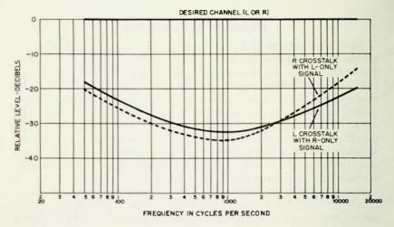
Fig. 5-4. Channel-separation curves.
