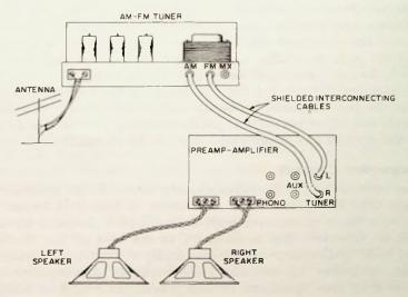
Fig. 3-18. Typical stereo component setup.
