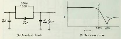
Fig. 4-19. Practical low-pass filter for switching demodulators.
