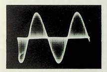
Fig. 2-8. L-only 400-cps waveform.
