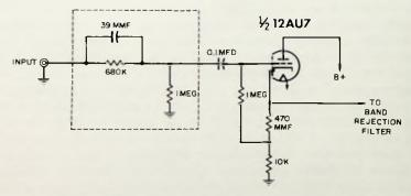
Fig. 5-6. Partial circuit of first stage of Pilot 100 and 200.
