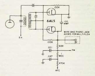
Fig. 3-15. Typical discriminator circuit.
