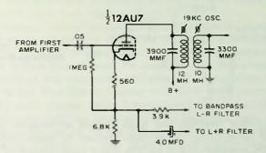
Fig. 4-9, Second (split-load) stage of Bogen PX-60.
