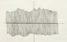
Fig. 5-2. Random modulation at junction of diodes X1 and X2 of Fig. 5-1.
