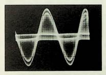
Fig. 2-11. Composite waveform with a left-only (or right-only) 400-cps tone.
