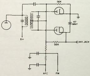
Fig. 3-16. Modified discriminator circuit.
