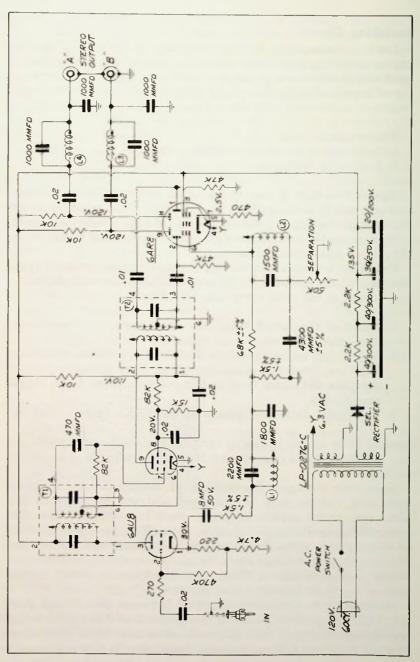
Fig. 5-3. Knight KN-MX adapter circuit.
