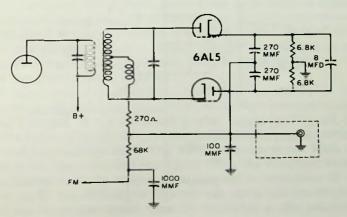
Fig. 3-14. Typical ratio-detector circuit.
