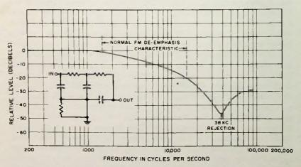
Fig. 4-33. Response of the filter shown in Fig. 4-32.
