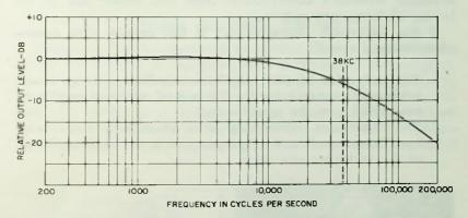
Fig. 3-11. Discriminator response with severe rolloff at subcarrier frequencies.
