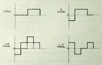
Fig. 1-1. Combining signals to obtain L+R and L-R.
