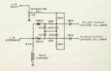
Fig. 4-29. Heath AC-11 detection and adding circuit.
