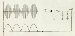
Fig. 2-10. Waveform obtained by rectifying sidebands without subcarrier.
