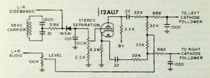
Fig. 4-30. Bogen PX-60 additive matrix circuit.
