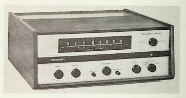
Fig. 7-9. Crosby RMX-30 stereo FM receiver.
