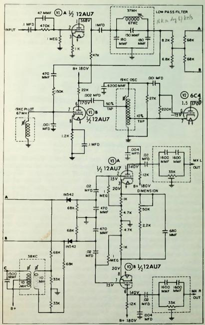
Fig. 7-8. Crosby RMX-30 multiplex section.
