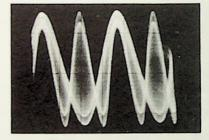
Fig. 2-13. Composite modulating signal with L=400~cps and R=800~cps.
