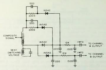
Fig. 4-31. Pilot Radio 100 and 200 demodulator circuit.
