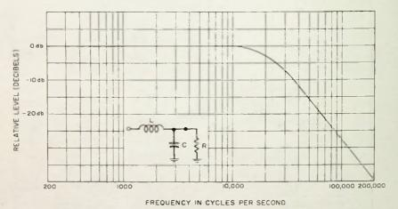
Fig. 4-2. Curve of low-pass filter
