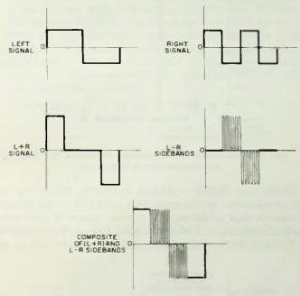
Fig. 2-14. Development of interleaving principle.
