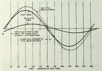
Fig. 5-11. Effect of multipath on 15-kc signal.
