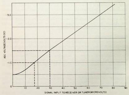
Fig. 3-6. AGC voltage developed at limiter grid.
