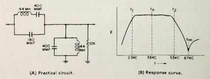
Fig. 4-18. A 5-element, m-derived, bandpass filter.
