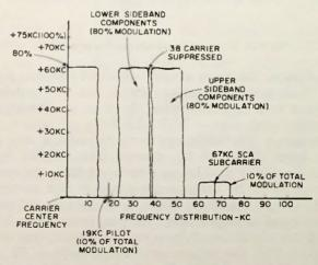
Fig. 2-16. Spectral distribution for stereo and SCA broadcasting.
