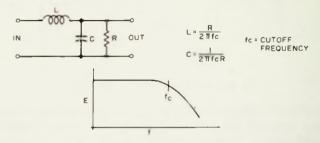
Fig. 4-17. Constant-K low-pass filter.
