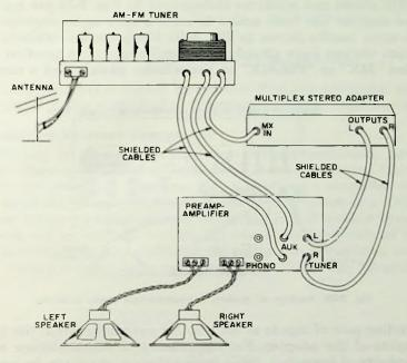
Fig. 3-19. System after multiplex adapter has been added.
