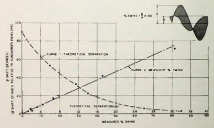
Fig. 5-13. Effects of phase shift on separation.
