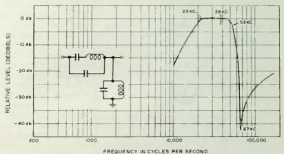
Fig. 4-3. Response of bandpass filter.
