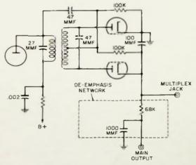
Fig. 3-7. Partial schematic of typical discriminator circuit.
