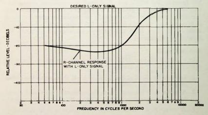
Fig. 5-5. Separation at high audio frequencies.
