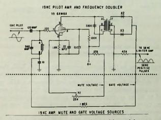
Fig. 7-21. Zenith 12H26 multiplex pilot amplifier and frequency doubler.
