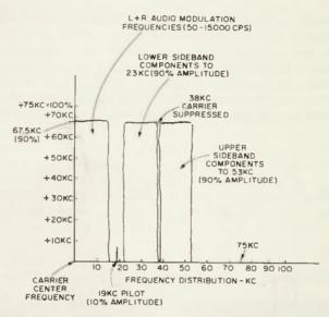
Fig. 2-15. Frequency and modulation distribution for stereo broadcasting without SCA service.
