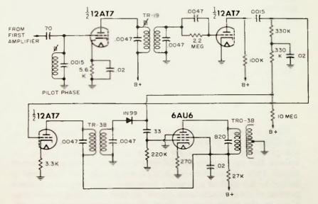
Fig. 4-14. Unusual circuit for developing 38-kc voltage.
