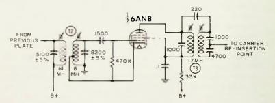
Fig. 4-12. Bogen TP-60 oscillator circuit.
