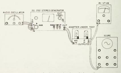
Fig. 6-6. Setup for aligning and testing multiplex equipment.
