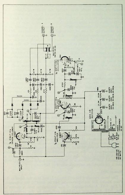
Fig. 7-16. Pilot Radio Model 100 adapter circuit.
