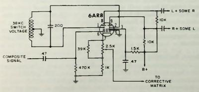
Fig. 4-25. Altac Lansing 359A demodulator circuit.
