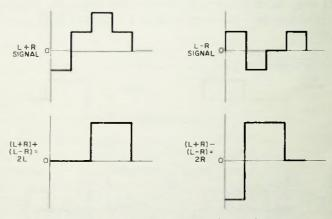
Fig. 1-2. Recovering left and right signals.
