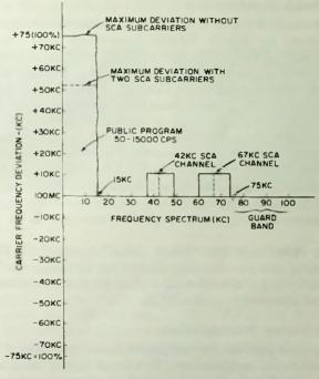
Fig. 2-2. Frequency distribution and deviation for monophonic plus SCA transmission.
