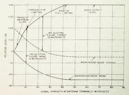
Fig. 3-4. Quieting curve for typical FM receiver.
