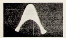
Fig. 3-13. Oscillograph showing unbalanced recovery of main and subchannel sidebands.
