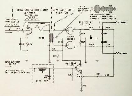
Fig. 7-22. Zenith circuitry showing subcarrier amplifier and reinsertion, L and R signal demodulation and matrixing.
