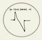
Fig. 5-10. Waveform indicating regeneration.
