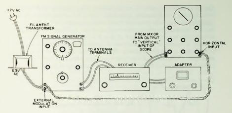
Fig. 5-8. Sweep-alignment setup.
