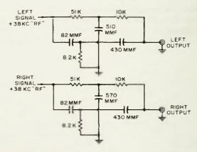
Fig. 4-32. Harmon-Kardon MX-500 twin-T notch filter (38 kc).
