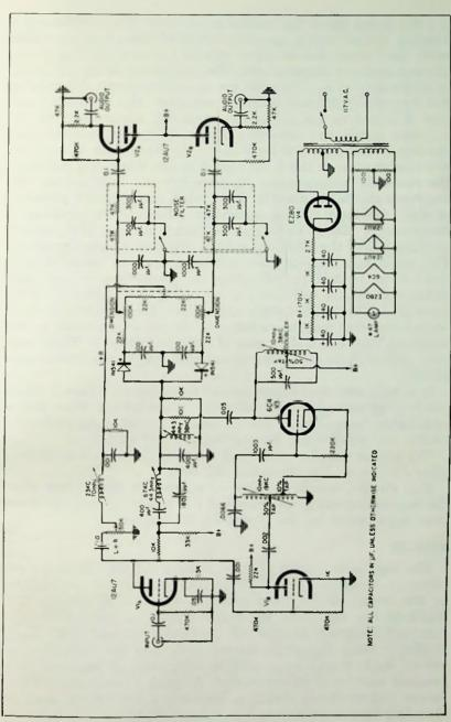
Fig. 7-7. Crosby MX-101 adapter circuit.
