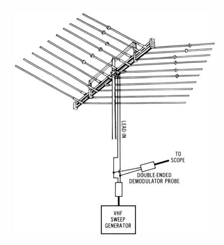
Fig. 3-41. Check of antenna impedance.
