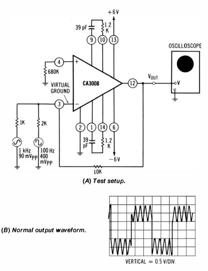
Fig. 6-10. Checking the operation of an op-amp scaling adder.
