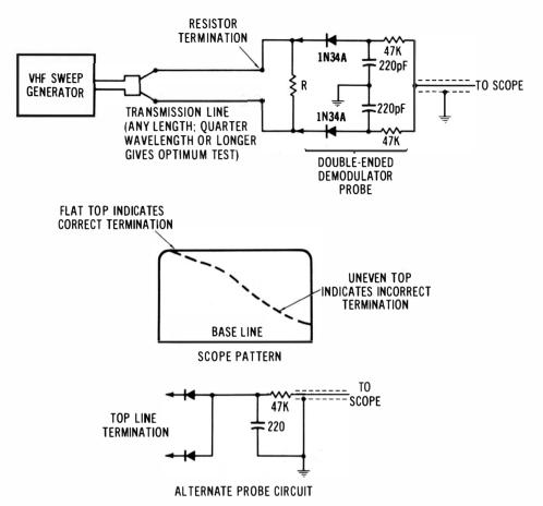
Fig. 3-39. Measurement of lead-in (transmission line) characteristic impedance.
