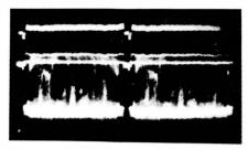
SYNC PUNCHING; VERTICAL-SYNC INTERVAL IS BELOW HORIZONTAL-SYNC LEVEL.
