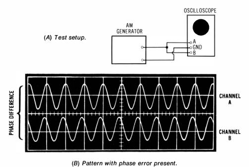
Fig. 7-4. Checking a dual-trace scope for A/B phase shift.
