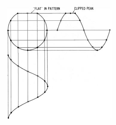
Fig. 3-34. Pattern becomes flattened when one of the input waveforms is clipped.
