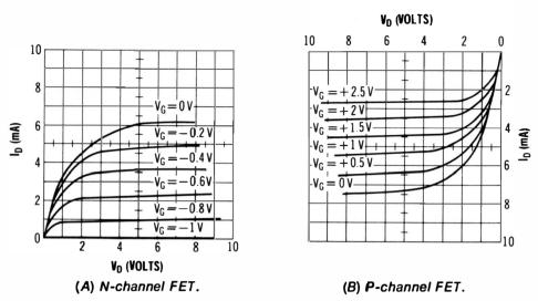
Fig. 5-17. Typical FET drain family characteristics.
