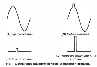
less. On the other hand, if any waveform is displayed, the amplifier is distorting, as exemplified in Fig. 1-3.
