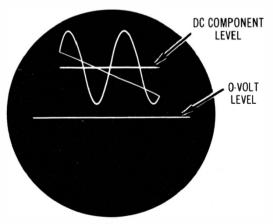
Fig. I-7. How an ac waveform with a dc component is displayed on the screen of a dc scope.
