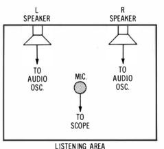
Fig. 1-18. Check of ringing frequencies (acoustic standing waves) in a listening area.
