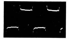
Fig. 3-19. Checking square-wave response of a high-performance video amplifier.
