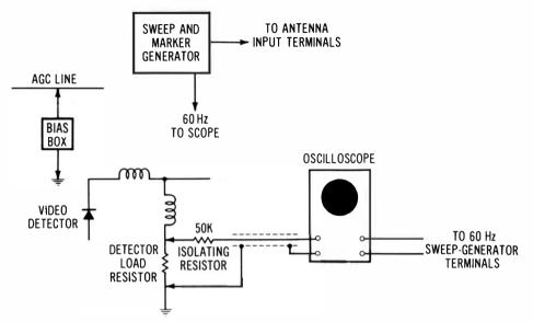
(A) Test connections for check of overall rf/if response curve.
