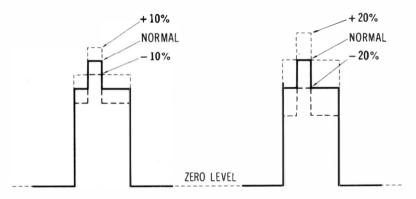
Fig. 3-24. Sync pulse amplitude tolerances.
