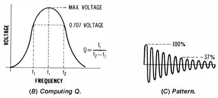
Fig. 6-1. Determination of bandwidth for LC circuit.
