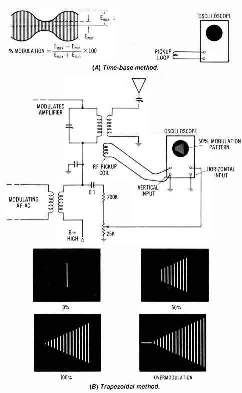
Fig. 6-4. Measurement of percentage amplitude.
