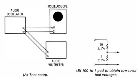
Fig. 7-2. Checking the accuracy of a calibrated vertical attenuator.
