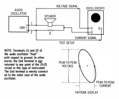
Fig. 2-1. Measurement of speaker impedance.
