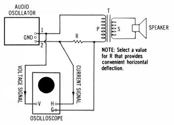
Fig. 2-2. Measurement of input impedance of a transformer.
