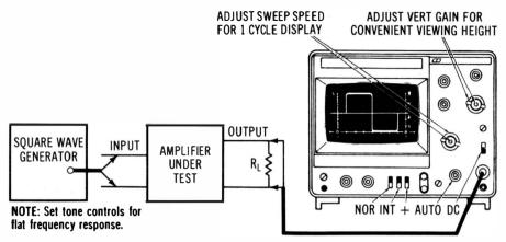
Fig. 1-9. Test setup for square-wave response.
