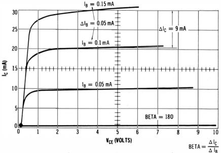
Fig. 5-7. Determination of transistor beta value.
