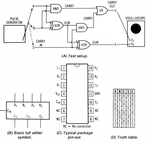
Fig. 4-9. Check of full adder operation.
