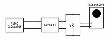
(A) Output voltage is measured at 1 kHz.
