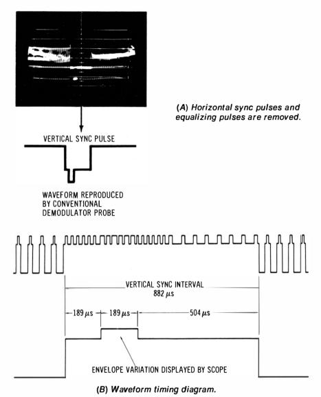
Fig. 3-7. Only the lower frequencies are reproduced by a conventional demodulator probe.
