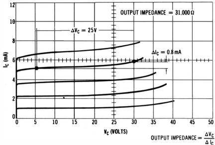
Fig. 5-9. Determination of transistor output impedance.
