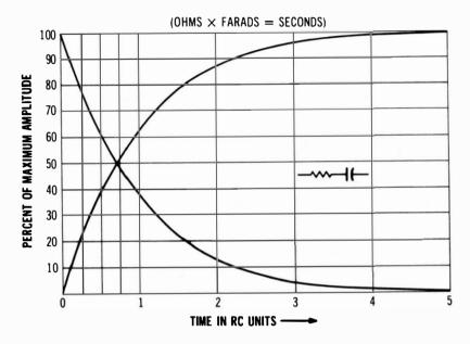
Fig. 6-8. RC differentiators and integrators produce exponential output waveforms.
