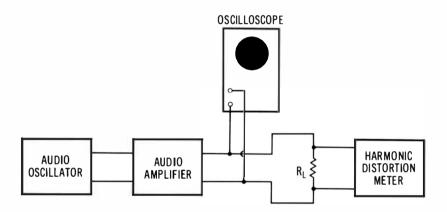
Fig. 1-11. Test setup for checking power bandwidth.
