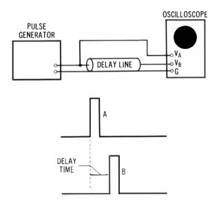
Fig. 3-44. Checking delay line action.
