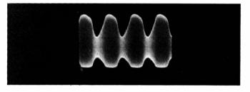
Fig. 6-5. Output signal from an economy-type am generator.
