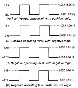
Fig. 4-4. Basic example of positive and negative operating levels, with positive and negative logic conventions.
