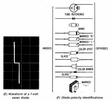
when the test leads are connected to a diode.
