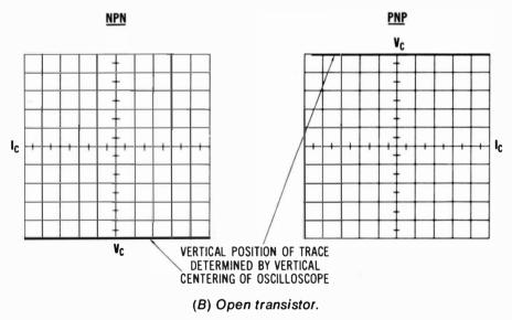
Fig. 5-6. Transistor curves.
