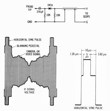
Fig. 3-10. A medium-impedance demodulator probe that can reproduce horizontal sync pulses.
