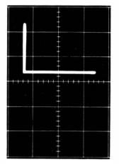
(B) Black test lead connected to diode anode.
