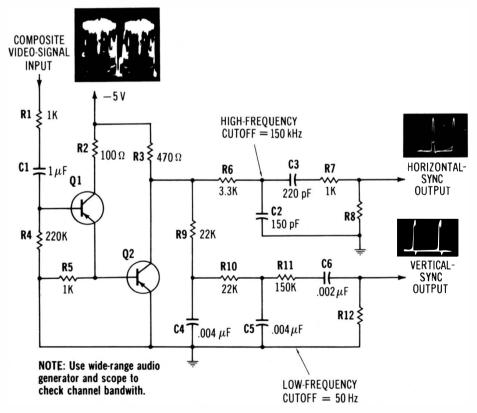
Fig. 3-23. A widely used sync-separator arrangement.
