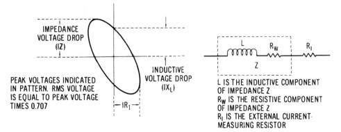
Fig. 2-6. Voltage indications in a Lissajous figure for a coil.
