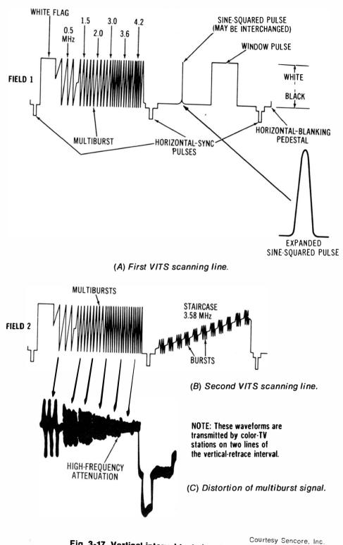
Fig. 3-17. Vertical-interval test signal (VITS).
