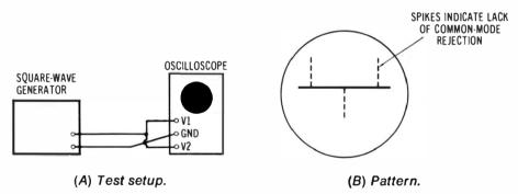
Fig. 7-6. Checking a differential-input scope for common-mode rejection.
