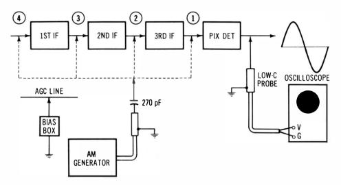
Fig. 3-11. Gain of third if stage is measured by transferring signal-injection point from (1) to (2).
