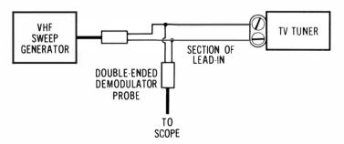
Fig. 3-40. Check of tv tuner input impedance.
