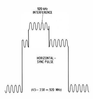
Fig. 3-29. Appearance of 920-kHz interference in the video signal.
