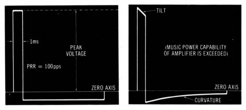
(B) Undistorted output pulse.
