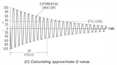
Fig. 3-45. Ringing test for yoke or other inductor.
