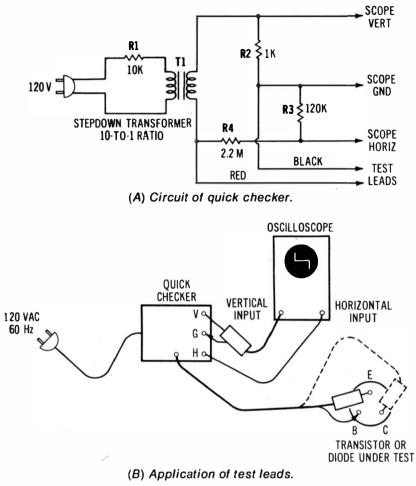
Fig. 5-1. Test of diode junction action.
