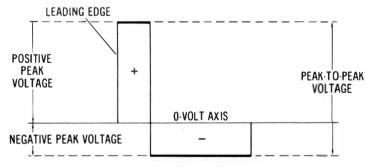
Fig. I-5. Basic pulse waveform.
