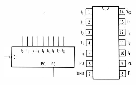
(B) Basic parity checker/generator symbol. (C) Typical package pin-out.
