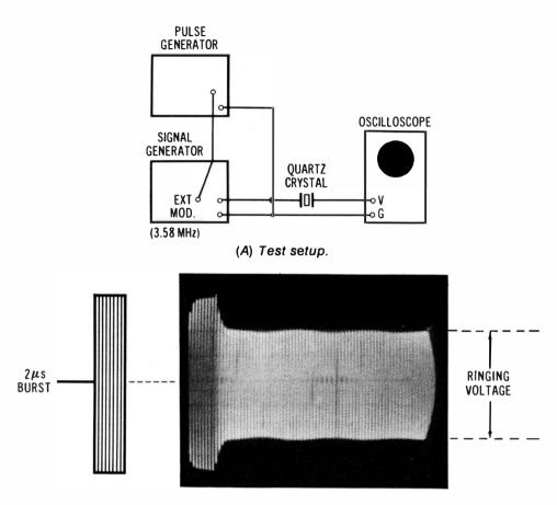
(B) 3.58-MHz ringing pattern (Q=8000 approximately). Fig. 3-38. Pulse ringing test of color subcarrier oscillator crystal.
