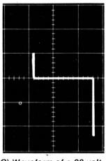
(C) Waveform of a 30-volt zener diode.
