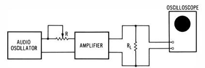
(B) Potentiometer resistance inserted to reduce output voltage to one-half.
