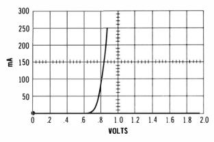
Fig. 5-23. Example of forward voltage drop display for an SCR.
