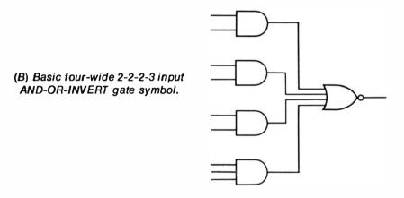
Fig. 4-8. Test of AND-OR-INVERT gate operation.
