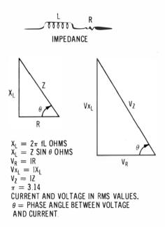
Fig. 2-7. Relations of resistance, inductance, and phase angle in coil in response to ac. divided finally by  $2\pi f$ , where f is the test frequency. The rms voltage is equal to 0.707 times the peak voltage. Pi is equal to 3.14.
