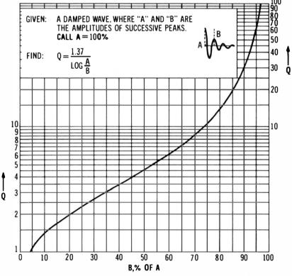
Fig. 3-46. Chart of Q values for a ringing system in terms of successive peak amplitudes.
