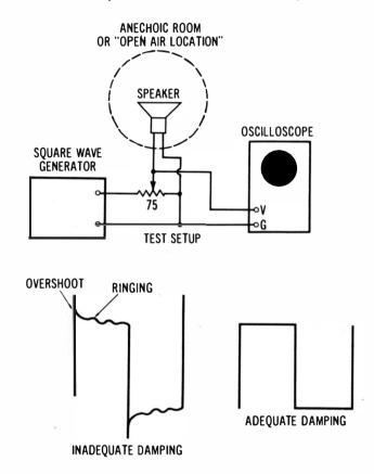
Fig. 1-17. Checking the optimum value of speaker damping resistance.
