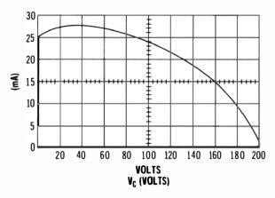
Fig. 5-22. Example of forward conduction at 200 volts, followed by holding-current indication of 5 mA.
