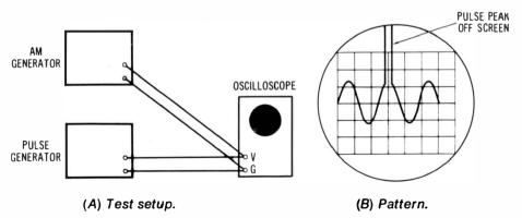
Fig. 7-5. Checking the overload recovery capability of an oscilloscope.
