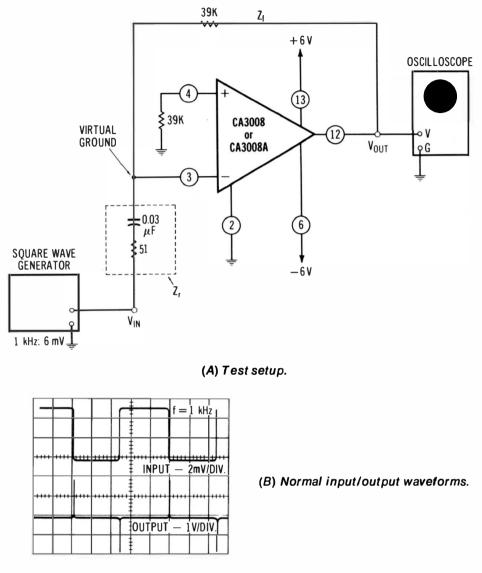
Fig. 6-7. Checking the operation of an op-amp differentiator.
