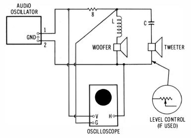
Fig. 2-5. Measurement of input impedance characteristic of an LC crossover network.
