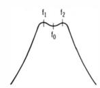
(B) The two resonant frequencies are  $f_1$  and  $f_2$ , and the ringing frequency is  $f_0$ .
