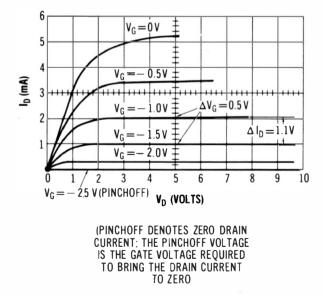
Fig. 5-18. Example of transconductance measurement.
