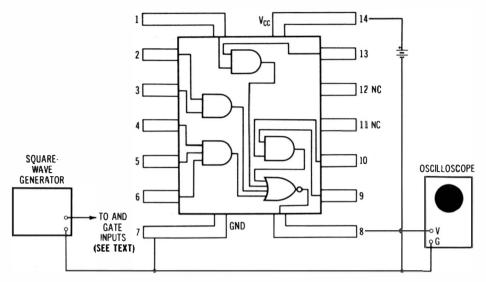
(A) Typical package pin-out and test setup.
