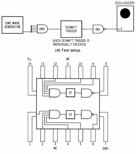
(B) Typical dual Schmitt trigger package pin-out. Fig. 4-14. Checking operation of a Schmitt trigger.
