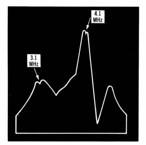
Fig. 3-35. Typical bandpass-amplifier response curve, with absorption markers at 3.1 and 4.1 MHz.
