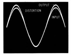
Courtesy Sencore, Inc. Fig. 1-1. Checking for audio distortion with a dual-trace oscilloscope.
