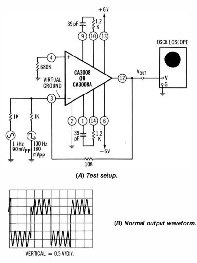
Fig. 6-9. Checking the operation of an op-amp summer (adder).
