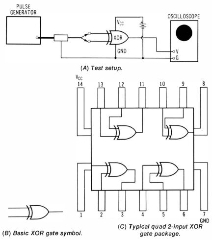
Fig. 4-6. Checking the operation of an XOR gate.
