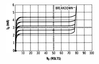
Fig. 5-20. Example of FET breakdown voltage measurement.
