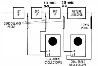
(B) Two dual-trace scopes monitoring four signal points in the if section.
