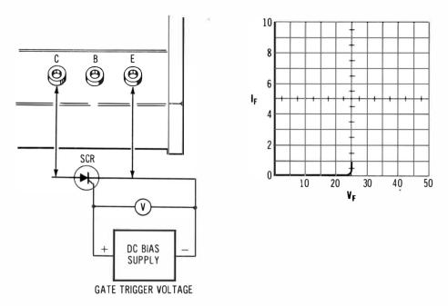
Fig. 5-24. Check of gate trigger voltage for an SCR.
