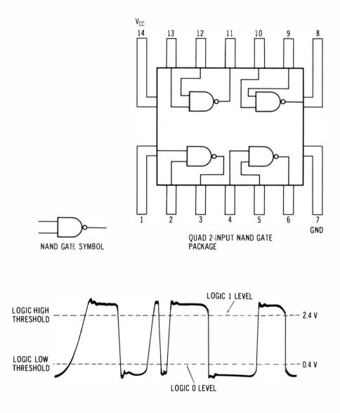
Fig. 4-2. Typical digital waveform in TTL circuitry, showing High (1) and Low (2) thresholds. (CMOS circuitry employs supply voltages in the range from 3 to 18 volts; check manufacturer's data sheet).
