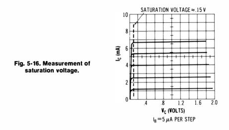
gion up to and including the knee of each curve. Thus, the display can be expanded, using a low-voltage horizontal calibration value, such as 0.2 volt per division. This facilitates accurate measurement of low collector voltage values. Data sheets usually specify saturation-resistance values as maximum acceptable limits.
