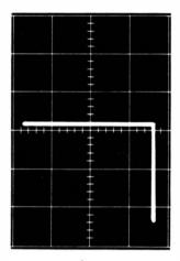
(A) Black test lead connected to diode cathode.
