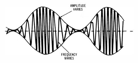
Fig. 3-22. A 100-percent amplitude-modulated output signal from an am generator, with incidental frequency modulation.
