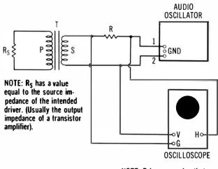
NOTE: R has any value that provides ample horizontal deflection on the scope screen.
