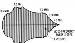
(B) Representative scope pattern at picture detector output.
