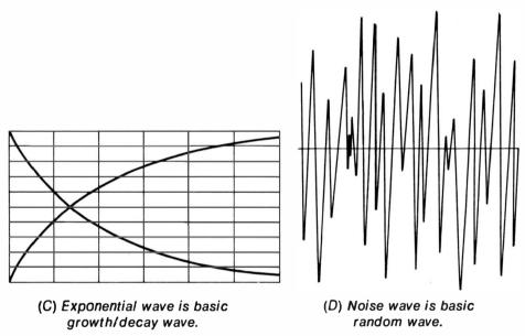
Fig. 3-5. Four fundamental waveforms.
