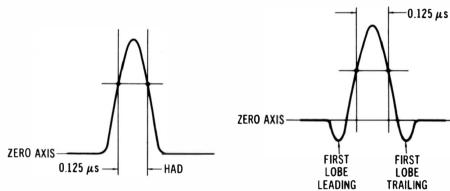
(A) Transmitted waveform with halfamplitude duration (H.A.D.) of 0.125 μs.
