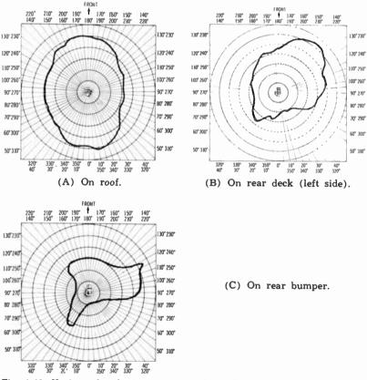
Fig. 4-19. Horizontal radiation patterns when whip antenna is mounted at various places on a car.
