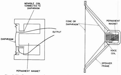
Fig. 2-25. Cross-sectional view of a dynamic microphone.
