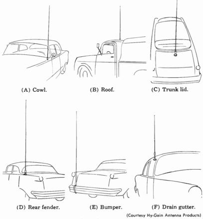
Fig. 4-18. Typical mobile whip mounting locations.
