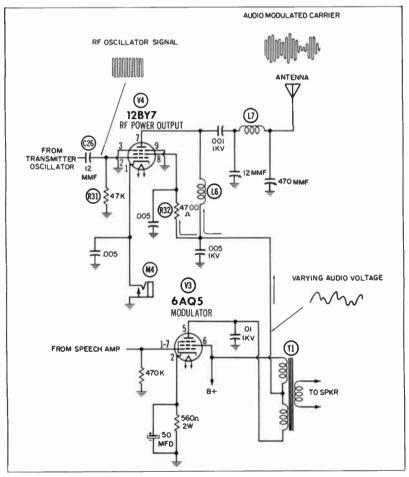
Fig. 3-24. A typical RF power-output stage.
