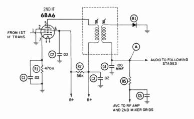
Fig. 3-15. An AVC system using the second detector as the rectifier.
