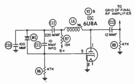
Fig. 3-22. A crystal-controlled transmitter oscillator circuit.
