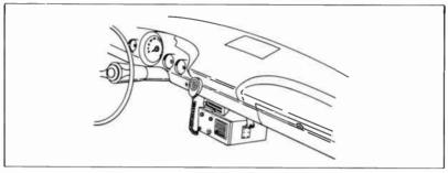
Fig. 5-6. Suitable brackets permit transceiver to be mounted below interfering objects.
