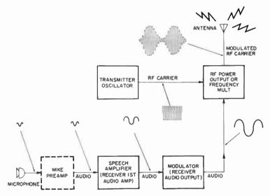
Fig. 3-20. Functional block diagram of a typical Class-D transmitter.
