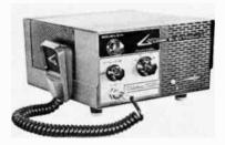
(Courtesy Globe Electronics Co.) Fig. 2-3. The Globe Star Class-D transceiver has a five channel crystal-controlled transmitter and a dual conversion superhet receiver.
