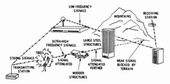
Fig. 1-2. An example of the UHF signal's line-of-sight characteristics.
