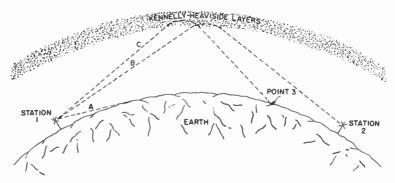
Fig. 4-3. Characteristics of high-frequency (HF) signals.
