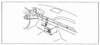
Fig. 5-7. A floor mounting can be used if no space is available under the dash.
