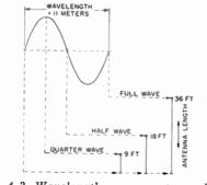
Fig. 4-2. Wavelength versus antenna length.
