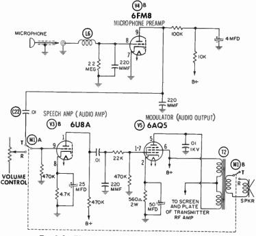
Fig. 3-21. The transmitter audio-amplifier section.
