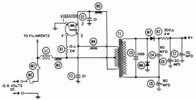
Fig. 3-26. Vibrator power supply employed for DC operation.
