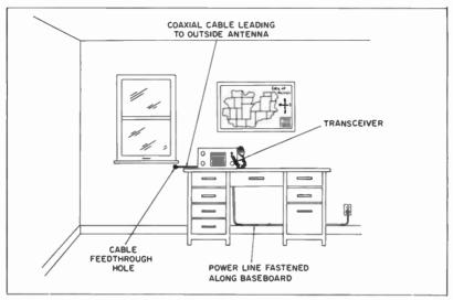
Fig. 5-1. A typical Class-D fixed-station installation.
