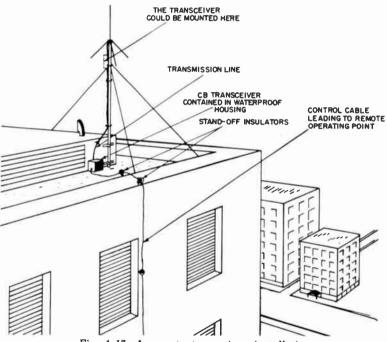
Fig. 4-17. A remote transceiver installation.
