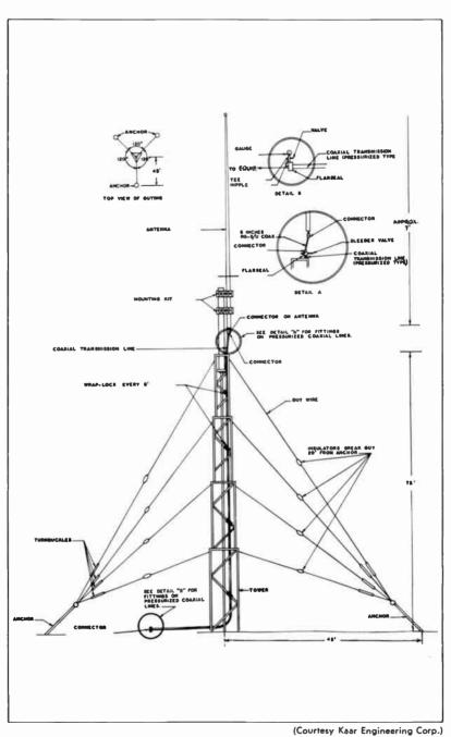
Fig. 4-12. Typical antenna installation for a Class-A base station.
