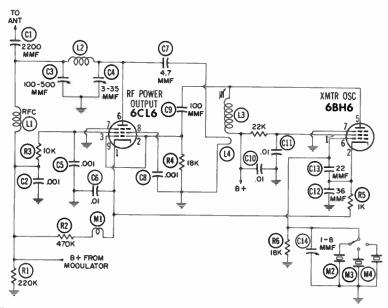
Fig. 7-7. RF section of a CB transmitter using a single trimmer capacitor for all three crystals.
