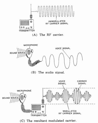
Fig. 8-4. Producing an amplitude-modulated carrier.
