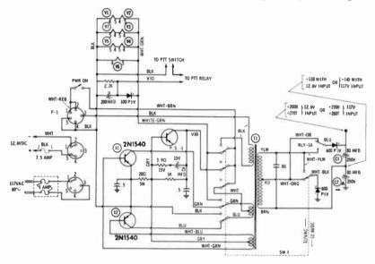
Fig. 3-30. Schematic of the transistor power supply used in the transceiver of Fig. 3-29.
