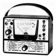
(Courtesy SECO Electronics, Inc.) Fig. 7-4. SECO Model 510B CB transmitter tester.
