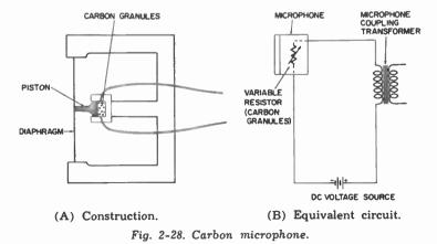
the resistance offered by the carbon will affect the DC current accordingly (Fig. 2-28B). Sound waves striking the diaphragm set it and the attached piston into motion. This action varies the pressure applied to the carbon "button," as it is called. This variation in resistance varies the DC current in accordance with the frequency and intensity of the sound waves.
