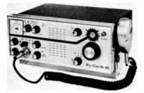
Fig. 2-18. The Poly-Comm Senior 23 provides crystal-controlled operation over all 23 Class-D channels. Includes such other features as built-in tone squelch, dual-conversion superhetrodyne receiver, nuvistor RF and mixer stages, and adjustable modulation.
