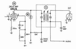
Fig. 3-19. A simple noise-clipping circuit using a neon bulb.
