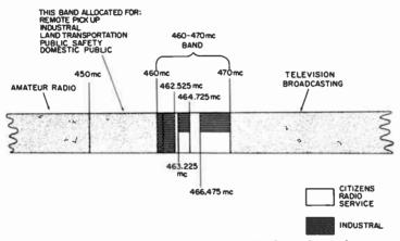
Fig. 1-1. Position of Class-A and -B channels in the frequency spectrum.
