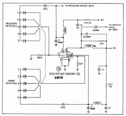
Fig. 3-23. A circuit incorporating the transmitter and receiver oscillators in in the same tube.
