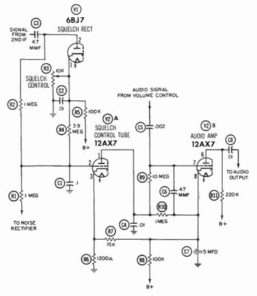
Fig. 3-17. A typical signal-operated squelch circuit.
