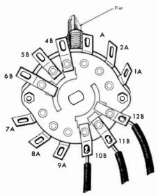
Fig. 3-7. A detailed diagram showing multielement-switch connections.
