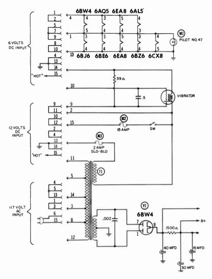
Fig. 3-27. Schematic of a universal power supply.
