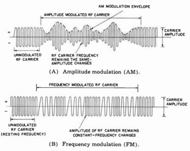
Fig. 1-4. Two types of modulation used in CB radiotelephone communications.
