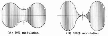
Fig. 8-5. Effect of modulation on the RF carrier.
