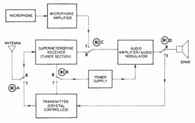
Fig. 3-2. Block diagram of a Class-D transceiver employing a superhet receiver.
