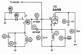
(C) Combination fixed-tuned and tunable. Fig. 3-12. Typical oscillator circuits in CB receivers.
