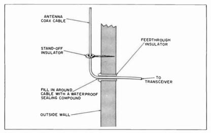
Fig. 5-2. Method of feeding the antenna cable through a wall.
