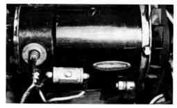
Fig. 5-14. A noninductive capacitor installed on a generator.
