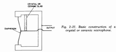
Fig. 2-27. An inherent characteristic of the ceramic or crystal slab is its ability to generate a minute voltage when twisted or bent. As the sound waves move the diaphragm back and forth, the slab bends and produces a corresponding voltage. Crystals cannot withstand prolonged temperatures above approximately 120°F. This important point should be kept in mind when choosing equipment which uses such a microphone.
