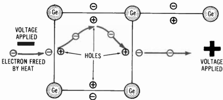
**Fig. 3-5.** Electron flow through intrinsic germanium.
