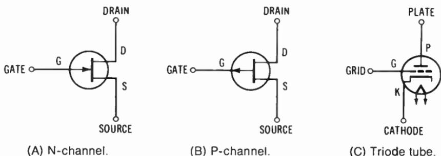
**Fig. 8-2. Field effect transistors.**
