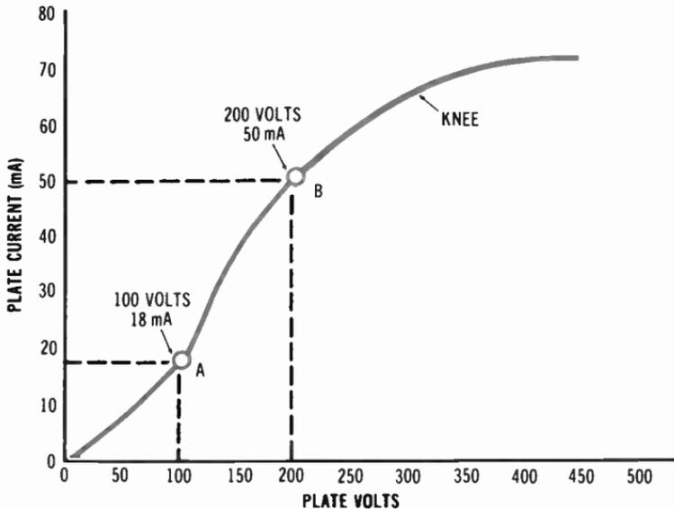
**Fig. 1-23.** Graph of plate voltage versus plate current.
