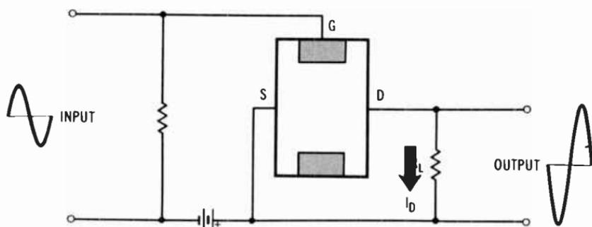
Fig. 8-9. JFET with an ac input signal.
