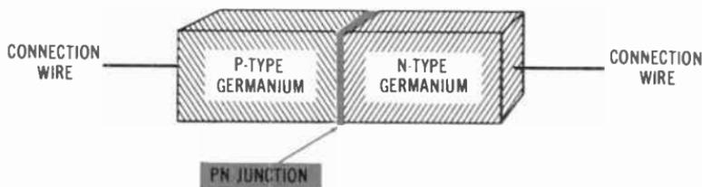
Fig. 3-13. Diagram of a solid-state diode.
