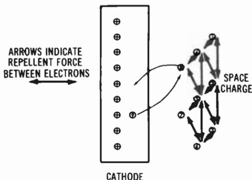
**Fig. 1-16. Emission saturation.**
