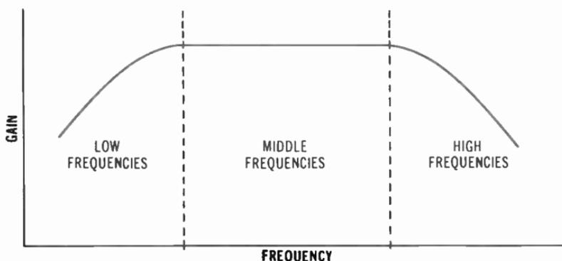
**Fig. 5-18. Graph showing relationship of gain to frequency.**
