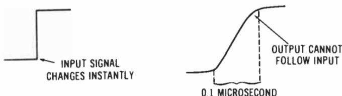
Fig. 7-1. Limited transient response of a transistor.
