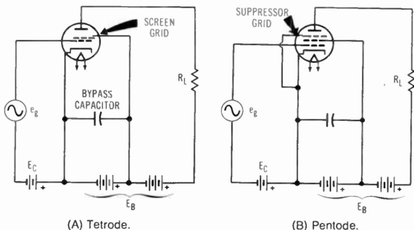
**Fig. 5-5. Amplifiers with multigrade tubes.**
