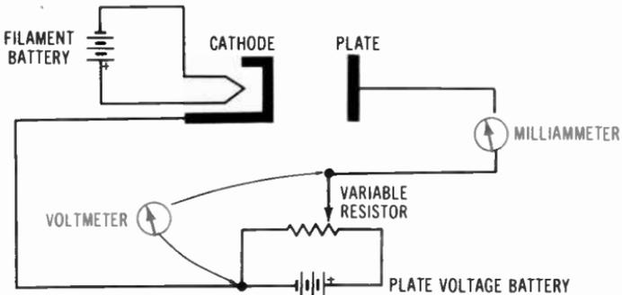
**Fig. 1-24. Circuit to obtain data for graph.**
