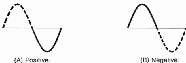
**Fig. 7-18.** Sine waves limited at zero volts.
