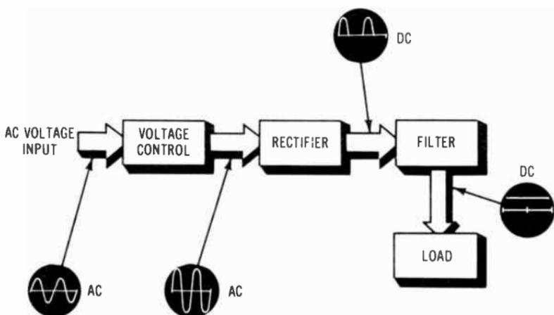
**Fig. 4-1. Components of a dc power supply.**
