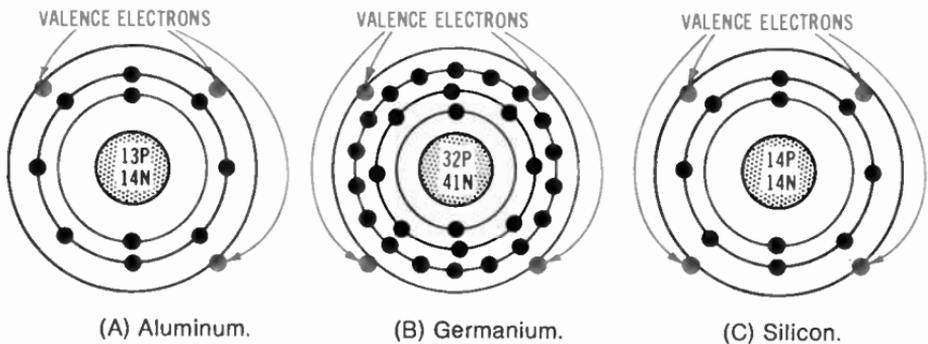
Fig. 3-2. Diagrams of atoms.
