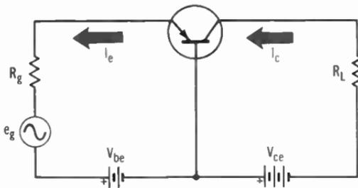
Fig. 6-3. Common-base circuit with ac signal source.
