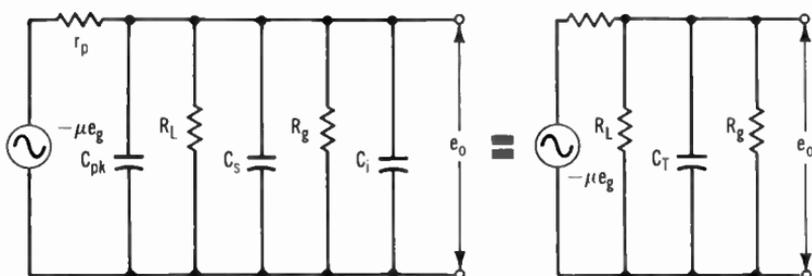
**Fig. 5-17. High-frequency equivalent circuit.**
