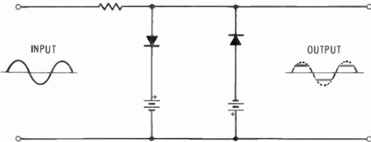
**Fig. 7-20. A positive and negative limiting circuit.**
