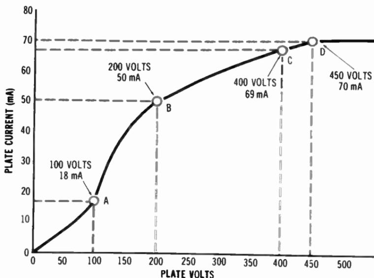
Fig. 1-25. Points for calculating dc plate resistance.
