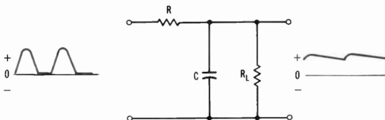
**Fig. 4-19.** L-section filter with series resistor.
