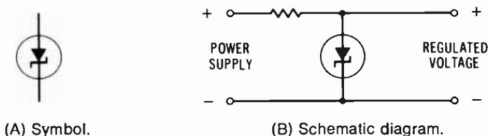
**Fig. 4-24. Zener-diode voltage regulator.**
