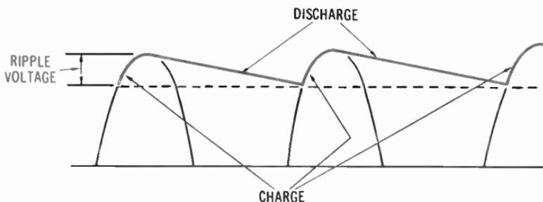
**Fig. 4-18. Capacitive filter charge and discharge.**
