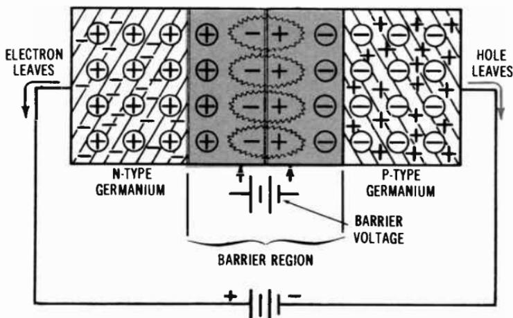
**Fig. 3-16. Reverse-biased diode.**
