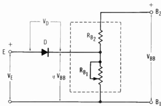
Fig. 8-11. Unijunction transistor equivalent circuit.
