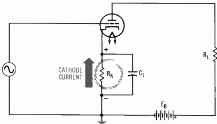
Fig. 5-12. Circuit using cathode-bias resistor.
