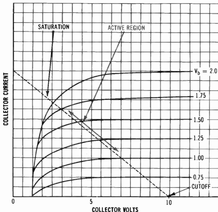
Fig. 7-4. Transistor characteristic curves.
