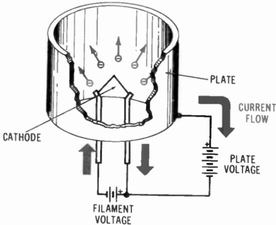
**Fig. 1-8. Positive plate attracts electrons from cathode.**
