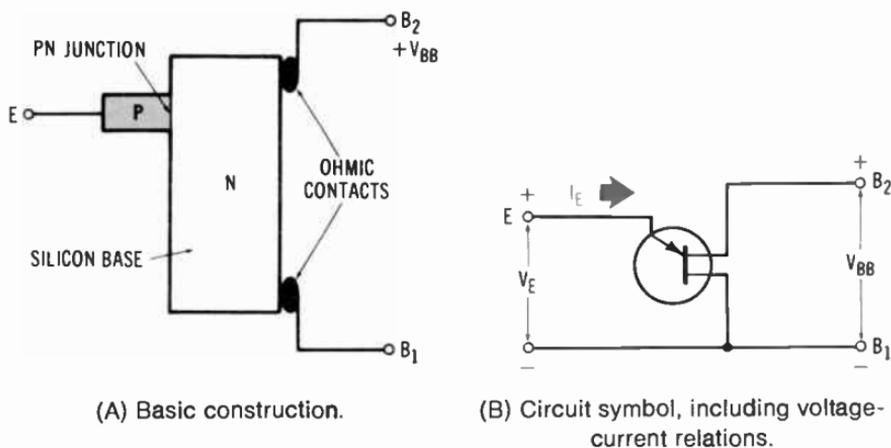
Fig. 8-10. Basic construction of unijunction transistor.
