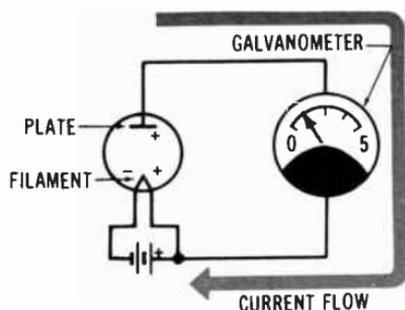
Fig. 1-9. Circuit for demonstrating Edison effect.
