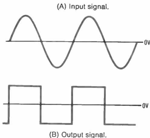
**Fig. 7-22. Schmitt-trigger waveforms.**
