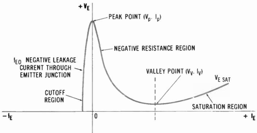
**Fig. 8-12.** Unijunction transistor voltage-current characteristic.
