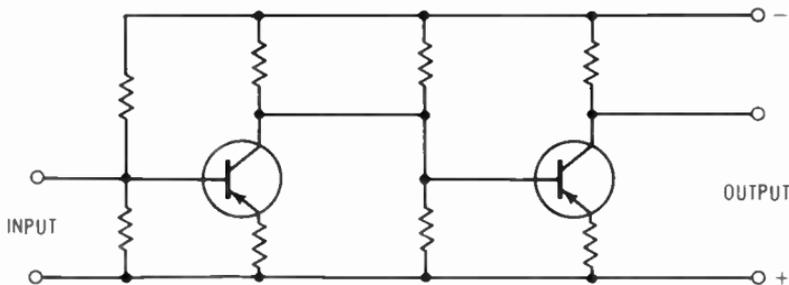
**Fig. 6-10. Direct-coupled transistor amplifier.**
