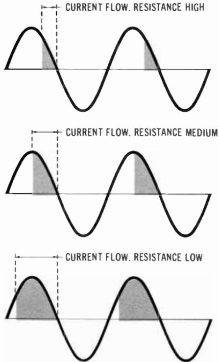
**Fig. 8-17. Phase control of current through a load.**
