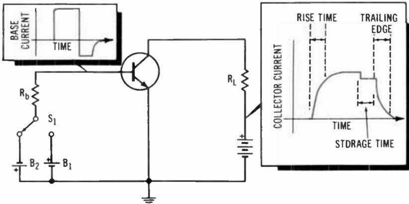
Fig. 7-2. Transient response of a circuit.
