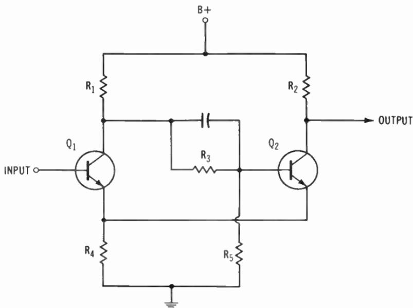
**Fig. 7-21.** A Schmitt-trigger circuit.
