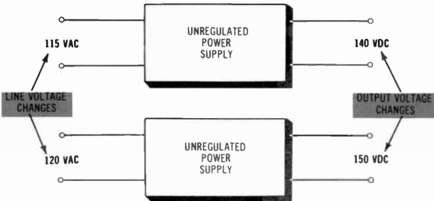
**Fig. 4-7. Unregulated power-supply action.**
