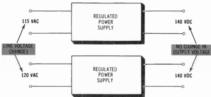
**Fig. 4-8. Regulated power-supply action.**
