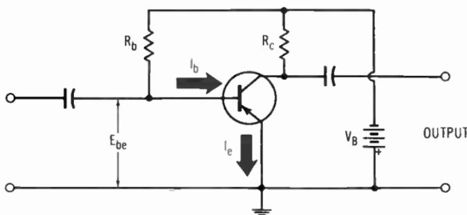
**Fig. 6-5.** Circuit for applying fixed bias.
