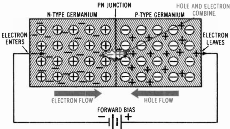
Fig. 3-17. Forward-biased diode.
