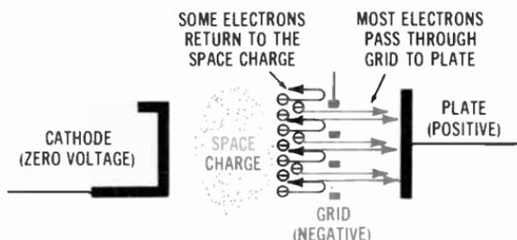
Fig. 2-4. Electron movement in a triode.
