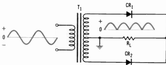
**Fig. 4-13 Full-wave semiconductor rectifier.**
