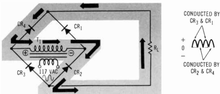
**Fig. 4-15. Bridge rectifier (negative half cycle).**
