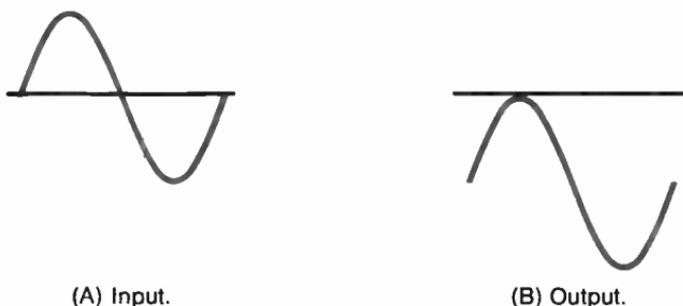
**Fig. 7-24. Waveforms in a negative dc restorer.**
