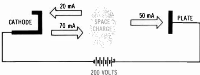
Fig. 1-20. Plate 200 volts positive.
