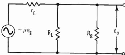
**Fig. 5-16. Medium-frequency equivalent circuit.**
