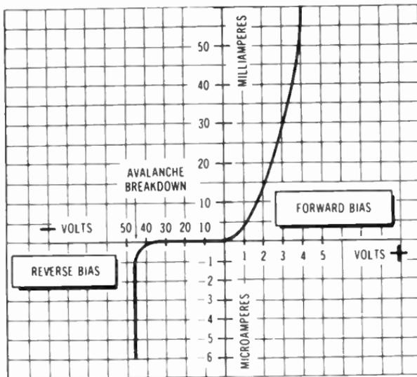
**Fig. 3-19.** Current-voltage characteristic curve.
