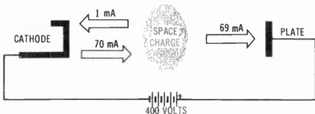
**Fig. 1-21. Plate 400 volts positive.**
