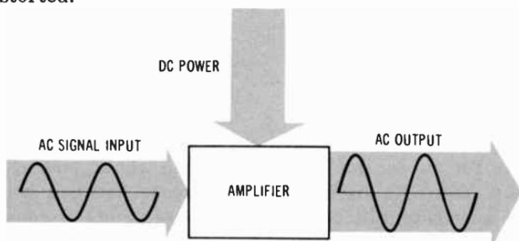
**Fig. 5-1. Basic amplifier principle.**
