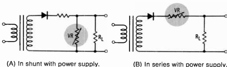
**Fig. 4-22. Voltage regulators represented as variable resistors.**
