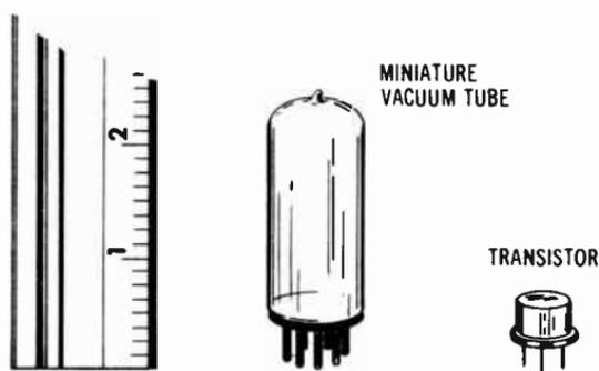
Fig. 3-1. Transistors are smaller than vacuum tubes.
