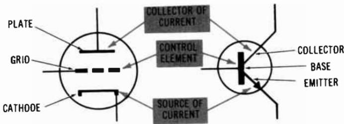
**Fig. 3-11. Comparison of transistor and triode tube.**
