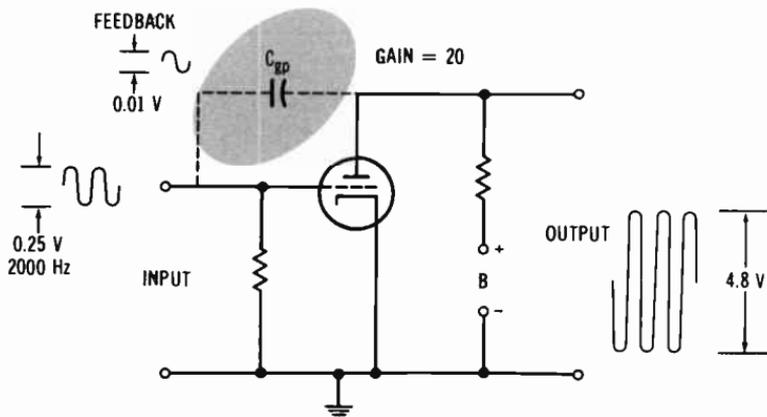
**Fig. 2-22. Effects of grid-plate capacitance.**
