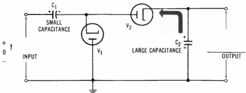
**Fig. 7-16.** A pulse-counter circuit.
