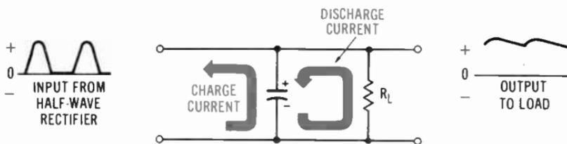
**Fig. 4-17.** Capacitive filter action.
