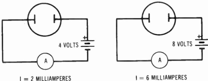
**Fig. 1-4.** Current depends on voltage between plates.
