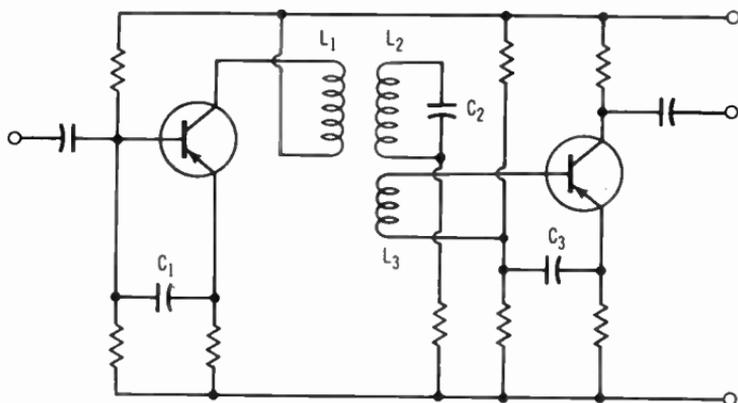
Fig. 6-13. Tuned transistor amplifier.
