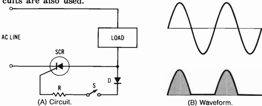
**Fig. 8-15.** Use of SCR to control ac load and waveform.
