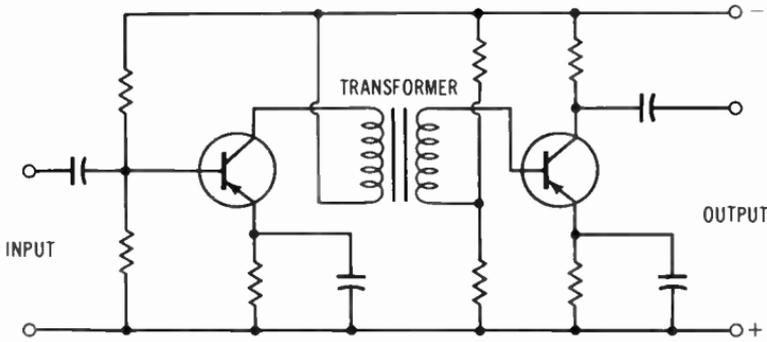
**Fig. 6-9. Transformer-coupled transistor amplifier.**
