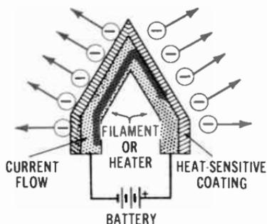
Fig. 1-6. Directly heated cathode.
