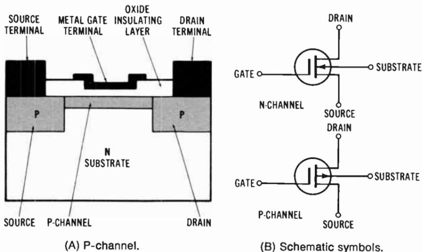
**Fig. 8-3. Depletion-type MOSFET.**
