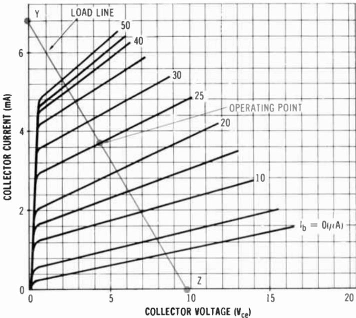
**Fig. 6-4.** Load line for transistor amplifier.
