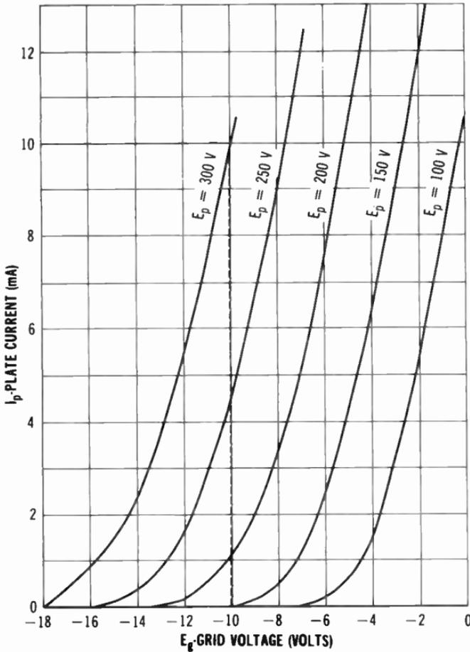
**Fig. 2-15. Ac plate resistance.**
