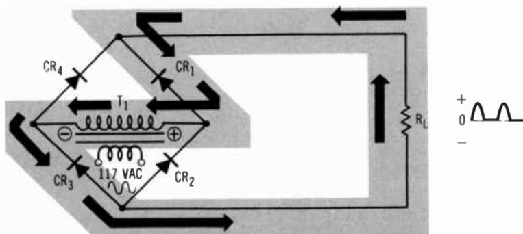
**Fig. 4-14. Bridge rectifier (positive half cycle).**
