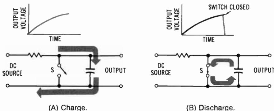
**Fig. 7-5. Sawtooth-generator action.**
