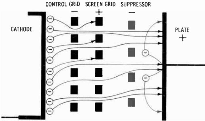
Fig. 2-27. Action of a suppressor grid.
