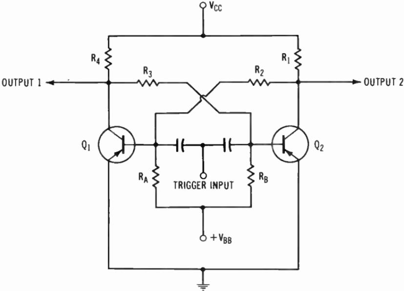
**Fig. 7-11. Bistable-multivibrator circuit.**
