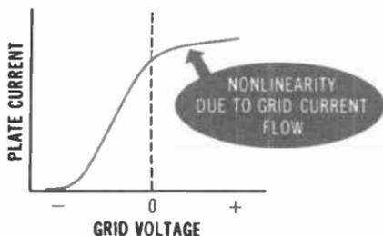
**Fig. 2-20. Effect of positive grid voltage.**
