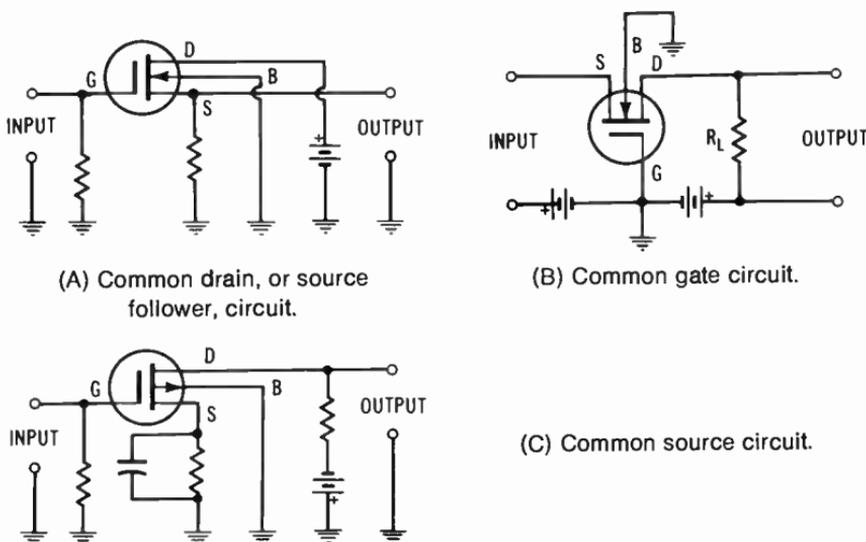
Fig. 8-6. Basic MOSFET circuits.
