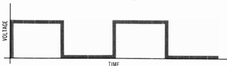
**Fig. 7-10. Theoretical output of a multivibrator.**
