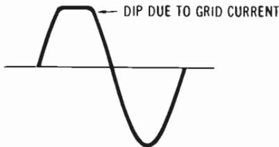
**Fig. 5-6. Distorted plate-current waveform.**
