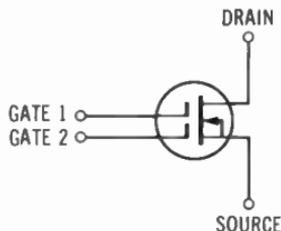
(B) Schematic symbol (includes substrate and case).
