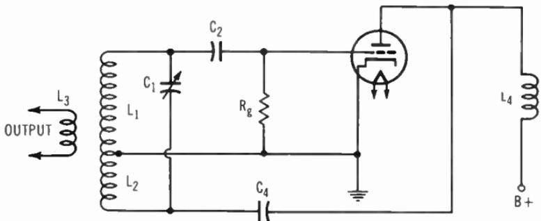
**Fig. 5-23. Shunt-fed Hartley oscillator.**
