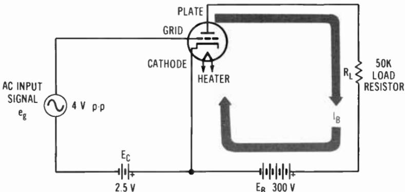
Fig. 5-3. Amplifier with input signal.
