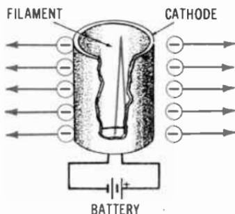
Fig. 1-7. Indirectly heated cathode.
