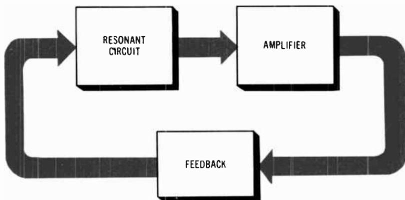
**Fig. 5-22. Feedback oscillator.**
