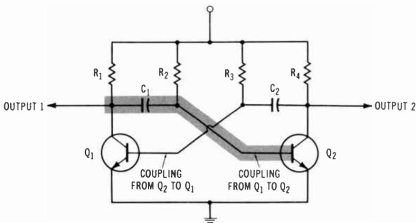
**Fig. 7-7. A multivibrator circuit with the output of  $Q_1$  applied to the base of  $Q_2$ .**
