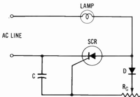
**Fig. 8-16.** SCR circuit for dimming a lamp by phase control.
