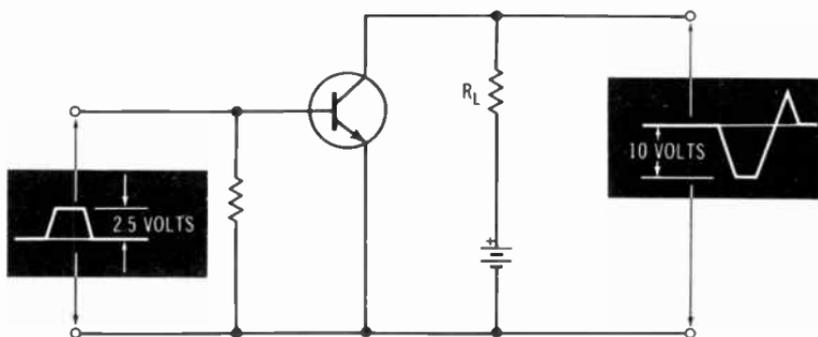
Fig. 7-3. A pulse-amplifier circuit.
