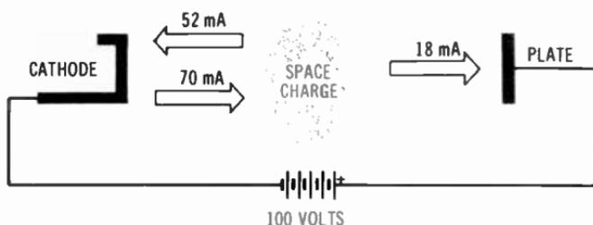
Fig. 1-19. Plate 100 volts positive.
