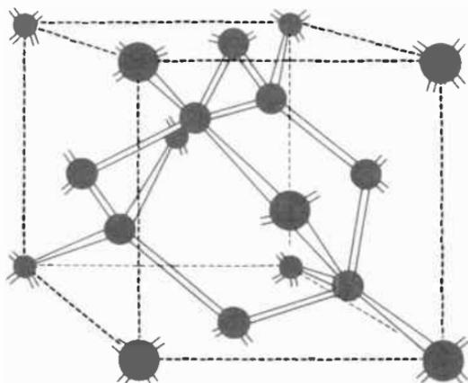
**Fig. 3-3. Semiconductor crystal lattice.**
