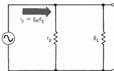
**Fig. 5-11.** Equivalent circuit using constant-current generator.
