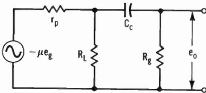
**Fig. 5-15. Low-frequency equivalent circuit.**
