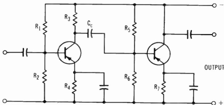
**Fig. 6-8. RC-coupled transistor amplifier.**
