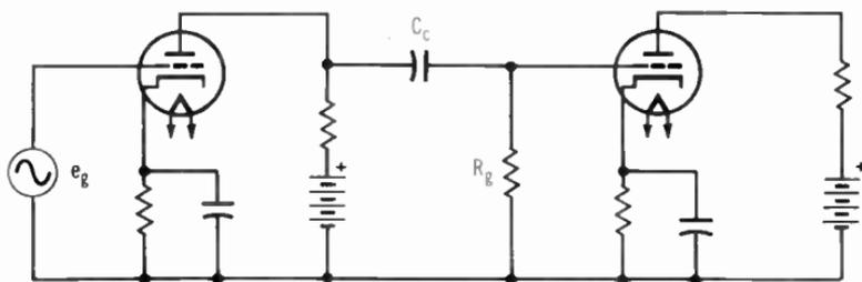
**Fig. 5-14. Resistance-capacitance coupled amplifier.**
