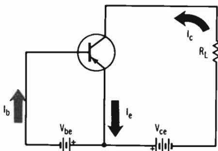
Fig. 6-1. Common-emitter circuit.
