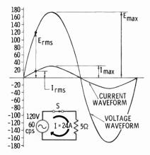
VOLTAGE AND CURRENT IN A BASIC AC CIRCUIT
