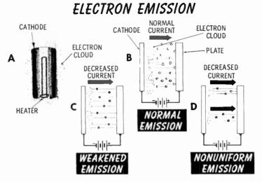
capability of the cathode has decreased after many hours of operation. A smaller quantity of electrons in the cloud causes a reduction in plate current. In figure D the cathode has weakened more in some areas than in others, resulting in a reduced number of electrons available for plate current.
