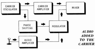
The oscillator generates a stable frequency which is simultaneously fed to an **amplifier** and a **phase-shifting** network. The phase-shifting stage shifts the frequency by a quarter of a cycle. The carrier and the shifted signal **a**re no longer in step. The amplified audio from the microphone is mixed with the out-of-phase signal in the **modulator**. The output of the modulator is a series of sine waves that vary in amplitude in **a**ccordance with the amplitude of the original sound.
