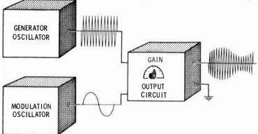
A gain control is normally provided to vary the amplitude of the output signal. To permit impedance matching of the signal generator with the circuit to which the test signal is fed, a cathode follower or similar impedance-matching stage is often employed. An attenuating network may be included to provide signals at a precise level of amplitude.
