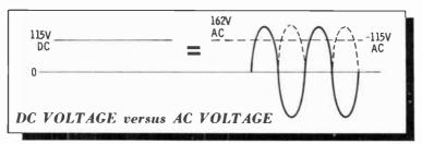
The peaks of 115 volts AC are actually 162 volts. A capacitor with a 150-volt rating will work well on 115 volts DC but not 115 volts AC. Standard practice is to use a capacitor with a working voltage about 50% higher than any voltage expected in the circuit.
