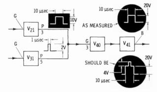
The first test should be made at the converging point (G<sub>3</sub> of V<sub>40</sub>). A comparison of the two output waveforms—the measured waveform and the correct waveform—indicates that the 1-microsecond pulse is missing. A proper deduction shows that the small pulse does not leave  $V_{31}$ , therefore it is correct to make a test at the output of  $V_{31}$ .
