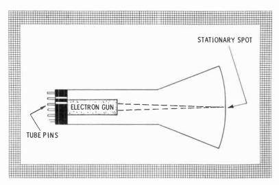
As you have learned, an electrostatic field can bend the path of a moving electron.
