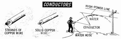
Some materials are better conductors of electricity than others. The availability of more free electrons in silver and copper, for example, makes them better conductors than iron or steel.
