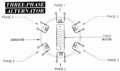
The three single-phase voltages of a three-phase alternator are usually 120 electrical degrees apart. As in the two-phase machine, it is possible to obtain single-phase voltages and also voltages between phases. The relationship
