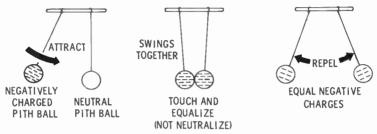
You can perform another experiment using an electroscope to illustrate the principle of attraction and repulsion between static charges.
