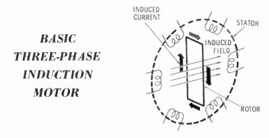
motor). This voltage, in turn, creates a large current in the rotor circuit. The current is large because the only resistance opposing it is the resistance of the wires. This high current in the rotor loop creates a magnetic field of its own. The rotor field and the stator field tend to attract each other. This situation creates a torque which spins the rotor in the same direction as the rotation of the magnetic field produced by the stator.
