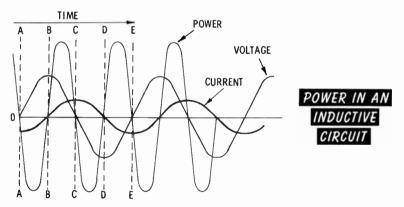
Between points B and C, both current and voltage are positive. If you multiply their values, it appears that power is being dissipated exactly as in a resistive circuit. Between points D and E, both current and voltage are negative, and again you have exactly the same situation as in a resistive circuit—power appears to be dissipated. But between points A and B and points C and D there is a situation that never exists in a resistive circuit.
