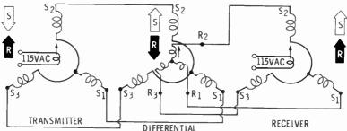
Zero position for a synchro differential is where  $R_2$  lines up with  $S_2$ . The stator windings of the transmitter develop a magnetic field in the differential stators as shown. This field induces an opposing differential rotor field which develops a receiver stator field in the opposite direction. The interaction of these fields when the transmitter and differential rotors are turned cause the receiver rotor to turn to the difference between the other two rotor positions.
