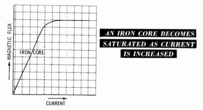
As the current in the coil and the flux in an iron core increase, a point is reached where the curve bends. A further increase in the current produces less and less of a flux increase until, finally, a further increase in current produces no additional flux. At this point the core contains as many lines of flux as it can possibly receive; it is said to be saturated.
