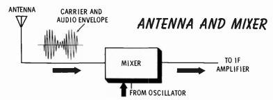
The Antenna and Mixer—Carrier frequencies from all stations within range of a receiver appear on the antenna of the receiver. When you turn the dial of your radio to a specific station, you adjust the electronic components of the **mixer** input so that the receiver will accept a particular carrier frequency and reject all others. The received carrier enters the mixer to be amplified. Some radios have, in addition, an **RF** amplifier between the mixer and antenna.
