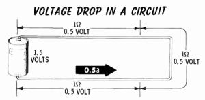
All of the source voltage is distributed proportionally across the resistance in a circuit. The voltage drop between any two points in a circuit can be determined by the ratio of the individual resistance to the total resistance of the circuit. The diagram, for example, shows a 3-yard length of wire connected to the terminals of a 1.5-volt cell. The resistance of the wire is one ohm per yard, or a total of three ohms for the circuit. Current for the circuit (E/R) will be 0.5 amp.
