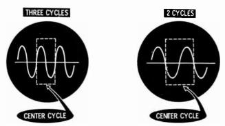
The center cycle of three cycles gives you an undistorted waveform in its correct phase. The center of a two-cycle presentation will appear inverted, but will be undistorted.
