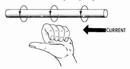
A16. In what plane do the magnetic lines around a current-carrying conductor lie?
