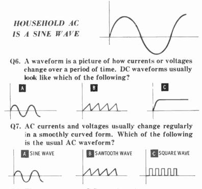
Q8. The most common DC waveform is a \_\_\_\_\_ \_\_\_\_. The most common AC waveform is a \_\_\_\_\_
