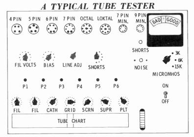
Q8. Will a dynamic tube tester test for emission? Q9. What are the four basic areas in a tube tester?
