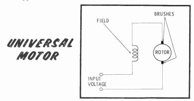
As you recall, a DC series motor will continue to turn in the same direction if the line connections are reversed. A series DC motor will therefore work on AC. In fact, a universal motor is simply a DC series motor whose windings and pole pieces are designed to operate efficiently with AC power.
