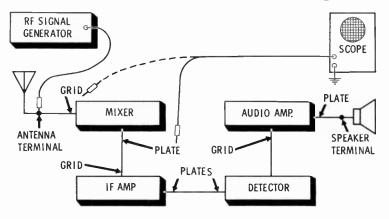
An oscilloscope is best for signal tracing. You can use a VTVM, however, to check for the presence of a signal. You must use an RF probe with the meter when testing at points where either RF or IF signals are present.
