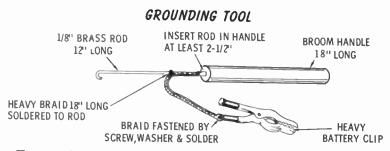
Fasten the clip of the grounding tool to the bare metal of the chassis. Touch the terminals or leads of the capacitor with the tip of the rod.
