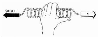
It was stated previously that the flux density is much greater in a block of iron than it is in air. Therefore, if an iron core is added to the current-carrying coil, the magnetic loops will concentrate through the core, increasing the flux density and strength of the electromagnet. The magnetic lines around the coil are called **induction lines**. Soft iron cores are used in electromagnets because of the high permeability of iron.
