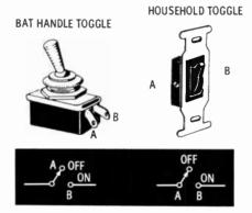
A toggle switch is an improved knife switch. It uses a spring-loaded mechanism to open and close the contacts.
