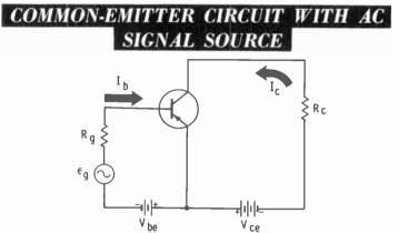
The voltage across load resistance  $R_L$  (which is a separate property of the circuit) is  $\Delta I_c R_L$ , where  $\Delta I_c$  is the signal current in the collector circuit.
