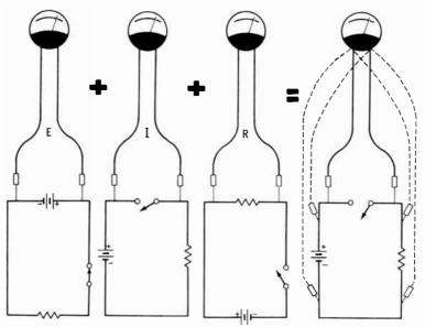
A multimeter can be used to measure voltage, current, and resistance within the limits of several ranges of values. From the technician's point of view, all multimeters consist of three basic sections—meter, circuitry, and front panel.
