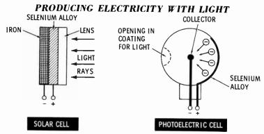
The photoelectric cell is often called a PE cell. A PE cell has many uses where a light beam can be broken, such as the automatic foul-line indicator on a bowling alley. Another application is an automatic lamp control. Here the PE cell is mounted so light from the sun will cause it to conduct and energize a relay. The energized relay turns the lamp off.
