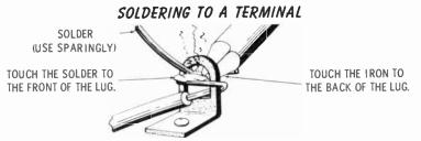
The iron should be applied to the back side of the terminal and held firmly against the wire. After a few seconds, touch the solder to the wire at the front of the terminal. If the solder readily melts, the connection is sufficiently heated. If the connection is not hot enough, remove the solder and continue heating until it is. Do not touch the solder to the iron.
