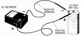
Voltage Measurements With a Multimeter
