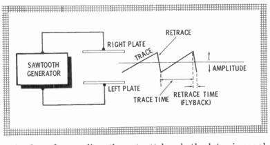
At the reference line, the potential on both plates is equal. Below the line the waveform makes the left plate more positive, and above the line the right plate is made more positive than the other. The waveform amplitude causes a uniform movement of the beam **across** the screen. The retrace line (trailing edge of the waveform) brings the be**a**m quickly back to the starting point.
