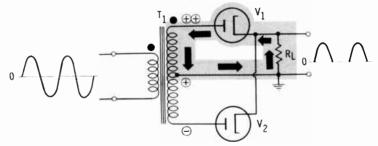
Two diodes are employed in this circuit. A special transformer is used with its center tap connected to one side of  $R_L$  and to ground. When the dot side of  $T_1$  is positive with respect to the center tap,  $V_1$  will conduct. The plate of  $V_2$ is connected to the other end of  $T_1$ , which is negative with respect to the center tap. Thus  $V_2$  will not conduct. The output of the circuit is as shown in the figure. Compare this output with that of the half-wave rectifier.
