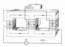
The two parts of the load winding are connected in series in such a way that the AC flux lines they induce in the center leg are equal and opposite, and thus cancel each other. This means there is no AC induced in the control winding, yet the control winding still exerts its influence over the load circuit.
