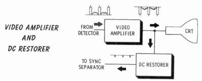
Video Amplifiers—The output of the detector is a relatively weak signal, not strong enough to cause a reproduction of the picture. Video amplifiers are therefore required to achieve the necessary signal amplitude. These must be wide-band amplifiers because the frequency content of the picture signal covers a wide frequency range.
