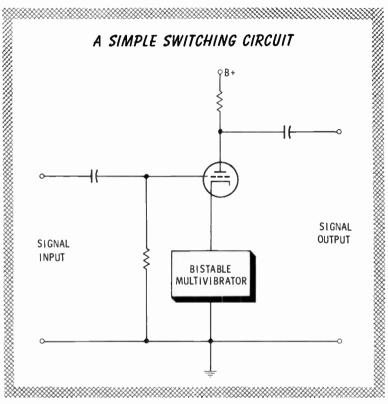
a large positive voltage to the cathode. This has the same effect as making the grid negative, and the tube is cut off. Another pulse to the multivibrator causes it to change states again, the cathode of the tube is returned to its operating voltage and the tube is able to amplify.
