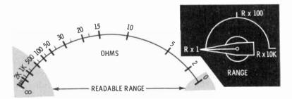
Q25. Using the above diagram, which range setting should be used to measure an estimated 1,500 ohms?
