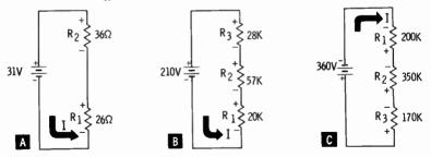
Q8. How does the voltage drop across the 36-ohm resistor affect the amount of voltage drop across the 26-ohm resistor in (a) above?
