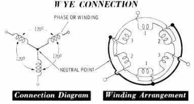
The neutral point is normally grounded (connected to the earth or a large mass of metal), in which case the wye connection is as shown below. This system is called a threephase, four-wire wye connection.
