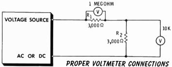
The internal resistance of a voltmeter is normally very high. The higher it is, the greater the meter accuracy.
