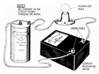
CONNECTING AN AMMETER IN A CIRCUIT
