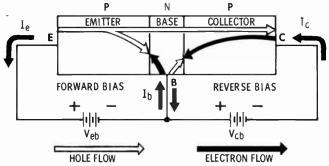
the emitter-base junction. In a similar fashion, a battery whose negative terminal is connected to the P-type collector will reverse-bias the collector-base junction.
