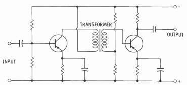
Suppose the output impedance of the first stage is 25K and the input impedance of the second stage is 1,000 ohms. What turns ratio would the coupling transformer need? In a transformer, the impedance ratio is equal to the square of the turns ratio. The required turns ratio may be calculated as follows:
