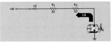
Q30. What is the resistance of the motor when the switch is in the MED position?
