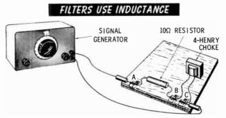
Voltages can be measured between points A and C, A and B, and B and C. Pick about 12 equally spaced frequencies. Using each as an input, measure and record both the input and output voltages.
