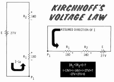
The sum of voltages in the loop from point 1 back to point 1 is zero. The current was assumed to be in the correct direction, and  $I_T$  and the IR drops were calculated properly.
