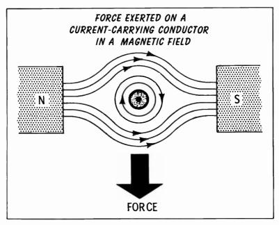
The magnetic field around the conductor in the above figure is clockwise. The current appears to be coming out of the page. The direction of the magnetic field of the permanent magnet is from the north-seeking pole to the southseeking pole, or from left to right in the figure above. Notice that the lines above the conductor and the lines around the conductor are going in the same direction, reinforcing the field above the electron path. Below the conductor the fields are opposing each other.
