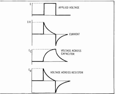
The voltage across the capacitor will start at zero and will build up smoothly until it equals source voltage E. The voltage across the resistor will, at any instant, equal the difference between the source voltage and the voltage across the capacitor; it will also be a spike as shown.
