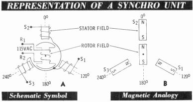
$S_1$ ,  $S_2$ , and  $S_3$  are the three stator windings of a synchro. They are physically displaced  $120^{\circ}$  apart, or at equal distances around a circle. The rotor is free to rotate and is said to be positioned at  $0^{\circ}$  when the axis of the rotor is in line with the axis of winding  $S_2$ , as shown in part A.
