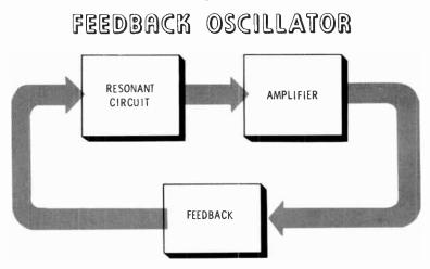
The type of oscillator discussed in this chapter produces an output waveform that is considered to be a sine wave. An oscillator producing such an output is sometimes called a sinusoidal oscillator. You will learn about nonsinusoidal oscillators later in this volume.
