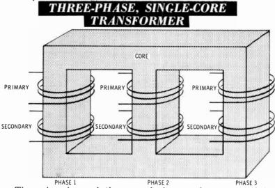
The primaries and the secondaries can be connected in any combination of delta and wye. For example, the primaries can be wye-connected and the secondaries delta-connected, or vice versa. Or both the primaries and the secondaries can be wye- or delta-connected.
