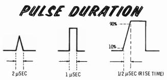
Another way to examine the response of a scope is in terms of **rise time**. The rise time is the time between the 10% and 90% amplitude points on the leading edge of a pulse. The minimum rise time that a scope can reproduce is determined mainly by the charge time of certain capacitances in the scope.
