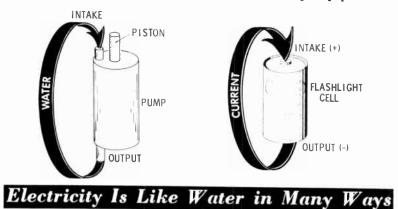
both the **pressure** and the **water** to cause a flow through the **water system**. A voltage source provides electrical pressure (voltage) and current (electrical equivalent of water) to cause a flow through an electrical circuit.
