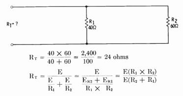
To find the total resistance of a parallel circuit containing resistors of equal value in parallel, all that needs to be done s to divide the value of one of the resistors by the number of resistors in parallel.
