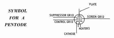
The fifth element of the pentode is called a suppressor grid. This element is usually connected internally to, and has the same potential as, the cathode. In other words, the suppressor grid is negative with respect to the plate. Spacing between the turns of wire of the suppressor grid is wide enough for plate current to pass through, but yet sufficiently close enough to repel the negative secondary electrons back to the plate.
