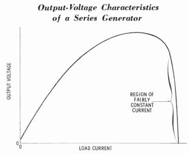
As more current is demanded (within practical limits) from a series-wound DC generator, the output voltage increases. When the practical limit of current is reached, a further demand has a reverse effect. The practical limit is reached when the magnetic field strength reaches its maximum value.
