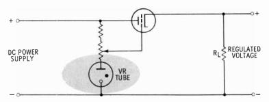
A vacuum-tube circuit can be used as a series voltage regulator. The current passing through the tube from cathode to plate depends on the grid bias. Another way to say this is that the resistance of the tube depends on the grid bias. Therefore, by varying the voltage on the grid, the tube resistance can be changed as necessary.
