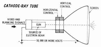
The basic construction and connections of a CRT are illustrated above. At the left end is shown an electron gun which shoots a narrow stream of electrons toward the screen. To speed the electrons on their way, the inner surface of the flared portion of the tube has a conductive coating energized with a voltage that is several thousand volts positive with respect to the electron source.
