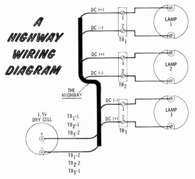
TB1 is the abbreviation for terminal board 1. TB2-1 (terminal 1 of terminal board 2) is positive and therefore connected to the positive pole of the cell. Although only two wires are shown connected to the cell, there are actually three at each pole as indicated by the TB listings.
