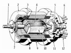
1 - ROTOR SHAFT 2 - UPPER END CAP 3 - STATOR COILS 4 - ROTOR COILS 5 - BEARING 6 - ROTOR LEADS 7 - BEARING 8 - MOUNTING FLANGE 9 - SHELL 10 - ROTOR 11 - LOWER END CAP 12 - STATOR LEADS
