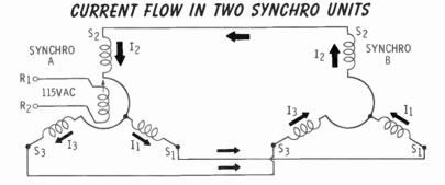
rotor in the left-hand synchro unit, maximum voltage is developed across  $S_2$  and lesser voltages across  $S_1$  and  $S_3$ . The voltages are such that induced current  $I_2$  is equal to the sum of  $I_1$  and  $I_3$  induced in  $S_1$  and  $S_3$ , respectively. Identical currents are flowing through the respective stators of synchro B. As a result, the voltages developed across the synchro-B stator windings are equal to those across the respective windings of synchro A.
