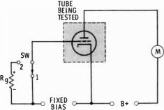
the meter reading if very little or no gas is present. However, if positive gas ions are present, current will flow through  $R_{\kappa}$  and develop a positive polarity from the grid to cathode. Bias will be reduced, plate current will increase, and an increased reading of the meter will be noted.
