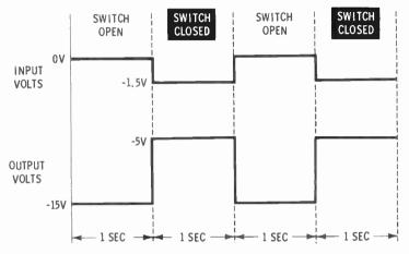
With the switch open, the input registers 0 volts and the output -15 volts. With the switch closed, the input changes to -1.5 volts and the output to -5 volts. The same readings occur each time the switch is opened and closed.
