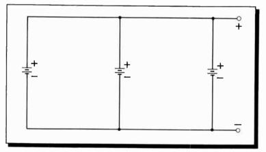
Still another example of a parallel circuit is the filament circuit for the vacuum tubes used in automobile radios. The filaments are all connected in parallel, and either 6 or 12 volts is applied to each. The tubes have either 6- or 12volt filaments, depending on the type of battery in the automobile.
