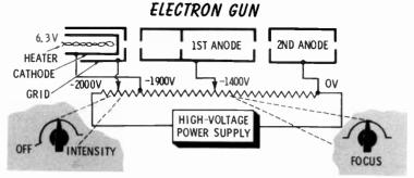
required, the other electron-gun elements are operated at negative potentials. The control grid normally operates near 2,000V negative, 90 to 100V more negative than the cathode. The first anode (focusing) can be maintained between -1,200 and -1,600V. These voltages are typical but vary among instruments.
