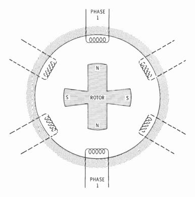
Now look at the figure above. This machine has four poles on the rotor. Four poles pass each winding during each revolution. Therefore there are two complete cycles of current in each winding for each revolution of the rotor. A machine with **eight** poles will have **four** complete cycles of current in each winding for each revolution of the rotor, etc. The formula relating the frequency to the speed and to the number of poles in a synchronous generator or motor is as follows:
