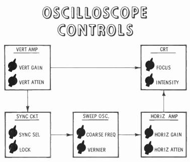
Q71. State the purpose and how it is accomplished for each of the following controls:
