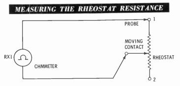
If the rheostat contact is at terminal 1 and the meter has been properly zeroed, the resistance reading should be zero ohms. Leaving the probes connected, the meter will show the gradual increase of resistance as the contact is moved toward terminal 2. At terminal 2 the total resistance of the rheostat will be read on the meter scale.
