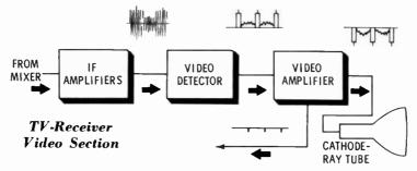
IF Amplifiers—The output of the IF amplifiers contains the video signal and is fed to the video detector, as shown in the diagram.
