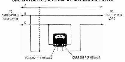
is taken with one voltage lead connected to line B. The lead is then moved to line A, and another reading is taken. The sum of the readings gives the total power. A power factor less than 0.5 produces the same result in the one-wattmeter system **a**s in the two-wattmeter system.
