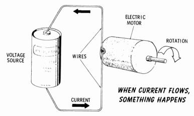
Current flows through the wires of an electrical or electronic device in much the same way water flows through pipes.
