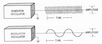
Amplitude Modulation—There are several types of modulation. Amplitude modulation is the form used in standard broadcast transmissions (535 to 1,605 kc) and is defined as the process by which the carrier is varied in amplitude to resemble the amplitude and frequency of the intelligence.
