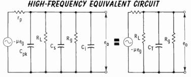
In the high-frequency range, three unwanted capacitances become important. They are the plate-cathode capacitance  $(C_{pk})$ , the stray capacitance of the wiring  $(C_s)$ , and the capacitance of the input circuit of the second stage  $(C_i)$ . Since the equivalent circuit is a parallel one, all three capacitances may be combined into a total stray capacitance  $(C_T)$ .
