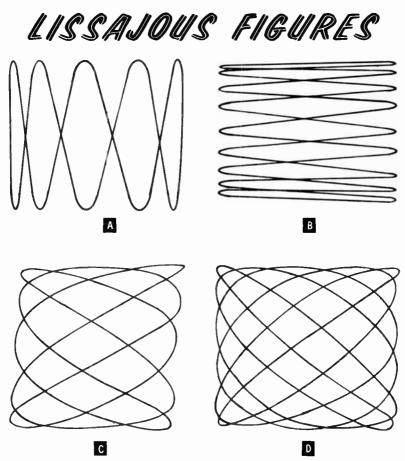
Q82. If the standard frequency is 180 cps, what is the frequency of the unknown in each of the above Lissajous patterns?
