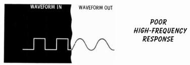
It depends on the application of the pulse whether a particular circuit is good enough or not. In a telegraph system, it may only be necessary to detect the presence or absence of pulses with no concern as to their exact shape. So, the high-frequency response of the circuit would not be critical.
