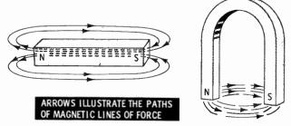
The lines formed by the magnetic loops are called magnetic lines of force. The area occupied by these lines is called the magnetic field. The magnetic field is the induced energy surrounding the magnet or the space through which the influence of these magnetic lines of force can be measured. The strength of the magnetic field is measured by determining the number of magnetic lines of force per unit area surrounding the magnet.
