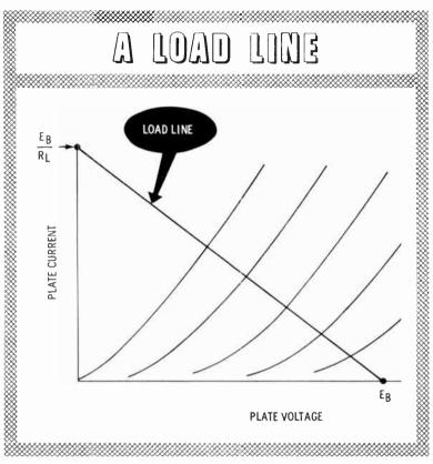
Changing the plate-supply voltage changes the position of the load line. Changing the load resistance changes the slope of the load line.
