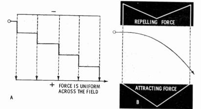
line? If this were true, an electron traveling between the plates with sufficient velocity to pass through the field would cover the distance in a stair-step pattern, as in A above. It is known that the path of an electron through a force field is curved, as in figure B. Force does not exist in distinct beams; it is continuous and uniform across the field. However, it is easier to talk about the field in terms of imaginary lines.
