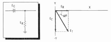
The values of C and R are selected so that the current in the circuit leads the applied voltage  $(E_T)$  by an angle of 60°. The voltage  $(E_R)$  across the resistor also leads the applied voltage by 60°;  $E_R$  is the output voltage of the RC combination. Three RC combinations produce a phase shift of 180°.
