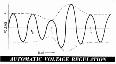
returns to normal. The time required to return to normal varies from a few cycles, as shown in the figure, to a few seconds.
