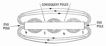
The poles between the ends of a magnet are called **consequent poles**. Notice there are magnetic fields existing between the consequent poles and the end poles. These fields are the same as the field that exists between the end poles. The magnetic lines of force leave a north-seeking pole and enter a south-seeking pole.
