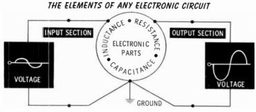
You might think that the symbol for a vacuum tube or transistor does not look like an inductance, capacitance, or resistance. You are correct. However, the way a vacuum tube or a transistor operates can be explained by how it reacts in terms of resistance, inductance, or capacitance when current is passing through it or when voltage is applied to it.
