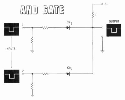
the negative battery terminal for the duration of the input pulses. Therefore, to produce an output, pulse 1 AND pulse 2 must be present. The condition necessary to produce an output from this AND gate is that two negative input pulses must occur at the same time.
