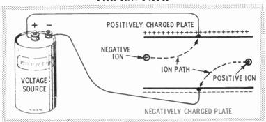
atom may be moved. How about the ion, could it be caused to travel in a directed line? Yes. If positive, it will be repelled by another positive force or attracted by a negative force.
