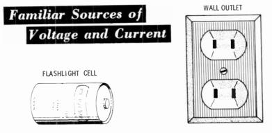
The battery shown in the illustration is more properly called a **cell**. A cell was originally considered to be a storage device. Cells, such as those used in a flashlight, develop 1.5 volts each. A **battery**, such as the 6- or 12-volt source in an automobile, is constructed of two or more cells. However, through long usage, a cell is often called a battery.
