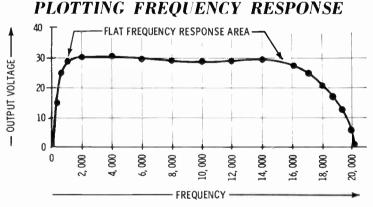
tings for readings in the rising and falling portions of the curve should be made in multiples of 500 cps. Intervals of 2,000 cps are satisfactory along the top part of the curve.
