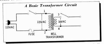
The lines between the primary and secondary windings indicate an iron core which provides an easier path for the magnetic field through the coils.
