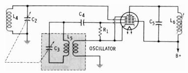
IF Amplifier—The IF stage consists of two tunable transformers separated by an amplifier. More sensitive receivers may have two amplifiers and three transformers. Each of the coils in the transformers has a metallic core that can be adjusted to give the value of inductance necessary to make the respective tank circuits resonant at 455 kc. By this method, only the difference frequency from the mixer or
