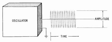
Signal generators are classified in accordance with the frequency range of their oscillators. Audio-frequency (AF) generators usually cover a range from about 20 to 20,000 cps. Radio frequency (RF) generators begin at 20,000 cps and end at several thousand megacycles.
