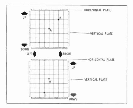
In the top diagram above, position A of the beam is in the center. It can be moved to position B by going up two units and then right two units. Movement of the beam is the result of the simultaneous action of both sets of deflection plates. The electrostatic field between the vertical plates moves the electrons up an amount proportional to two units at the screen. As the beam passes between the horizontal plates, it is moved to the right an amount proportional to two units at the screen.
