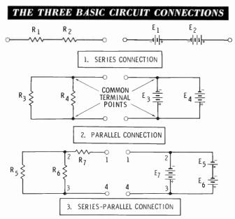
The illustration shows the three different connections and also the accepted method for labeling components. R stands for resistor; E designates a voltage source. Numbers are used with the letters to identify a specific component.
