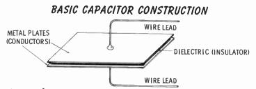
This basic principle is elaborated upon to produce the shapes shown on the opposite page. For example, the plates of the variable capacitor are curved and exposed. Since air is an insulator, it forms the dielectric.
