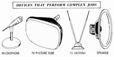
Many complex jobs are performed by combinations of simple devices. That is, two or more simple devices work together to perform a complex job. These devices fall into three categories: (1) input converters, (2) processing devices, and (3) output converters.
