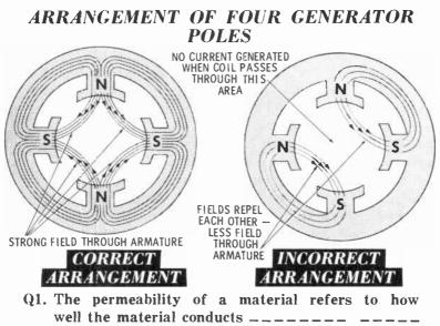
Q2. Magnetic pole pieces are placed in a generator so that poles of (the same, opposite) polarity are next to each other.
