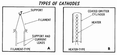
Part A shows a filament-cathode. The single wire serves as both the filament and cathode; it is made of a material (normally coated or uncoated tungsten) that emits electrons when hot.
