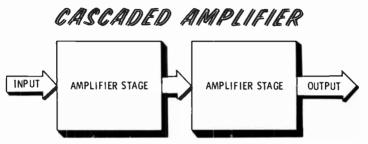
In a multistage amplifier chain, voltage amplifiers are generally used for all but the output stage. In this way only very small currents are handled. The signal is gradually developed to a higher voltage but with very little power. Only in the last stage is the signal converted into the necessary power output.
