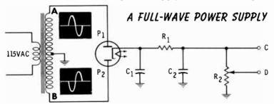
The transformer steps 115 volts AC up to the value desired on the secondary. Each terminal of the secondary is connected to a separate plate of the twin diode. The secondary winding of the transformer is center-tapped to ground.
