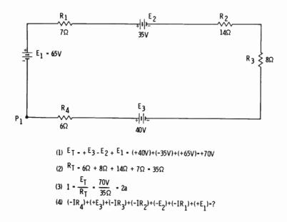
Calculating the IR drop across each resistor:  $IR_4 = 12V$ ,  $IR_3 = 16V$ ,  $IR_2 = 28V$ , and  $IR_1 = 14V$ . Kirchhoff's application (4) above: -12V + 40V - 16V - 28V - 35V - 14V + 65V = ? 105V - 105V = 0V.
