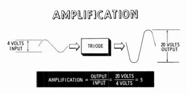
In the above figure, the amplification is 20 volts divided by 4 volts, or 5.
