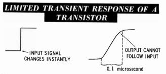
travel from cathode to plate in a vacuum tube is no longer negligible. For the same reason, the time for holes or electrons to diffuse from emitter to collector in a transistor must be considered.
