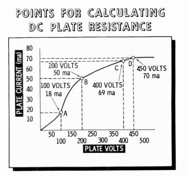
To see how the DC plate resistance varies with plate voltage, calculate  $R_p$  at each of the points marked on the graph. The calculations yield the following results:
