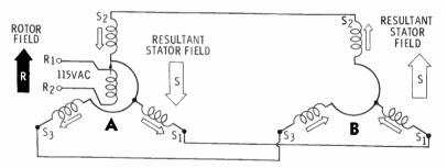
In synchro A, the direction of the developed rotor field is up, as shown. The induced magnetic fields in the individual stators are along their axis but in a downward direction. The combination of all the stator fields produces the resultant field shown by the large white arrow. It is an induced field and is directly opposite to the rotor field.
