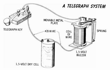
When the telegraph key is closed (pressed down), current flows from the battery through the coil of wire. The resulting magnetic force causes a movable metal plate to be attracted to the soft-iron core of the coil, producing a buzzing sound. In this manner dots and dashes (short and long buzzes) are transmitted.
