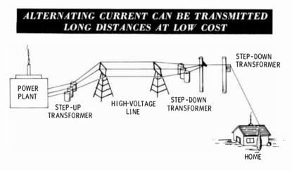
Alternating currents are generated in very large quantities in power plants. The electricity used in your home comes from a power plant. The total current capacity of a power plant can reach several thousand amperes at 4,160 volts. Another source of AC, usually for specialized purposes, is the oscillator. The current output of an oscillator is quite small, usually in the milliampere range. Oscillators are used primarily as signal sources in electronic equipment.
