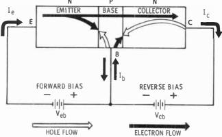
ion of  $V_{eb}$  and  $V_{eb}$ . The major portion of  $I_e$  is due to the electron flow from emitter to collector. Notice that current low in the base is due to both electron and hole flow. Thus here are current flows indicated in both directions.  $I_b$  is the lifterence between these two currents.
