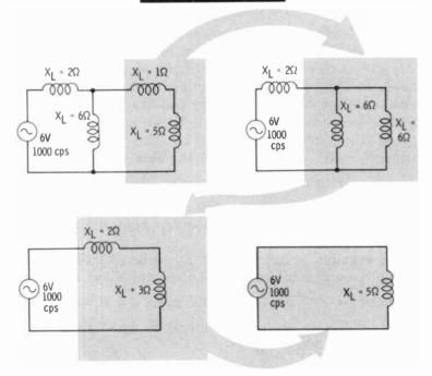
Q6. What is the equivalent  $X_L$  in the following circuit?
