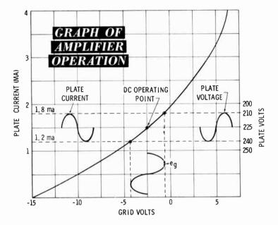
Since the plate-battery voltage is 300 volts, the voltage between plate and cathode will be 300 minus the load-resistor voltage drop (neglecting the small battery resistance). Thus, the plate voltage has a quiescent (no-signal) value of 225 volts, and with the 4-volt (peak-to-peak) input signal it swings between 210 and 240 volts.
