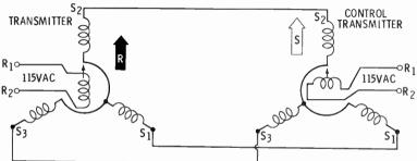
The rotor of a control transformer is at zero position when it is at right angles to  $S_2$  as shown in the diagram above. The induced stator field in the CT will be in the same direction as the rotor field of T. In the positions shown, no voltage will be produced between  $R_1$  and  $R_2$  of the CT.
