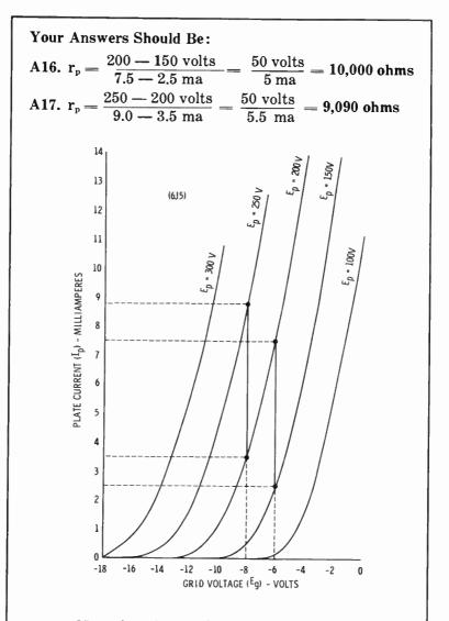
Note that these values (9,280, 10,000, and 9,090 ohms) are all fairly close to each other. When compared to the changes in  $R_p$  (from thousands of ohms to hundreds of thousands of ohms), the AC plate resistance  $(r_p)$  may be considered almost a constant for a particular triode.
