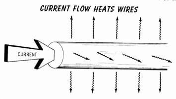
given off by a wire is determined by the type of metal in the wire and the quantity of current that is forced through it. A large current produces more heat in the same size and type of wire than a smaller current. If the current is the same, a smaller wire gives off more heat than one that is larger in diameter. Also, some metals produce more heat than others as the result of current flow.
