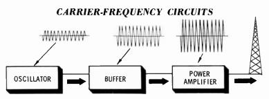
The Oscillator—The purpose of the oscillator is to generate a stable RF signal. The resistance, inductance, and capacitance that make up its input circuit are such that they will not allow the vacuum tube in the oscillator to amplify any other signal but that of the desired frequency. The stable-frequency, low-amplitude output of the oscillator is shown above.
