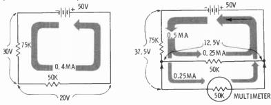
A Multimeter Loads a Circuit
