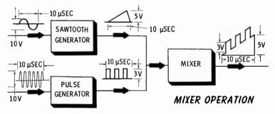
The sawtooth and pulse generators have sine-wave inputs of different frequencies. The input frequency of the pulse
