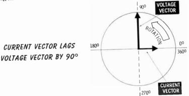
Inductance, unlike resistance, consumes no power. When the current in the circuit is increasing, inductance takes energy out of the circuit. It converts this energy into a magnetic field. When the current in the circuit is decreasing, however, this magnetic field collapses, and all the energy
