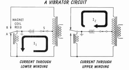
The vibrating reed causes the current to flow through first the lower section of the transformer primary and then the upper section. This is very much like having an alternating current flowing in the primary. This action causes an AC voltage to be induced in the secondary of the transformer. The voltage is not a sine wave, however, but has a generally rectangular shape. Filtering action can smooth out the waveform.
