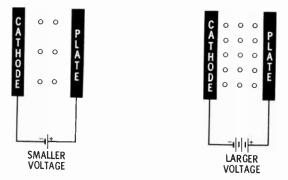
CURRENT FLOW IS AFFECTED BY PLATE VOLTAGE
