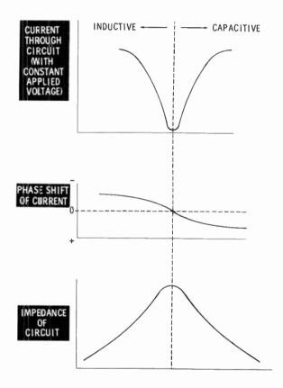
But, because one of the currents leads the applied voltage by  $90^{\circ}$  and the other lags the voltage by  $90^{\circ}$ , the two currents are  $180^{\circ}$  out of phase with each other. This means that they cancel (add up to zero).
