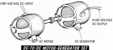
A shunt or compound DC motor is best because it has relatively constant speed for varying loads. The output voltage of the generator depends on the speed. A shunt or compound DC generator is best suited for use in M-G converters because it has good voltage regulation for varying loads.
