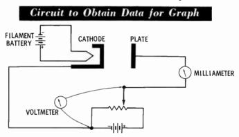
arm of the variable resistor is changed, read the voltage and the current. After recording several of these readings, plot a graph similar to the one on page 36.
