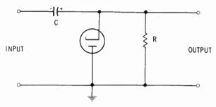
case the entire waveform is shifted above the zero level to clamp the bottom of the waveform to zero.
