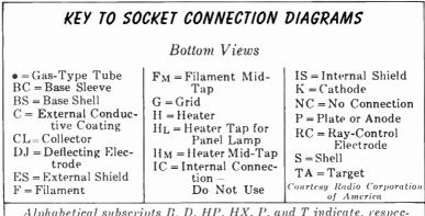
Alphabetical subscripts B, D, HP, HX, P, and T indicate, respectively, beam unit, diode unit, heptode unit, hexode unit, pentode unit, and triode unit in multi-unit types.
