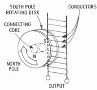
Q60. Will an automobile generator produce more electricity when the car is traveling at 60 mph or at 20 mph?
