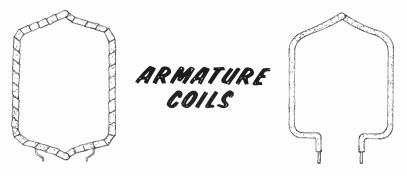
Sometimes the distance between the two sides of an armature coil is not equal to the distance between the adjacent magnetic poles. When this distance is less than the pole pitch, the coil is called a **fractional-pitch winding**.
