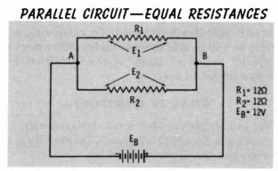
Disregarding the voltage drop in the conductors, the voltage difference between points A and B (above) will be that of the source (12V). The current through  $R_1$  and  $R_2$  will be 1 amp each, or a total circuit current of 2 amps. Since the resistances and currents in both legs are equal,  $E_1$  is equal to  $E_2$ . Now divide one resistance into four equal parts.
