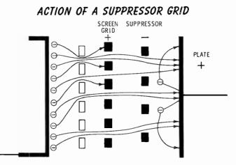
The addition of the suppressor grid between the plate and screen grid also serves to reduce the interelectrode capacitance between the plate and control grid still further. This results in a tube with even better high-frequency performance than the tetrode. Pentode amplification factors are in the order of 1,200 to 1,500 (as opposed to 200 or 300 for a tetrode).
