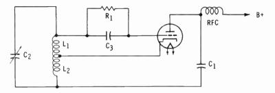
frequency of the tank is adjusted by  $C_2$ . The RFC (radiofrequency choke) in the B+ line prevents AC on the plate from entering the B+ source.  $R_1$  and  $C_3$  establish grid bias. Audio Oscillator—The major purpose of the audio oscilla-
