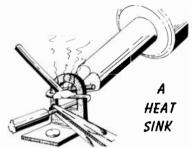
the illustration. The iron in the pliers dissipates most of the heat before it can travel further down the wire.
