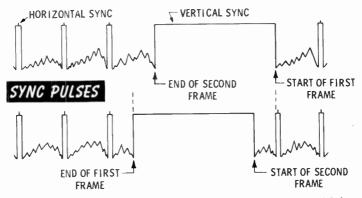
The above illustration shows the comparative widths of the horizontal and vertical sync pulses and the relative starting times of the first and second frames. The sync pulses are removed from the complete video waveform and sent to the sync separator.
