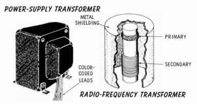
Most transformers are designed to transfer power. Others, however, are built to transfer only signal voltages.
