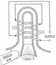
How can you make a thermocouple? One way is to twist the ends of an iron and a copper wire together. Heat the twisted junction over a flame. If the free ends are connected to a milliameter, a small current reading may be observed.
