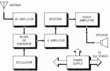
The purpose of the radio receiver is to amplify the weak signal of a selected RF carrier and its audio modulation, remove the audio component from the carrier, and then amplify the audio so that it can be heard clearly on a speaker.
