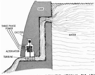
HYDROELECTRIC GENERATING PLANT
