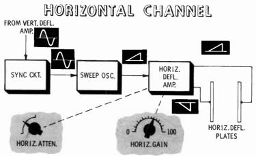
The sync circuit sends a sample of the observed waveform to the sweep oscillator for synchronization with the generated sawtooth wave. The sawtooth is then amplified by the horizontal-deflection amplifier and applied to the horizontal plates.
