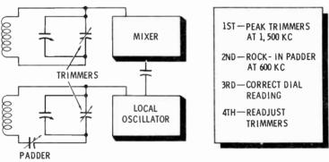
Now, set the generator and receiver dials to 600 kc. Rockin the padder tuning by making the same adjustment at several settings on either side of the 600-kc dial reading. The setting at which the highest output reading is noted is the true 600-kc position. Adjust the receiver dial pointer to indicate 600 kc. Recheck the trimmers for maximum output again, first at 1,500 kc and then at 600 kc. If no change is evident, tuning is completed.
