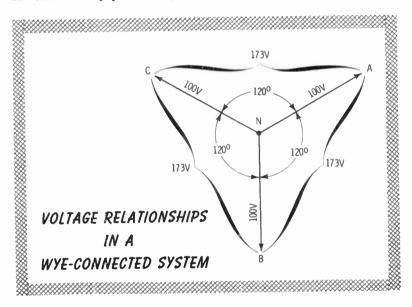
The phase-to-phase voltage is the between-the-lines voltage, or simply the line voltage. The voltage between a line and the neutral is the phase voltage. Because of the phase relationships, the line voltage is 1.73 times the phase voltage in a wye-connected system if the phase voltages are equal.
