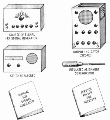
There are six items shown above, and each is important. A few other common hand tools are also needed to remove the receiver from the cabinet. An insulated screwdriver is used to prevent shorting or detuning of circuits while they are being adjusted.
