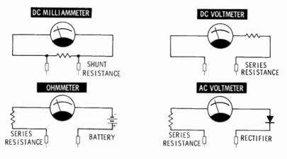
Meter-Circuit Components—The figure on the opposite page shows that multimeter circuitry requires series and/or shunt resistances, a battery for measuring ohms, and a diode for limiting current direction when measuring AC voltage. To obtain different ranges for volts, amps, or ohms, resistances of selected values must be used in the circuit. The circuits are connected to front-panel controls that provide means of selecting the desired function and range.
