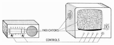
Many radio receivers have two output indicators, a speaker and a light (usually illuminating the dial); the receiver also has at least two controls. The change from desired performance can be registered in many ways—hums, squeals, squawks, low volume, two stations instead of one, or no sound at all. The light is either on or off.
