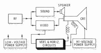
The schematic diagram included in the technical manual or servicing folder for the receiver should be used in locating the output test point of the probable faulty function. You will find that a schematic diagram will be your most valuable single item for troubleshooting.
