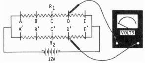
How much voltage would you measure between points D and D'? The answer is zero volts. The potential difference between A and D is 9V; this is equal to the difference between A' and D'. Therefore, no potential difference exists.
