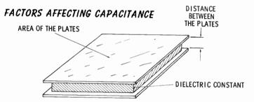
Capacitance (farads) is determined by three factors:
