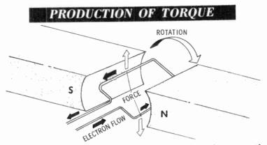
causes the magnetic field below the conductor to be strengthened and the field above to be weakened. This results in an upward force on the left side of the coil and a clockwise direction of rotation. The flow of current into the right side of the coil causes the magnetic field below the conductor to be weakened and the field above to be strengthened. This results in a downward force on the right side of the coil and a clockwise rotation.
