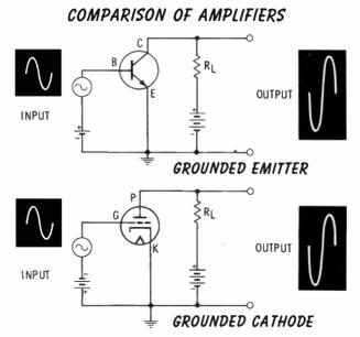
tively. A phase reversal of  $180^{\circ}$  occurs between the input and the output. This phase reversal will be explained in the chapter on triode amplifiers. The common-emitter amplifier has these characteristics:
