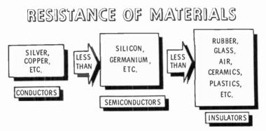
Most metals contain atoms that release electrons very easily. These materials, therefore, offer the least resistance to current flow. Insulators have the greatest resistance because their atoms resist the release of electrons. The in-between materials are neither good conductors nor insulators. Among these are certain materials, the **semiconductors**, from which **transistors** are manufactured.
