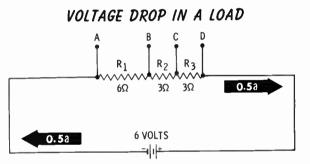
Normally, the relatively small voltage drop of conductors is disregarded since the wire resistance is usually a very small fraction of the total load resistance. The tapped resistance in the diagram above has a total of 12 ohms with a total of 6 volts (from the source) applied across it. A current of 0.5 amp flows through each portion. The voltage (IR) drop between terminals A and B will be 3 volts in accordance with Ohm's law, resistance ratio, or a voltmeter measurement.
