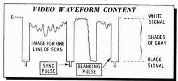
signals fed to the cathode-ray tube control the number of electrons striking the **fluorescent** screen. The fluorescent material on the screen gives off light in proportion to the number of electrons that strike it.
