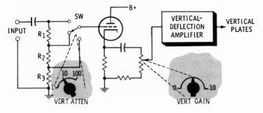
top tap of the switch in the schematic. The full voltage of the input is fed to the grid of the cathode follower. Attenuation equals 1/10 in position 10.  $R_1$ ,  $R_2$ , and  $R_3$  are selected so that 1/10 of the input voltage will arrive at the grid. Position 100 provides an attenuation of 1/100.
