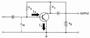
The base-bias voltage is obtained from resistor  $R_b$ . The resistance of  $R_b$  is  $\frac{V_B - E_{be}}{I_b}$ . Since  $E_{be}$  is usually small compared to  $V_B$ , it can be disregarded when determining biasing voltages. So  $R_b = \frac{V_B}{I_b}$ .  $I_b$  is the chosen quiescent base-current value.  $R_b$  is usually between 100K and 1 meg.
