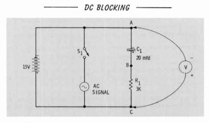
To develop a voltage across  $R_1$ , current must flow through it. At the instant the circuit is connected, current flows from the lower plate of the capacitor through  $R_1$  and the battery to the upper plate. In 5 RC times, the capacitor is fully charged and current stops flowing.
