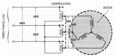
The autotransformer method is shown above. The group of autotransformers used to limit starting current is called a **compensator**. When the motor reaches running speed, the compensator is bypassed and the full voltage is applied. The autotransformer will dissipate almost no power. (Only a negligible amount will be dissipated by the resistance of its windings.)
