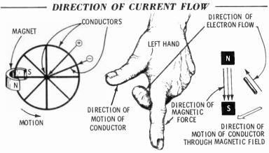
will be. Another factor is the speed at which the lines of force are cut by the wires. The faster the relative motion between the two, the greater the force generating electron flow will be. Finally, the greater the number of wires cutting through the magnetic field, the greater will be the number of electrons that flow.
