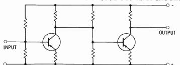
cannot be amplified when capacitors or transformers are used for interstage coupling. But amplifiers can be coupled without using capacitors or transformers. Connecting the collector of the first stage directly to the base of the next stage, as shown above, is known as **direct coupling**. Such amplifiers are called **direct-coupled amplifiers**, **direct-current amplifiers**, or simply **DC amplifiers**.
