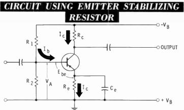
Capacitor  $C_{e}$  is connected across  $R_{e}$  to bypass the AC signal current. If this capacitor were not used, signal voltage would be present across  $R_{e}$ . If this happened, the action just described would tend to reduce the gain of the amplifier. This is one type of negative feedback and is the same action that takes place in a triode amplifier in which the cathode resistor is not bypassed.
