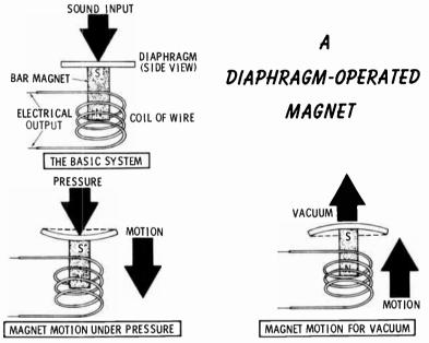
As in other phones, this diaphragm vibrates at the frequency of the sound waves striking it. As it vibrates, the bar magnet moves back and forth within the coil. This induces a current which changes direction at the same frequency as the sound. If the transmitter is connected to a sound-powered receiver, current will flow back and forth through the circuit.
