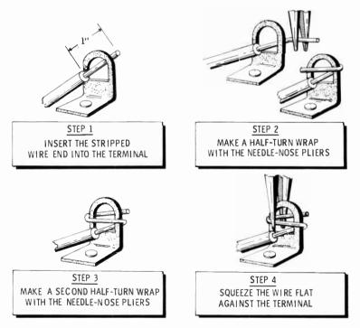
**Preparing the Wire**—The insulation must first be removed from the end of the wire. From 3% to 1 inch or more of bare wire is needed, depending on the type of connection to be made. If the wire is not bright and shiny, it probably has an oxidized film on it. The film should be removed by scraping with a knife or rubbing with fine sandpaper.
