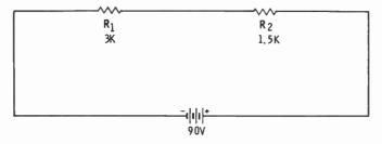
$R_1$  is twice the value of  $R_2$  in the above circuit. Both are in series across 90 volts. How do you find the voltage drop across each resistor?
