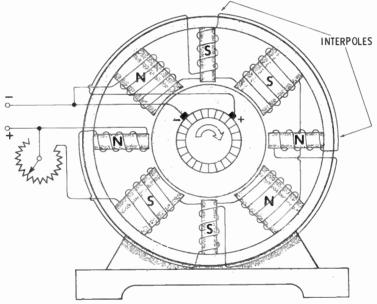
Interpole windings are connected in series with the armature windings and are wound in such a direction that the polarity of the interpole always has the same polarity as the nearest main-field pole in the direction of rotation.
