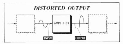
In the figure above, the leading half of the cycle in the output has been distorted. You would, therefore, suspect that the amplifier had gone into saturation and was clipping off that portion of the wave. You could also reasonably conclude that the most probable cause of the trouble was a change in tube bias.
