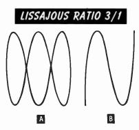
the starting point. The figure is continuous; it has no beginning or end. Figure B, however, is not continuous; it has a beginning and an end. Its pattern is **open**.
