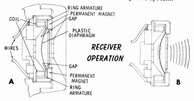
Part B shows that the diaphragm vibrates when a soundvarying current passes through the receiver. The current passing through the coil develops a magnetic field which varies in strength with the changes in current. Thus, the field developed by the current periodically repels and attracts the steady magnetic field of the permanent magnet, causing the magnet to which the diaphragm is fastened to move back and forth. This action reproduces the original sound.
