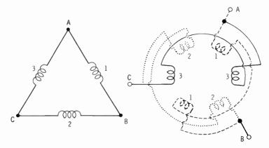
The windings are connected end to end in a sort of loop. When the system is properly balanced, almost no current flows around the loop because of the phase differences of the voltages. The delta-connected system has no neutral point. Delta-connected systems are not usually grounded.
