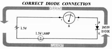
With the connections made as shown, current will flow and the lamp will light. The ammeter will record very close to 200 milliamps. Now reverse the connections of the diode. Will the lamp light? No. And, as indicated in the next drawing, the meter pointer will remain on zero. The plate-tocathode resistance of the diode is sufficiently high to prevent a flow of current. A small amount may leak through, but it is not enough to record on the meter.
