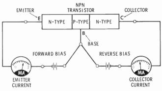
The figure shows an NPN transistor biased properly to operate as an amplifier. Addition of certain resistors (which you will see later) would complete the picture.
