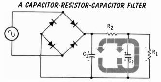
By adding another capacitor in parallel with the load resistor and another current-limiting resistor in series with the discharge path, the filter network can reduce more of the ripple.
