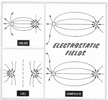
This area therefore contains electrostatic lines of force between two charged bodies. There is an electrostatic field around each charged body. When two positively or two negatively charged particles are placed near each other, their electrostatic fields repel each other. However, when a positively charged particle is placed near a negatively charged particle, their electrostatic fields attract each other. Like charges repel, and unlike charges attract.
