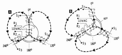
In part A, the rotor is positioned at zero degrees. When 115V AC is applied to the rotor winding (the primary), a magnetic field is developed. As in any transformer, lines of flux cut the secondary windings inducing a voltage in them.
