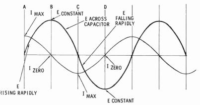
Current and voltage vectors in a capacitive circuit are  $90^{\circ}$  out of phase. In this case the current vector is **ahead** of the voltage vector by  $90^{\circ}$ .
