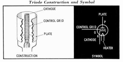
**Operation**—Plate current in a diode is determined by cathode temperature and plate voltage. In a triode, the voltage of the grid with respect to the cathode also controls the amount of plate current.
