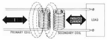
Q1. Magnetic lines must be (moving, stationary) to induce current in a conductor.
