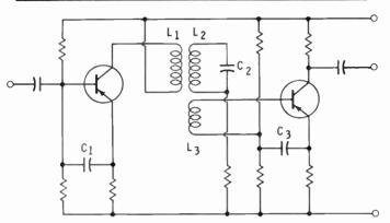
of the tuned circuit. Energy is easily transferred to  $L_3$  by transformer action. At all other frequencies the circulating current is much less, and the energy transfer is very low.
