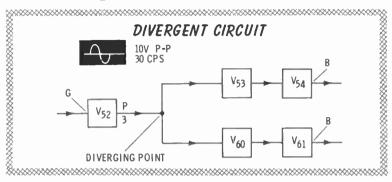
The illustration shows that the input to the divergent circuit  $(V_{52})$  is good and that the output should be a 30-cps sine wave at 10 volts peak-to-peak. If the B indicates no output at either point, the first test should be made at the output (pin 3) of  $V_{52}$ . If there is no output at this point, enclose  $V_{52}$  with a G and a B, and Step 4 is concluded.
