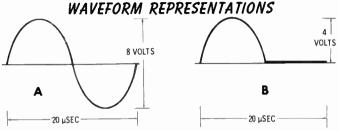
Part A above shows the same sine wave as on the preceding page. The dimensions are 8 volts from its positive peak to its negative peak. The time duration of one cycle is 20  $\mu$ sec (microseconds). A microsecond is one-millionth of a second.) Part B shows the same waveform after it has been rectified (using a diode circuit, for example). The single peak remaining is 4 volts from zero to maximum positive. The time duration of the cycle is still the same 20  $\mu$ sec.
