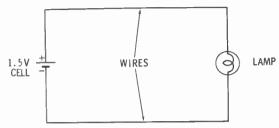
The lamp and cell symbols are connected by lines representing wires. Note that the lines run in only two directions—horizontal and vertical. Slanted or curved lines lessen the clarity of a diagram. Also note that a voltage value and polarity markings appear on the cell.
