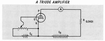
Battery  $E_B$  is connected in such a way that the plate is positive with respect to the cathode. In an actual circuit the positive voltage for the plate is normally obtained from a power supply. Battery  $E_C$  places a negative voltage on the grid with respect to the cathode. A resistor takes the place of this battery in an actual circuit.
