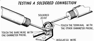
An ohmmeter test does not always reveal a poor soldering job. But if the meter reads zero; the solder looks neat, smooth, semishiny, and well blended into the metal; and you observed all the precautions, the connection should be electrically good. The precautions are restated below.
