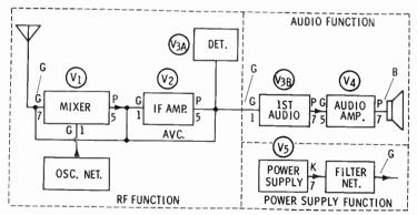
Good test indications are made at the input of  $V_{3B}$ , and the output of the filter network in the power supply. A bad test is identified at the speaker input.
