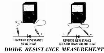
Diode Test Set—Test sets are available to check the rectifying qualities of a diode. Some of them provide a combination resistance and current test. When the set is used as an ohmmeter, it will measure forward and reverse resistance. When it is used as a milliammeter, it will measure forward and reverse current. Others use one or the other to obtain the forward-to-reverse ratio. Most sets are constructed as shown in the following diagram.
