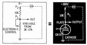
In effect, the grid varies the resistance of the vacuum tube.  $P_2$  is always +300V (to ground).  $P_1$  is a positive
