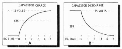
RC is a quantity obtained by multiplying R (ohms) by C (farads). Any capacitor in an RC circuit (such as this one) charges to 63% (actually 63.2%) of its final value (battery voltage) in one RC second. In 5 RC seconds it reaches full value. The arithmetic statements are:
