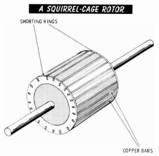
the rotor instead of a wire winding. The winding resembles a squirrel cage, from which it derives its name. The squirrelcage motor has the advantages of requiring practically no maintenance and of costing much less than a wound-rotor motor.
