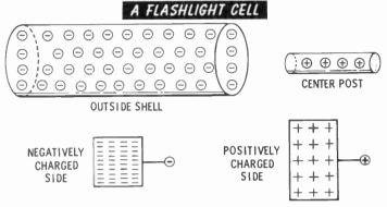
A battery is one such form of voltage source. It has an excess of negative charges on one terminal and a lack of negative charges on the other terminal. When the two battery terminals are applied properly to other elements, a complete path from one terminal to the other is formed. The more negative terminal gives off negative charges that pass through the other elements to the positive terminal.
