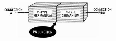
DIAGRAM OF A SOLID-STATE DIODE
