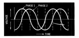
PHASE RELATIONS IN A TWO-PHASE GENERATOR The armature windings of a two-phase generator can be connected in two different ways. It is possible to simply make individual connections to the two separate windings. This arrangement gives four output connections and is called a **four-wire system**.
