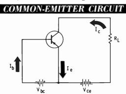
As you know, *a* is the ratio of collector-current change to emitter-current change and is equal to  $\frac{\Delta I_c}{\Delta I_e}$ . It is also called the **common-base**, forward-current transfer ratio. If the transistor were connected in a common-base circuit, *a* would represent its current gain (with the collector voltage held at a constant value).
