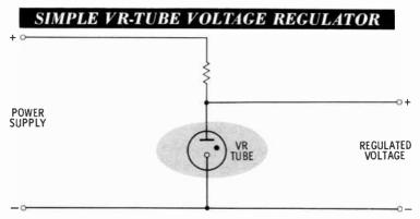
The limiting resistor in series with the VR tube is selected to limit the current through the tube to a safe value. Gaseous voltage regulators keep the output voltage constant to within about 1%. They come in a number of specific voltage ratings. To change the constant output voltage, it is necessary to change the tube. To obtain higher voltage ratings, VR tubes can be connected in series so that only part of the output voltage appears across each one.
