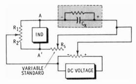
Essentially this is the same basic circuit as before. A switch on the front panel connects a variable resistance in place of  $C_1$  and changes the voltage source to a variable DC. Voltage is set at the rated working voltage of the capacitor. An electrolytic capacitor will be damaged if polarities are not observed when connecting it to the measuring posts.  $R_s$  is adjusted to balance the bridge and obtain a null reading. If the measured resistance is low, leakage is high.
