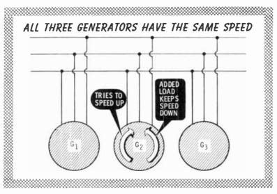
For instance, say that  $G_2$  in the figure above tries to speed up. Additional load is immediately placed on this generator. This tends to hold the speed down. This action keeps all of the generators operating at the same speed.
