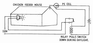
Selenium, used in solar and photoelectric cells, contains atoms that give up free electrons when struck by light. If iron is used as backing, the selenium will emit electrons into the iron. This will cause the iron to take on a negative charge, and the selenium to take on a positive charge. Wires connected to the two metals form the electrical source terminals.
