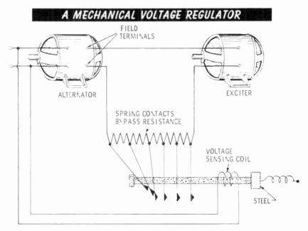
the resistance between the exciter and the alternator increases. This causes less field current to flow to the alternator, and the output voltage decreases to normal. If the voltage falls, the spring is able to pull the steel piece away from the coil. This closes more of the contacts. The resistance then decreases and the field current and output voltage increase. The resistance could also be placed in the exciter shunt-field circuit.
