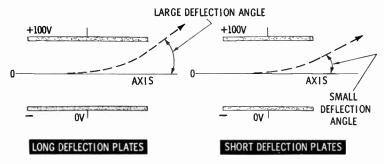
Spacing Between Plates—The closer together the plates, the more effect the electric force has on the electron beam.
