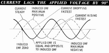
In a DC circuit, inductance has an effect only when the direct current first starts to flow, and then again when you try to stop it. But in AC circuits the voltage is constantly changing and inductance constantly acts to retard the change in current.
