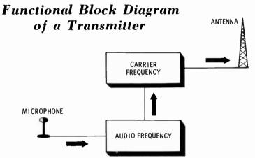
The arrowheads between blocks show the direction of signal flow. You can probably already read what the diagram reveals.
