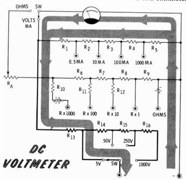
As you can see, the DC voltmeter circuit is a network of four resistors in series with the meter-shunt resistor combination. Simplified schematics for the 5- and 50-volt positions are shown in the diagrams below.
