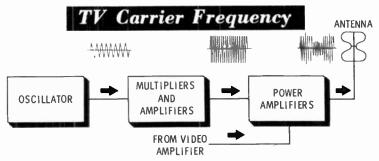
For VHF (very high frequency—channels 2 to 13), the frequency of the carrier is between 54 and 216 megacycles. For UHF (ultra high frequency—channels 14 to 83), the carrier is between 470 and 890 megacycles. Transmission of signals at these frequencies is quite different from that for the lower radio frequencies. High frequencies have short wavelengths. A wavelength is the time duration, or length, of one cycle. The higher the frequency of a signal, the shorter is its wavelength.
