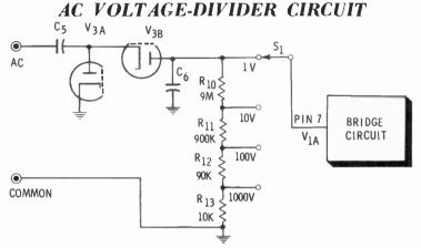
vent the DC that may be present in the input voltage from reaching the bridge circuit. In this arrangement the VTVM actually measures the peak value of the AC voltage. The rms value of a sine wave is 0.707 times the peak value. The scales of most VTVM's are marked to read the rms value.
