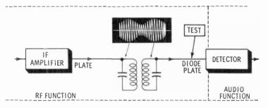
From the schematic diagram of the receiver, locate the pin number of the upper diode plate of the detector. Connect the oscilloscope to the proper socket terminal and rotate the tuning control. If no audio-modulated signal is noted at several station settings, the RF function is not operating properly.
