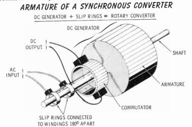
Under ordinary conditions, an alternating voltage is connected to the motor portion of the converter through slip rings, causing the machine to rotate at synchronous speed like an AC synchronous motor. At the same time, the machine also acts like a DC generator. This DC output is taken from the commutator by brushes and can be used to provide current for the field winding. This DC output can, in addition to energizing the field winding, furnish DC to an external load.
