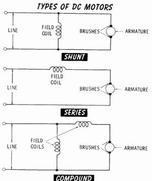
The direction of rotation of any DC motor can be reversed by reversing the leads of the field coils but leaving the armature connections unchanged. If both the field-coil and armature leads are reversed at the same time, the motor will continue to run in the same direction.
