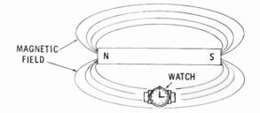
You probably know the danger to your watch if you wear it when working near magnets. Many watches made today are said to be nonmagnetic. This doesn't mean that you can lay your watch on a strong magnet with safety, but it does mean that the watch is shielded from ordinary magnetic fields (lines of force surrounding a magnet).
