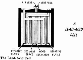
The lead-acid cell is the type used in an automobile battery and has a normal output of approximately 2 volts. Since it can be recharged, a lead-acid cell is called a secondary cell. A lead-acid battery must be constructed of a material that will not be eaten away by the highly corrosive electrolyte. For this reason, rubber or glass is normally used for the case that contains the cells and solution.
