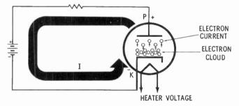
The Plate—The plate (sometimes called an **anode**) is a metal cylinder mounted around the cathode. With a battery connected to the diode as shown in the diagram, current flows through the tube. Negative voltage on the cathode (symbol K) repels the negative electrons from the cloud toward the plate (symbol P). Positive voltage on the plate attracts the electrons. Current flows from the plate through the external load, through the battery, and back to the tube via the cathode.
