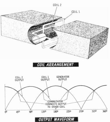
OUTPUT OF A TWO-COIL DC GENERATOR
