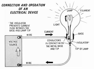
Wires, connectors, and terminals allow current to flow in a circuit because they are made of conducting metals. Care must be taken, however, when joining these parts to each other. Metal at the contact points must be clean and free from the insulating properties of dirt, grease, etc. Sandpaper or a small file can be used to clean these junction points when necessary. After a wire has been stripped, it should be cleaned of any remaining insulation.
