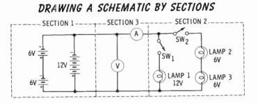
As you recall, an ammeter is always connected in the circuit path. Therefore, the ammeter in the above illustration is placed in series with the source and the load. A voltmeter is always placed across (in parallel with) the load or source.
