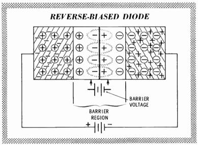
in a larger barrier voltage. The action continues until the barrier voltage equals the reverse bias (battery voltage). No current flows because these voltages are equal and opposite. This condition is called equilibrium.
