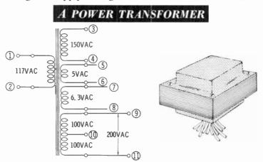
these windings (3 and 4) provides 150 volts AC, and the other (9, 10, and 11) provides 200 volts AC with a center tap. The use of this center tap will be explained later.
