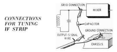
There is a choice of output indicators available. Whichever you choose, adjustments are made for maximum output indication and not for a precise numerical reading.
