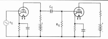
Resistor  $R_{g}$  is called the **grid-leak resistor**. This resistor serves to keep the grid at ground potential, thus preserving the voltage difference between the grid and cathode. This resistor actually serves a dual purpose, also being used as the component across which the signal voltage from the preceding stage is developed.
