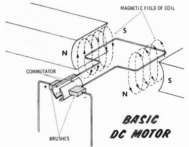
You can analyze the magnetic forces acting on the simple coil by using the left-hand rule for straight conductors. The figure above shows the field around the coil.
