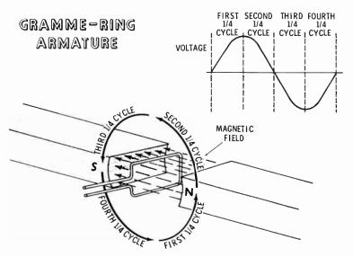
Since the armature windings of the Gramme-ring core are wound on the surface of the core, the distance between the core and the pole pieces must be great enough that there is no danger of the armature windings touching the pole pieces. This causes a reduction in the strength of the magnetic field. The weakened field results in reduced output from the generator.
