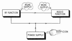
The new Step-2 conclusion places the probable location of the trouble in the power-supply function. A Step-3 check of the schematic for the receiver indicates that there should be a pulsating DC output of 90V. With a VTVM or multimeter, the DC reading shows less than half this value. The faulty function has been confirmed.
