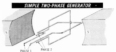
apart. Thus, when the voltage in one coil reaches its peak, the other one is at zero, and vice versa. The figure below indicates the phase relationships in a two-phase alternator.
