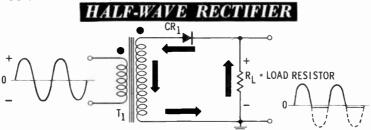
Above is a typical half-wave rectifier with a power transformer in the input. Notice the dots at the top of each winding of  $T_1$ . These dots indicate that the transformer is wound in such a fashion that the voltages at the ends of the windings marked with the dots are in phase with each other; when the top of the primary is positive, the top of the secondary is also positive.
