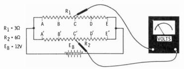
Suppose that a parallel circuit had unequal resistances, as shown above. The voltage across  $R_1$  or  $R_2$  would be identical, that is, 12V. Again assume quarter-section divisions.
