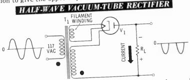
In its operation, this circuit is very similar to the semiconductor half-wave rectifier. On the positive half cycles, a positive voltage is applied to the cathode of the diode, and the diode will not conduct. On the negative half cycles a negative voltage is applied to the cathode, and the diode does conduct. Current flows down through R<sub>L</sub>, producing an output of the polarity shown. Thus, only negative half cycles appear at the output.
