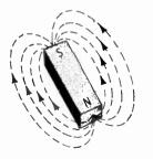
when the magnet is suspended in air, the north end of the magnet points toward the north geographic pole. Such a magnet has a magnetic field existing in the space surrounding it, with the lines of magnetic force taking the directions shown.
