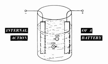
In order for electricity to be produced, there must be a way to transfer charges from one place to another. This transfer of charges is made possible by the use of conductors.
