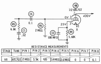
As in the previous example, part numbers and their values are shown on the schematic. If the trouble is isolated to one section of the circuit, the individual parts can then be measured. If, for example, something other than 25V and 920 ohms were read from pin 3 to ground, either  $C_3$  or  $R_4$  would be suspected of causing the trouble.
