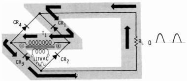
On the positive half cycle, current flows through  $CR_3$ , up through the load resistor, and back through  $CR_1$ .  $CR_2$  and  $CR_4$  are reverse-biased and act like open switches.
