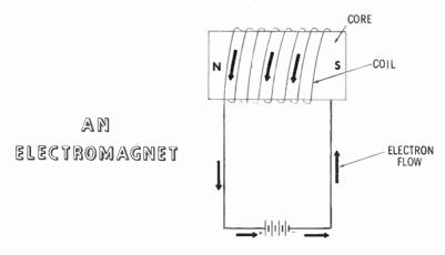
When a current flows through the coil, a magnetic field is produced around the coil. If the core conducts the magnetic lines of force easily, it becomes a temporary magnet when current flows through the coil. The current supplied to an electromagnet is DC, since AC would cause the polarity to constantly change.
