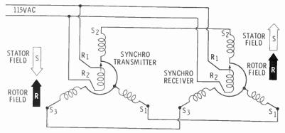
Since the rotor currents are in phase, the directions of their magnetic fields will be identical. The stator field in the transmitter is opposite to the rotor field. However, the stator field of the receiver will be in the same direction as the transmitter rotor field. The rotor field of the receiver will be attracted to align itself in the stator field direction.
