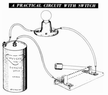
There are many other types of switches, some of which you have used. For example, there are switches on the walls of your home, on the front of your appliances, and on the dashboard of your car. Nearly all operate on the knifeswitch principle. In the closed position, a metal blade makes an electrical contact between at least two conductors.
