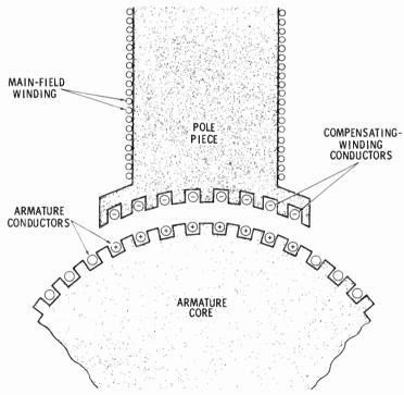
in the faces of the pole pieces. They are connected in series with the armature coils, like interpoles, but are wound in the opposite direction from the armature coils. The field of the compensating windings completely cancels the field of the armature that would tend to distort the main field of the generator.
