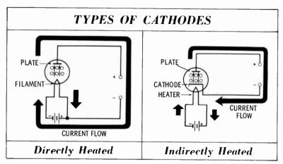
emitted by the thorium are replaced by the tungsten. The figure shows how the filament battery sends current through the filament, heating it and causing it to emit electrons.
