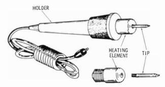
The heating power of an iron and gun is rated in watts. Irons are available with ratings from 6 watts or less to 500 watts and more. The larger irons are for heavy industrial use. Irons rated from 25 to 75 watts are best for most electronic work. Remember to use no more heat than necessary to obtain a properly soldered connection.
