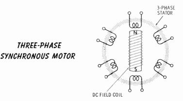
As the magnetic field in the stator rotates, the constant DC field rotates to keep aligned with it. As you can see, the speed of this motor depends on how fast the magnetic field rotates. The speed of the magnetic field depends on the frequency of the three-phase AC source. The synchronous motor cannot operate at any speed except that of the rotating field, which is called **synchronous speed**. Synchronous motors are used where it is important to maintain constant speed.
