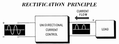
This simple principle is shown above. An AC voltage is applied to a unidirectional current-control device. Current flows only during the positive portions of the input signal. The output voltage is therefore composed of only the positive portions of the input. This output is called **pulsating DC.**
