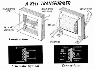
The Primary Winding—The primary winding is the input to the transformer. It receives AC voltage and current from a source. The primary of the bell transformer, for example, is connected to a 115-volt line.
