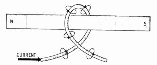
through them. A coil with a large number of turns has a magnetic field of greater strength than one with a small number of turns. The magnetic field is greater when a larger current flows through the coil.
