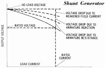
The shunt DC generator is well suited for constant-voltage applications at a specified rated output. When an additional load (beyond a critical limit) is placed on the generator, the output voltage falls off almost to zero. Any attempt to force a shunt DC generator to deliver more than its rated output could cause it to break down.
