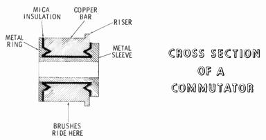
the segments. The raised part of the segment is called a riser and is slotted to hold the coil ends. The brushes ride on the lower portions of the commutator segments.
