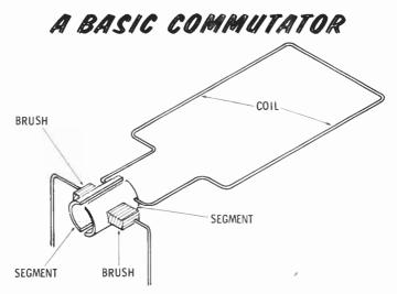
of the coil is connected to the other segment. Two brushes touch opposite sides of the commutator. As the commutator turns, the two sides of the coil are short-circuited for a moment as the brushes touch both segments of the commutator at once. Then the connections are reversed.
