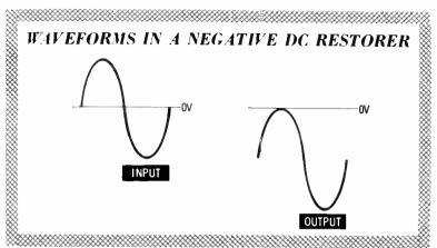
In this way the entire waveform has been shifted below the zero level to clamp the top of the waveform to zero volts. This circuit is known as a **negative DC restorer**. A **positive DC restorer** can be obtained by reversing the diode. In this
