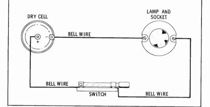
No two manufacturers will necessarily use identical symbols for the same part. Each symbol however, will be a close representation of the real thing. The switch symbol thus should show the terminals and make clear the difference between the open and hinged ends.
