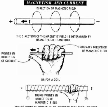
FINGERS POINT IN DIRECTION OF ELECTRON FLOW THROUGH WIRE.
