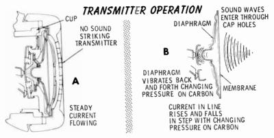
When the handset is lifted from its cradle, a steady current from the phone system starts to flow through the carbon granules. Sound striking the diaphragm places a varying pressure on the carbon. When the granules are packed tightly, current in the circuit increases. When the diaphragm releases its pressure, the granules become loose and less current flows.
