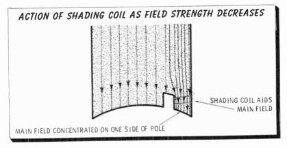
The effect of the shading coil is to produce a small sweeping motion of the main field from one side of the pole piece to the other as the field pulsates. This slight rotating motion is enough to start the motor.
