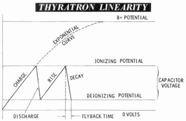
across the capacitor, the capacitor discharges rapidly. When the capacitor voltage falls to the **deionizing potential** of the tube, the thyratron stops conducting and acts as an open switch. Then the cycle repeats. The charge of the capacitor corresponds to the rise of the sawtooth, and the discharge corresponds to its decay.
