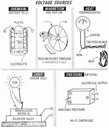
A battery or cell is a voltage source in which chemical action is used to develop a voltage potential. The cell is the basic unit. A battery consists of two or more cells placed together, end to end. For practical, uniform application, a dry cell is considered to be a 1.5-volt source. A lead-acid cell is a 2-volt source.
