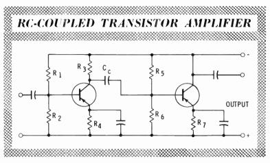
The output of the first stage is developed as a voltage across the load resistor  $(R_3)$  and is fed to the base circuit of the second stage through coupling capacitor  $C_{e}$ . This capacitor represents an open circuit to all DC voltages. Thus, the biasing circuits of the two stages are not influenced by the DC voltages on the other elements.
