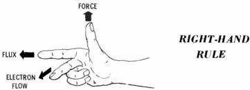
If a loop of wire is positioned in a permanent magnetic field, a force acts on the wire each time current passes through it. This force causes the loop of wire to rotate, if it is free to turn, as shown in the figure below.
