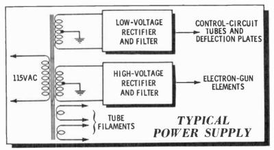
Most test scopes have both high-voltage and low-voltage power-supply sections fed by a single transformer. The high-voltage, low-current section takes care of the electrongun requirements. Voltage needs for the remainder of the circuits are supplied by the low-voltage section. This section may provide potentials as high as 300 or 400V. A third or fourth winding on the transformer provides voltage and current for the vacuum-tube heaters.
