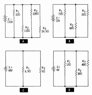
Q9. What is the power dissipated by each resistor and the total power for each circuit above?
