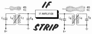
converter will be allowed to enter the IF strip. IF strip is a common term that includes the IF-amplifier tubes and transformers.
