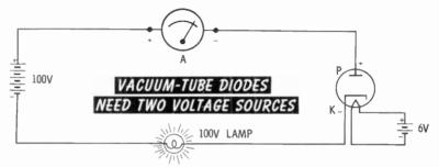
Current flows. Note that this particular diode requires a 6-volt source to heat the filament and 100 volts across the cathode and plate. Other vacuum-tube diodes operate with higher or lower voltages, but all require two sources.
