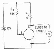
In effect, the path through the transistor from C to E has decreased from a very high resistance to a very low resistance. The transistor is operating as if it were a switch. The pair of diagrams below show the transistor acting as a switch. With no current through B, the transistor acts as an open switch; with current it acts as a closed switch.
