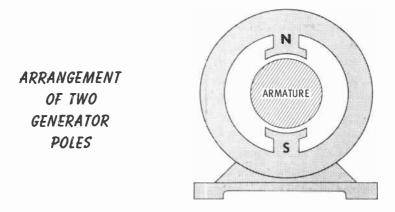
More than one pair of poles are sometimes used in order to produce a stronger magnetic field. When this is done, opposite poles are always next to each other. You can see from the following illustration how this arrangement creates the strongest magnetic field through the armature.
