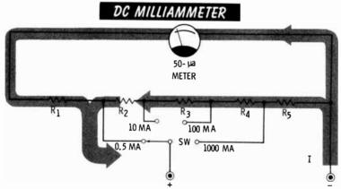
Notice that the arrangement is a parallel circuit in which the resistance can be changed in both branches by rotating a switch. Since the meter has a 50- $\mu$ a movement (full-scale deflection), the ratio of resistances must be such that 50  $\mu$ a will be the maximum current flowing in the meter branch at each switch setting. Redrawing the circuit for each switch position may help make this clear.
