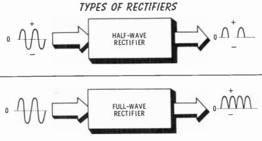
When AC voltage is applied to a full-wave rectifier, the load receives current during both half cycles. Notice that the negative half cycles have been inverted so that all the half cycles are positive at the output of the rectifier. This type of pulsating DC is much easier to smooth (filter) than the output of the half-wave rectifier. Thus, smaller and less expensive components can be used in the filter section.
