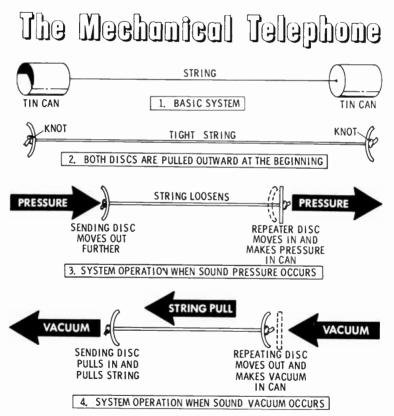
Note that the key part of the mechanical telephone system is the flexible metal disc at the bottom of each can. Speaking into the can causes sound waves to strike the disc and make it vibrate. The vibrations from one disc are carried to the other disc by a tightly stretched string. The second disc repeats the in-and-out motions of the sending disc and develops varying air pressures in the can. These are sound waves which are crude reproductions of the original sound waves.
