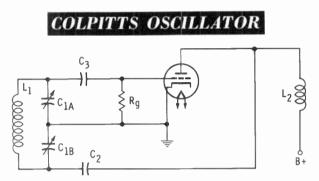
$C_{1A}$ ,  $C_{1B}$ , and  $L_1$  make up the tank circuit. The resonant frequency of the tank is changed by varying  $C_{1A}$  and  $C_{1B}$ . (These capacitors are usually on a common shaft so that both of them can be adjusted at the same time.) The output of the amplifier is introduced into the tank circuit through capacitors  $C_2$  and  $C_{1B}$ . The tank-circuit voltage is introduced into the grid of the amplifier by the coupling network consisting of  $C_3$  and  $R_{\rm g}$ .
