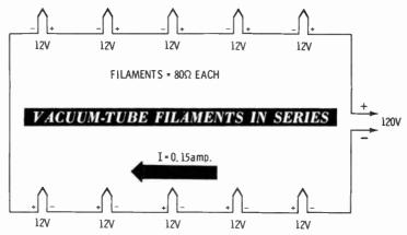
Another application of the series circuit is the economical series-string Christmas-tree lamps. The number of lamps needed in a string or the amount of voltage to apply can be determined by Ohm's law. If the voltage drop required by each lamp is 15 volts and the string is to be connected to a 120-volt outlet, then eight lamps are required in series.
