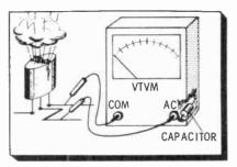
During the circuit-checking tests it is best to remove the transistor if it is the plug-in type. Removal is not absolutely necessary if you exercise necessary care.
