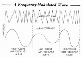
The Detector—FM and AM detectors have the same purpose—to remove the audio component from the modulated intermediate frequency. For FM, the variations in frequency are changed into voltage variations by the detector. The output of the detector (quite frequently called a discriminator because it discriminates between AF and IF), is an audio frequency representing the tone and amplitude of the sound originating at the studio.
