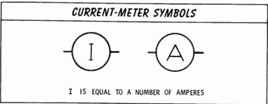
An ampere is the standard unit of measure for current (I) in a circuit. However, there are methods for describing very small or very large currents.
