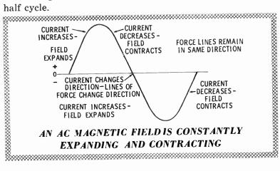
The diagram on the opposite page demonstrates how the magnetic field expands and contracts with the rise and fall of current. The field is in constant motion. An alternating current, therefore, induces current to flow in another conductor or coil. In this case, the induced current will also be alternating.
