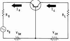
equal to  $\Delta I_e R_i$ . The voltage across the load resistor is  $\Delta I_e R_i$ . The voltage gain in this case is  $\frac{\Delta I_e R_L}{\Delta I_e R_i}$ . Note that  $\frac{\Delta I_e}{\Delta I_b}$  in this case is not *a* because the collector voltage does not remain constant.
