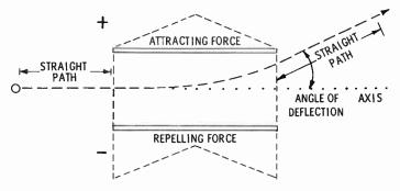
Length of Field—A long field has more time to exert its deflecting forces on an electron beam than a shorter field. Therefore, it bends the beam to a greater deflection angle. This fact assumes that all other factors are equal.
