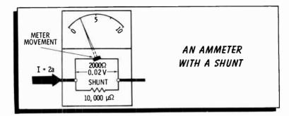
This meter has a movement with 2,000 ohms of resistance and is shunted by a 10,000 micro-ohm (0.01 ohm) resistor. This permits 10  $\mu$ a of current to flow through the movement and 2 amps (minus the 10  $\mu$ a) of current to flow through the shunt. These may not be the exact values for a particular multimeter, but all multimeters employ similar ratios.
