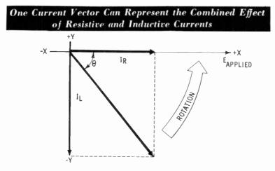
think of it as being generated by a rotating current vector. However, this vector is a combination (or resultant) of the resistive and inductive current vectors.
