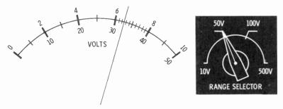
apply. With the range shown, the meter reads 32.5 volts.
