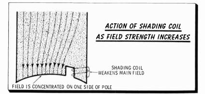
site side of the pole piece. The result is that the field in the part of the pole piece inside the shading coil reaches a maximum intensity later than the rest of the field. As the field in the part of the pole opposite the shading coil begins to decrease, the shading-coil field will start aiding the main field, and the concentration of flux moves to the other edge of the pole piece. The resulting field in the part of the pole piece inside the shading coil reaches zero after the main field.
