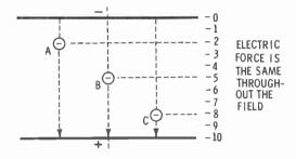
In the figure above, three electrons are located in an electrostatic field. All three are attracted by the positive plate and repelled by the negative plate. The distance between the plates is marked off in 10 equal units; electron A is 2 units away from the negative plate, electron B is 5 units away, and electron C is 8 units removed.
