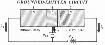
reverse bias between collector and base is provided by  $V_{ce}$  in series with but opposing  $V_{be}$ , and  $V_{ce}$  is large compared to  $V_{be}$ . Thus,  $V_{ce}$  replaces  $V_{cb}$  in series with  $V_{be}$ . This is called a grounded-emitter circuit.
