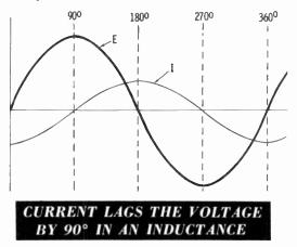
In a circuit containing only resistance, the voltage and current are in phase, and the voltage and current vectors have the same position. In a circuit having only inductance, the current vector is  $90^{\circ}$  behind the voltage vector. The length of each vector represents its magnitude.
