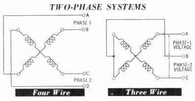
It is also possible, however, to combine two of the output connections to produce what is called the **three**-wire system. In this system the voltages of the two separate phases remain the same. Phase 1 appears between A and B. Phase 2 appears between B and C. But a third voltage is also available, the voltage between A and C. This voltage is the vector sum of the other two voltages.
