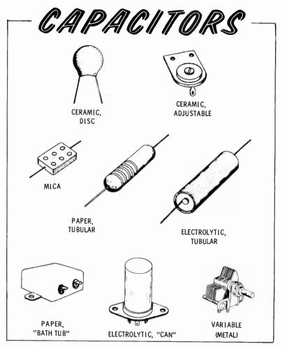
Several of each kind of capacitor are probably in your home. They can be found in radios, television receivers, intercoms, audio systems, and other electronic equipment. A capacitor is used with some electrical motors and even in the ignition systems of automobiles.
