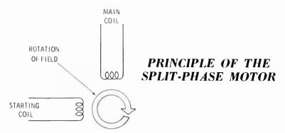
If used to run the motor, the starting winding is likely to burn out because of the small wire from which it is made. For this reason, a centrifugally operated switch is used to disconnect the starting winding when the motor reaches about 60% of operating speed.
