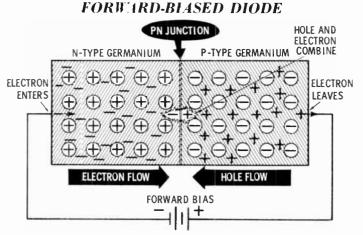
comes negative when a hole combines with an electron **a**t the barrier. Thus, it gives up an electron to the positive battery terminal. A solid-state diode symbol is shown below.
