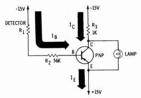
Current Flow in the Transistor Alarm Circuit
