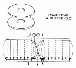
Since its path is parallel to the force lines, electron B will pass straight through the axis (center line) of the holes. Electron A starts in the same direction as electron B. When electron A enters the field, it turns in the direction of the force lines. Just before it leaves the field, it is turned even further and in the direction of the curvature of the force lines.
