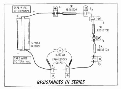
This is logical, because the total resistance in the circuit determines the amount of current allowed to flow with a given voltage source. Therefore, to find the total resistance in a circuit, add the values of the individual resistances.
