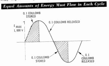
Q16. How much energy will be stored in a 100-mfd capacitor in the first quarter cycle of an applied AC voltage of 1,000 volts maximum?
