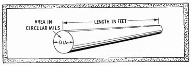
A circular mil is used as a unit instead of square inches to measure cross-sectional area of a wire. Circular mils can be determined by squaring the diameter (in mils) of a wire. A mil is 0.001 of an inch.
