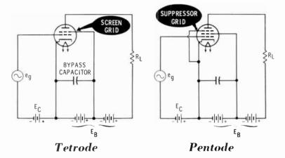
The suppressor grid prevents this current from flowing. It is electrically connected to the cathode, making it negative with respect to the plate, and thus repels any electrons that try to travel from the plate to the screen grid. The suppressor grid is actually a fairly coarse screen so that it does not interfere with the main current flow between cathode and plate.
