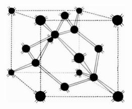
together. This electron-pair bond, called a **covalent bond**, is formed because each atom of germanium attempts to complete a full count of eight electrons in its outer ring. Whenever several cubic structures combine, the lattice-like effect becomes evident. A visible crystal of germanium is composed of many millions of these basic crystal lattices. This crystalline germanium is electrically neutral.
