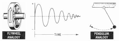
The LC circuit, the flywheel, and the pendulum have one quality in common—damping effect. Damping is the reduction of energy in a mechanical or electrical system as a result, in these cases, of absorption. The flywheel and the pendulum lose energy through absorption which is caused by the friction of the bearings and the surrounding air. The LC circuit (containing an unseen R) gives up part of its energy in the form of heat as the current passes through the resistive parts of the circuit.
