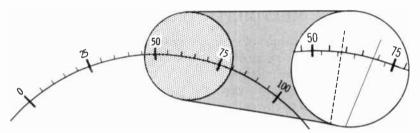
Q16. The solid pointer in the diagram above is between 65 and 70 and slightly beyond the midmark. The meter reads 68. What is the reading indicated by the dotted pointer?
