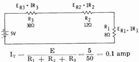
The voltage across  $R_1$  equals  $IR_1$ , or  $0.1 \times 8 = 0.8V$ . The voltage across  $R_2$  equals  $IR_2 = 0.1 \times 12 = 1.2V$ . The voltage across  $R_3$  equals  $IR_3 = 0.1 \times 30 = 3V$ . The total IR drop is equal to the source voltage.
