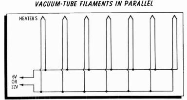
In each case, you can see that all sources or all loads are connected across the same two points. This produces a circuit which has one common voltage applied to all loads.
