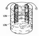
CURRENT FLOW IN THE CELL The dry cell is the most common type of DC-voltage source. It is constructed with an outside shell of zinc, a center rod of carbon, and a paste form of electrolyte which is a solution of ammonium chloride.
