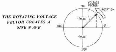
One complete cycle of a sine wave (from zero to a positive peak, down to a negative peak, and back to zero) simply represents one complete rotation of the voltage vector.
