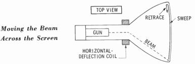
A horizontal-deflection coil wrapped around the neck of the tube moves the beam from side to side. Current moving through the coil sets up a magnetic field which has an attracting and a repelling effect on electrons similar to positive and negative voltage. The stronger the field, the greater is its effect on the beam. To increase the strength of the field requires an increase in current through the coil. The illustration shows the beam deflected to the left.
