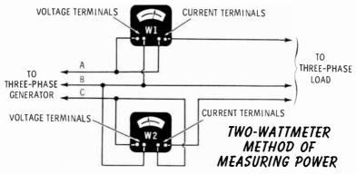
Total power is found by adding the two readings shown on the wattmeters. If the power factor of the load is less than 0.5, the wattmeter readings must be subtracted to obtain the total power. The sum (or difference) of the meter readings gives the total power because of the phase relationships of the voltages and currents in the three-phase system.
