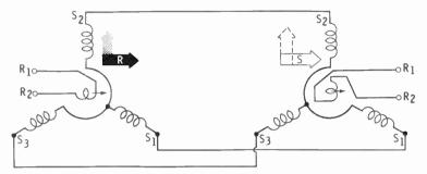
Assume that the T rotor has been turned clockwise from  $0^{\circ}$  to  $90^{\circ}$ . The CT stator field will make the same rotation. If the CT rotor remains at  $0^{\circ}$ , maximum voltage in phase with the AC line voltage can be measured across  $R_1$  and  $R_2$ . If the CT rotor is now turned to  $90^{\circ}$ , the voltage reading will reduce to zero. In this position the rotor winding is at right angles to the stator field.
