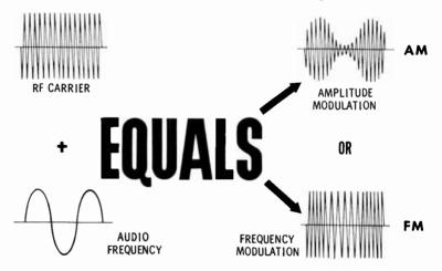
Both AM and FM start out with a carrier frequency and an audio frequency (sound originating in the studio). In amplitude modulation, as you already know, the sound is superimposed on the carrier frequency (which is constant) by varying the carrier amplitude in conformance with the voltage and frequency of the audio.
