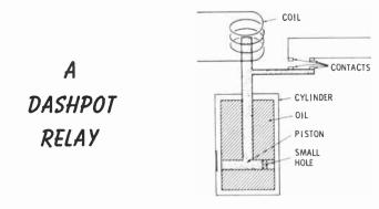
Q26. Two types of time-delay relays depend on a \_\_\_\_\_ or a \_\_\_\_\_ to determine the amount of time delay.
