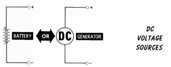
Symbols used for DC voltage sources in schematic diagrams are normally those of a battery or a DC generator.
