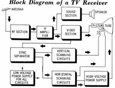
The illustration above shows a single antenna bringing both the FM sound carrier and the AM video carrier to the RF (radio frequency) circuits. This is satisfactory since the sound- and video-carrier frequencies are fairly close together (the sound carrier is 4.5 megacycles higher).
