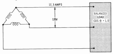
A18. Line current, 17.3 amps; line voltage, 120V Phase current, 10 amps; phase voltage, 120V Power =  $I_L \times E_L \times 1.73 \times 1 = 3,600$  watts or  $I_p \times E_p \times 3 \times 1 = 3,600$  watts
