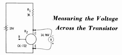
Under these conditions, current in the circuit would be very small, about 15 millionths of an amp. In effect, the high resistance of the transistor is very close to being an open circuit—no current flowing.
