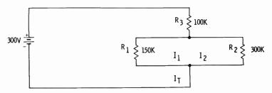
To find the effective load for the 300V source,  $R_T$  must be calculated. One approach for finding  $R_T$  is to first find the total resistance for the parallel branch ( $R_1$  and  $R_2$ ); then the sum of the total parallel resistance plus  $R_3$  should be found. After the total resistance has been determined, the total current can be calculated.
