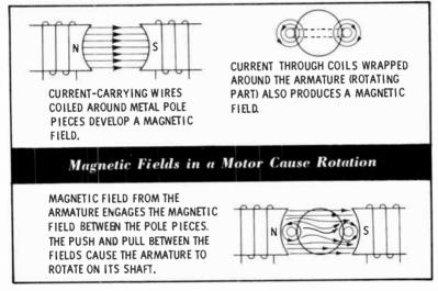
The magnetic forces in the motor are created by current flowing through the motor coils.
