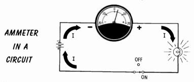
indicates plus, the auto is getting electrical power from the generator and, at the same time, the battery is being charged. Therefore, a minus meter reading indicates the battery is being used, and a positive meter reading indicates the battery is being charged. Before the days of long trips and dependable voltage regulators on the automobile, the operator had to watch the ammeter very closely.
