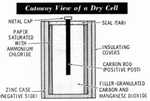
The zinc and the electrolyte are gradually "used up" as the dry cell supplies electricity. A dry cell is called a **primary cell** for this reason. The consumption of material in the cell is a result of chemical action between the zinc and the electrolyte. When the zinc case and the electrolyte have been used for some time, the chemical action which created the ion movement will decrease to a point where the cell is considered run-down (discharged).
