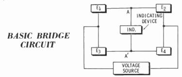
If voltage were applied across the bridge (parallel) circuit, current through the indicating device would be zero only when the voltages appearing at points A and A' were equal. Another fundamental principle is that the voltage across a parallel network is the same for either leg. In other words (disregarding voltage dropped in the conductors),
