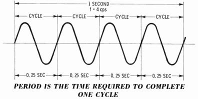
Frequency is measured in cycles per second (cps). The symbol for frequency is f. The most common type of current (household current) has a frequency of 60 cps in most localities.
