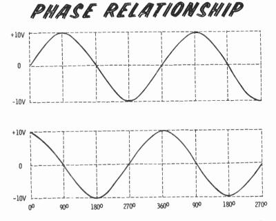
The top waveform (sine wave) rises from zero to 10 volts positive in  $90^{\circ}$  (one-quarter cycle). During the same time period the bottom sine wave decreases from 10 volts to zero. In other words, the two are  $90^{\circ}$  out of phase.
