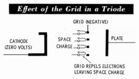
The direction of this field is determined by the polarity of the voltage applied to the grid. For reasons which will become evident later, the grid is operated with a small negative voltage (relative to the cathode) applied to it. The effect of this voltage is to repel electrons which would otherwise leave the space charge and flow to the plate.
