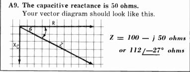
If you have a table of trigonometric functions, you can get more accurate measurements of impedance, using the same formulas you used to find inductive impedance. Remember, these formulas apply to both inductive and capacitive impedance.
