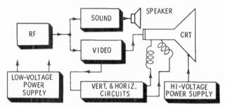
Suppose that during Step 1 you learned the following symptoms. Audio appears to be good, but the picture covers only half of the screen vertically. Width appears to be proper. Adjustment of the vertical control makes no apparent change in height, but does cause the picture to roll.
