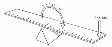
of five pounds is applied to the right end of the ruler, the resulting torque is calculated as follows:
