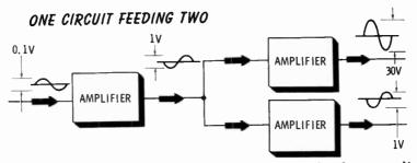
A low-amplitude sine wave is amplified by the first amplifier and fed to two others. Their outputs are quite different.
