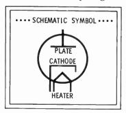
Each element is connected to a **pin** (two are for the heater) on the base of the tube. The pins fit into a tube **socket** having terminals to which connections can be readily made.
