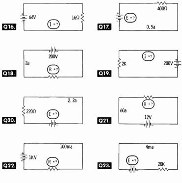
Your Answers Should Be: A16.  $I = \frac{E}{R} = \frac{64}{16} = 4 \text{ amps}$ A17. E = IR = (0.5) (400) = 200 voltsA18.  $R = \frac{E}{I} = \frac{200}{2} = 100 \text{ ohms}$ A19.  $I = \frac{E}{R} = \frac{200}{2,000} = 0.1 \text{ amp}$ A20. E = IR = (220) (2.2) = 484 voltsA21.  $R = \frac{E}{I} = \frac{12}{60} = \frac{1}{5}$ , or 0.2 ohm A22.  $R = \frac{E}{I} = \frac{1,000}{0.1} = 10,000$ , or 10K ohms A23. E = IR = (0.004) (20,000) = 80 volts
