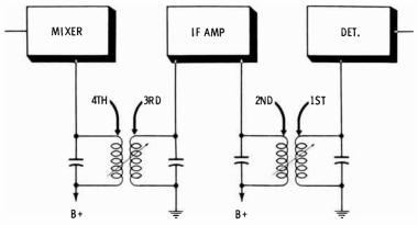
During this and all following alignment steps, keep the gain of the signal generator no higher than necessary to give an indication on the output indicator used. If the gain is too high, receiver stages will overload or saturate, and output readings will be invalid. Readjust all coils until you are sure they have been peaked to maximum.
