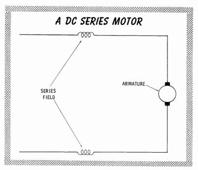
The starting and stalling torque of a series motor is excellent. It will start and carry very heavy overloads. Speed regulation, however, is very poor. The speed decreases as the load increases. Therefore, the motor turns slower with
