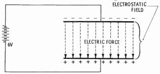
If a 6-volt battery is connected to the plates in the manner shown on the opposite page, the battery will draw electrons from the bottom plate and deposit them on the top plate until the difference in potential between the plates equals the battery voltage. The potential of the plate having an excess of electrons will be negative. The other plate, being deficient in electrons, will be positive.
