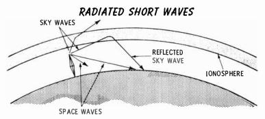
High frequencies radiate a space wave and a sky wave. Both of these waves travel essentially in straight lines. To receive a space wave, the receiving antenna must be within line-of-sight of the transmitting antenna. If the receiving antenna is beyond the horizon, the space wave (if it still retains sufficient power) passes over it.
