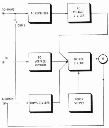
BLOCK DIAGRAM OF A TYPICAL VTVM
