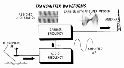
Superimposing the Sound—The process of superimposing AF on the carrier, as shown in this particular example, is called amplitude modulation (AM). In amplitude modulation the audio frequency (varying at the changing rate of the original sound) is mixed with the carrier (a constant frequency) in a manner that causes that carrier amplitude to vary at the same rate as the audio. The carrier frequency remains unchanged.
