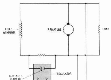
VOLTAGE REGULATION BY USING VIBRATING CONTACTS
