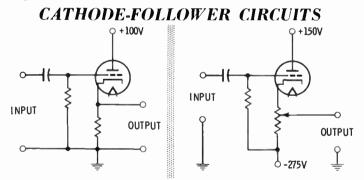
The only true way to determine whether the same triode will operate in either one of these cathode-follower circuits is actual trial in the circuit and observation of its performance. Laboratory models of tube testers approach this capability, but the simpler types do not.
