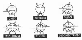
The tubes shown above are just a few of many combinations of tube elements. To conserve space, equipment manufacturers use multipurpose tubes as much as possible. The duodiode, twin triode, and duodiode triode are just three of many examples. A number next to an element indicates the number of the pin to which it is connected. This is normal practice in most schematic diagrams.
