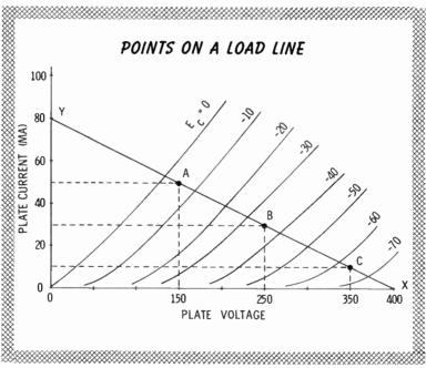
If the amplitude of the AC input signal is known, it can be marked off along the load line, as shown in the figure.
