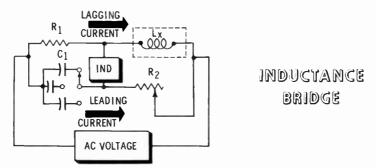
In this circuit, however, a capacitor is used to balance the inductance of a coil. A standard inductance could be used in place of the capacitance, but this would result in a few undesirable conditions.
