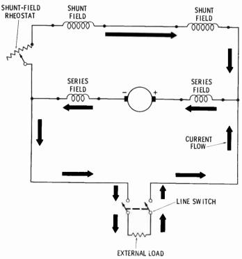
In a long-shunt compound generator, the shunt field winding is connected to the ends of the series field windings away from the armature. In a short-shunt compound generator, the ends of the shunt field winding are connected between the series field windings and the armature.
