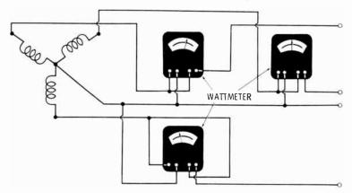
anced and unbalanced systems. Three wattmeters are simply used to measure the power in all three phases. A typical connection is shown at the bottom of the opposite page.
