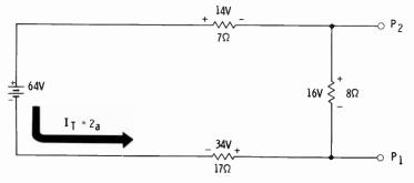
of its resistance. That is, the 17-ohm resistor in the above circuit will have 34V (2 amps times 17  $\Omega$ ) developed across it. The other voltages are determined similarly. Thus the voltage between P<sub>1</sub> and P<sub>2</sub> is 16V.
