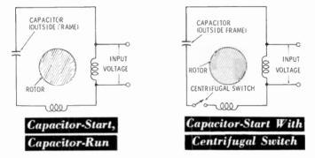
**Capacitor-Start Motor**—This motor starts with a capacitor in series with one of the windings. At about 75% of full speed a centrifugal switch opens the capacitor-winding circuit, and the motor operates as a single-phase inductor motor. This type is made in sizes from  $\frac{1}{8}$  to  $\frac{3}{4}$  HP.
