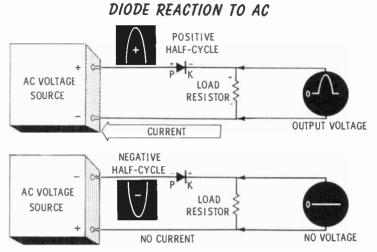
During a positive half cycle, the upper terminal of the source is positive with respect to the lower terminal. This means the lower terminal may be at zero volts, but it is negative when compared to the positive upper terminal. Therefore, the plate of the diode is positive with respect to the cathode. A changing half cycle of current flows.
