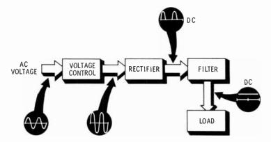
The basic functions of a power supply are to **rectify** and filter. The voltage-control function is actually incidental to the operation of the power supply. Once you learn to separate the rectifier and filter circuits from the power supply, you will see that the leftover components are in the voltagecontrol portion.
