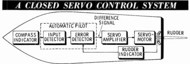
When the ship drifts off course, the change in compass heading generates a voltage signal which is transmitted to the error detector. Since the rudder and heading (compass) positions no longer agree, a difference signal is sent to the servo amplifier and motor to turn the rudder an amount and in the direction required to bring the ship back on course. When the ship is back on course, the rudder will have been returned to its amidships (straight ahead) position.
