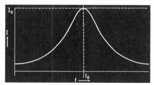
The quality of a resonant circuit can be measured by the Q factor. Q is the ratio of the energy stored in the capacitor and inductor divided by the energy dissipated in the resistor.
