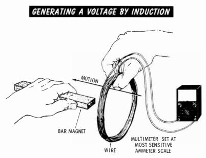
If an electric conductor is moved through a magnetic field in such a way that it cuts the lines of force, a voltage is generated, or induced, in the conductor. The induced voltage is greatest when the conductor moves at right angles to the magnetic field, and is zero when the conductor moves parallel to the lines of force.
