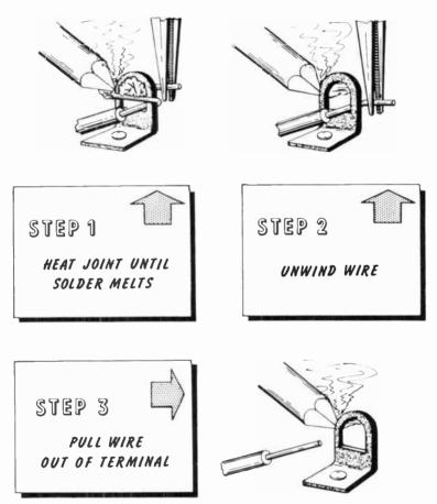
Place an ice pick or soldering aid into the eye of the terminal by following Step 3. This will prevent the opening in the terminal from remaining filled with solder.
