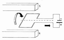
The simple motor shown in the figure above is not very practical. The coil cannot rotate very far because the current always moves through the wire in the same direction. When opposing poles appear opposite each other, the loop stops. Furthermore, any permanent connections to the loop of wire will not allow it to rotate very far.
