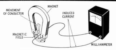
If a coil is connected to an ammeter and a bar magnet is moved through the coil, the ammeter will show that an electric current flows. This current is **induced** by the magnetic field only. If you move the bar magnet back and forth through the coil continuously, the induced current will be AC. Use the lowest amperage range on the multimeter for this experiment.
