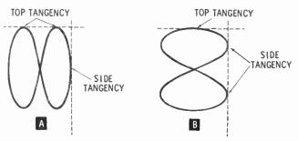
In figure A (above) one cycle of standard frequency appears on the horizontal plates at the same time that two cycles of the unknown are on the vertical plates. There are two points (loops) of top tangency and one point of side tangency. Frequency ratios should be expressed in terms of vertical (unknown) to horizontal (standard). The frequency ratio of figure A is 2/1.
