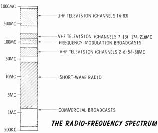
Commercial transmitters (radio and television, for example) are assigned a transmitting frequency in the appropriate part of the radio-frequency spectrum. Transmitters broadcasting in the home radio band, 535 kc to 1,605 kc (kilocycles), are required by law to be on their assigned frequency within plus or minus 20 cycles per second.
