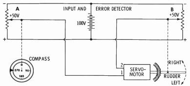
The input and error detectors contain a balanced potentiometer—the resistances of both potentiometer legs are identical. Potentiometer arm A responds to the turning of a compass. Arm B follows the movement of the rudder. Arms A and B are connected to the servomotor at terminals 1 and 2, respectively. A 100-volt battery is connected across the potentiometer.
