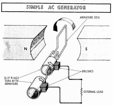
the armature coils, the ends of the coils are connected to slip rings which rotate with the armature. Stationary con-
