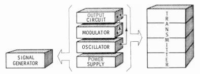
transmitter may emit signals at a higher power and include more circuitry than a signal generator, the basic functions of the two are identical. As shown, the basic functions include a power supply, an oscillator, a modulator, and an output circuit. Each function may require a group of many circuits in a transmitter; in a signal generator, however, each can be accomplished by only one or two circuits.
