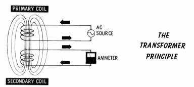
One coil has a current flowing in it. It is an AC current that sets up an alternating magnetic field in and near the coil. If another coil is placed next to it, there will be a second alternating current induced in the second coil. The first coil is the **primary**, the second coil is the **secondary**, and the combination of the two is a **transformer**. Most commercial transformers appear as shown on the next page.
