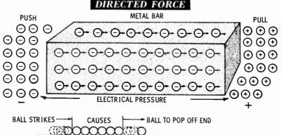
Electrical pressure is the most common form of control. This electrical pressure, or force, is made available by many forms of voltage sources.
