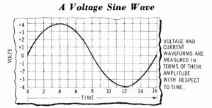
The illustration shows a single cycle of a voltage waveform. The AC sine wave, as this particular waveform is called, is continually changing at the rate indicated by its curvature.
