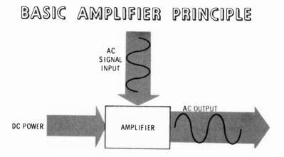
You can see from this diagram that the amplifier does not magically transform a low-power or low-voltage signal into a larger one. You can't get more power out than you put in. Instead, an amplifier controls the DC power from the power supply according to the variations in the AC input signal.
