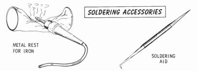
Soldering Aids—Soldering aids come in several shapes. They are used primarily to remove excess solder during soldering and unsoldering. The one shown above has a sharp point and hook. An ice pick can also be used.
