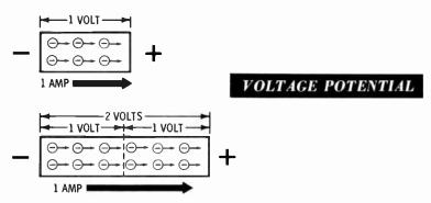
You can see that current will be the same through a conductor (with a specific voltage applied) as it is through a similar conductor twice as long but with twice the voltage applied. In each case, you could describe the voltage applied as a potential difference between the two ends of the conductor. What happens if the conductor is twice as long and the same potential difference is applied?
