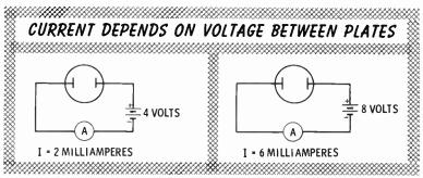
The resistance of the 4-volt circuit is 2,000 ohms. The resistance of the 8-volt circuit is 1,333 ohms. It can be seen that as the voltage between the plates increases, the resistance between the plates decreases.
