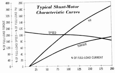
The main characteristics of a shunt motor are its constant speed and low starting torque. This means that DC shunt motors cannot be used for hard-starting loads.
