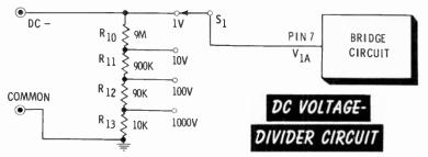
to the **COMMON** jack. A schematic representation of a fourposition switch is shown at the right of the voltage divider. Each position represents a tap in the resistor string. Each tap corresponds to a range setting. The sum of the resistances in the voltage divider is 10 megohms. This large resistance will be in parallel with the measured circuit at any range setting. Loading of the circuit under test is therefore very small.
