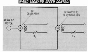
The shunt fields of both the generator and motor are supplied from a constant-voltage source. The DC-generator output voltage is controlled by rheostat  $R_1$ . The voltage variation (out of G and into M) gives a wide range of speed control. In addition, by varying the motor rheostat  $(R_2)$ , a wider speed range can be obtained.
