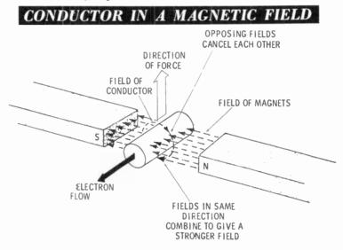
The direction of the magnetic field surrounding the conductor can be determined by applying the **left-hand rule** for straight conductors. Wrap the fingers of your left hand around the conductor so that your thumb points in the direction of electron flow through the conductor. Your fingers then show the direction of the magnetic field surrounding the conductor. External magnetic fields are considered to flow from the north pole to the south pole.
