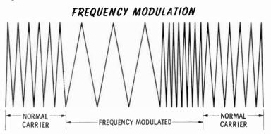
Notice in the diagram above that the frequency of the FM carrier varies, but its amplitude remains the same. Study the following diagrams.
