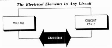
Voltage, as you know, is an electrical pressure that causes current to flow under proper conditions. Current flows if there is a closed loop (complete path) from one side of the voltage source through the circuit components to the other side. The amount and type of voltage to be applied and how much current will flow is dependent on the type and value of components used in the circuit. As an example, you have seen circuits similar to those shown in the schematic diagrams below.
