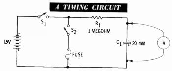
The resistor limits the amount of current flow which charges  $C_1$ . The values of  $R_1$  and  $C_1$  determine the charge time.
