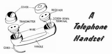
The transmitter contains a diaphragm resting against carbon granules (grains). The granules are loosely packed with enough freedom to expand and contract in volume.
