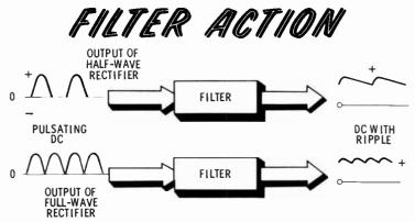
close the output is to DC. The higher the amplitude of the ripple voltage, the farther the output is from DC.
