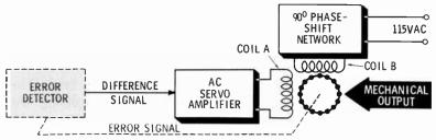
Coil B, the reference winding, is excited from an AC line through a 90° phase-shifting network. Since the same line feeds the rest of the servo system, the difference signal, in phase or 180° out of phase with the line, will either lead or lag the voltage in coil B by 90°. The servo amplifier amplifies the difference signal before it is applied to coil A.
