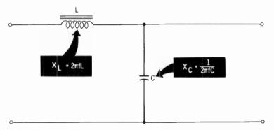
To understand the L-section filter with an inductor, the reactance of the inductor must also be considered. The reactance is high for AC, but it is nonexistent for DC. The inductor presents a high reactance to the AC current produced by the ripple voltage. The inductor therefore tends to block this current. It presents zero reactance to the DC and allows it to pass readily. The AC that is not blocked by the inductor is mostly bypassed by the capacitor.
