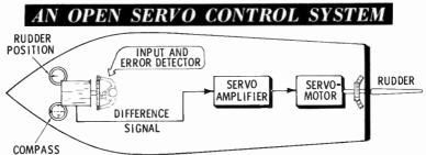
In this case, the man at the wheel is the input and error detector. He moves the wheel to maintain the ship on a specified course. He does this by watching the direction on a compass. When wind or ocean currents move the ship off course, he turns the wheel (and consequently the rudder) to bring the ship back on course. Because it is not automatic, the system is open.
