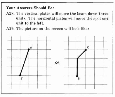
If the amount of deflection (in A29 above) to the left and down occurred so that each set of plates acted at the same time, the picture would be like the one on the left above. For example, if the vertical plates moved the beam downward at the rate of 1 unit per second and the horizontal plates moved it to the left at the rate of  $\frac{1}{3}$  unit per second, both movements would have been completed in 3 seconds at point B'. The result would be a straight line.
