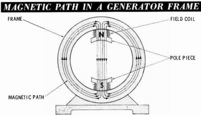
At one time, most generator frames were made of cast iron. Cast iron is heavier than steel and has a poorer **permeability** (ability to conduct magnetic lines of force), so it is used less frequently now. The frames of large generators are made of steel castings; those of smaller generators are made of rolled sheet steel. The frame of the generator also includes a base or mounting brackets.
