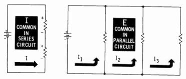
A parallel circuit has a common supply voltage, and thus a possible different current through each resistance (branch), depending on the value of the resistance.
