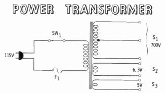
The diagram above shows a power transformer similar to those used in some radio receivers. It has three secondary windings— $S_1$ ,  $S_2$ , and  $S_3$ . Disregard the center tap on  $S_1$ .
