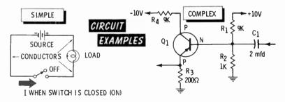
travels from the voltage source through the conductors and the load and returns to the source. This includes the path from terminal to terminal through the source.
