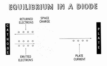
(plate current). The remaining or surplus electrons not required by the plate are returned to the cathode. The quantity returned is the difference between the amount of electrons originally emitted by the cathode and the amount going to make up the plate current. The result of all this is that the space charge is maintained at a constant size. In other words, it reaches and stays in a state of equilibrium.
