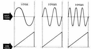
The sweep frequency should always be kept lower than or equal to the waveform frequency; it should never be higher. If the sweep frequency were higher, only a portion of the waveform would be presented on the scope.
