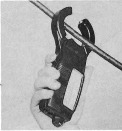
Fig. 22-12A. The General Electric Model AK-5 hook-on volt-ammeter being hooked on a cable.
