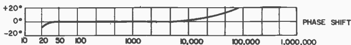
Fig. 12-168. Phase-shift characteristics for an amplifier with a frequency response of 20 to 20,000 Hz.
