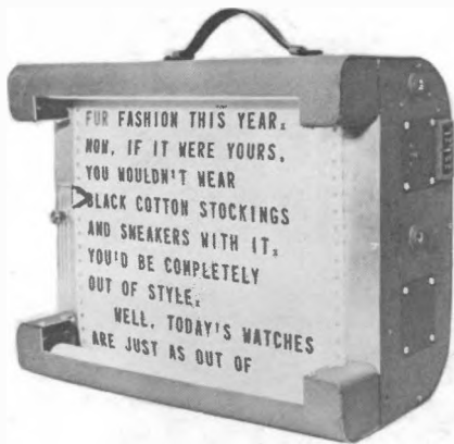
Fig. 2-72A. Teleprompter unit with script. The "hot line" appears to the right of the plastic pointer.
