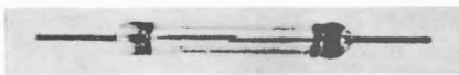
Fig. 25-147A. Reed relay encased in an envelope of glass, filled with nitrogen. Contact capacitance is 0.1125 picofarad. (Courtesy, Bell Telephone Laboratories)
