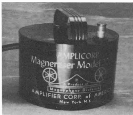
Fig. 17-66C. Hand bulk eraser manufactured by the Amplifier Corporation of America.
