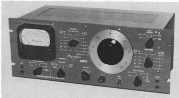
Fig. 22-126. Waveforms Inc Model 452A Transmission set designed for audio and telephone carrier use.
