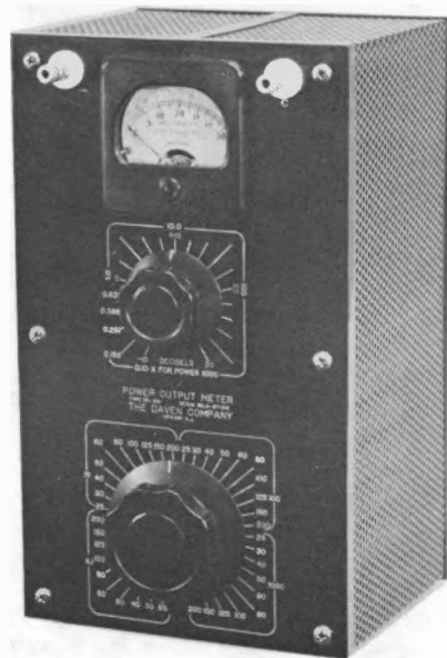
Fig. 10-35A. A power-output meter manufactured by the Daven Company.
