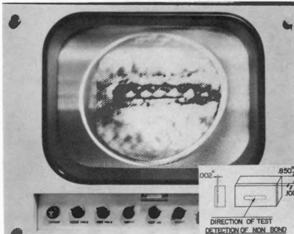
Fig. 25-215C. Ultra-Scan picture of a nonbond. Frequency, 2 MHz. Material, aluminum. The nonbond area is indicated by the dark pattern in the center of the display.
