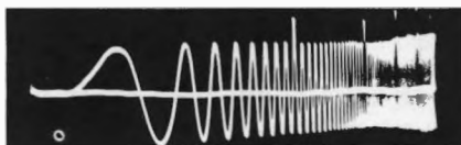
Fig. 16-49B. Pattern obtained for a reproducing system of uniform frequency response, using a sweep-frequency record as shown in Fig. 16-49A.
