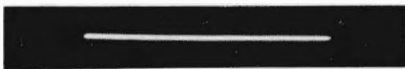
Fig. 22-129K. Appearance of an undistorted signal after passing through the 500-Hz, low-pass filter.
