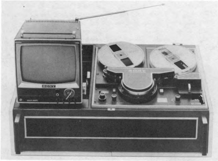
Fig. 17-231K. Sony Videocorder designed for home use. This machine uses a spiral tape transport system with two rotating heads.
