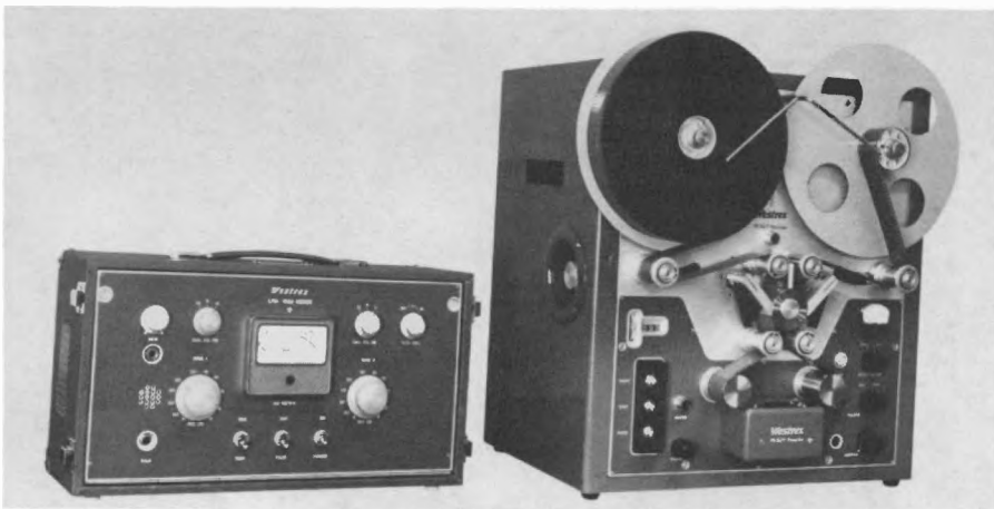
Fig. 17-177A. Westrex Series 1200 portable magnetic film recording channel, manufactured in Rome, Italy.
