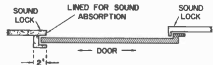
Fig. 2-69. Plan view of a typical sound-stage door installation. The sound lock on the left side starts at the floor and continues to the top and across to the right side. Rollers at the bottom support the weight of the door when it is opened.
