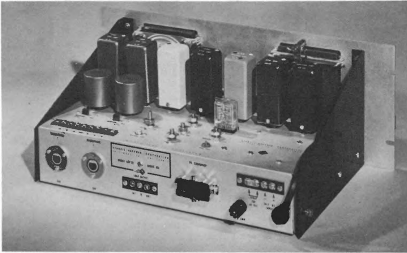
Fig. 17-180B. Stancil-Hoffman Model ARP70 transistor amplifier system for mixing, recording, or reproducing either magnetic tape or film.
