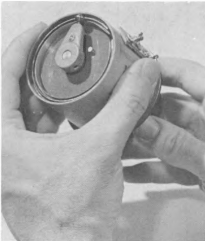
Fig. 9-8. Slide-wire ladder mixer control.
