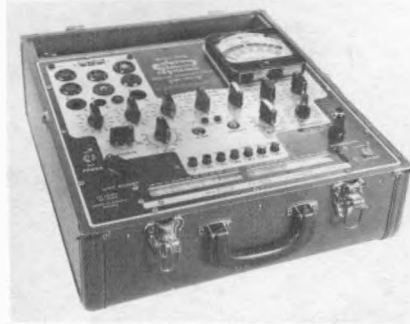
Fig. 22-115A. Dynamic mutual conductance tube tester Model 9-66A manufactured by Stark Electronic Instruments (Canada).
