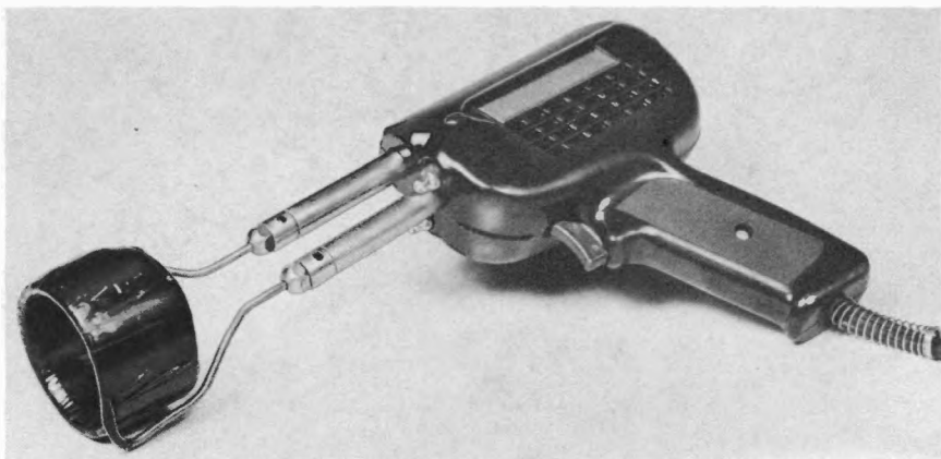
Fig. 17-90A. A degaussing tool made from a 250-watt soldering gun.
