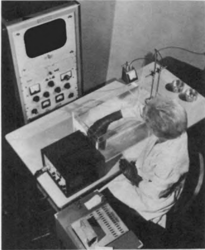
Fig. 25-215A. James Electronics, Inc. Ultra-Scan ultrasonic camera system.
