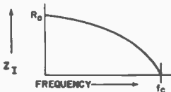
Fig. 7-25. Impedance characteristic of a constant- k filter.
