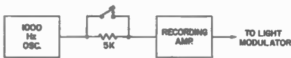
Fig. 18-65A. A circuit for measuring the opening and closing times of a noise-reduction system.
