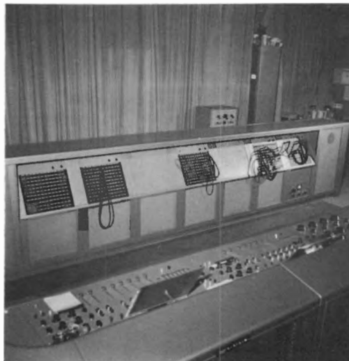
Fig. 9-22D. View taken looking over the console toward the patch bay. Here changes in the method of operation are made by the use of patch cords. (Courtesy, Universal Studios Sound Department )
