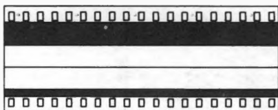
Fig. 17-30B. 35-mm stripe magnetic film.
