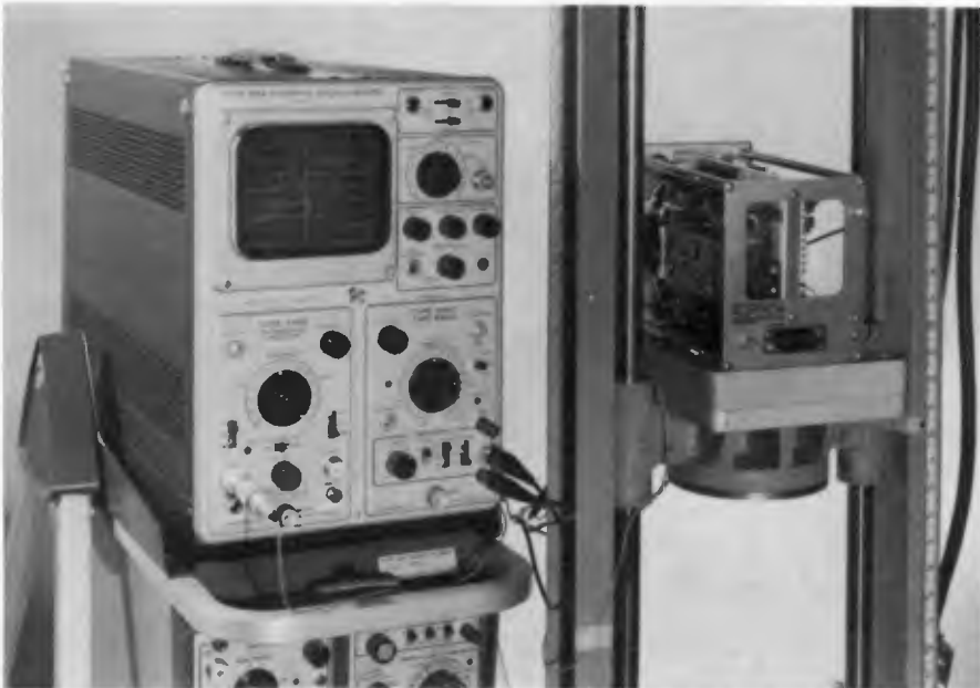
Fig. 22-70F. Tektronix Inc. Model 564 storage oscilloscope, using plug-in differential amplifier and time base.
