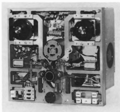
Fig. 17-229I. Interior view of 3M Dynatrack tape recorder with front panel removed.
