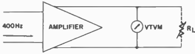
Fig. 23-138A. Circuit that is used for measuring the internal output impedance of an amplifier.
