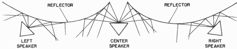
Fig. 20-187. Stereophonic loudspeaker system using two reflectors and a center-derived speaker.
