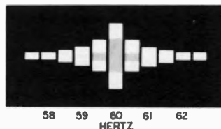
Fig. 22-37D. Appearance of tuned reeds in a Fram frequency meter when actuated by a frequency of 60 Hz.
