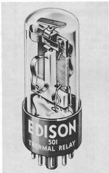
Fig. 25-155A. Interior view of a Thomas A. Edison, Instrument Division Model 501 thermal time-delay relay.
