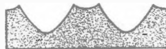
Fig. 13-82. Cross-sectional view of a sound track in a disc record showing the small horns raised at the upper edges by the recording stylus, caused by cold flow in the recording medium.
