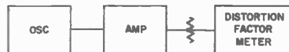
Fig. 22-129B. Block diagram of the method of measuring harmonic distortion of an amplifier.
