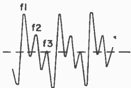
Fig. 23-172B. Resulting complex waveform when three oscillators are connected in series. Frequency f_1 is the fundamental; f_2 and f_3 are the second and third harmonics.
