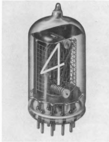
Fig. 25-25B. Interior view of cold-cathode readout tube Model NL-803 manufactured by National Electronics Inc.
