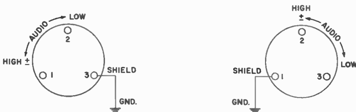
Fig. 4-95. Pin count used on microphone cables.
