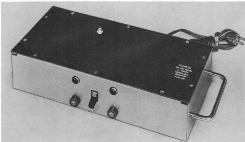
Fig. 17-65A. A magnetic tape or film bulk eraser manufactured by the Hallen Corp.
