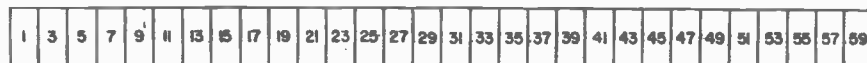
Fig. 2-131F. Playback with a compression ratio of 50 percent. Every 2nd section is omitted.
