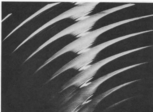
Fig. 16-49A. A typical light pattern of a sweep record. The pattern shown covers a frequency range of 50 to 12,000 Hz repeated 20 times per second using the standard RIAA reproducing characteristic.
