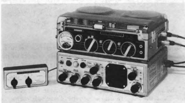
Fig. 3-84C. Kudelski Nagra III and Model SLO resolver, with Variator manual control at left.
