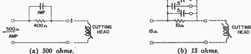
Fig. 14-21B. RC networks used with nonfeedback cutting heads to maintain a constant-amplitude, constant-velocity frequency characteristic.
