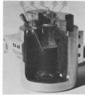
Fig. 14-2D. Cutaway view of Neumann Model SX-45 stereophonic cutting head showing the interior construction. (Courtesy, Gotham Audio Corp.)
