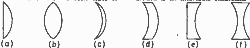
Fig. 19-7. Basic lenses. (a) Plano-convex. (b) Double-convex. (c) Converging concavo-convex. (d) Diverging concavo-convex. (e) Plano-concave. (f) Double-concave.
