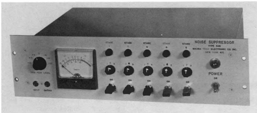
Fig. 18-104B. Magna-Tech Model 34B, solid-state background-noise suppression amplifier.
