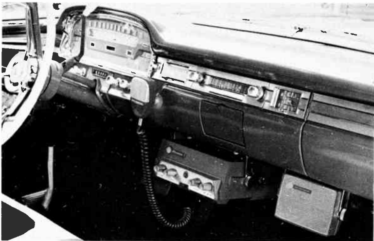
Fig. 1-12. A transistorized GE dash-mounted two-way radio.
