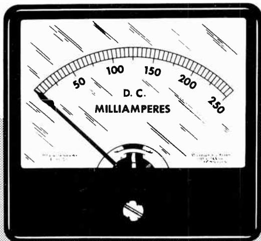
Fig. 5-1. A meter calibrated in milliamperes.
