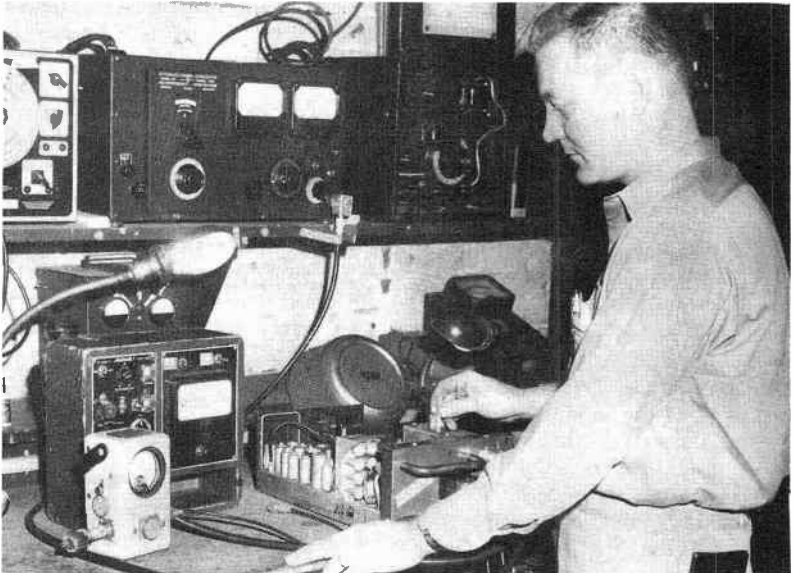
Fig. 10-30. Using a "thru-line" type of RF wattmeter. (Photo by Jacques Saphier.)
