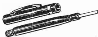
Fig. 9-29. Contact burnisher for cleaning relay contacts. (Courtesy of P. K. Neuses, Incorporated.)
