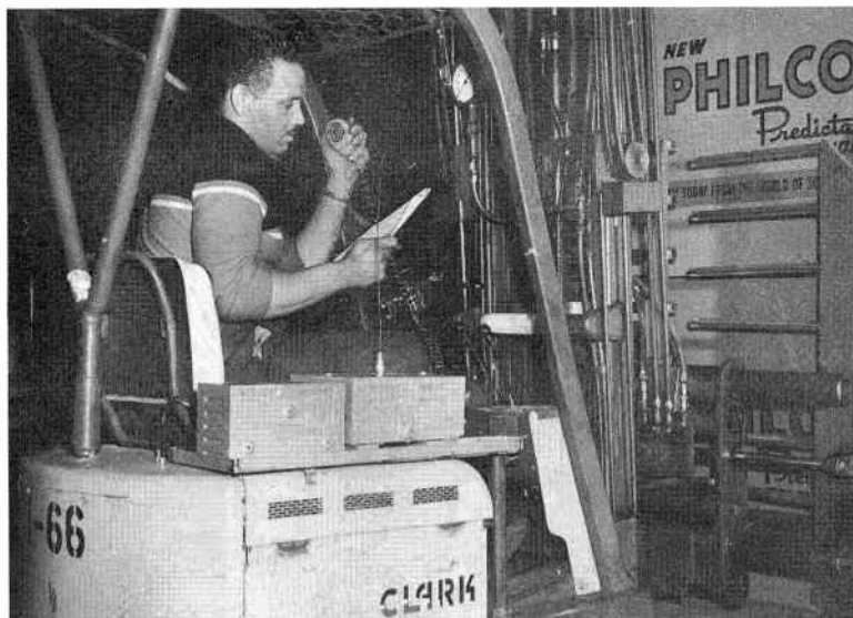
Fig. 8-40. Mobile radio installed on a fork lift truck. (Courtesy of Kaar Engineering Corp.)
