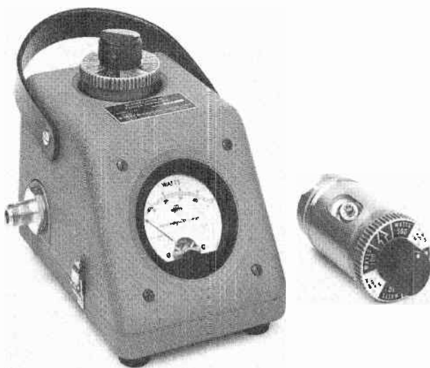
Fig. 9-23. RF wattmeter for measuring transmitter power output. (Courtesy of Sierra Electronic Corp.)
