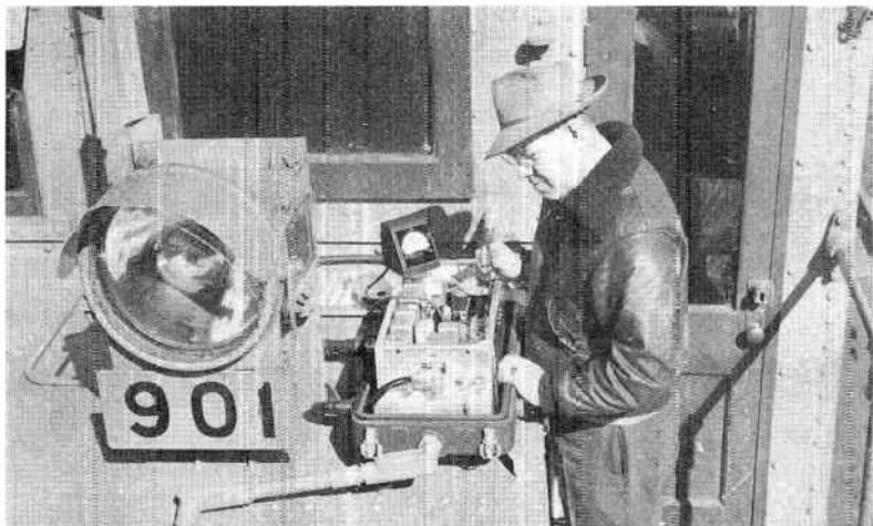
Fig. 5-34. Metering jack and switch on chassis of this railroad radiotelephone allows selection of circuits to be measured. (Courtesy of Chicago, South Shore & South Bend Railroad.)
