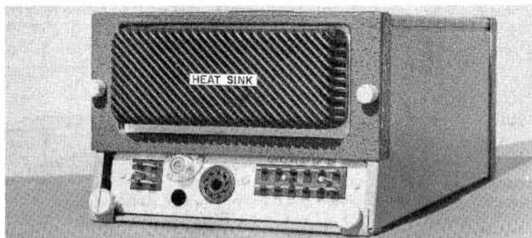
Fig. 8-26. Heat sink on a transistor power supply. (Courtesy of Allen B. DuMont Laboratories, Inc.)
