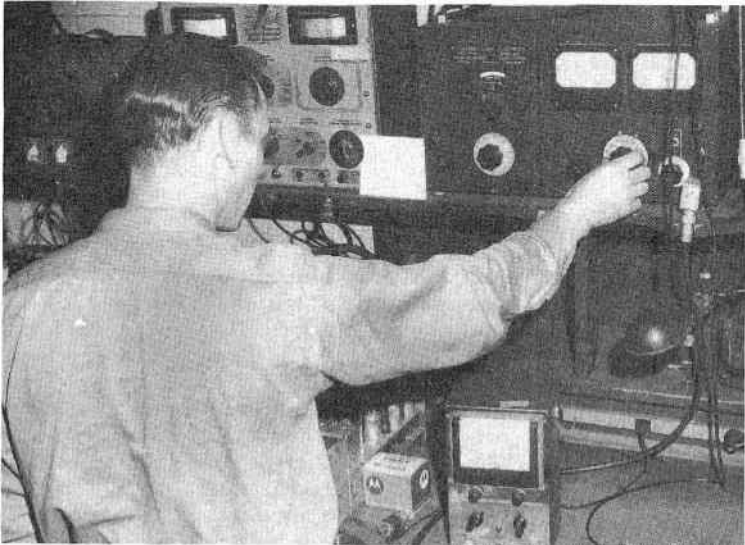
Fig. 10-34. This signal generator delivers a signal between 5 and 475 mc. (Courtesy of Mobile Communications.)
