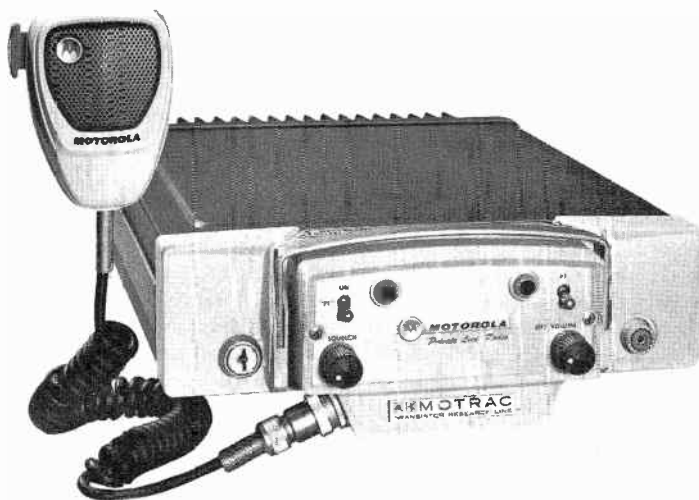
Fig. 9-11. A mobile unit with all controls on the front panel. (Courtesy of Motorola Communications and Electronics, Inc.)
