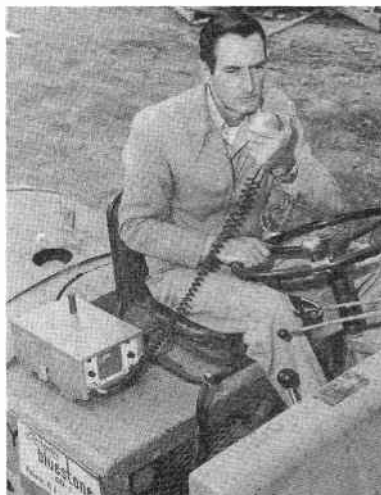
Fig. 1-8. Low-power radiotelephone. Can be licensed in the Business, Manufacturers, or Citizens Radio Service. (Courtesy of Kaar Engineering Corporation.)
