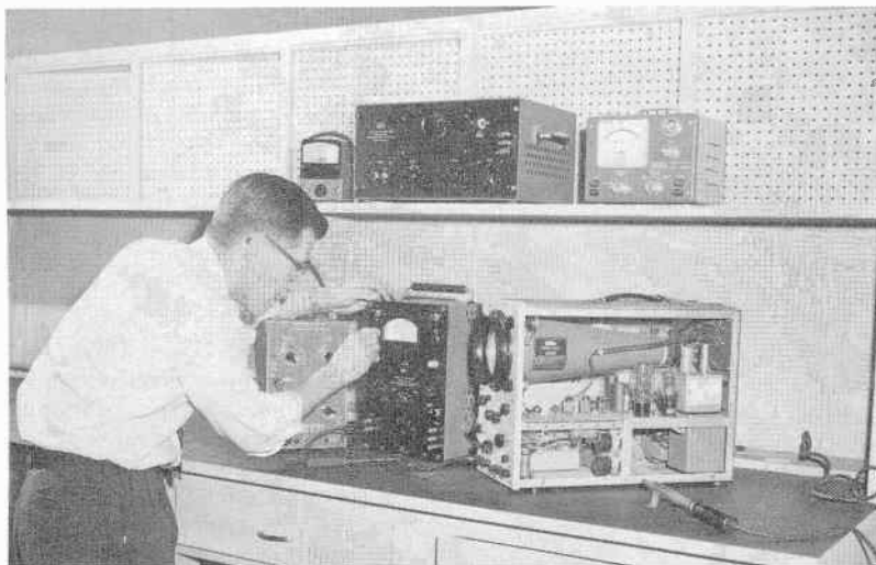
Fig. 10-10. A shelf above the bench is handy for test equipment. (Courtesy of Ault Associates.)
