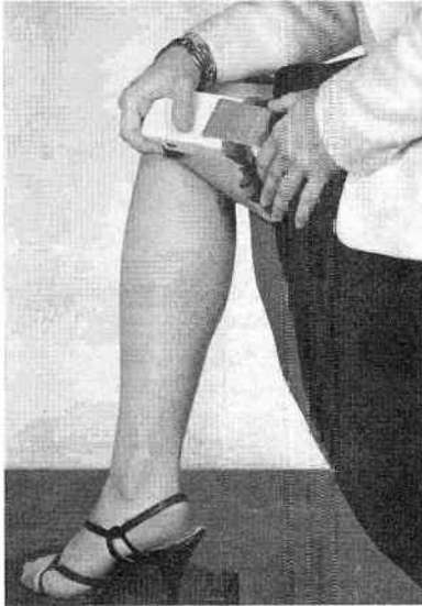
Fig. 1-12. Selective "beep" receiver that can be easily concealed by strapping it to the user's leg. (Photo by Ronald Ambler.)
