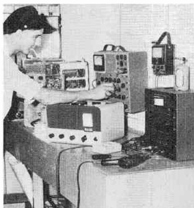
Fig. 10-12. Pegboard behind the bench permits test equipment to be suspended within reach. (Courtesy of Freepoint Communications, Inc.)
