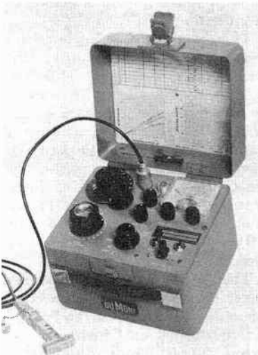
Fig. 10-20. DuMont Model 5890 frequency meter. (Courtesy of Allen B. DuMont Laboratories, Inc.)
