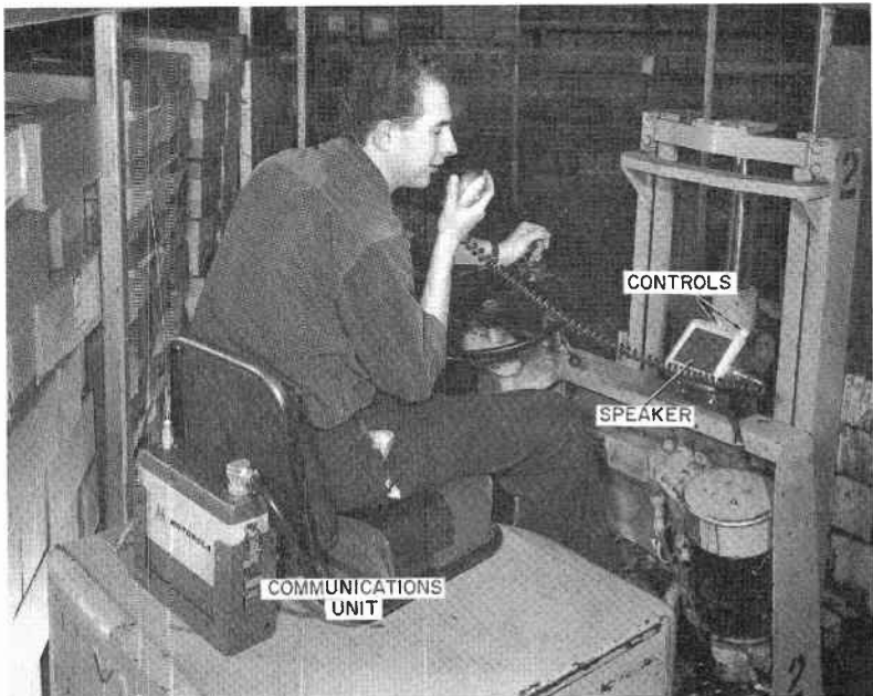
Fig. 1-1. Mobile unit on board a fork-lift truck. (Courtesy of Motorola Communications and Electronics, Inc.)
