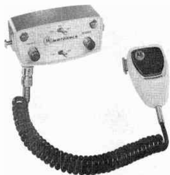
Fig. 9-12. Control head and mike for remote control of a mobile unit. (Courtesy of Motorola Communications and Electronics, Incorporated.)
