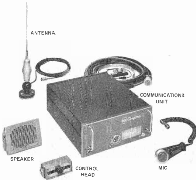
Fig. 1-2. Basic components of a mobile unit. (Courtesy of Radio Corporation of America.)
