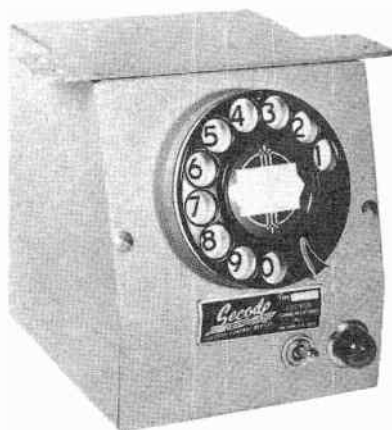
Fig. 6-21. Under-the-dash mobile dial code sender. (Courtesy of Secode Corporation.)
