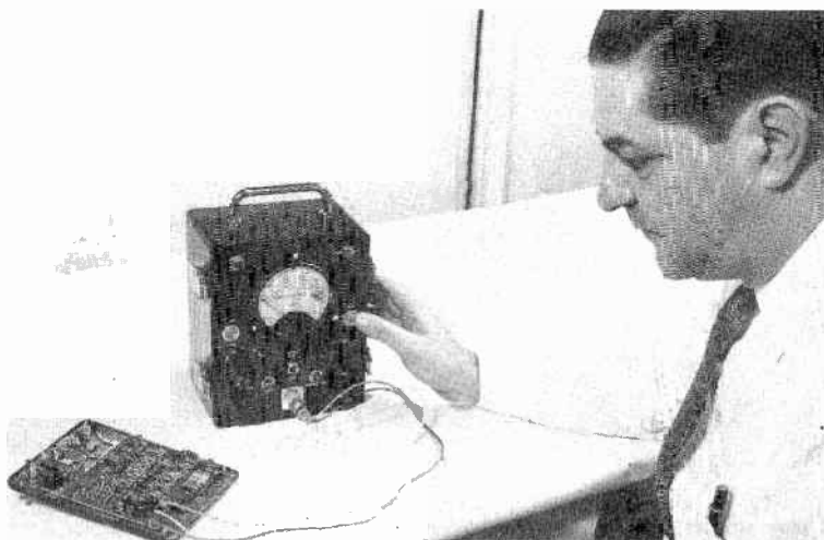
Fig. 10-14. In-circuit transistor tester. (Courtesy of Philco Corporation.)
