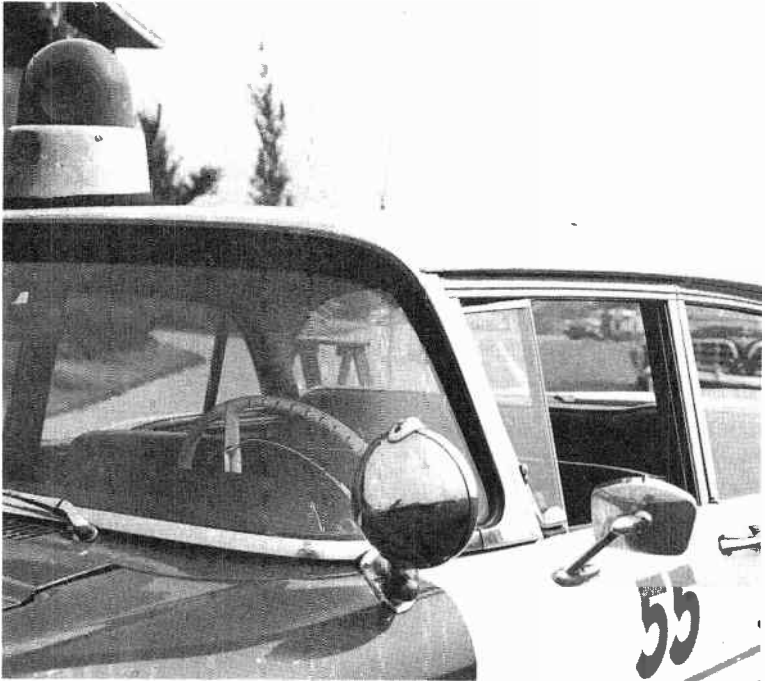
Fig. 7-14. Vertical 18-inch whip antenna is most commonly used for the 152-174 mc band.
