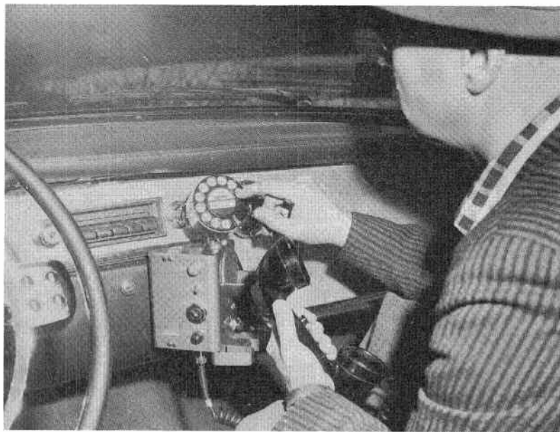
Fig. 1-13. A two-way dialing system installed in an automobile. (Courtesy of Secode Corporation.)
