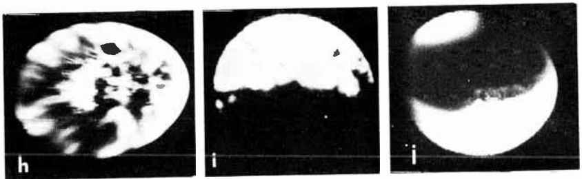
Figs. 722-h,-i,-j. These photos of the scanning spot indicate that a large area of the picture-tube cathode is dead. The dark shadows mean loss of cathode emission. The scanning spots are also severely distorted.
