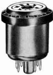
Fig. 301. Test adapter for making above-chassis voltage checks. Adapters for seven- and nine-pin miniature tubes are commercially available.
