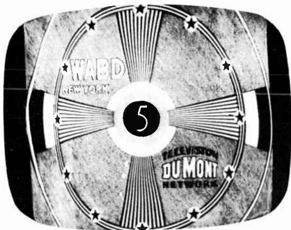
Fig. 305. Photo of test pattern indicates insufficient width.
