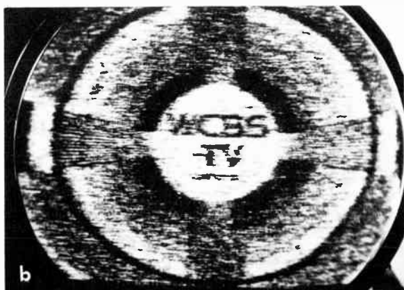
Fig. 409. (a). Weak picture with snow present. (b) Effect of advancing the contrast control setting with a snowy picture.
