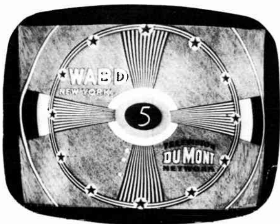
Fig. 308. The test pattern is pulled in. The photo shows inadequate width and height.
