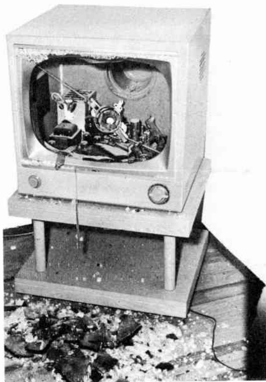
Fig. 102. Result of a cathode-ray implosion due to inadequate safety precautions.
