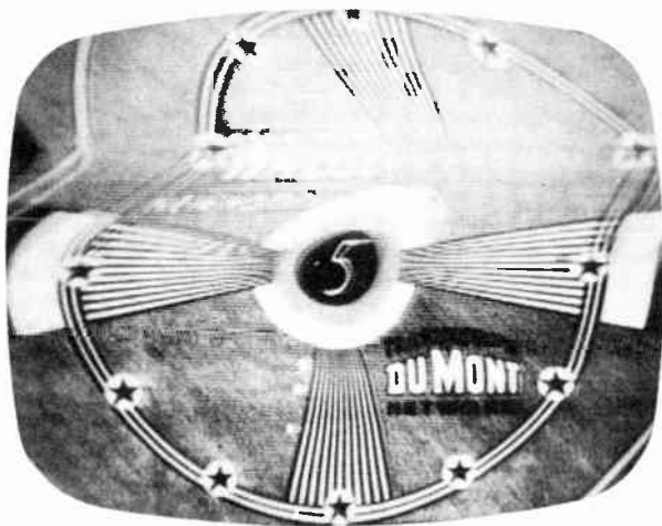
Fig. 507. A case of severe picture "hook" in the test pattern.
