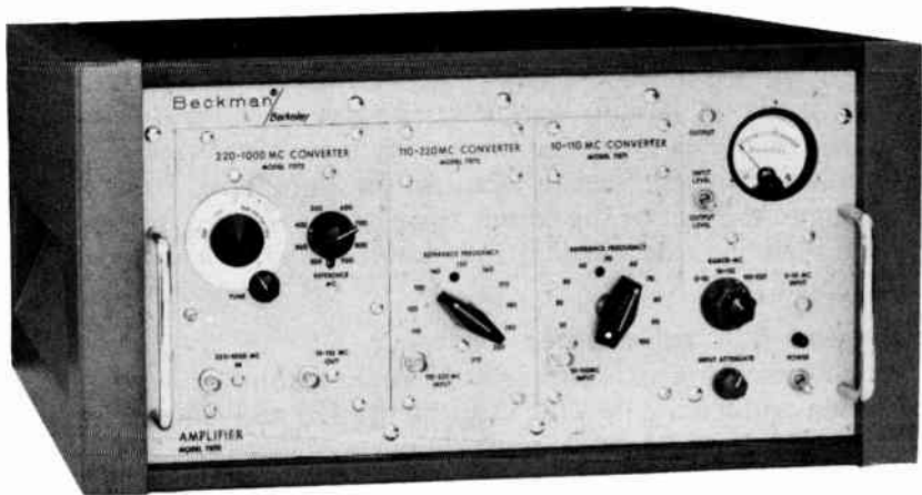
Fig. 604. It is necessary to heterodyne a high frequency that is not within the frequency range of a counter. Stable oscillators can be included in the same case. (Beckman, Inc.)
