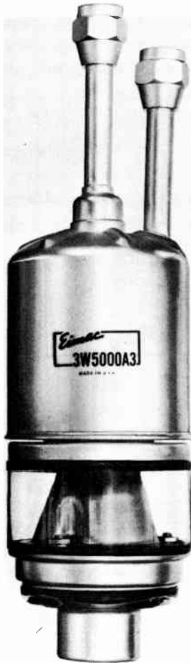
Fig. 207. Water-cooled tubes have been rated as low as 1,000 watts while air-cooled types have exceeded 20,000 watts. Water-cooled tubes, though, are often used in the range of 10 kw or more.
