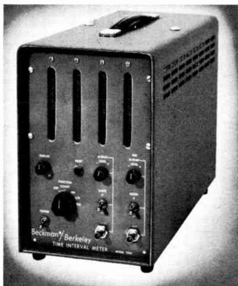
Fig. 504. One form of counter is called a time interval meter . (Beckman Div. Berkley Inst.)
