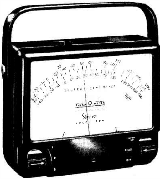
Fig. 1207. This millivoltmeter is calibrated for direct readings of Fahrenheit and Centigrade temperature measurements with the proper thermocouple. (Simpson Electric Co.)
