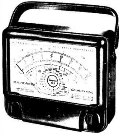
Fig. 1203. The 100,000-ohms-per-volt sensitivity of this instrument allows it to be used for tests that would normally require a vtvm. (Simpson Electric Co.)
