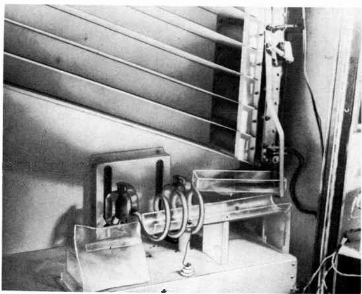
Fig. 314. Frankfurters are cooked rapidly by a dielectric generator in this vending machine. Hot dog slides on plastic guide through the coil of the generator.
