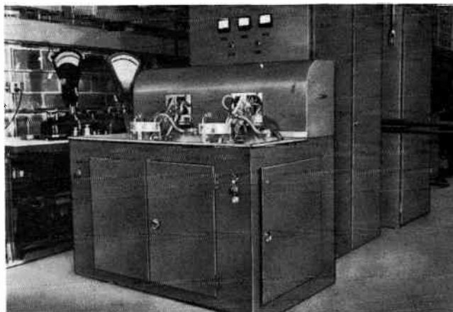
Fig. 307. A 25-kw induction heater is used to harden valve stems. (General Electric Co.)
