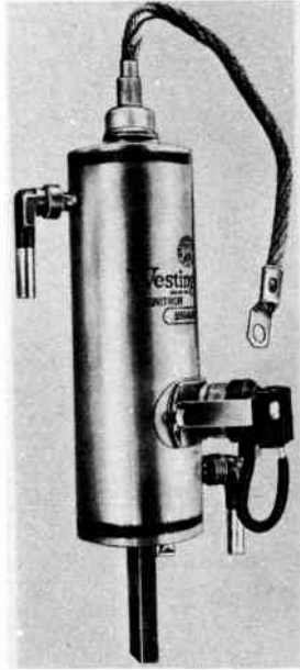
Fig. 209. Heavy current applications call for the ignitron, the big brother of the thyatron.
