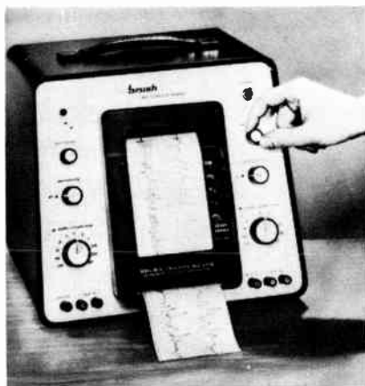
Fig. 1009. Dual electronic recorder has both traces on one tape for easy comparison.
