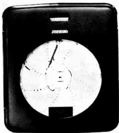
Fig. 1018. Circular chart recorder may cover an hour, day or week, depending on details required for process.
