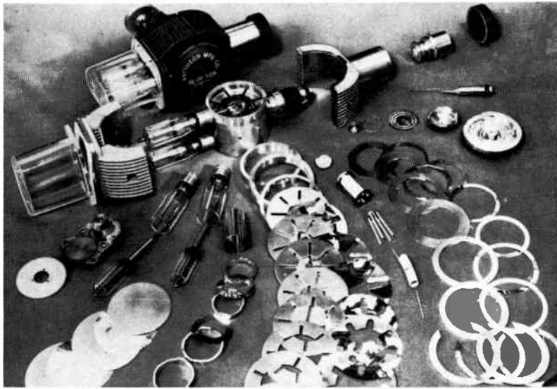
Fig. 211. Magnetron construction is much more complicated than ordinary vacuum-tubes.
