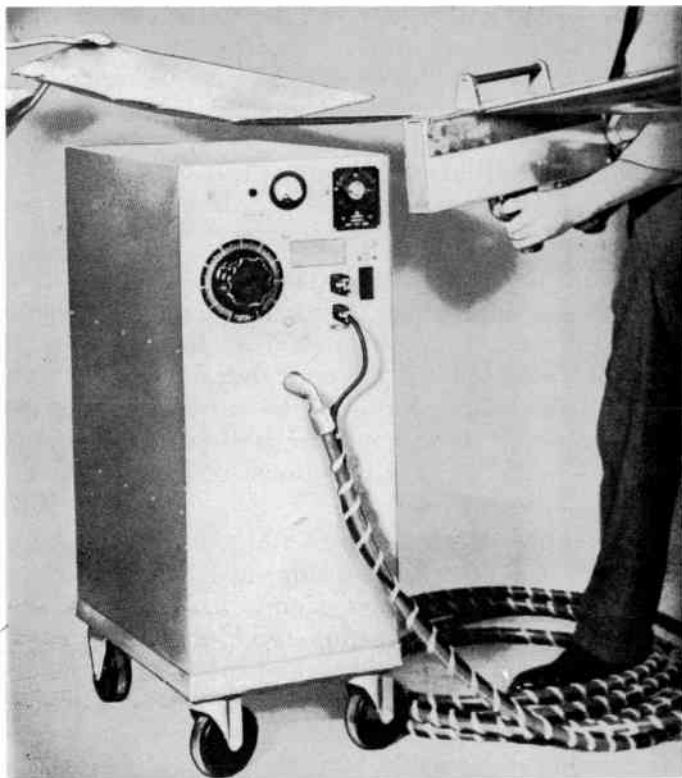
Fig. 311. This impedance-matched generator uses a long cable to take the work head to the job.
