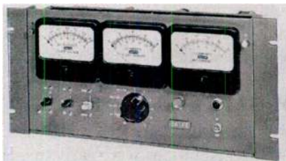
The Gates RDC-10AC like this one was used for years at KOIL and KOIL FM. It's typical of first-generation remote controls, with 10 metering/control channels using stepping relays in the studio and transmitter site.
