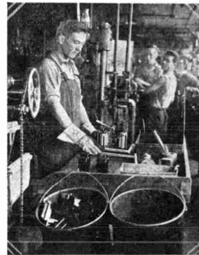
Fig. 3: Removing four Bakelite transformer cases from the die.
