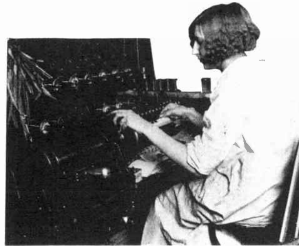
Fig. 3. Automatic coil winding machines turn out thousands of transformer coils each day.
