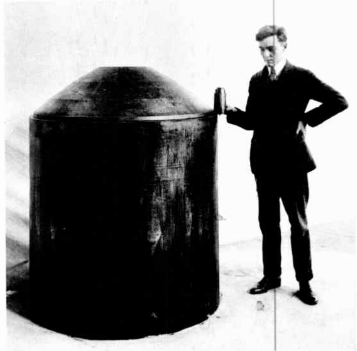
Colin B Kennedy, holding the lower magnet pole of a Federal 2 kw arc transmitter, standing next to a 500 kw pole, about 1919. (photo from Leonard F. Fuller)
