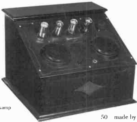
Similar to the Thermiodyne TF6, but the tuning condensers are coupled in two pairs, rather than all four together.
