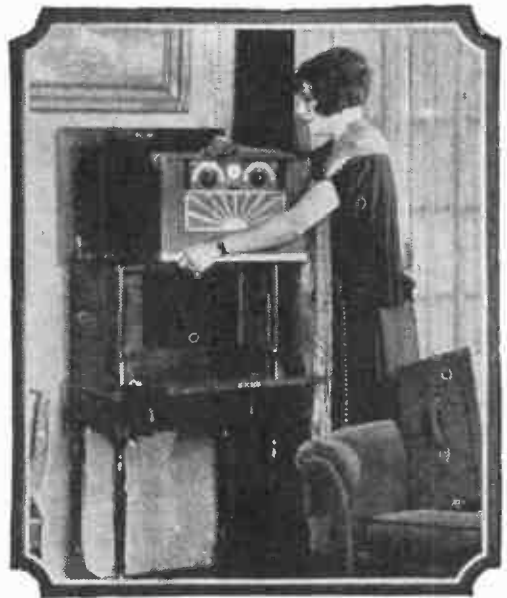
Removing the set from the cabinet. A separate cover (containing loop aerial or wave-bridge) is applied to the case—and the set becomes a smart-looking piece of hand-luggage.
