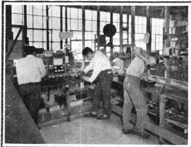
Final test and inspection. Every Neutrowound Set is tuned on at least three stations before being shipped.
