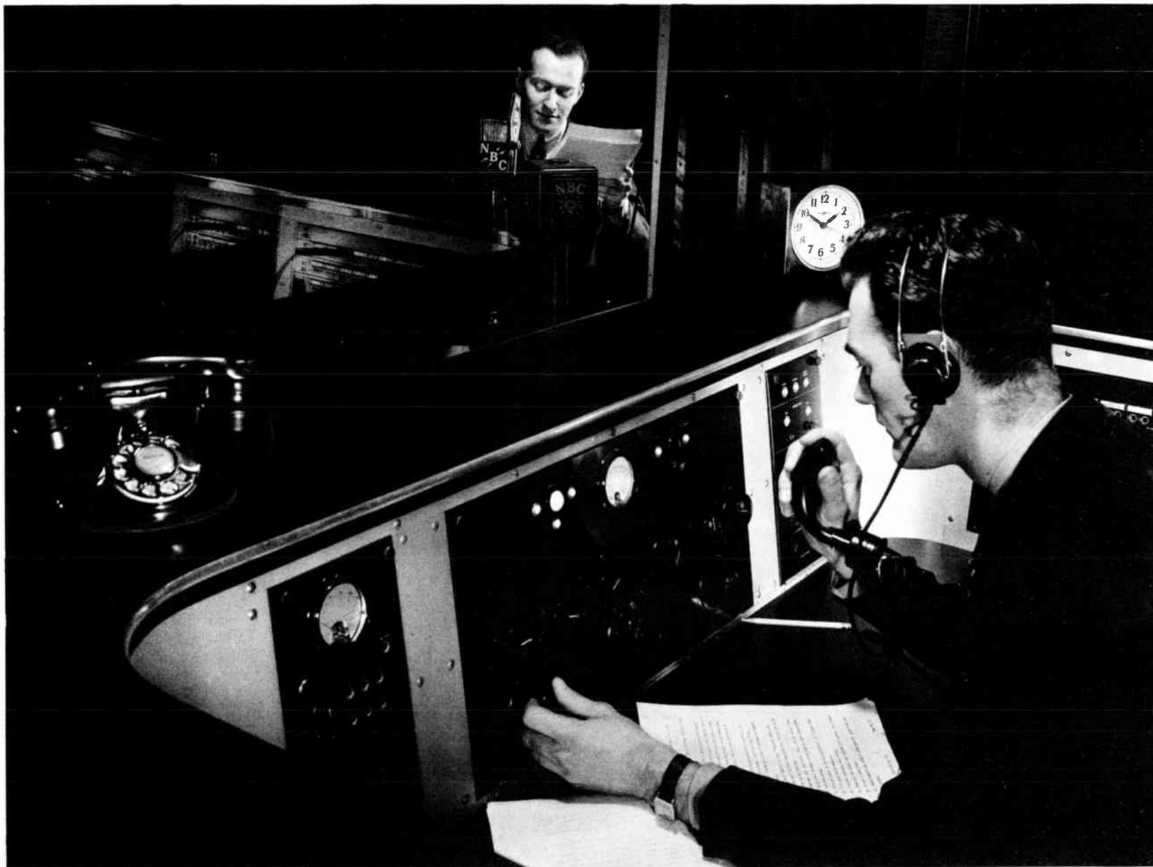
*Through the looking glass. The announcer is seen through the Studio Control Room window—reading his script into the microphone while the engineer contacts the Master Control Room by phone.*
